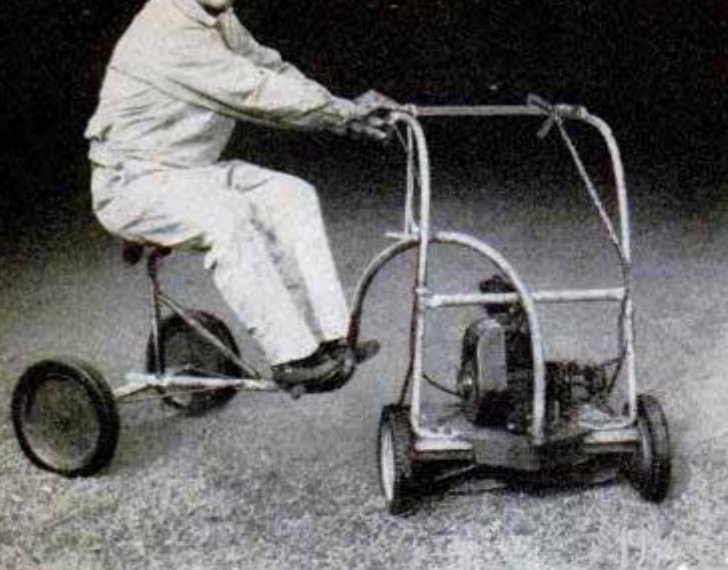
The lawn mower-trailer unit can be made to turn in its own length, an essential feature when mowing around flower beds and in irregularly shaped plots
