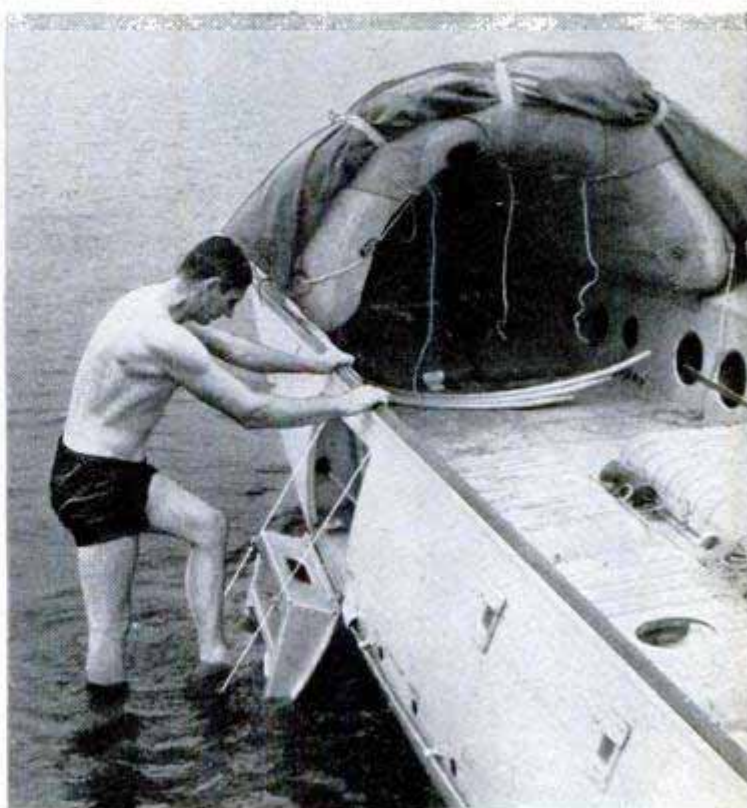
Above, engine is mounted below deck of the craft and can be entirely controlled by unit in hands of engineer. Or, if the passengers are too weak, the operation can be performed from plane by radio. Below, ladder drops into water for survivors
