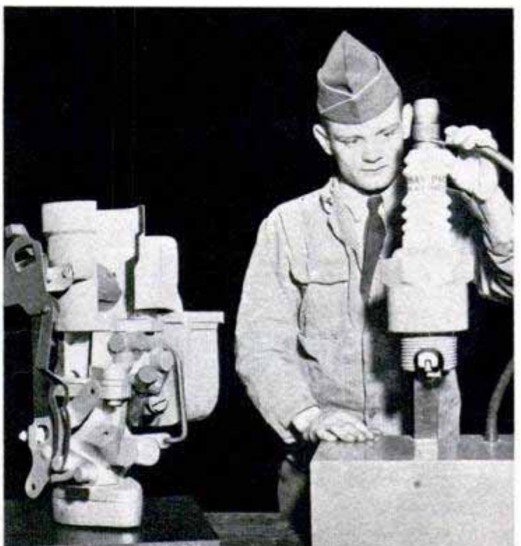
Giant-sized versions of spark plugs and carburetors help GI mechanics understand how an engine runs
