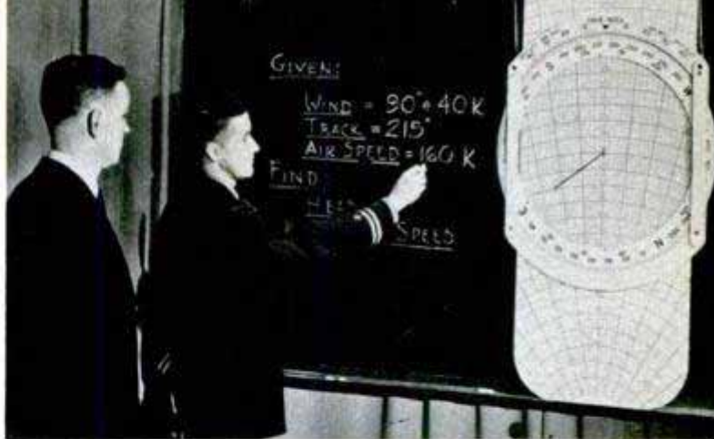
Actual dead-reckoning computer would fit in pocket, but this four-foot model is much easier to explain
