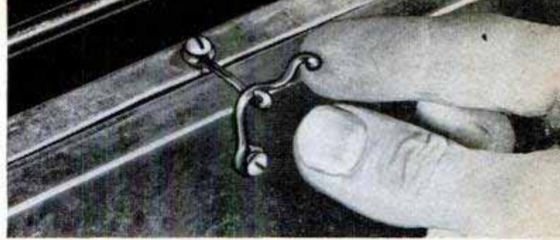
The latch is formed of stiff wire, each part being attached to respective covers with sheet-metal screws
