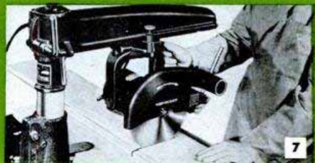
LONG END TO RIGHT is a poor way to operate saw when left hand must hold short cutoff
