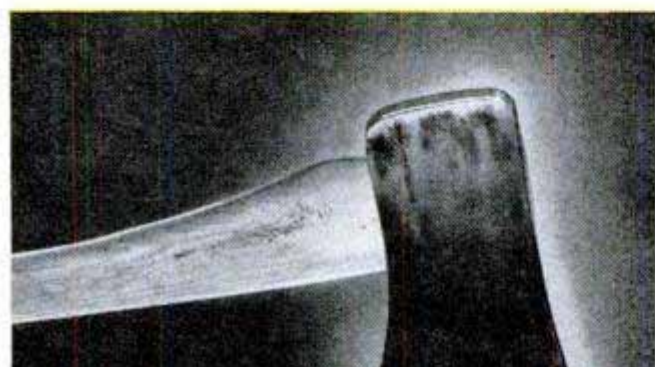
Slot handle for softwood wedge, above. Check fit, below, with ax on edge. End of handle and blade edge \frac{3}{8} from front should touch bench top
