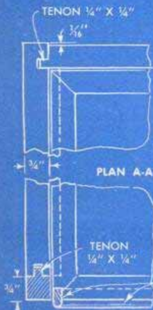
BEAD AROUND DRAWER FRONT, 1/4" X 3/16"
