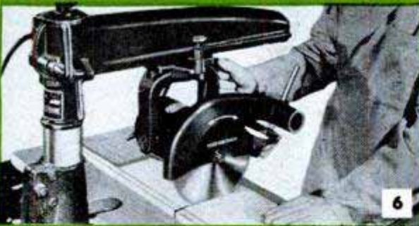
LONG END TO LEFT permits the left hand to hold solid portion of work safely and securely
