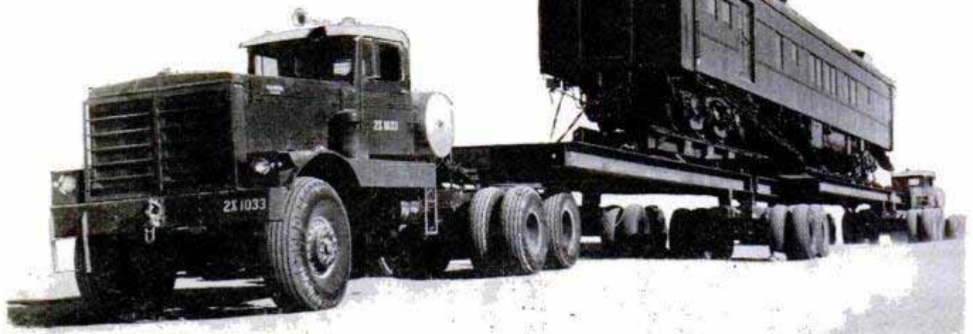
Hospital car converted from a Pullman was trucked across desert in Saudi Arabia to the new railroad
