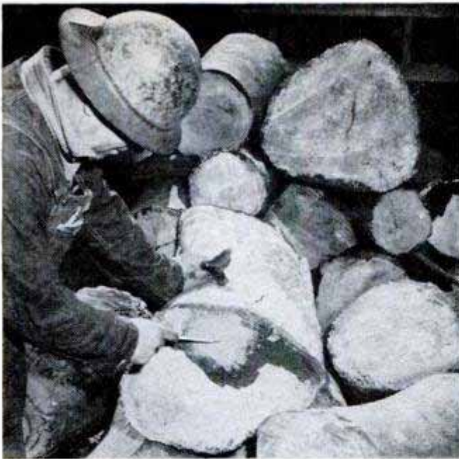
Rock-hard lignum-vitae logs, from which blocks will be cut to form a vital tail-shaft bearing on ship
