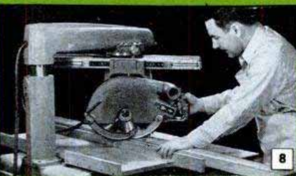
LEFT-HAND MITER is the most comfortable to use on all angle cuts up to approx. 60 deg.
