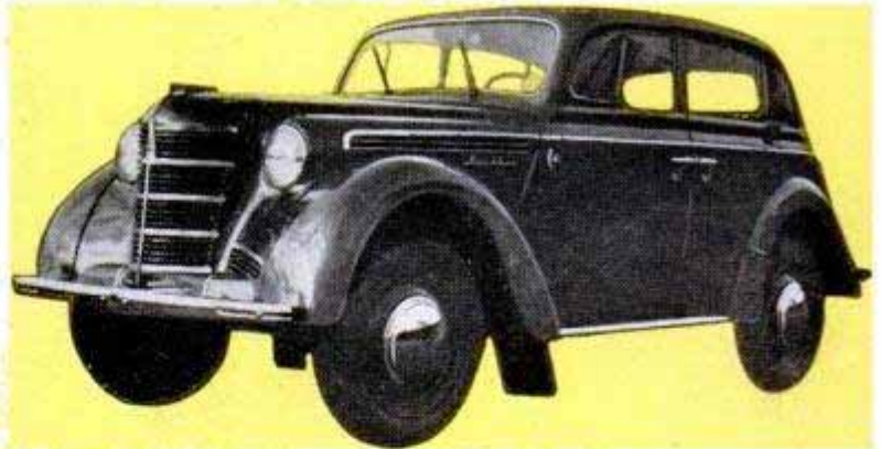
Above, Russian Moskvitch four-door sedan was tested by Clymer in Vienna—a copy of G.M. Opel of prewar vintage
