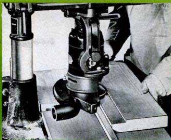
WIDE RABBETS CUT WITH SAW HORIZONTAL
