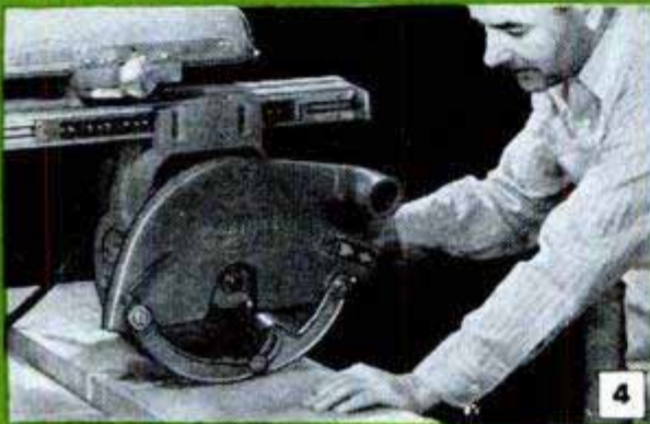
RIGHT-HAND FEED is the natural and practical position for crosscutting most types of work
