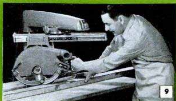
RIGHT-HAND MITER is an awkward position although it is useful in cutting angles over 60 deg.
