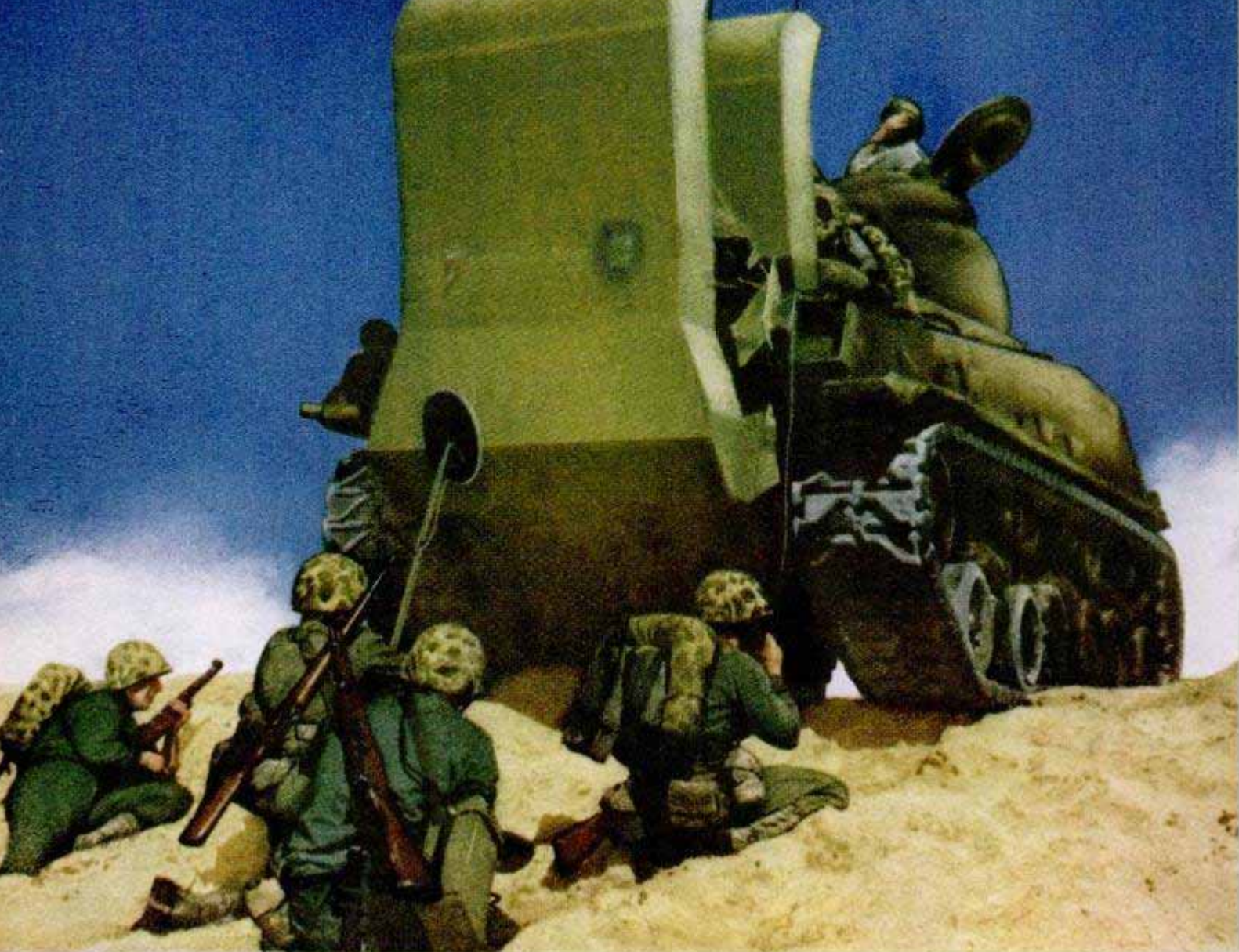
Big tank, equipped with "breathing" apparatus which enables it to ford streams, lumbers across beach supported by ground troops
