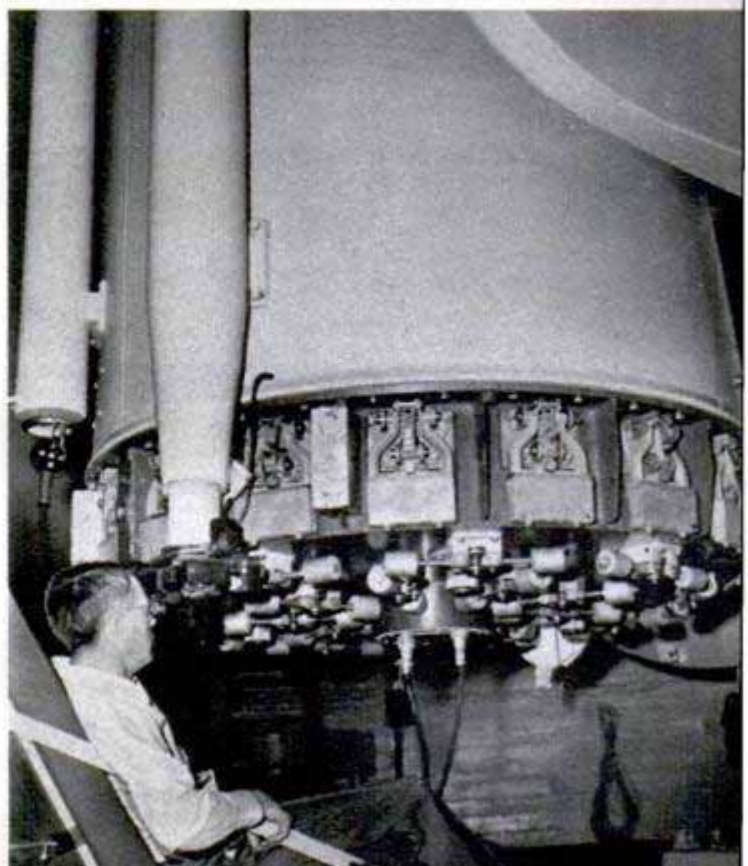
When the Schmidt camera is pointed toward the zenith, the observer can work from an easy chair
