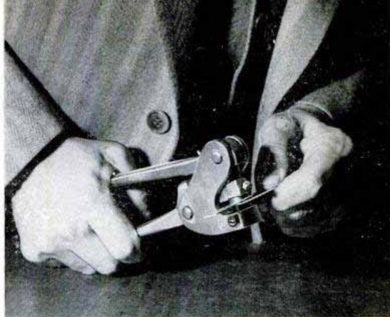
Dies are interchangeable in hand tools, too. These permit metalworker to make various on-the-spot welds
