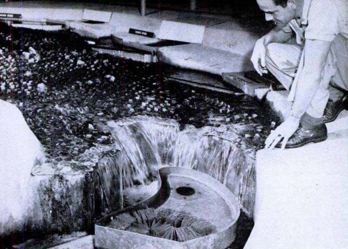
Engineers use a scale model of Niagara Falls to learn how to make better use of its thundering waters
