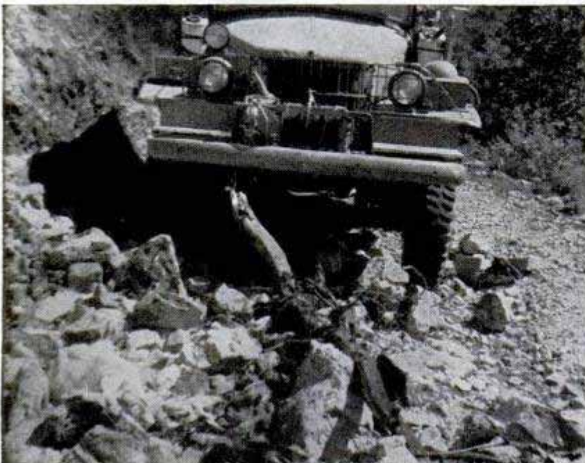
Military tread on tires was a boon to the Russells in traveling over jagged rocks which would have cut ordinary tires to shreds
