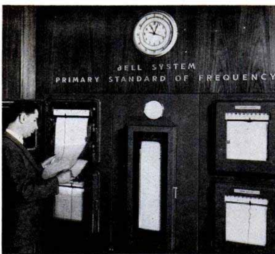
↑ Front of the new frequency-time standard at Bell Telephone Laboratories. In the rear there are 600 electron tubes and 25,000 soldered connections. Room temperature is maintained within two degrees.
