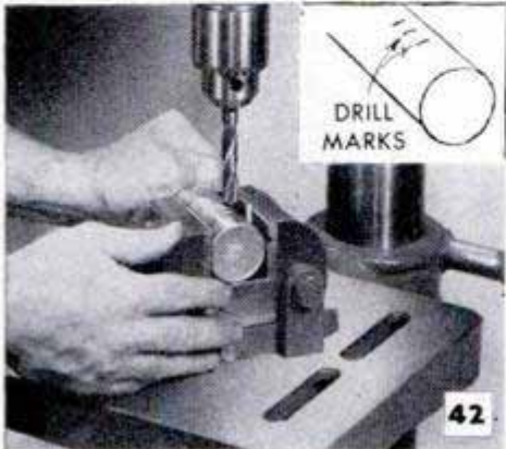
Center of round work is located by sliding work under bit so surface is just scratched, Fig. 42. If angle vise is tilted slightly before drilling, runoff can be corrected by changing of angle vise, Fig. 43. Hole in end of rod is located by drilling clamped block, Fig. 41, and pressing work upright in drilled block, Fig. 44
