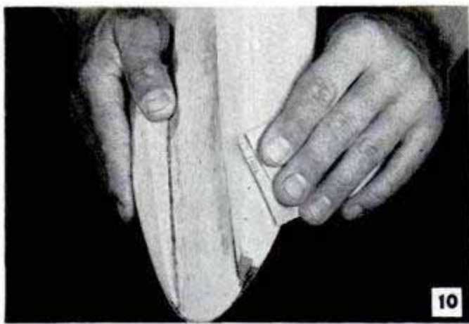
10 Fill all openings at seams with wood putty and sand entire hull, using special care to smooth the sponsons
