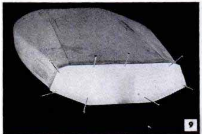
7 Above, use rubber bands and pins to hold sponson strips until cement sets. Below, cut transom to fit over No. 6 bulkhead, coat with cement and pin until dry
