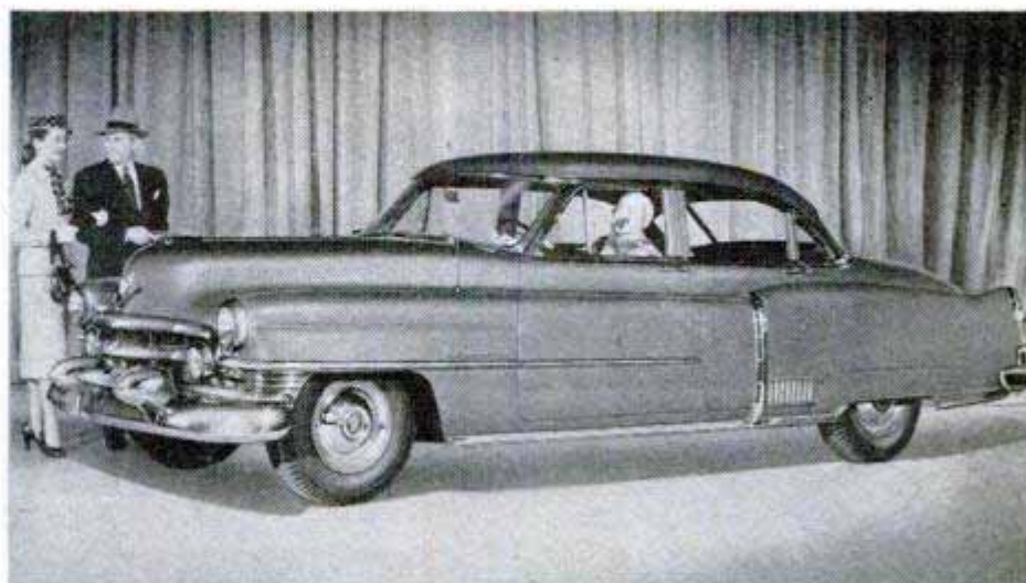
This 1952 Cadillac 60 Special sedan is powered by a new 190-horsepower, V-8 high-compression engine. It has the dual-range Hydra-Matic transmission
