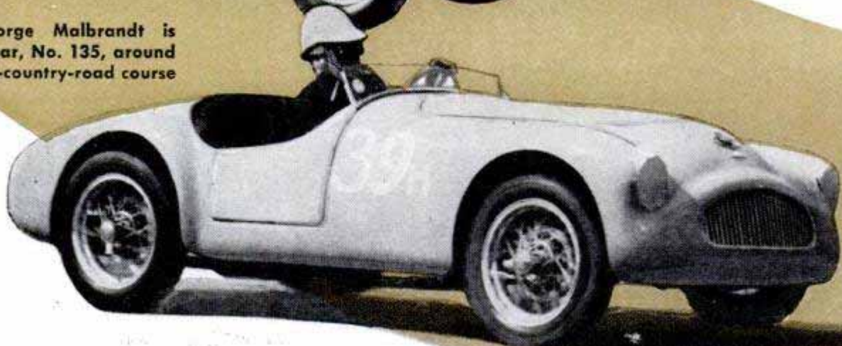
Turning up speeds of 100 m.p.h., the Fiat Siata uses 4.25 by 15 tires, weighs 850 pounds and is powered by a Crosley engine
