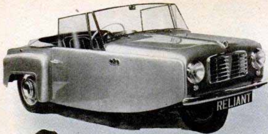
Left, British three-wheel Reliant Regal is a four-seater powered by four-cylinder engine easy on gas
