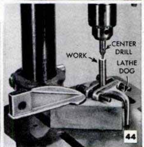
Center of round work is located by sliding work under bit so surface is just scratched, Fig. 42. If angle vise is tilted slightly before drilling, runoff can be corrected by changing of angle vise, Fig. 43. Hole in end of rod is located by drilling clamped block, Fig. 41, and pressing work upright in drilled block, Fig. 44
