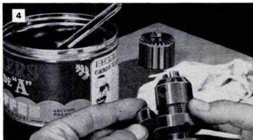
Clean all parts of the disassembled chuck in a clean solvent, using an old toothbrush to loosen accumulations of dirt and hardened grease from moving parts
