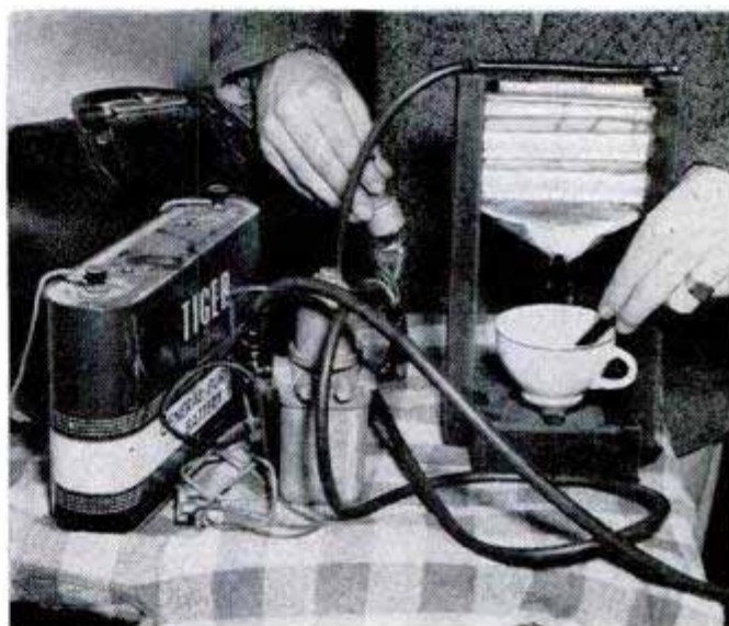
Soup cooler pumps hot liquid from cup to top of the radiator where it drizzles over grid and back to the cup. Below, the "grumplatch" has no known use
