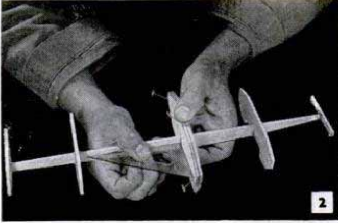
2 Begin construction by cementing the bulkheads to the keel. Check alignment with a triangle or square
