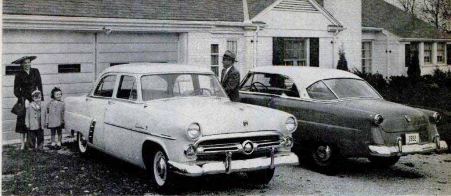
Parked at left of the Victoria, Customline Fordor Sedan features new Ford body with curved one-piece windshield
