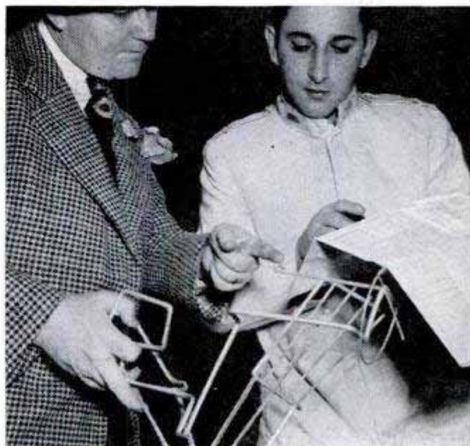
Soup cooler pumps hot liquid from cup to top of the radiator where it drizzles over grid and back to the cup. Below, the "grumplatch" has no known use
