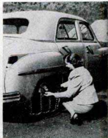
EASY-ON CHAINS eliminate reaching behind wheel to hook inner link because inner band is a rubber hoop, left. Wheel is driven inside hoop, chain lifted over wheel, center, and only outer link has to be snapped
