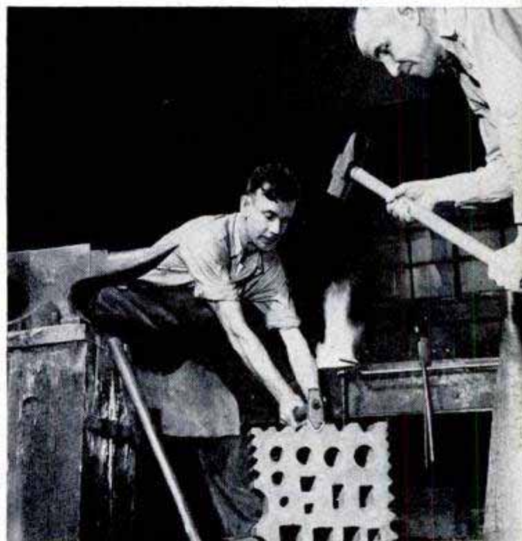
Heavy steel swage block contains variety of shapes into which metal is pounded to form desired contour
