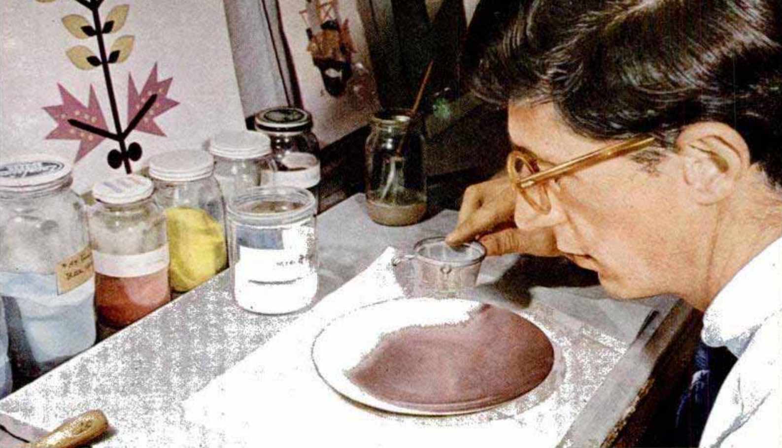
Enamel flux is sifted on gum coat, completely covering plate. Start near edge and work toward center
