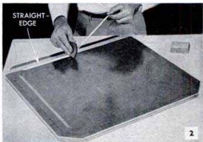
Above, the veneer is squeegeed smoothly to the surface with a soft-rubber block. Below, gold tooling is applied to leather before carrier is peeled off
