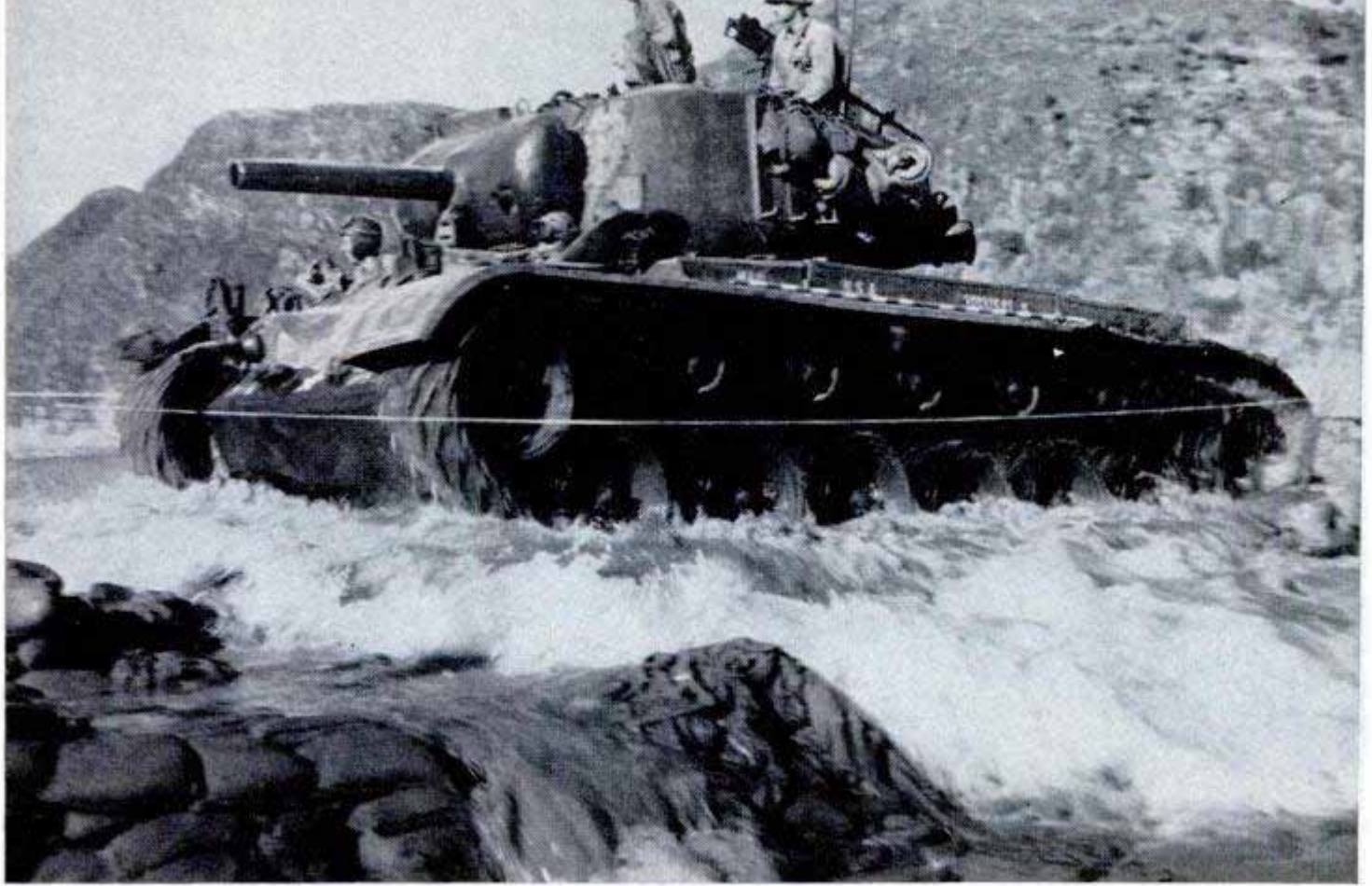
Big tank crosses river in Korea over newest type of "underwater" bridge made of rocks and many sandbags
