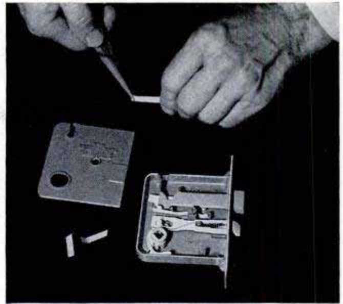
Above, replacing broken lever spring in free-action latch. Long-nose pliers are used to bend new spring
