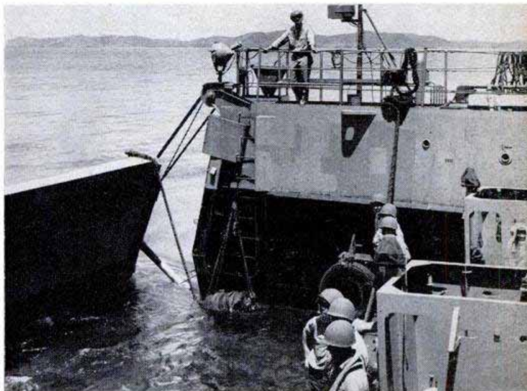
Top right, an LSU swings her blunt nose in through open stern gate of mother ship. Just below, stern gate is partly opened when taking on ballast so sea can rush in; man standing on top deck "talks" boats in
