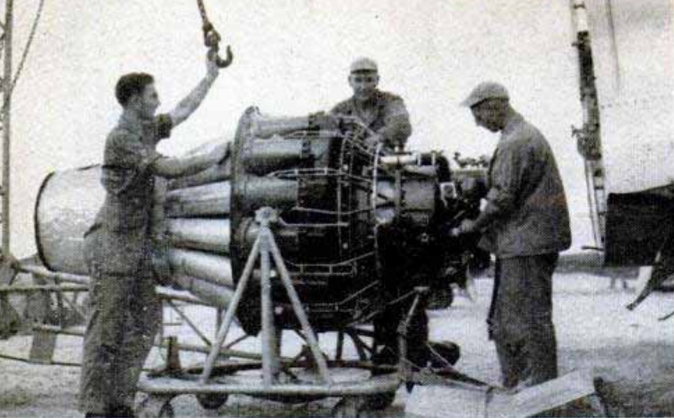
Mechanics hoist a jet power plant back into an F-80 that in a matter of minutes will again be combat-bound against the Chinese Communists
