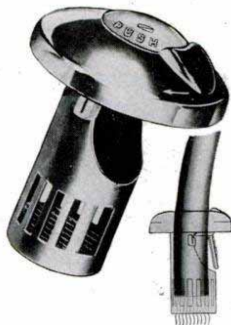
GAS-TANK "WATCHDOG" is screened to prevent siphoning. No key is used. Cover is opened by pushing pump nozzle into it
