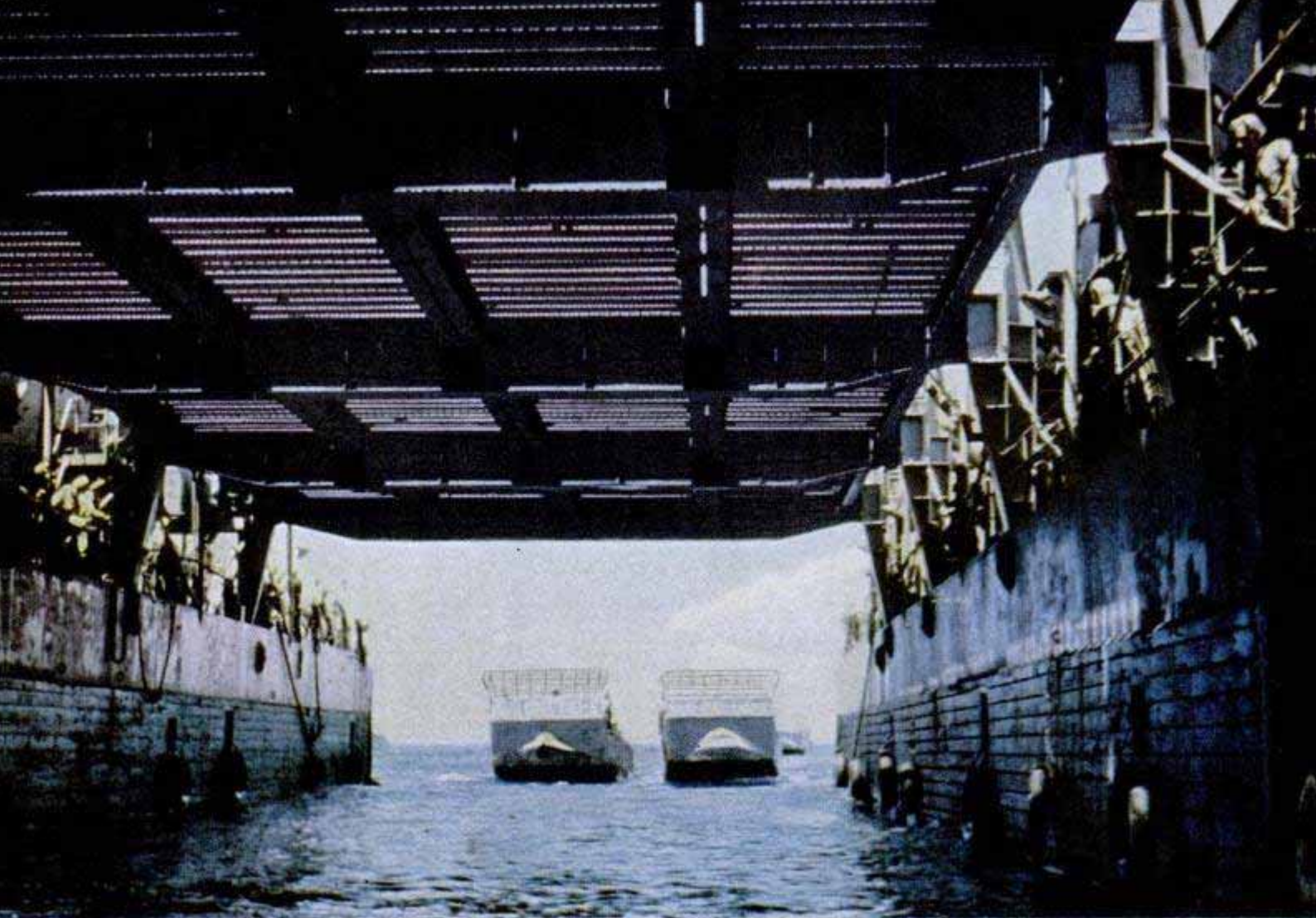
Small craft edge their way into the mother ship; the superdeck is made of removable sections of steel grating
