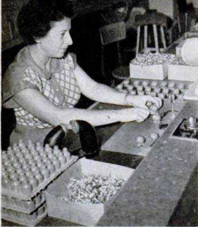
Looking like bonbons in a candy factory, the tiny motors are tested and "run in" until the drain and speed remain constant before they are shipped out
