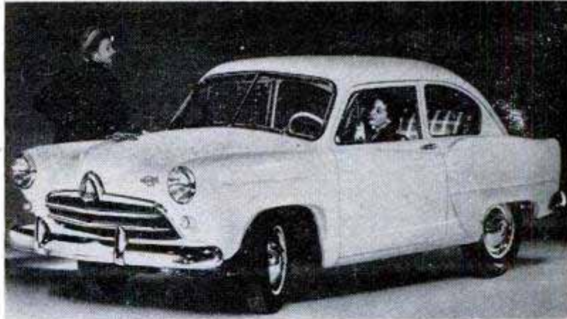
Sears' Allstate, with four or six-cylinder engine, is upholstered in plastic fabrics. Overdrive is optional equipment
