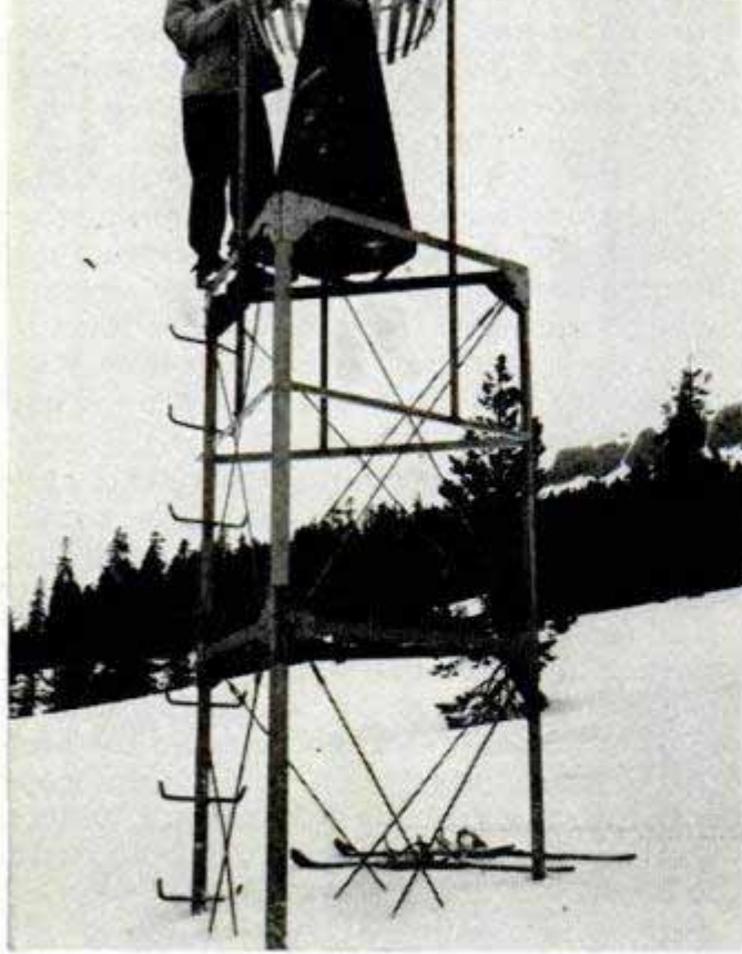
Located around the test valley are snow gauges that collect the snow so the total fall can be measured
