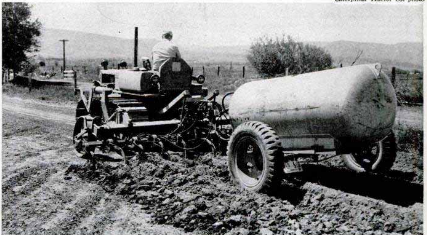
Caterpillar diesel, with attachments, applies gas fertilizer as it cultivates at rate of five acres per hour Caterpillar Tractor Co. photo
