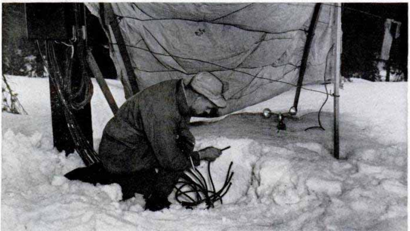
Electrical-resistance thermometers take readings at various levels under snow. Canvas screens off solar heat
