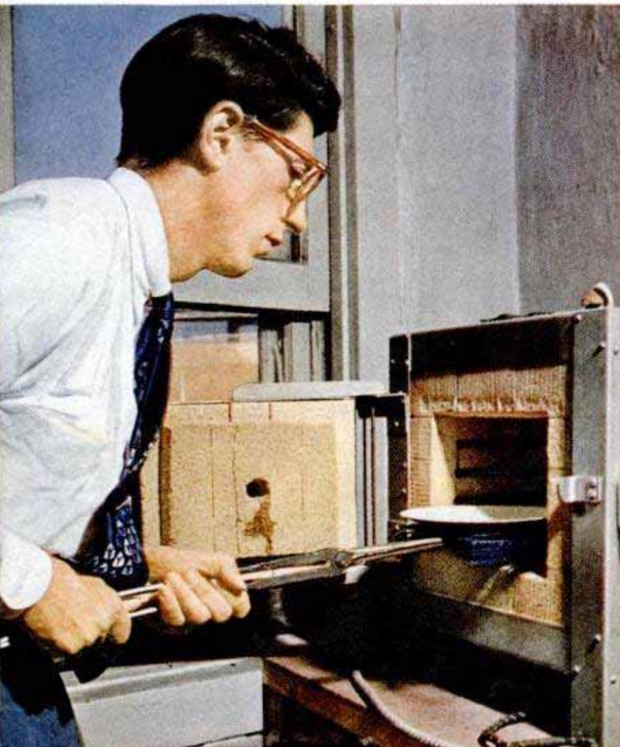
Below, a long pair of iron tongs is used to insert and remove the prepared plate from the furnace or kiln. Plate rests on grille of chrome-nickel mesh or wire to facilitate handling
