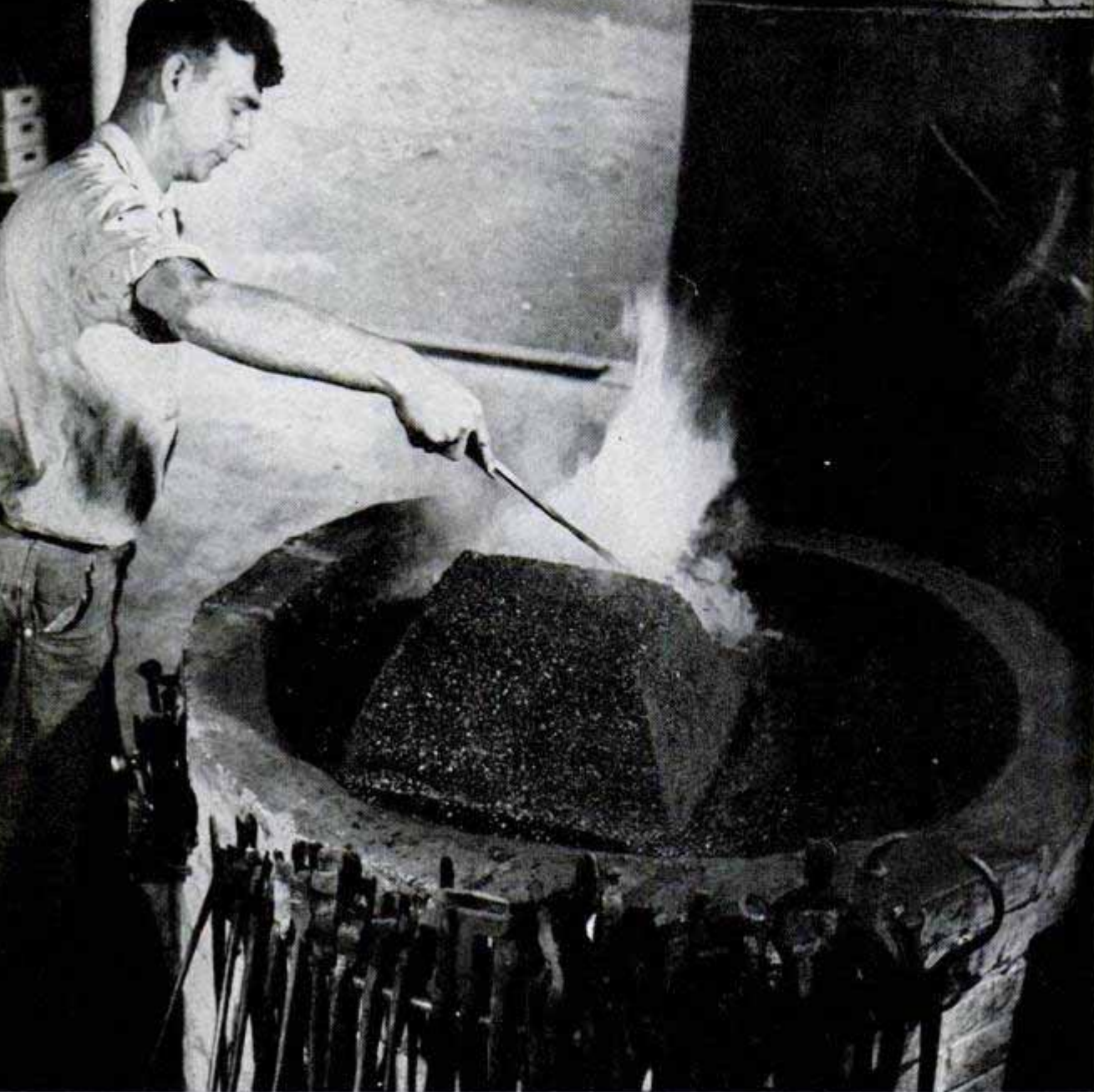
Daniel Boone the Sixth piles coal on the forge in a truncated-pyramid shape as did his ancestors
