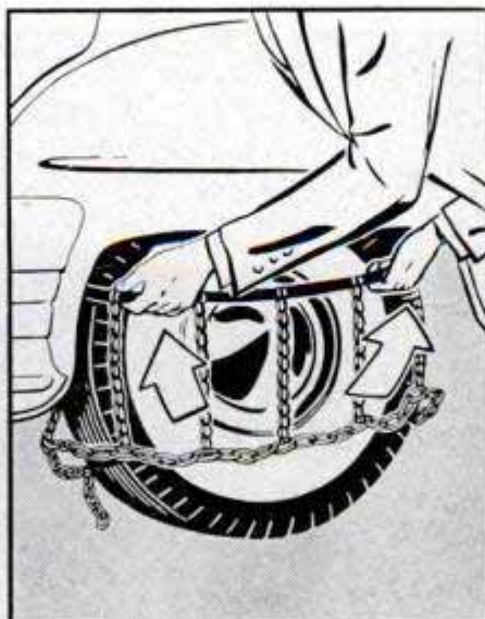
EASY-ON CHAINS eliminate reaching behind wheel to hook inner link because inner band is a rubber hoop, left. Wheel is driven inside hoop, chain lifted over wheel, center, and only outer link has to be snapped
