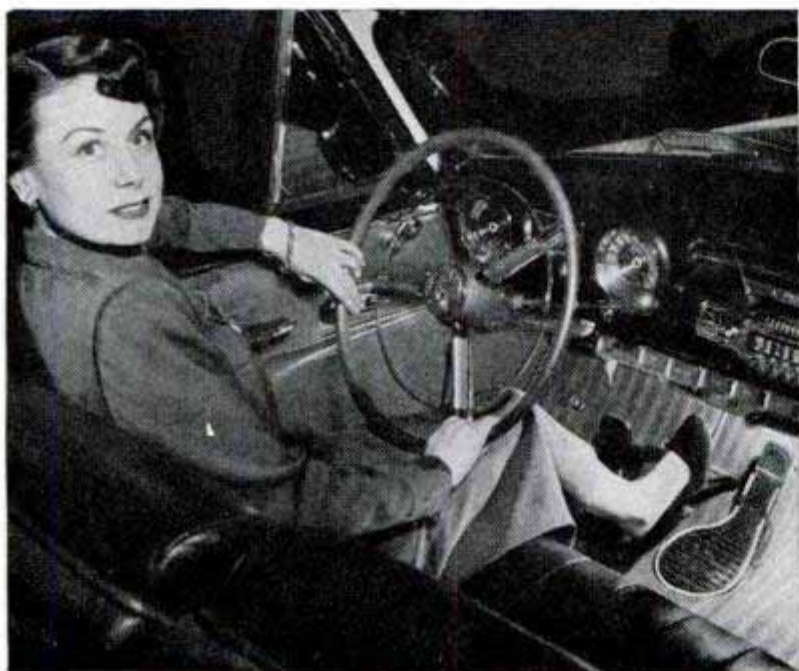
HEEL MAT slips over accelerator pedal to provide a "pillow" for the heel that stops shoe scuffing. Made of rubber, it is put on without tools. It prevents wear on the floor mat, too
