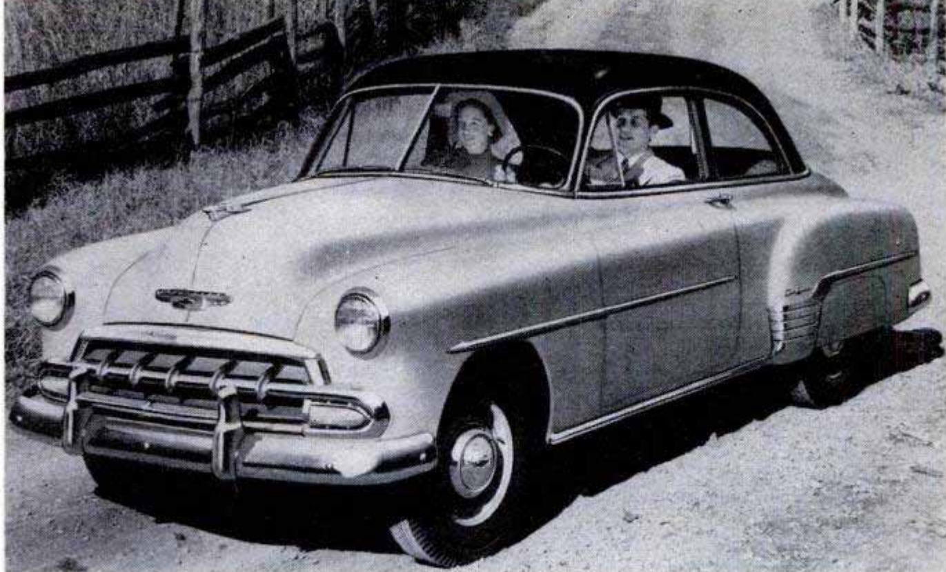
Two-door Styleline Chevrolet shows redesigned grille. Optional Powerglide models will have automatic choke
