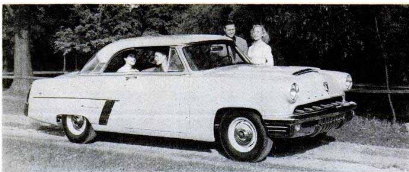
Mercury's Monterey hardtop convertible, above, has wider windshield, lower hood and raised fender crowns. Following the same lines is Lincoln's Capri hardtop convertible, below, with new 160-horsepower V-8 engine
