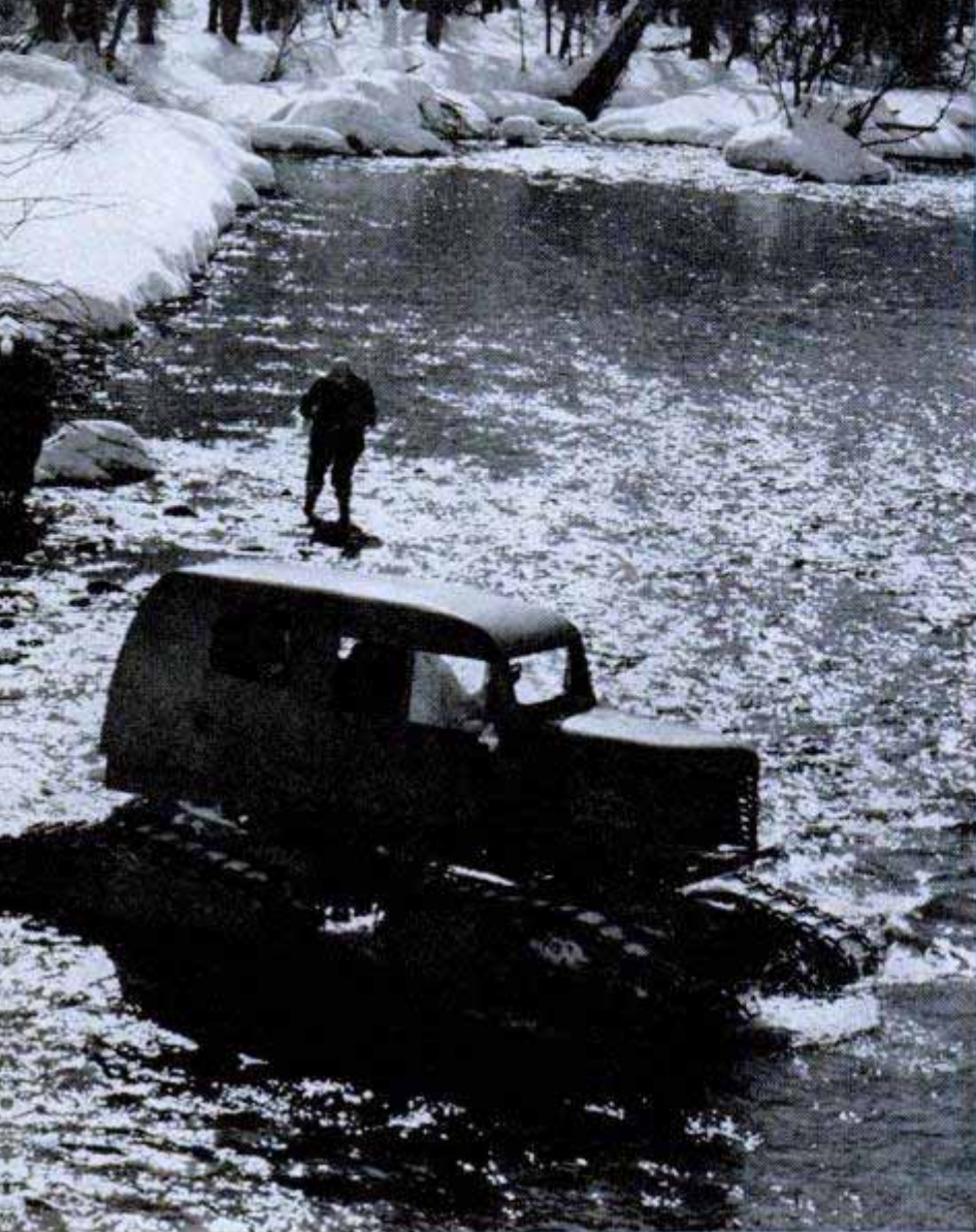
Nothing fazes this vehicle. Its snow tracks wrap around four pontoons that float it across rivers Dept. of Agriculture Soil Conservation photos
