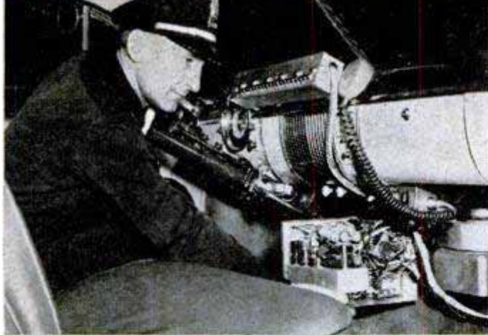
Left, the control device for the test speedometer is mounted on the dashboard. Right, the speedometer dial
