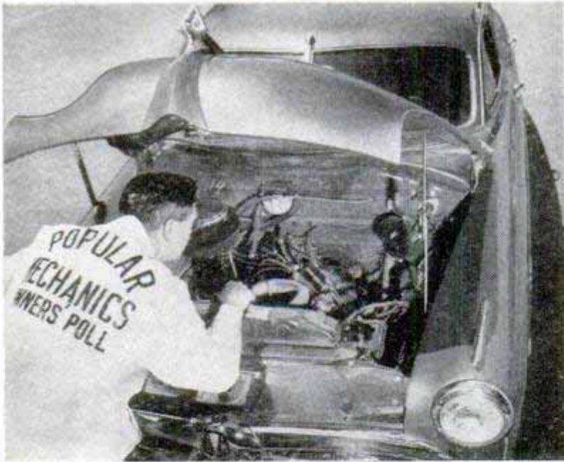
At end of a grueling test, Clymer's Hornet opens its "mouth" as he examines engine that used one pint of oil in 2750 miles
