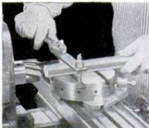
2 HOLDING BAR STOCK FOR END CUTTING is done with milling vise, left. Job is flattening carriage-bolt head to make T-bolt. Mounting work on index table, center, is solid, good for angle cuts. V-block, right, should have aligning bar fitted to the underside to permit quick and accurate placement on machine table
