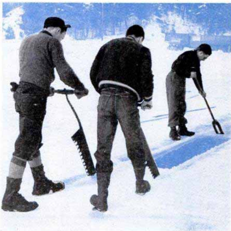
Ice is floated to the loading end in large sections, which are broken into blocks before going up the chute
