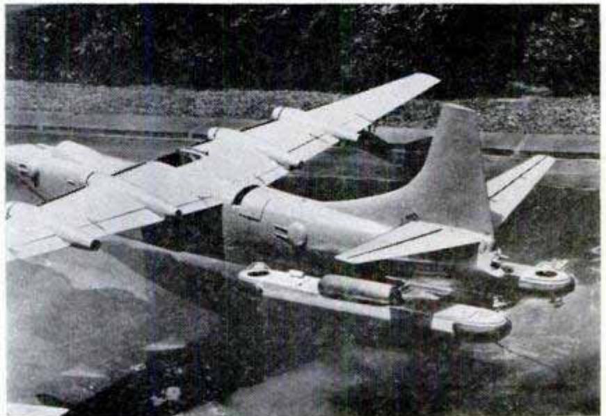
Beaching gear, above, is capable of lifting a 300,000-pound flying boat, carrying it ashore and wheeling it off on a repair platform. Two power units are located in diagonally opposite ends of the gear. Below, scale model shows how compact gear maneuvers under plane
