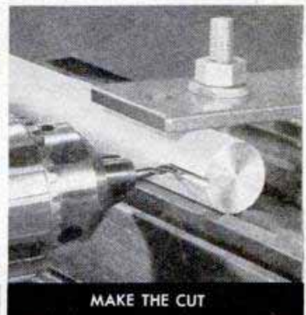
6 CUTTING A KEYWAY with an end mill often is a necessary operation. Use the test center to locate the work. Set the table stop to stop the feed at the desired position
