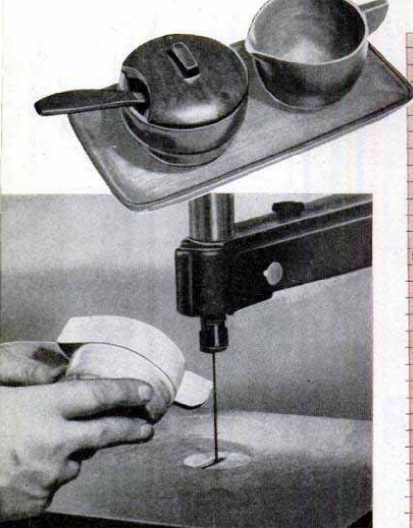
Blanks for handle and spout of cream pitcher are sawed from flange on turning. Sugar spoon is half-size version of salad spoon shown on opposite page
