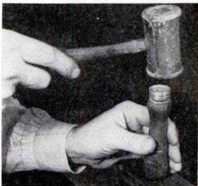
Photo at top of page shows how tubing sections can be held for polishing by slipping over bar. Above, tubing forms replacement ferrule for tool handle
