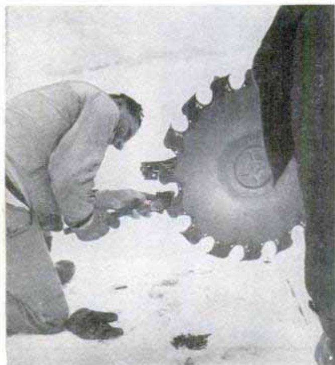
Teeth on the 30-inch blade of the power saw are replaceable. The saw scores the ice with 9-inch cuts
