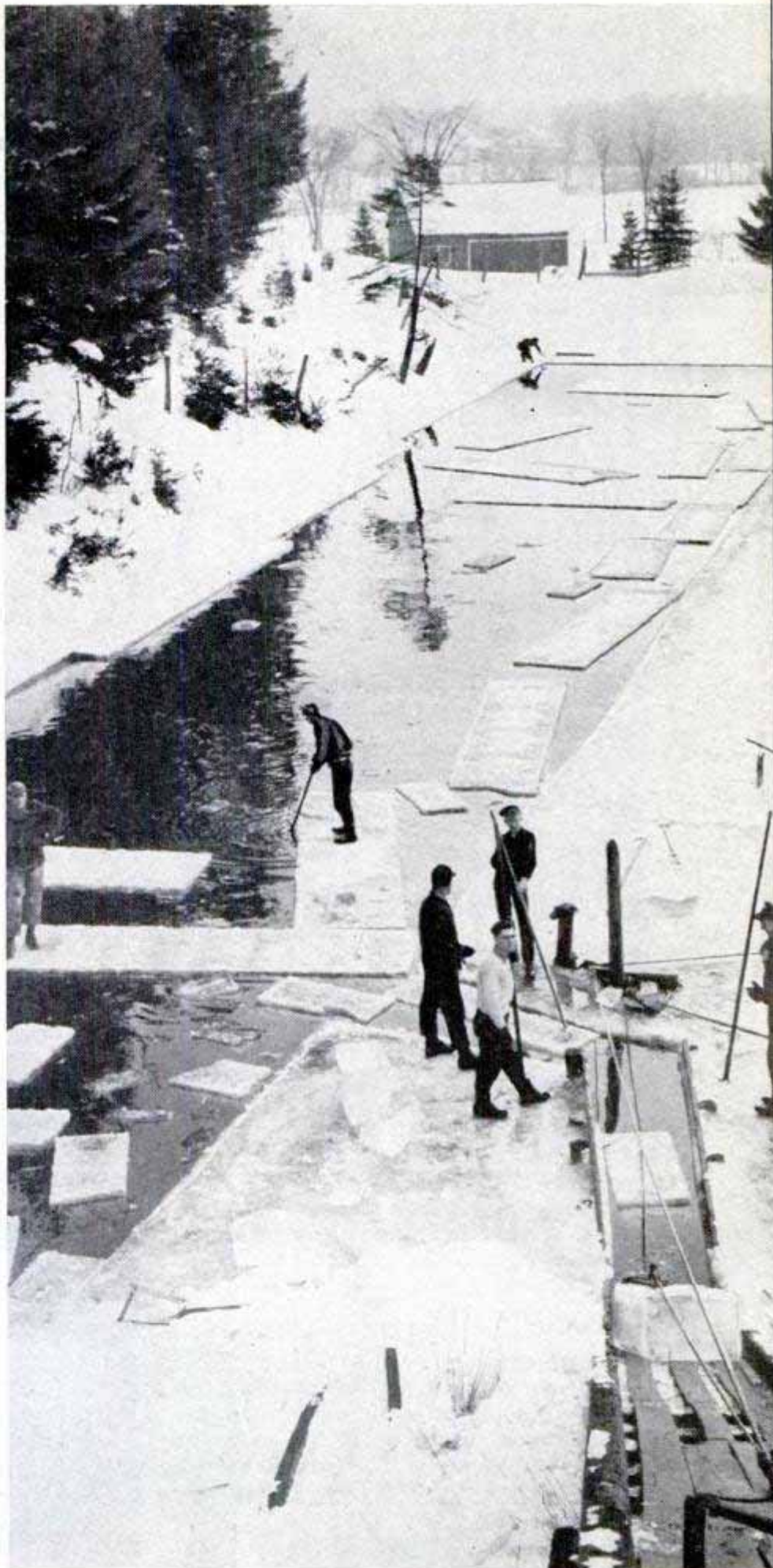
Here's an ice pond in full operation as seen from the top door of the icehouse. Blocks can be seen floating into the loading channel where they are picked up by the cable and hauled to the top of the chute to slide into the house. Workers ride ice floats like lumberjacks on logs
