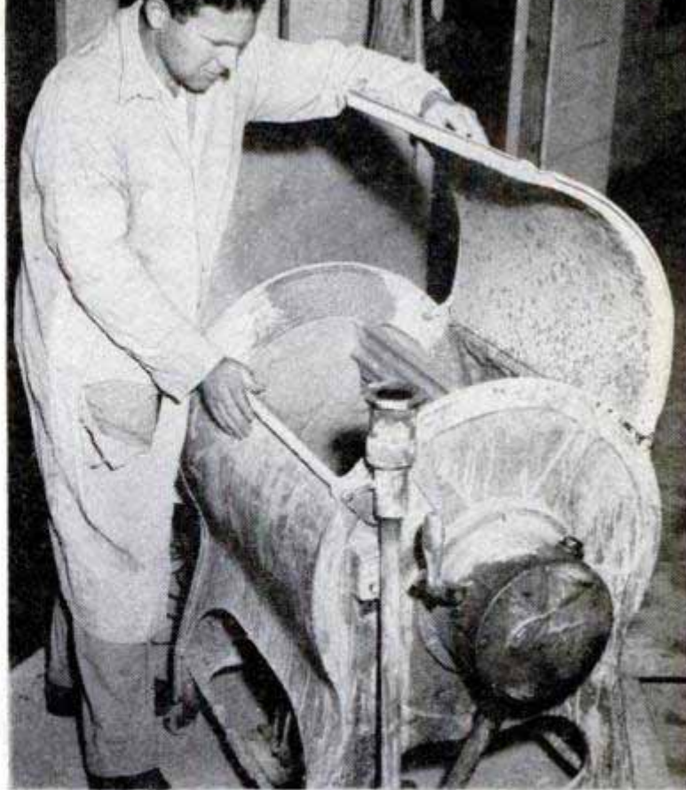
Drich converted an ancient washing machine into a mixer. It whips up week's supply of clay in two hours
