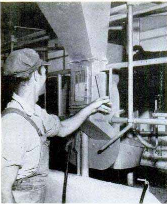
Milker releases lever, cutting off the flow of feed, when the desired level is reached in measuring glass
