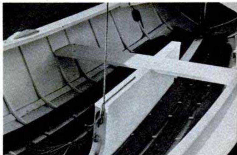
Close-up of the centerboard structure. The keel is dropped down through slit by means of a small rope
