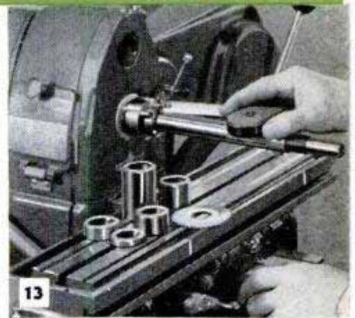
Above, spacing collars permit mounting saw close to spindle. Below, to avoid damage, use collar to push saw in place
