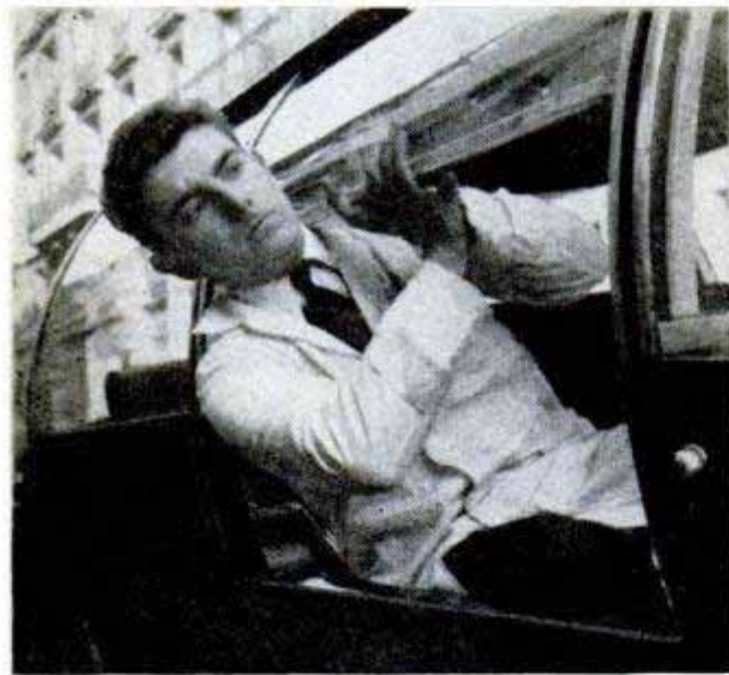
Doors open in the middle. The upper portion slides into the roof; the lower portion down into the floor
