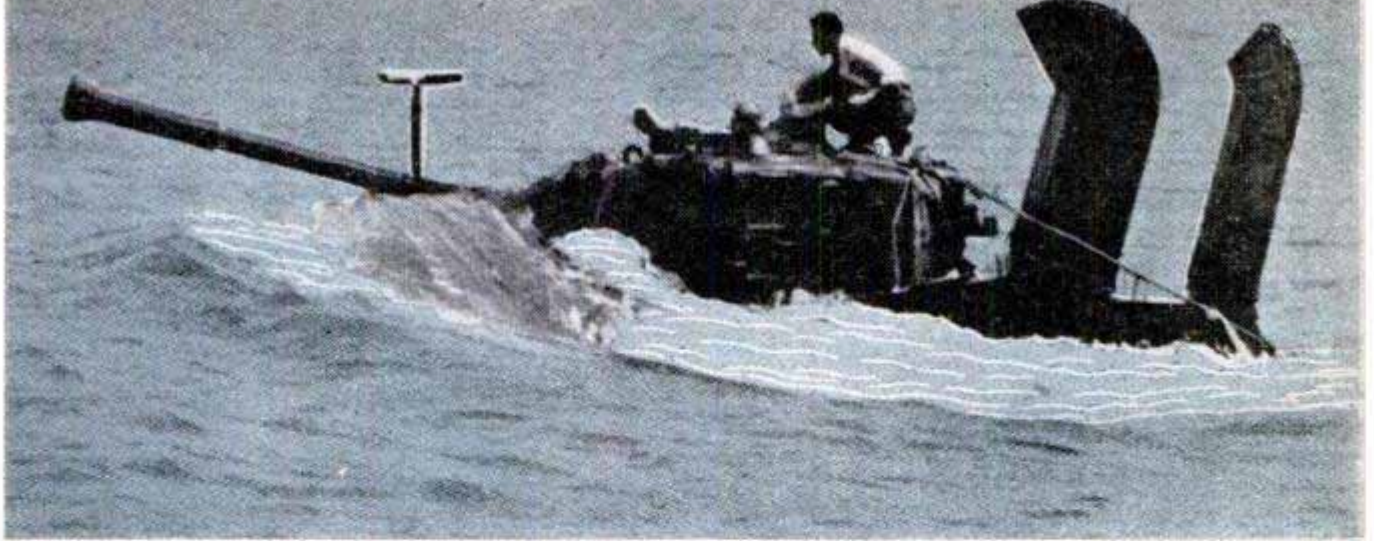
Today's tanks can "breathe" underwater and ford streams easily. Here, one of the heavier models, M-46, goes through its aquatic-test program
