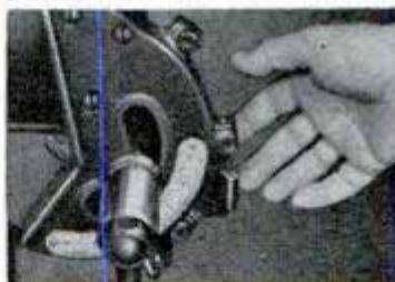
☆ Automatic stops set at 45°, 90° and 135°; large scale for accurate settings
