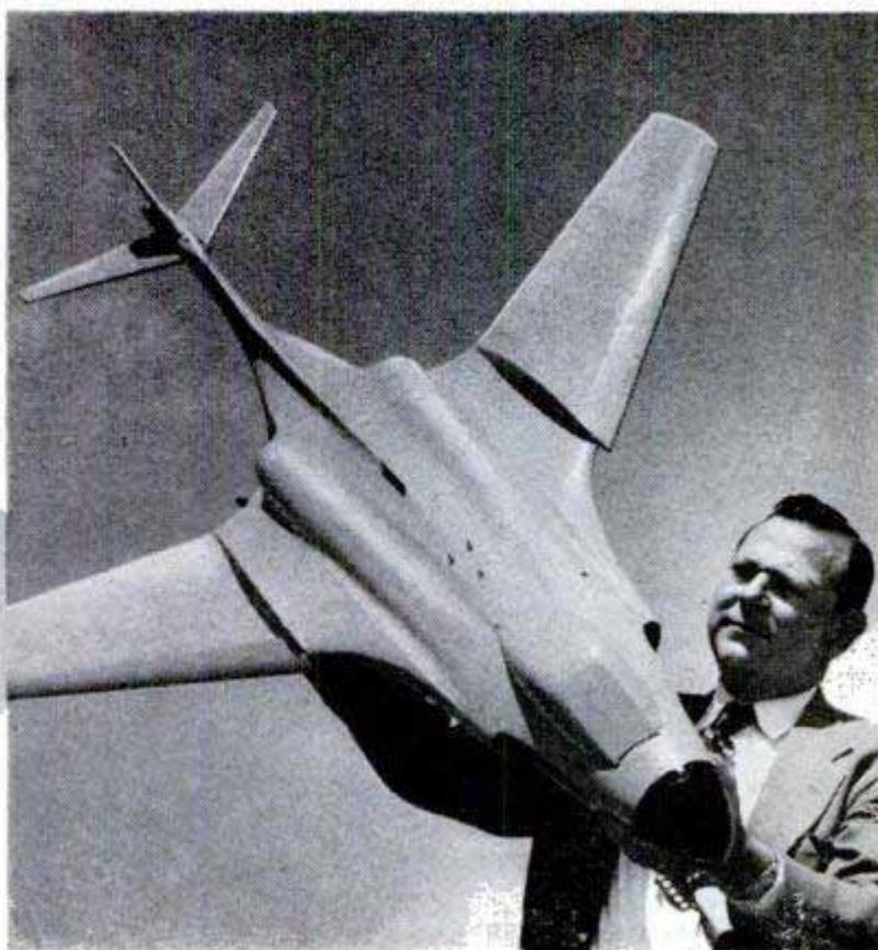
Model, powered by two jet engines and controlled by radio, behaves exactly like a full-size plane for airworthiness tests
