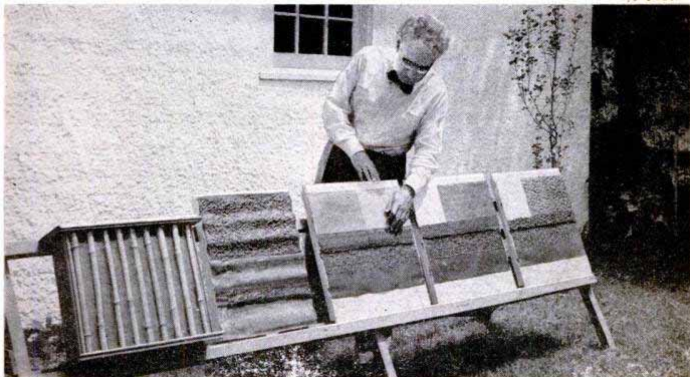
Plastic molasses sticks to almost anything. Here are construction samples made of bamboo, iron, chicken wire
