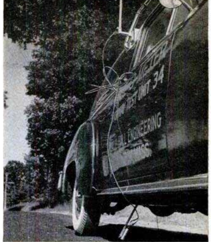
Some of the external instruments are the pitot tube and anemometer on the roof and a thermocouple near the ground that measures radiant heat from highway
