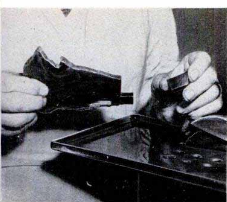
First step in making stone for a jade ring is to cut the ring blank from slab sliced from the rough
