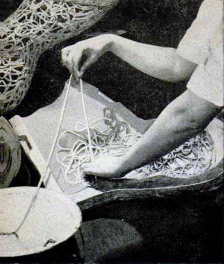
First step in the strange art is to make individual parts of mannequin by "doodling" strips in wet mold
