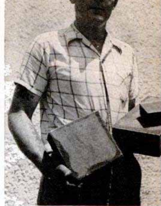
Resulting bricks, after hardening in the sun, are water-proof, hard as concrete, won't crumble in tropics
