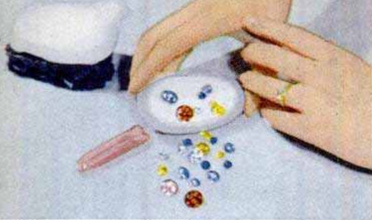
Displayed beside antique jade jewel box are synthetic rubies and sapphires, also a split ruby "boule"
