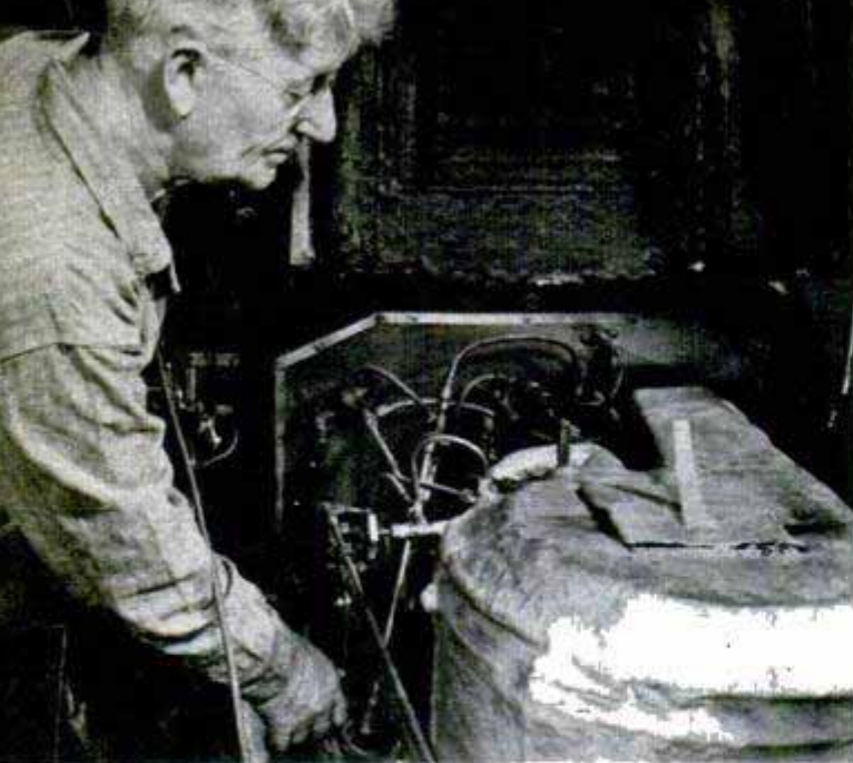
Brause's Stanley Steamer entry will be ready to roll when the pressure in this boiler gets to 500 pounds
