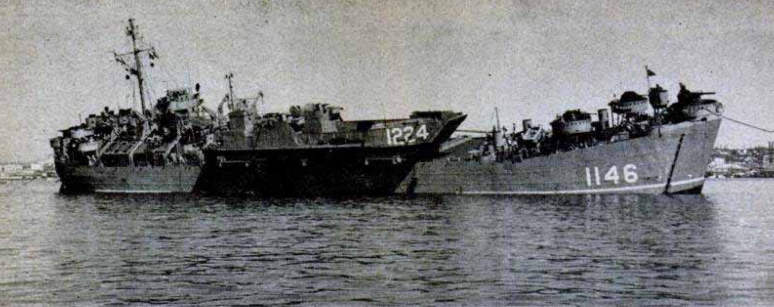
Stopped in mid-air by the Navy photographer, the LSU skids off the deck of the LST on its way into the water
