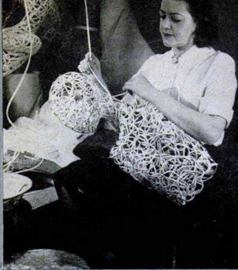
To finish figure, parts are mated with strips of same material, "scribbled" to make invisible joints
