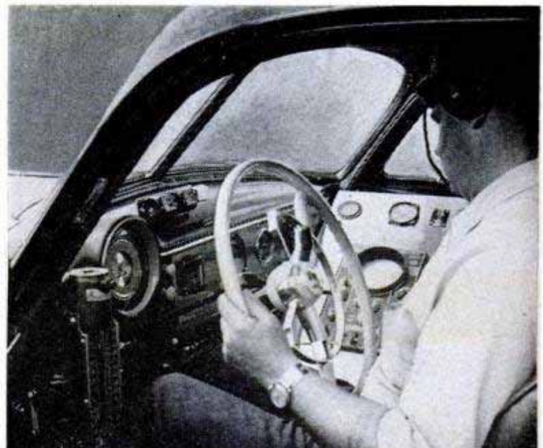
Wearing earphones, engineer Len Bell can listen to noises made by various parts of engine and chassis
