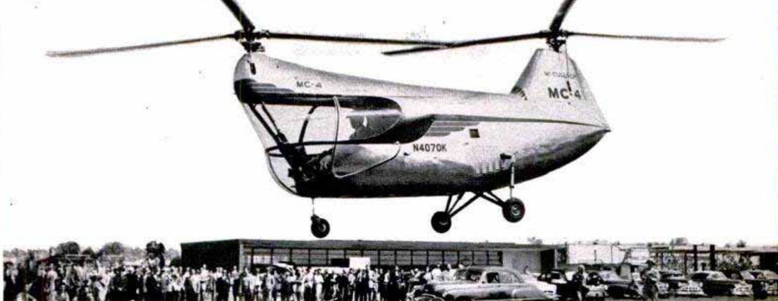
Rising straight up, the twin-rotored helicopter, above, travels 1520 feet a minute. Its horizontal speed is 100 miles an hour
