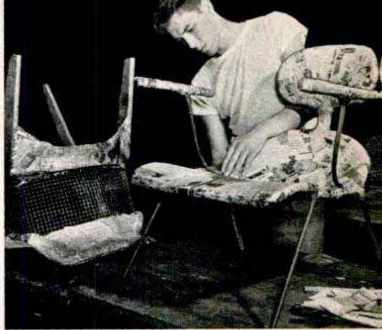
Wire mesh was used as foundation on this chair. Student covers frame with paper strips soaked in paste
