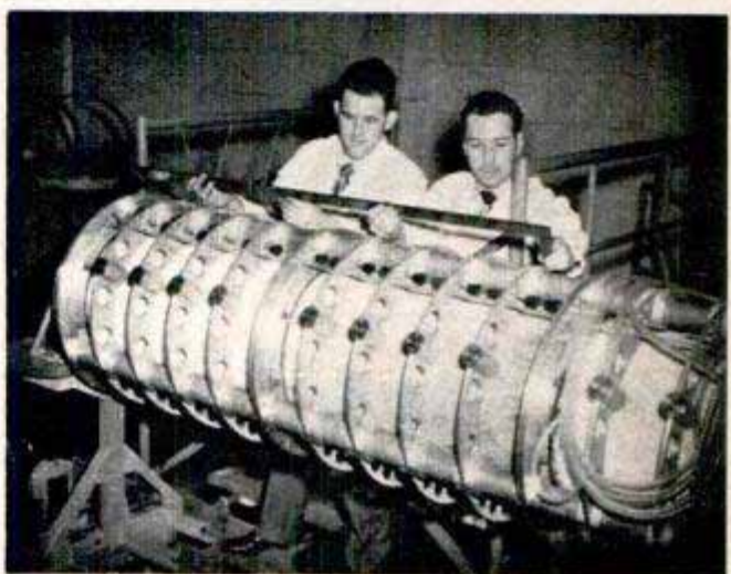
Above, using the scanning technique of television, an electron-gun X-ray device being developed at the institutes gets brighter pictures with less exposure
