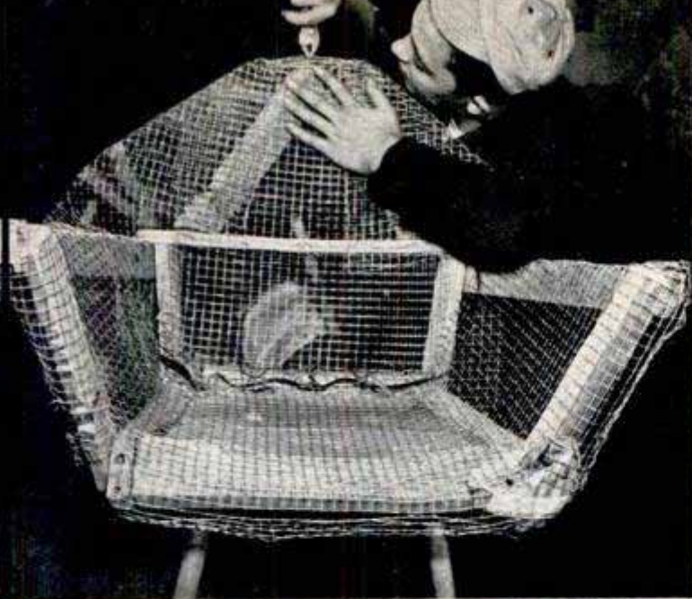
Crude foundation consists of wood frame covered with rabbit wire. Paper pulp will give it attractive lines
