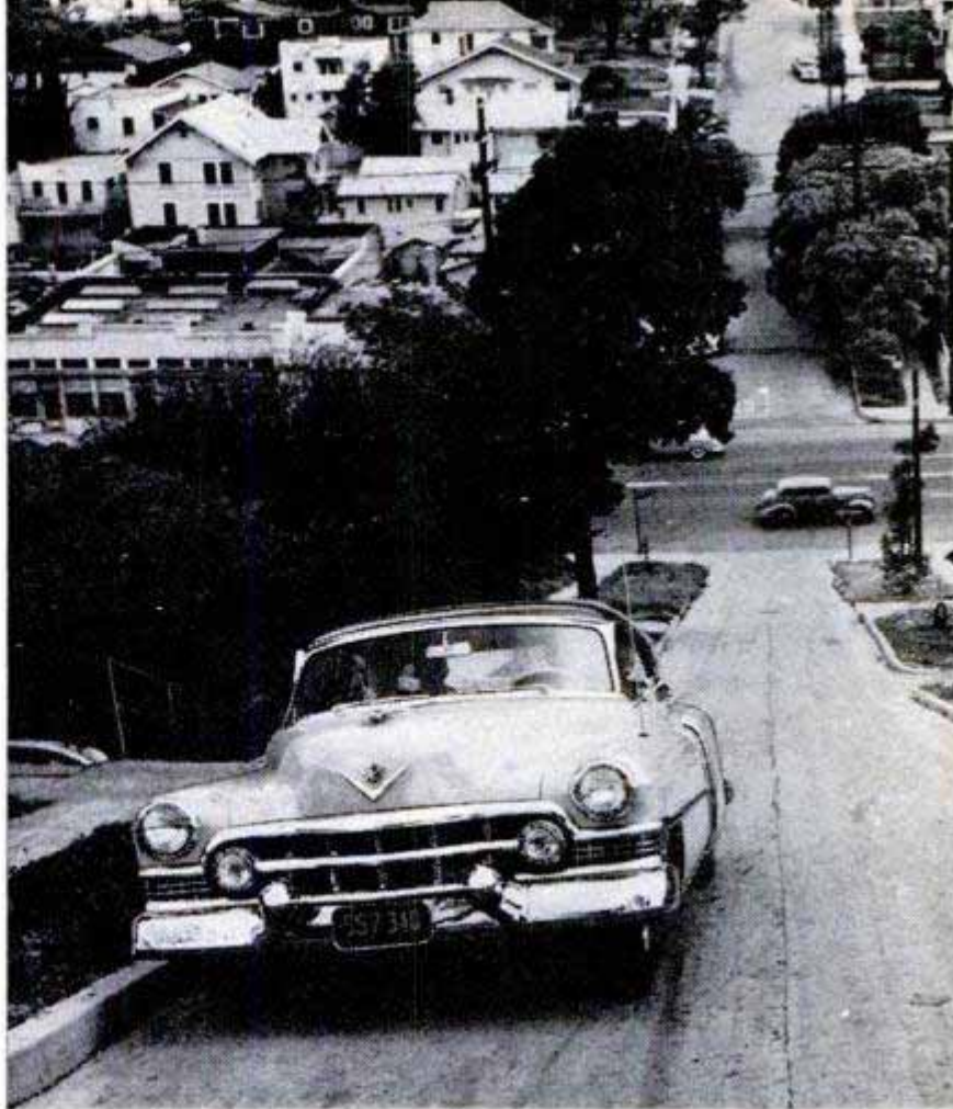
From a standing start the Cadillac Coupe de Ville tested by Clymer topped this 500-yard, 32-percent grade hill at 23 miles per hour
