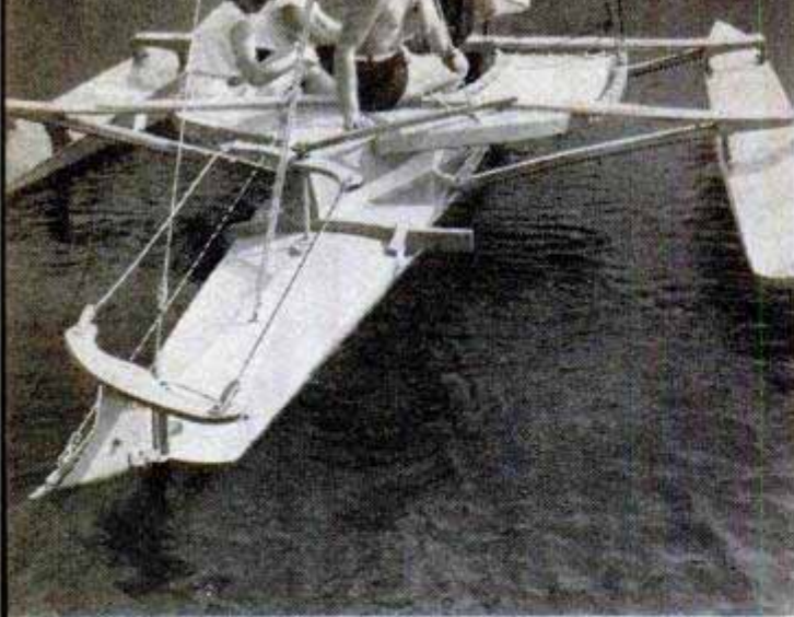
Above, stern view of Trimaran shows wooden bracket just aft of cockpit. This permits emergency mounting of outboard motor on starboard side of center hull
