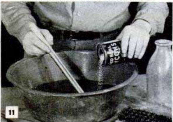
A CAN OF LYE (13 OZ.) WITH 1-GAL. HOT WATER WILL REMOVE OIL PAINT, WEAR RUBBER GLOVES. RINSE JOB WELL
