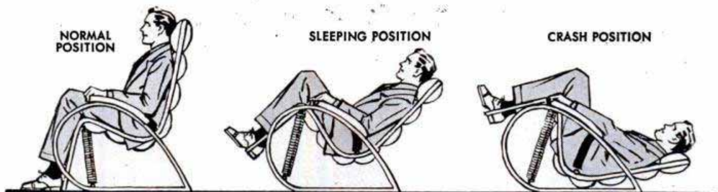
Resting position, above, of Bennett hammock-type seat. Sketches show how an impact tilts passenger backward, since his center of gravity is always lower than the front part of the seat
