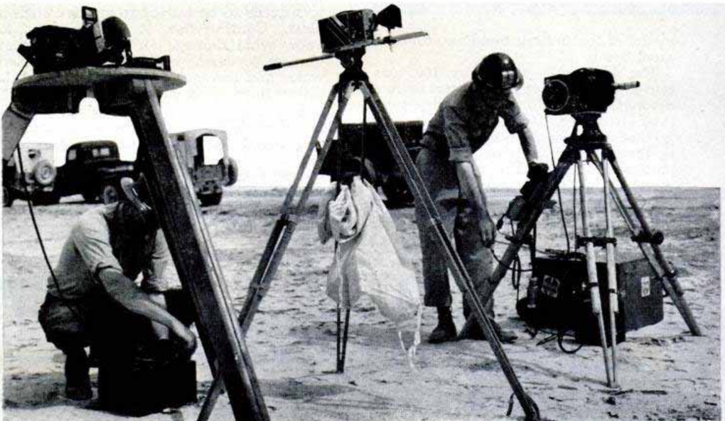
Numerous cameras record the explosions. One at left rotates to follow and photograph the huge dust cloud
