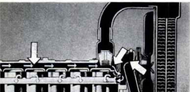
Under the Plymouth hood Floyd Clymer finds weather-proofed distributor and wires, accessible battery. Below, cutaway of built-in by-pass cooling system
