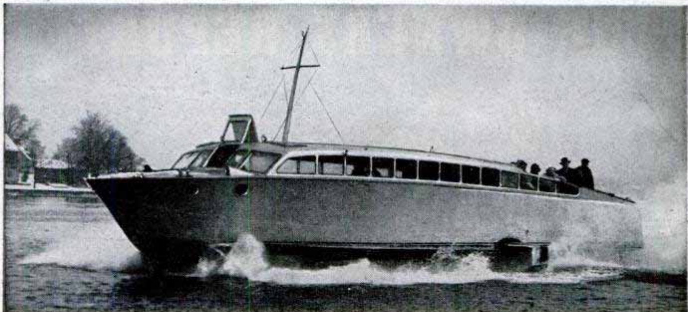
Spray stirred up by the "wings" hides the evidence, but the hull of this boat is almost entirely out of water
