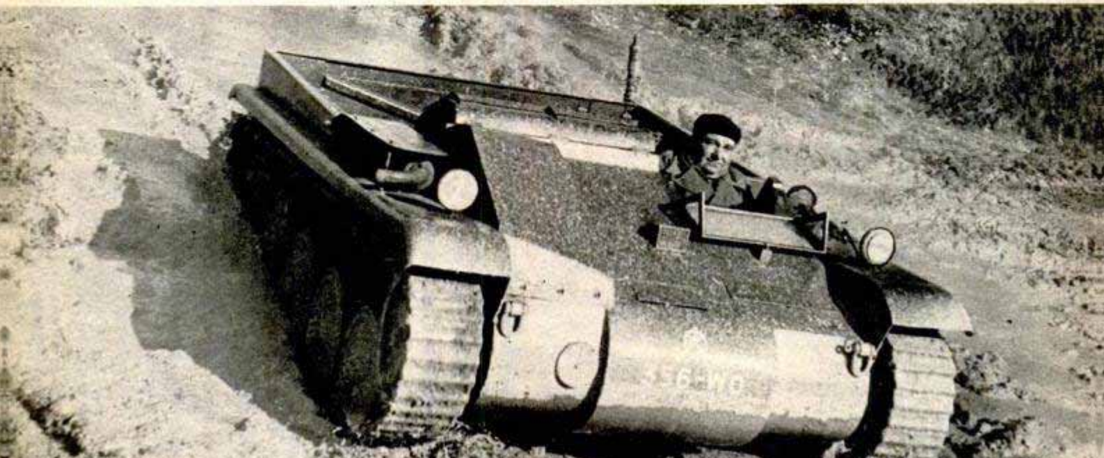
Sturdy and fast, the one-ton Hotchkiss ammunition carrier can be parachuted down with airborne soldiers
