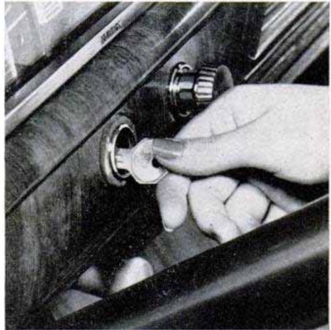
Combination ignition key and starter on Plymouth is handily placed to the right of steering column
