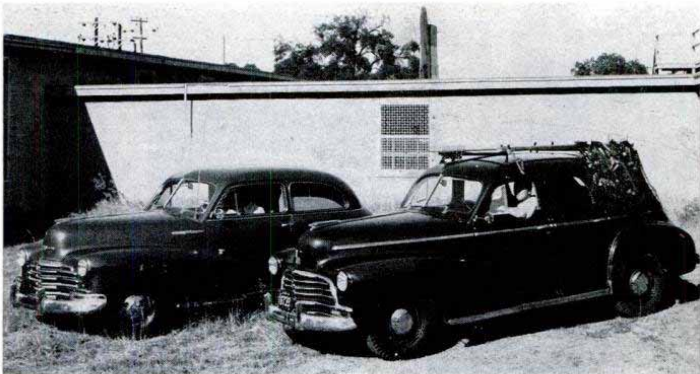
Rear car is the laboratory, interior details shown below. Other car carries geophones, stakes and explosives
