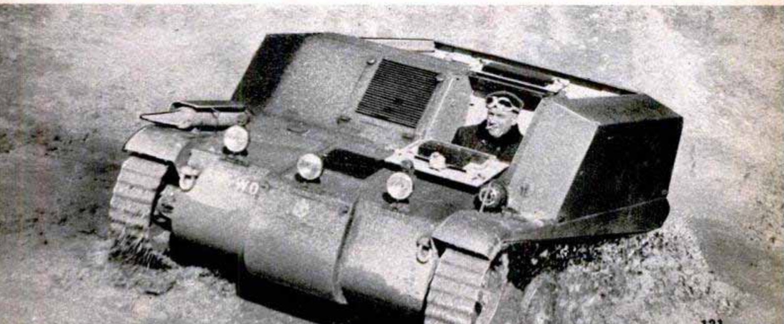
Armored reconnaissance model of Hotchkiss carrier operates effectively over rough ground and through water
