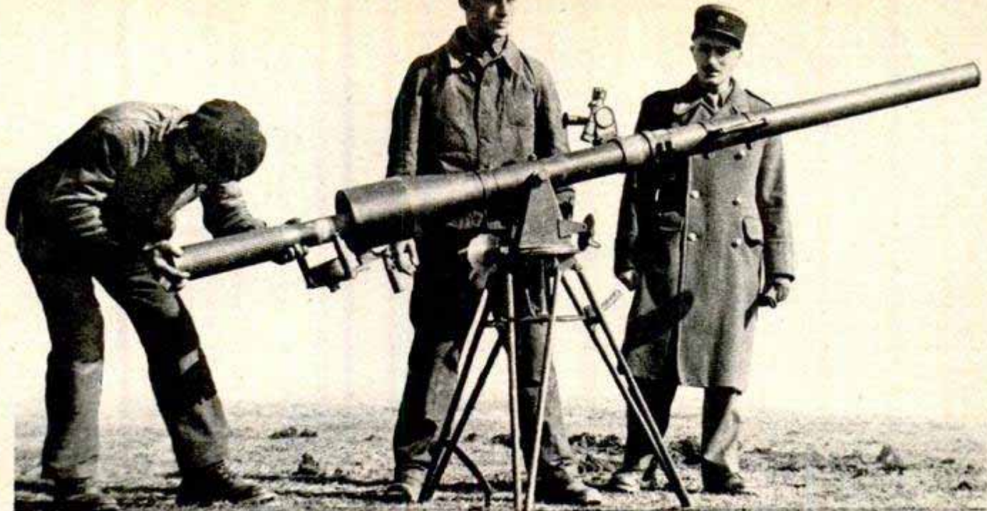
Resembling its American counterpart, the 75-mm. recoilless weapon for airborne troops weighs 150 pounds
