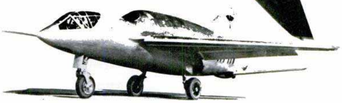
Ground view of fighter-bomber shows large air intake for jet engines to rear of canopy. It is slowed down after landing by a ribbon-type parachute
