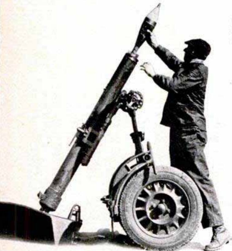
Firing a 28-pound projectile, the Brandt mortar at left has a firing rate of 10 rounds per minute. It is capable of lobbing shells (below) 4½ miles
