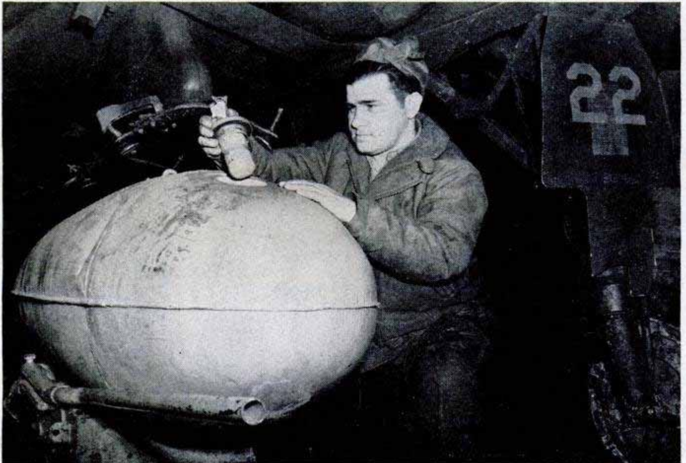
Just prior to "delivery," an ordnanceman on a U. S. carrier installs the igniter in a napalm belly tank U. S. Navy photo
