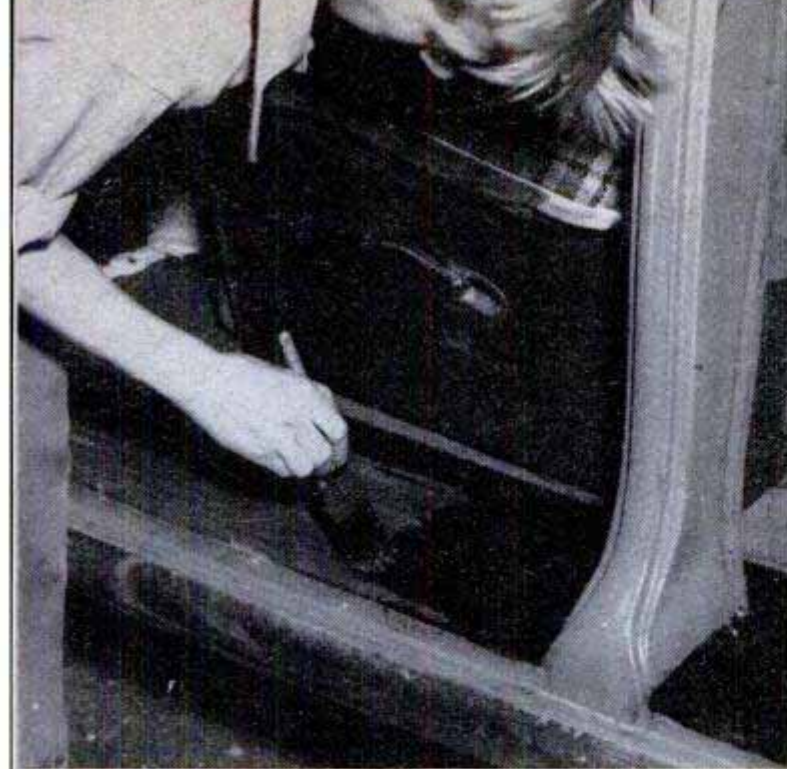
A thin mixture of drop black and turpentine makes a good dressing for the rubber mats and running boards
