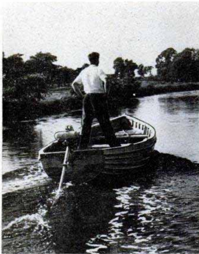
Left, shaft enters water at angle to keep bow of light craft from riding skyward. Right, same engine, with pump and nozzle, sprays trees. Below, fouled propeller can be swung inboard Atco Motor Mowers, 67 Broad St., New York City 4
