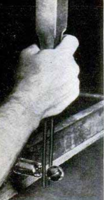
Small balls of glass, formed in a mold, are pinched off, then fused into place on the base of a bowl
