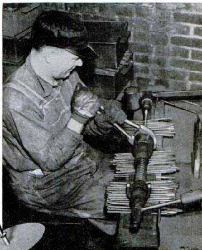
The Torsion Test to which every Crescent screwdriver blade is subjected before assembly
