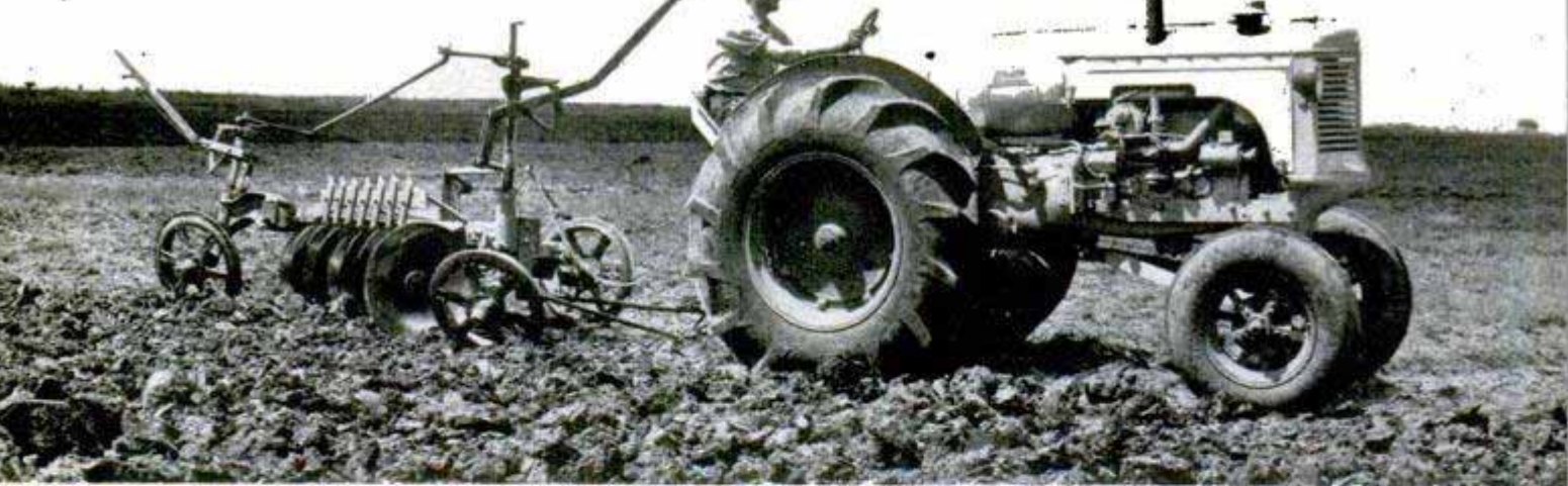
Operating on LPG, a Minneapolis-Moline tractor pulls a disk plow over a rice seed bed near Lake Charles, La.
