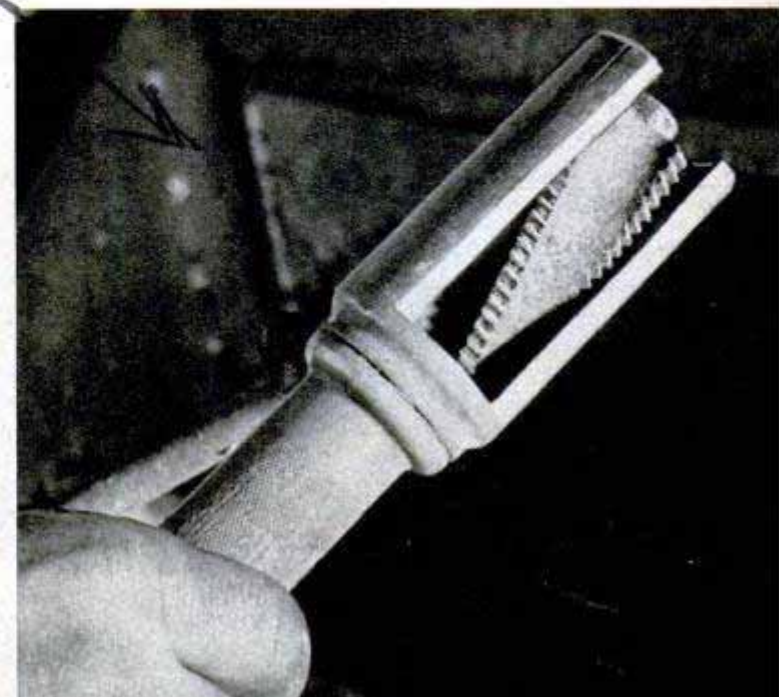
Water is pumped through rotary knife as workman scales fish with electrically driven tool shown at right
