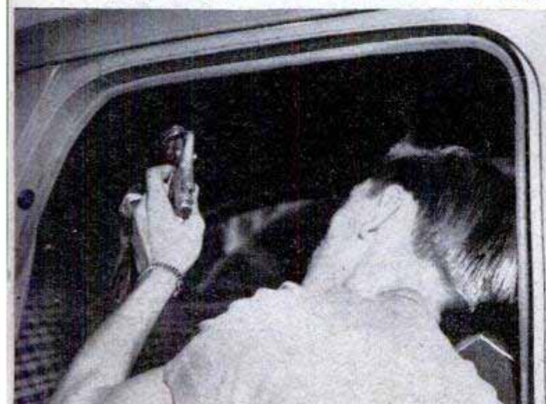
Above, to make seat covers fit snugly, compress the seat by standing on it while attaching them. Below, after cleaning the headliner and brushing thoroughly, spray on a light coat of fabric finish with spray gun
