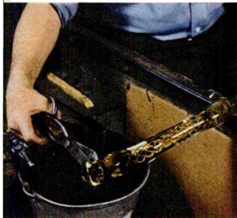
Grooved "gather" is pulled and twisted at the same time, producing long spirals in the molten glass
