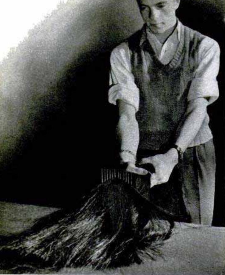
Worker combs Caslan fibers which look like coarse hair. They will be cut, used as paintbrush bristles
