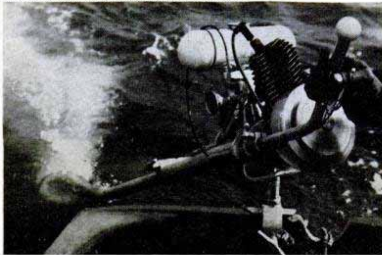
Left, shaft enters water at angle to keep bow of light craft from riding skyward. Right, same engine, with pump and nozzle, sprays trees. Below, fouled propeller can be swung inboard Atco Motor Mowers, 67 Broad St., New York City 4
