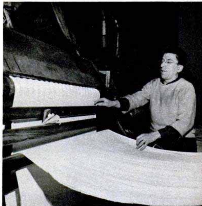
Chemical textiles are fuzzed into fluffy fabrics by special method. Here material passes over wavy roll
