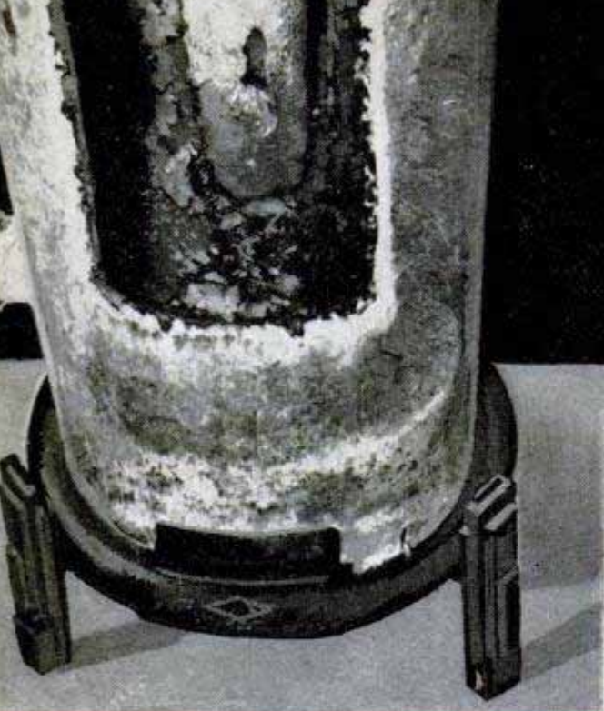
Cutaway view of water heater shows scale along sides of tank and material collected at bottom as a result of heating unsoftened water over long periods
