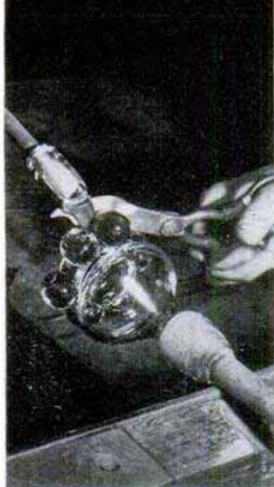
Small balls of glass, formed in a mold, are pinched off, then fused into place on the base of a bowl
