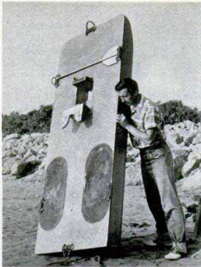
Emergency paddle is clamped to water bronco. Odd-shaped board prevents water from splashing rider
