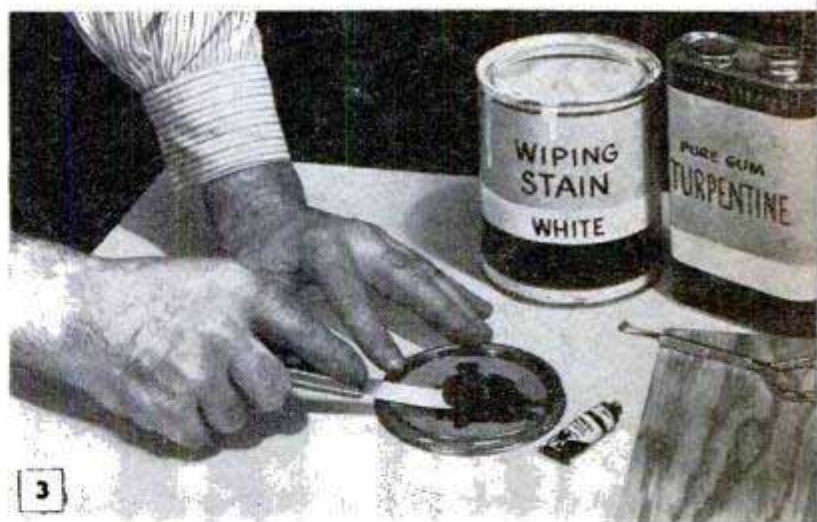
OIL COLORS added to white-pigment stain, above, will make any desired color. Below, the blond, or Beachwood, finish on fir plywood. Note grain variations with different treatment
