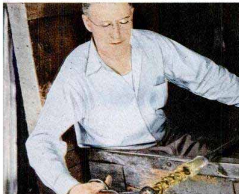
Grooved "gather" is pulled and twisted at the same time, producing long spirals in the molten glass
