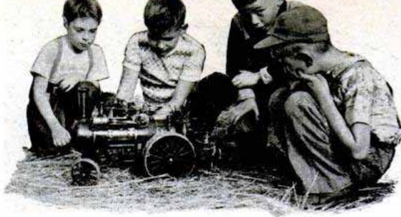
Complete in all details, the \frac{1}{3} -horsepower midget at left is a copy of one in the Busch collection. It has been tested to 120 pounds of steam
