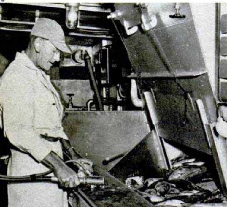
Water is pumped through rotary knife as workman scales fish with electrically driven tool shown at right
