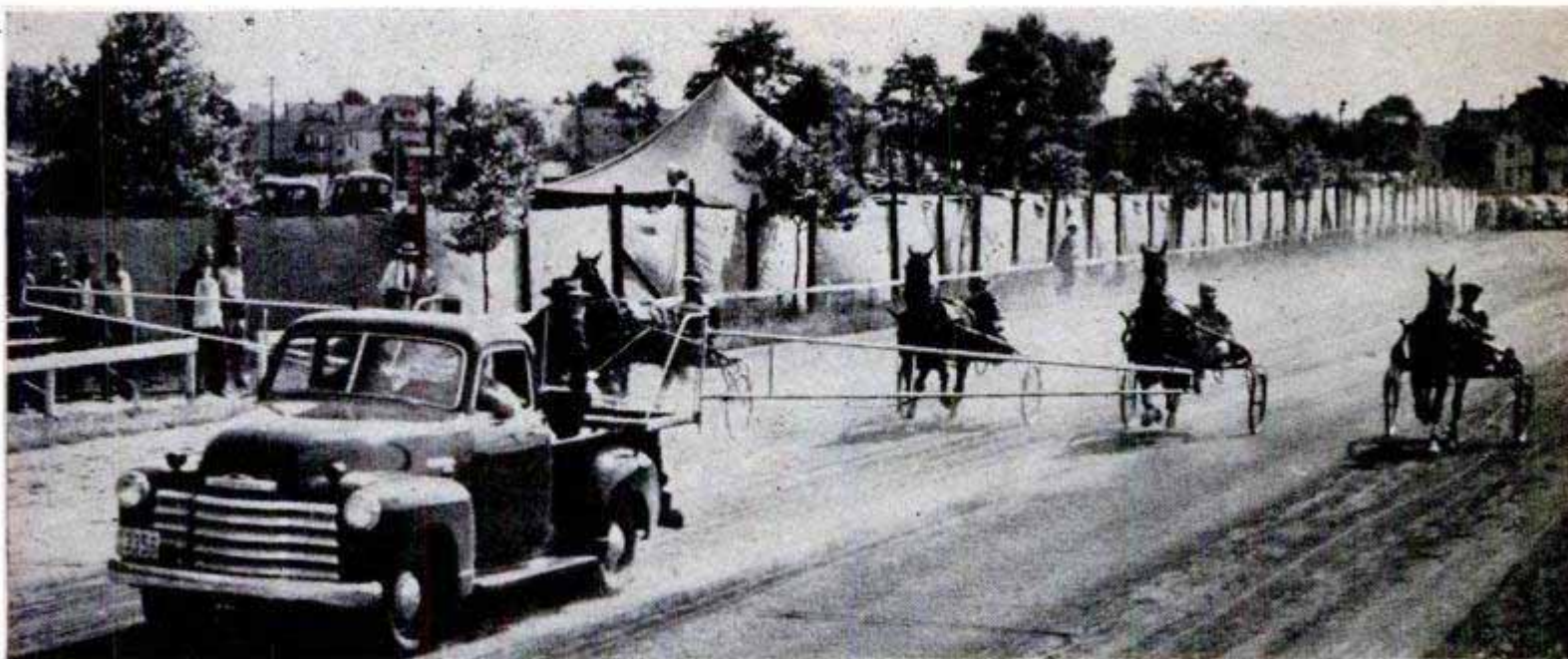
Homemade starting gate cost under $100. At starting line, wings swing forward and truck speeds out of way
