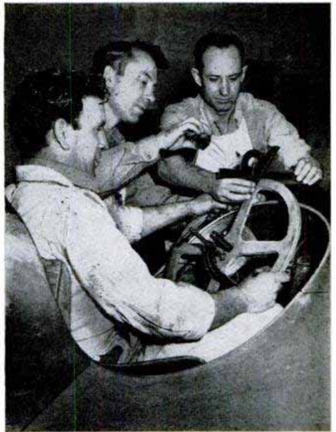
Driver sits in partly finished body while car builders measure the angle and position of steering wheel
