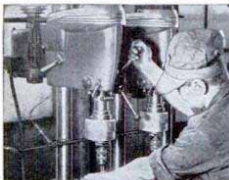
Typical gang drill press set-up for tapping. CRAFTSMAN flexibility can save you money in hundreds of similar industrial applications like this!
