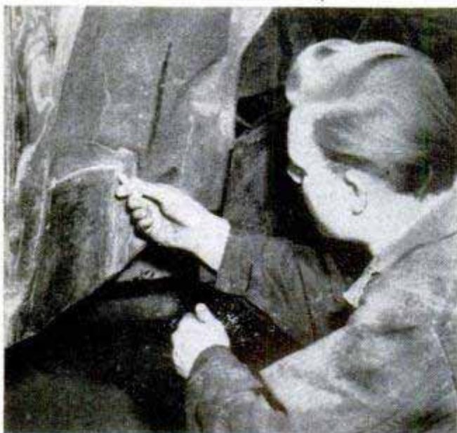
Here, sheet-metal patch is welded to car body where metal was broken through by rust and flying gravel
