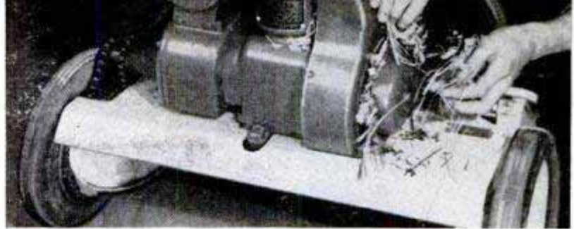
Clean the mower thoroughly after use to remove leaves and grass clippings from mechanism, especially from cylinder cooling fins
