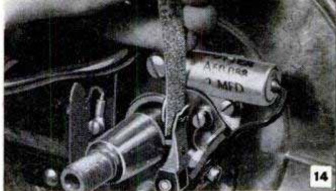
When truing breaker points, use a flexible hone made for the purpose. Clean ignition system thoroughly
