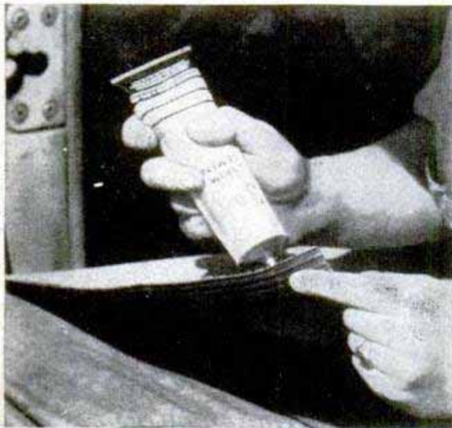
Worn floor mats can be repaired by applying patches of mat material, with rubber cement used as adhesive
