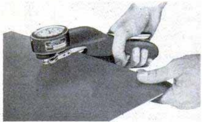
Federal Products Corp., Providence, R.I. PORTABLE THICKNESS GAUGE assures precise check on thicknesses of sheet stock used for stamping and forming. Full-jeweled dial indicator, of either the direct or continuous-reading type, is graduated to .001 in. Movable and fixed anvils, or jaws, grip stock and hold gauge perpendicular to the surface. Hardened contact points transfer measurement to dial hand
