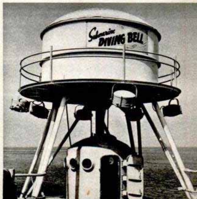
Below, left, sketch explains diving-bell operation. Right, structure above bell houses motor and compressor
