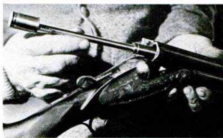
Top, .22 shot shell compared with large, standard shell. Above, barrel liner changes bore to .22-caliber
