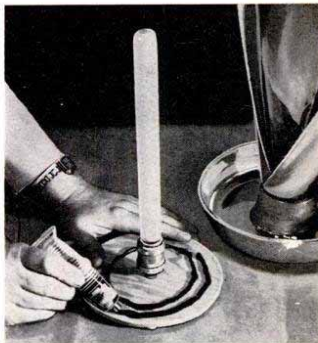
After fitting socket and lamp bulb, coat the plywood base with cement and attach to bottom of the planter
