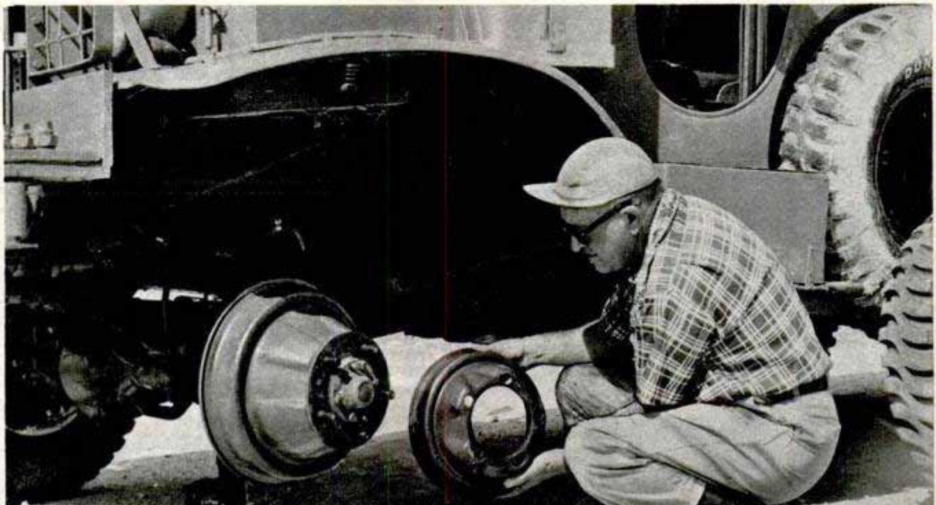
Tiny heating plant is a welcome addition when the Russells travel through mountain country. Below, he holds a small brake drum replaced with oversize
