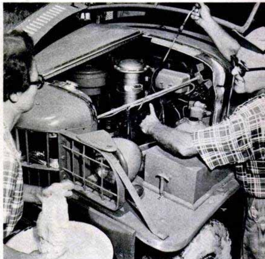
Front-wheel-drive lever was moved over with other two levers so that all would be under the driver's right hand. Below, an oil-refining device was added
