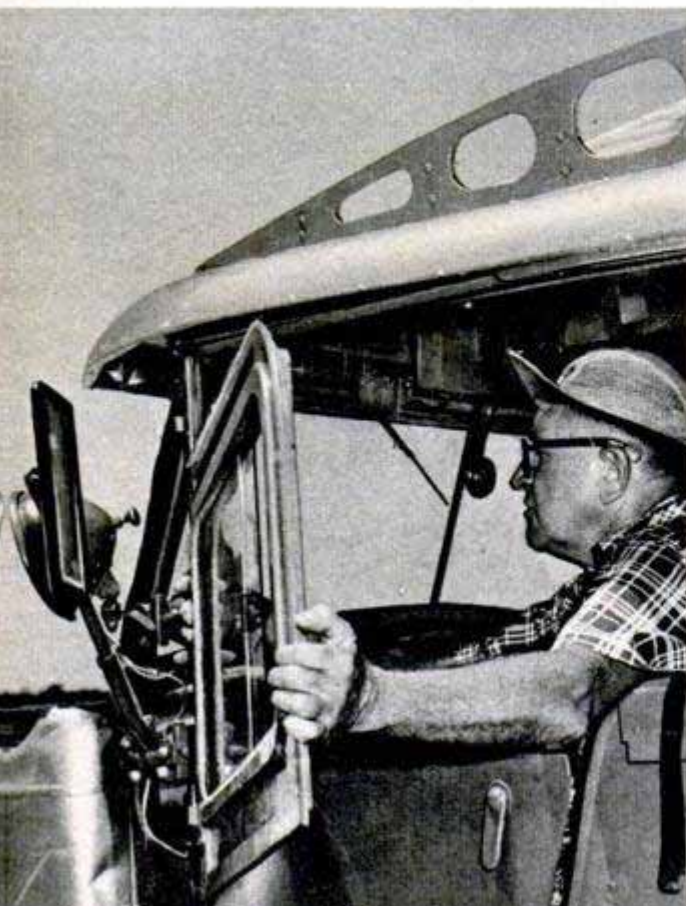
New winch, driven by conventional power take-off, can also be hand cranked. It replaces an electric winch. Below, airplane rib on cab lifts tree limbs
