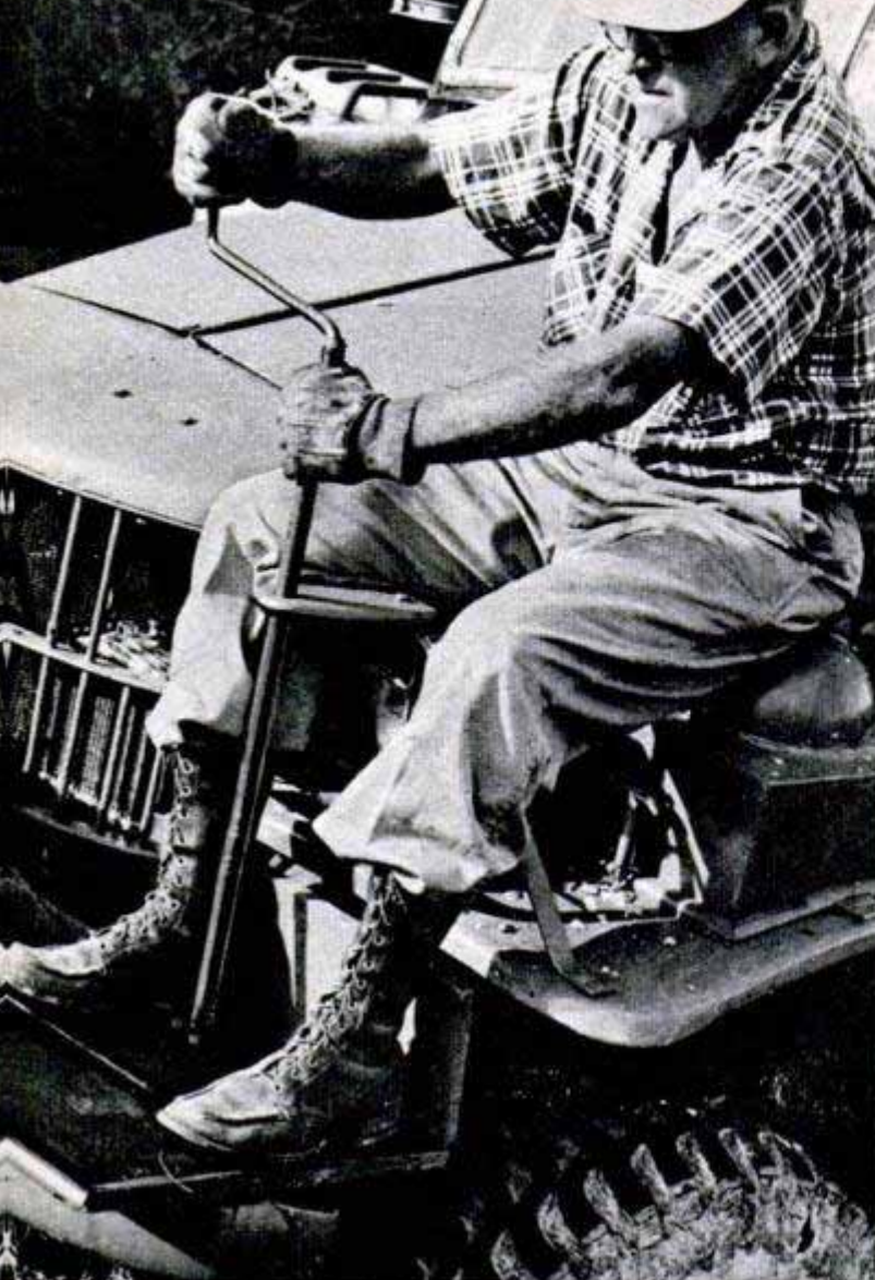
New winch, driven by conventional power take-off, can also be hand cranked. It replaces an electric winch. Below, airplane rib on cab lifts tree limbs
