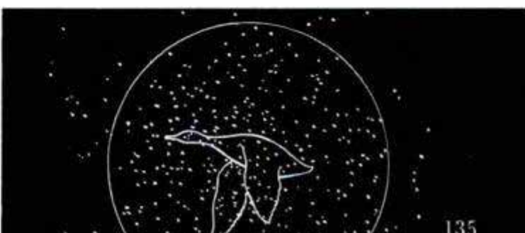
Gas leakage and wad produce spotty pattern. Bird can escape. Below, today's shell yields neat, even pattern
