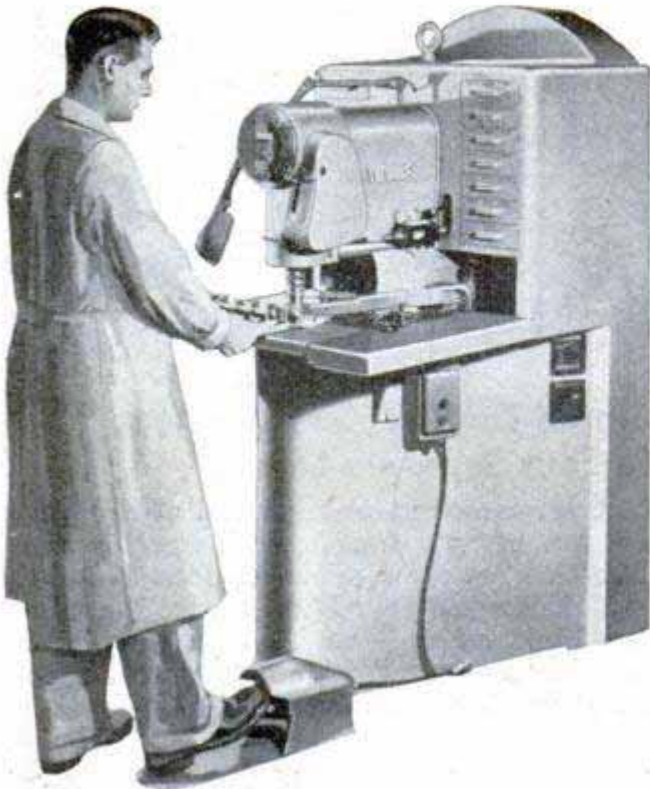
Wales-Strippit Corp., North Tonawanda, N.Y. MULTIPLE HOLE-PUNCHING SYSTEM in which the die units are self-contained and interchangeable permits the same units to be used in a variety of setups. Arranged in a box-type unit, the dies are inserted in holes drilled with a master template. In box-type assemblies, holes can be punched in almost any pattern over a working area 21 in. wide and 23 in. long. Twin-plate assemblies are used for larger work
