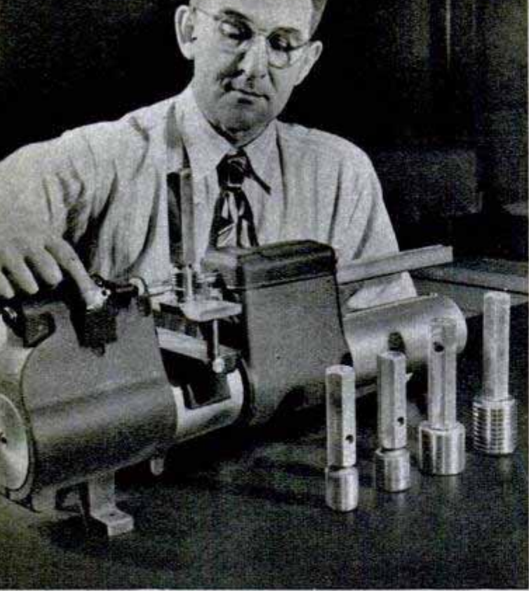
Double check: The gauges used to check the threads of bolts are themselves tested with supermicrometer
