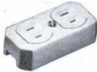
John I. Paulding, Inc., New Bedford, Mass. DUPLEX SURFACE OUTLET is designed for easy surface mounting and has extra knockout for use when wiring in series. Double-spring phosphor-bronze clips assure positive electrical contact when plug is inserted
