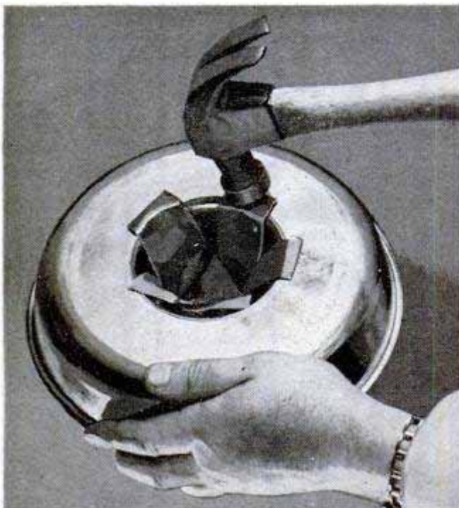
After inserting end of metal roll through baking tin, slit the metal with tin snips and hammer the ends over
