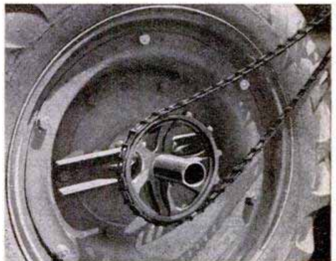
Drive sprocket is mounted on stub shaft welded to a steel channel which is cut long enough to span the hub bolts. Use a skip-tooth sprocket for the drive
