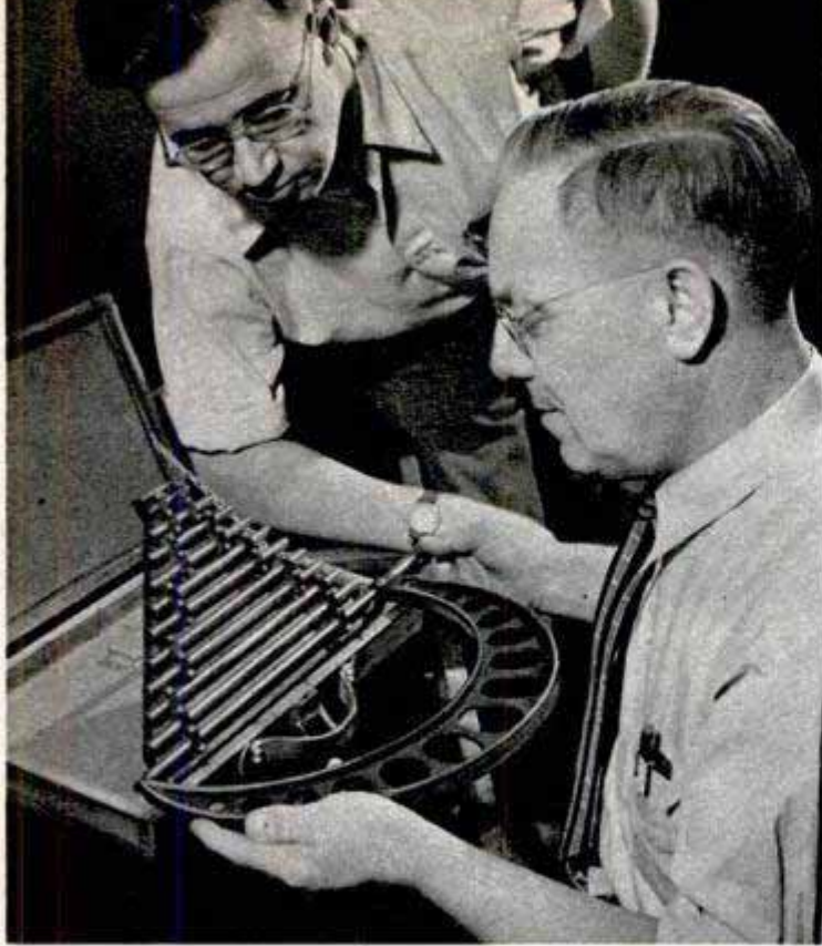
Kit of standard length bars determines whether instruments are accurate. Inaccurate gauges are rebuilt
