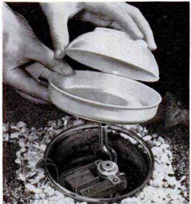
Rock-garden pump is concealed in deep bowl. Water from plastic dish set on bowl rim drains through holes near sides so motor and wiring are kept dry
