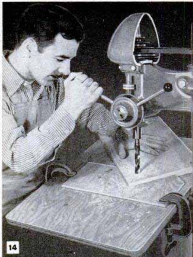
14 EQUAL COMPOUND ANGLES CAN BE CONVERTED TO SIMPLE ANGLES BY USING THE TABLE SHOWN AT THE TOP OF THE PAGE. NOTE THAT THE DRILLING LINE IS ALWAYS 45° TO THE EDGES OF THE WORK SURFACE
