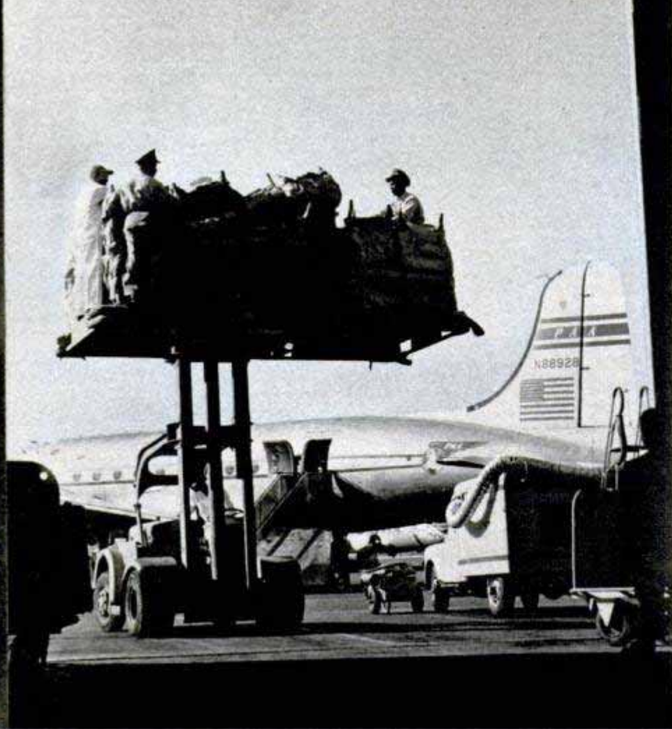
Like a waiter carrying a tray, the fork-lift truck moves a furniture shipment to a waiting cargo craft, where it'll be hoisted to the exact height of the loading hatch. Below, their speed and smooth riding make cargo airplanes popular carriers for animals like this husky alligator
