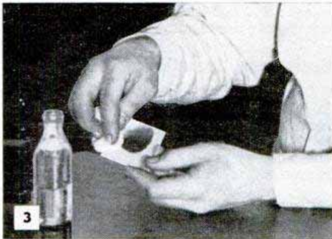
Above, to obtain an image of greater brilliance, coat ground glass with castor oil. Below, to shoot over the heads of people, or to get dramatic composition in high-angle shots, camera is held in this position
