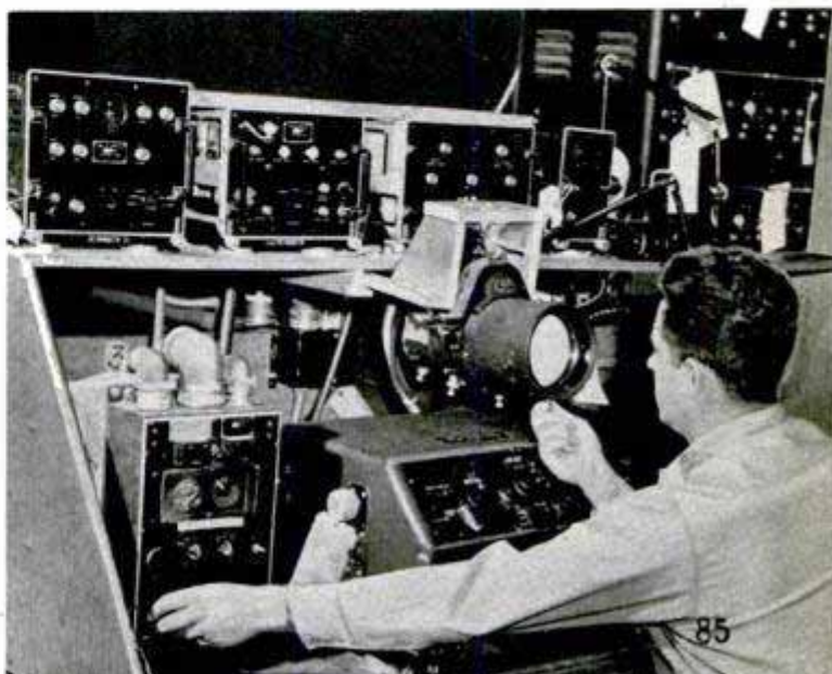
Using the supersonic trainer, a student simulates a mission of bombing and navigating entirely by radar
