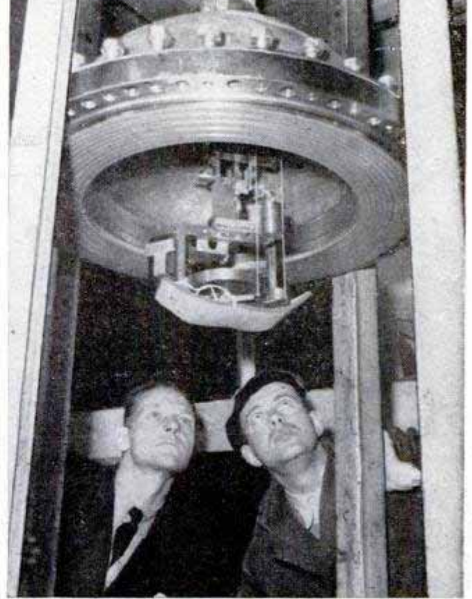
Bronze ball holds instruments for measuring earth magnetism to determine if it increases with depth
