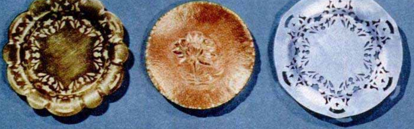
Scalloped brass plate shows how "etching" can be done with vibrating tool. Embossed flower in copper plate is raised by dishing background. Same pattern is used in aluminum plate as brass one, except it is jigsawed
