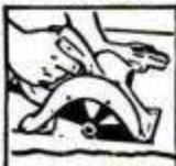
Cutting Tile, Transite, Slate
