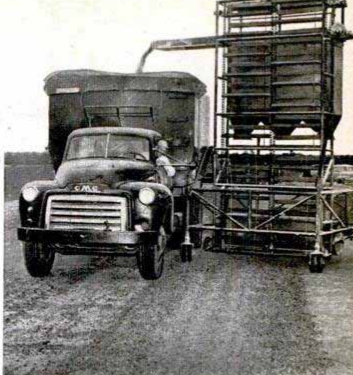
Powered by a small air-cooled engine, sweeper brushes push dried potatoes toward elevator buckets that lift them into truck
