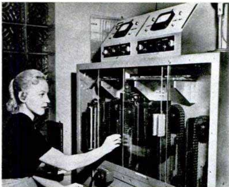
Telanserphone, 224 East 38th St., New York City. Above, this transmitter automatically calls doctors by radio when the triggering slides, below, are inserted in it. Right, the small battery-operated receiver looks like a hearing aid
