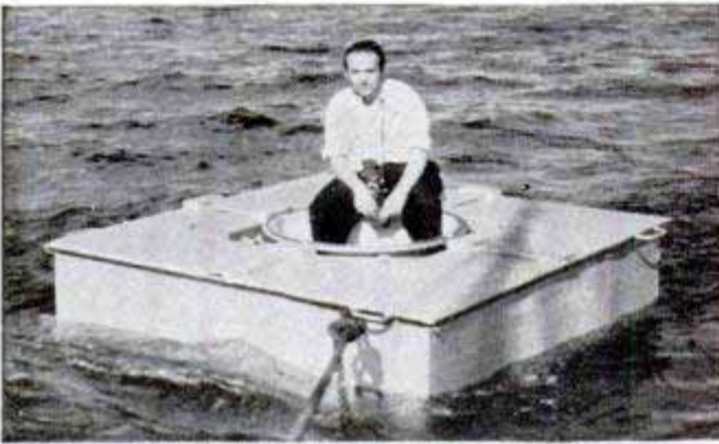
When a monster of the deep is pulled alongside the Galathea, a photographer can step overboard into floating tank which has camera port of thick glass
