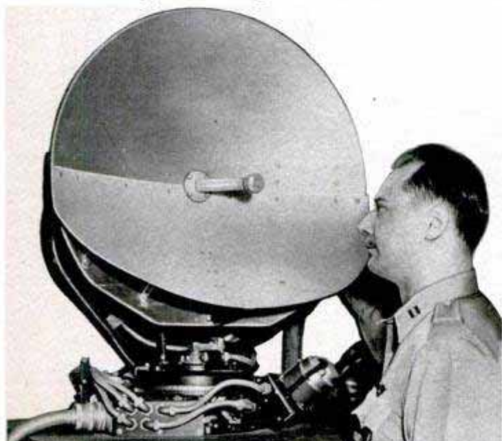
Scanner, or antenna, of radar that allows bombardier to watch ground through either clouds or darkness
