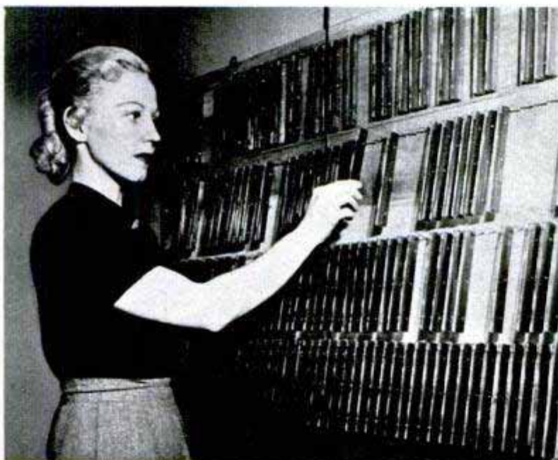
Telanserphone, 224 East 38th St., New York City. Above, this transmitter automatically calls doctors by radio when the triggering slides, below, are inserted in it. Right, the small battery-operated receiver looks like a hearing aid
