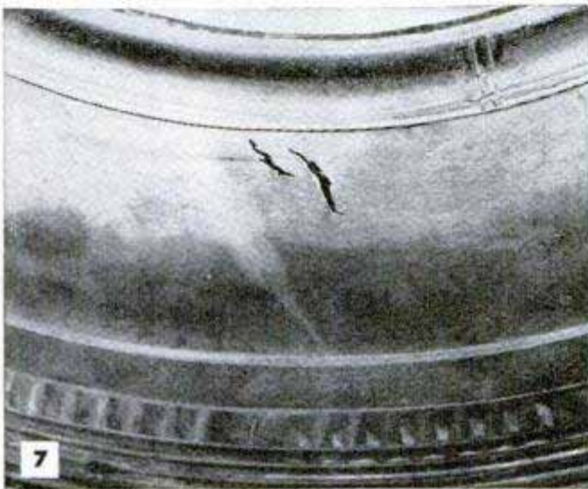
7 In older tires, breaks may appear on outer sidewall. A sharp fold in sidewall may also pinch the tube, causing an immediate break, or at best a delayed one
