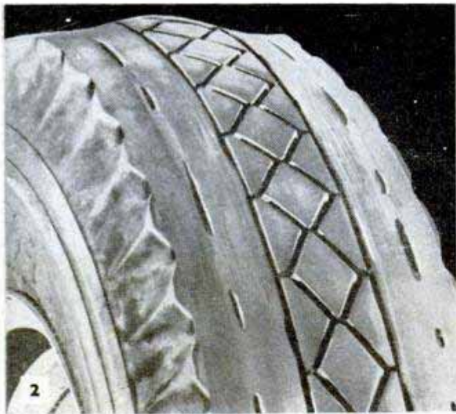
This tread wear is caused by running the tire under-inflated. Note the absence of wear at center of tread
