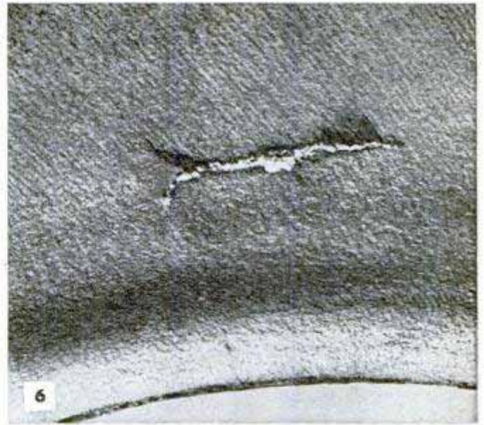
6 Here's what may happen inside the tire when you drive over a high obstruction or back onto the curb
