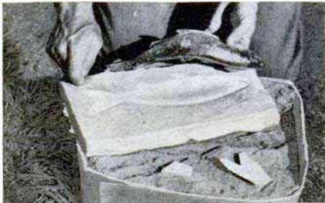
Plaster of paris is poured over the fish to make an impression mold as shown above. Below, the impression mold is oiled before the plaster casting is poured
