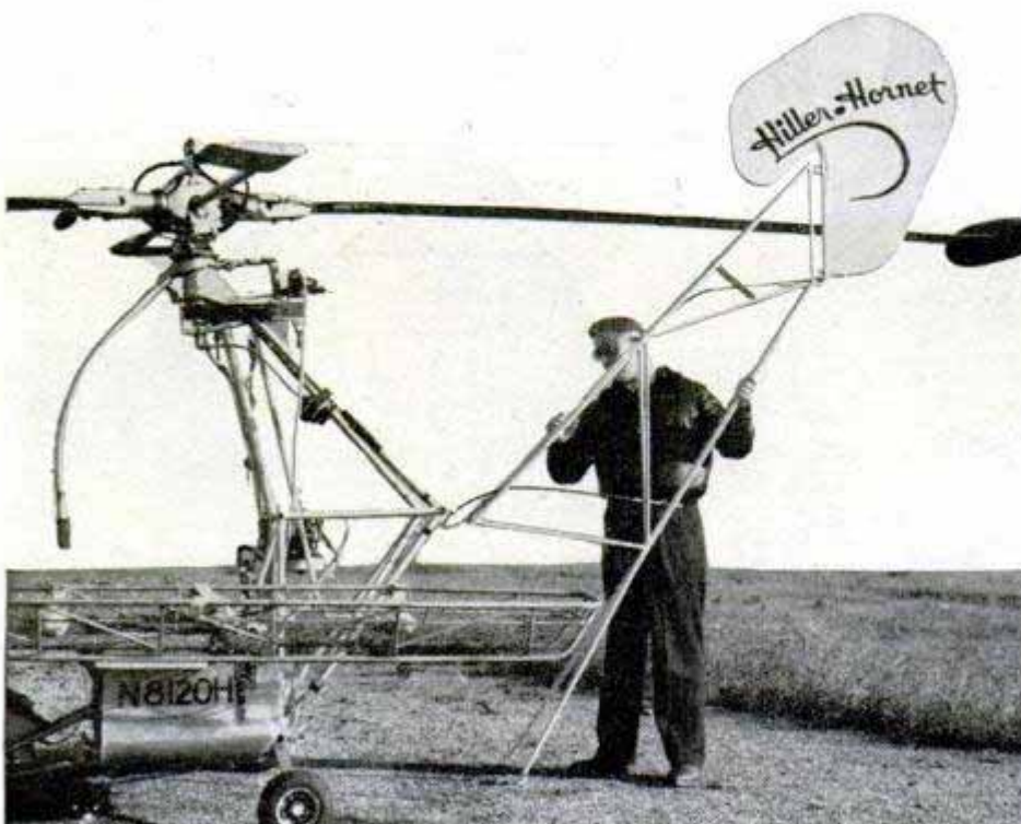
Facilitating storage, tail can be taken off in three minutes
