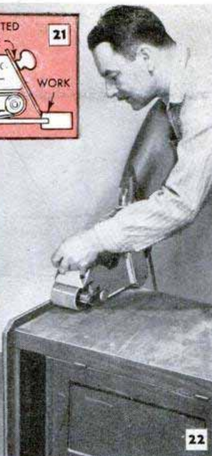
FLUSH RIGHT SIDE OF MACHINE PERMITS SANDING INTO CORNERS
