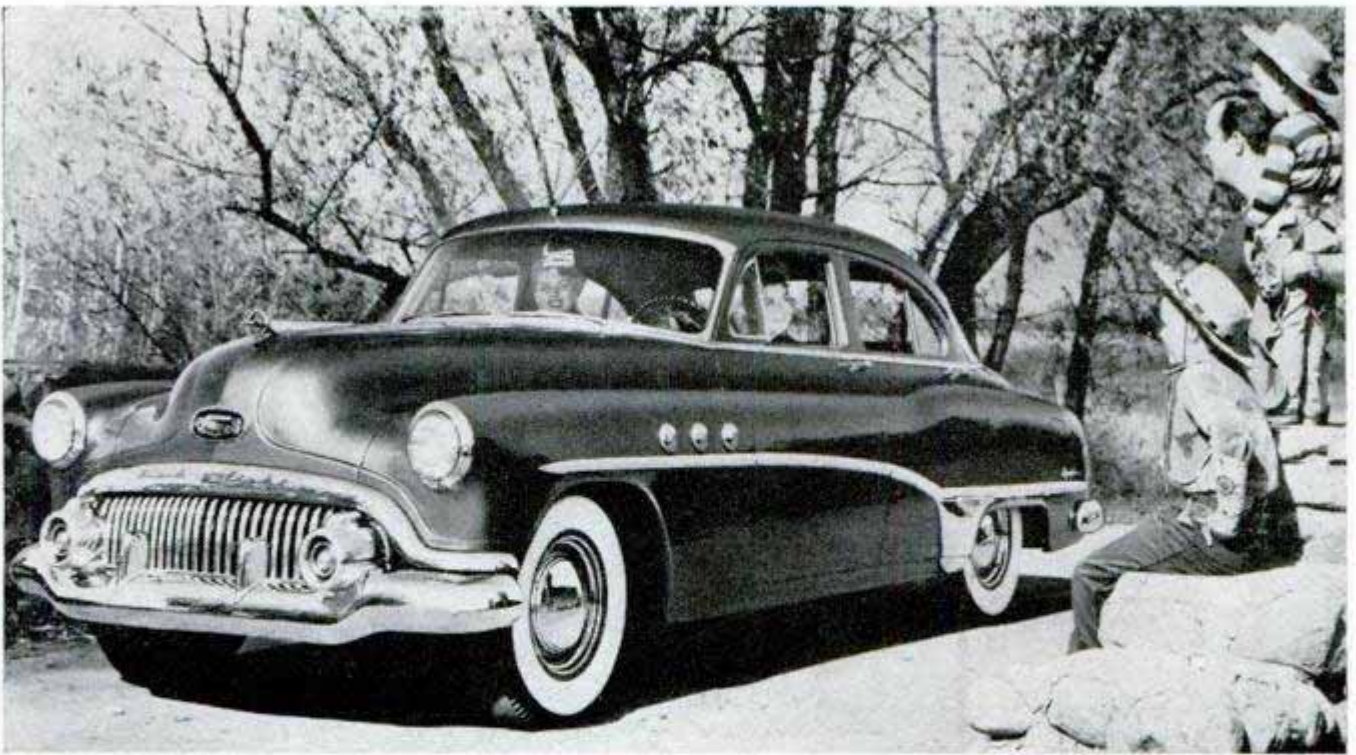
Four-door '51 Buick Special has new chassis and body including the Roadmaster's distinguishing "sweepspear"
