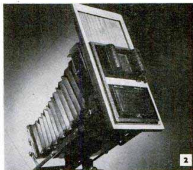
Above, the roll-film adapter in position for taking a horizontal picture. Panel has been moved down to bring film holder in position for exposure. Below, the camera-back adapter being checked for correct fit
