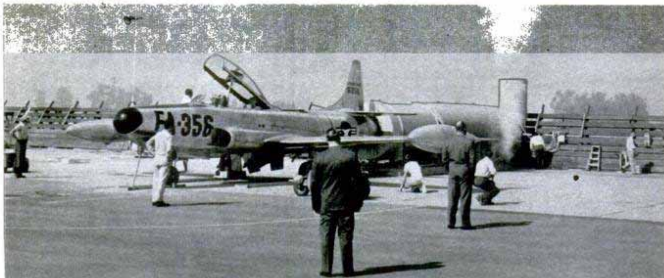
Front section of installation behind F-94 is the Lockheed-designed adapter. Silencer, at rear, is longer
