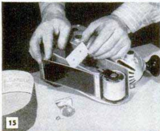
HUMP SHOE IS FAST FOR SPOT-SANDING JOINTS OR OTHER RAISED AREAS
