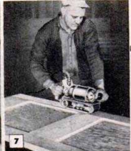
7 25-POUNDER CUTS ABOUT TWICE AS FAST AS LIGHTWEIGHT UNIT
