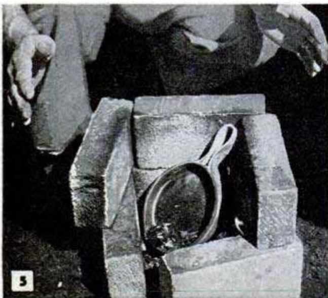
The work to be fired should be placed inside the improvised kiln, partly in the red-hot coals
