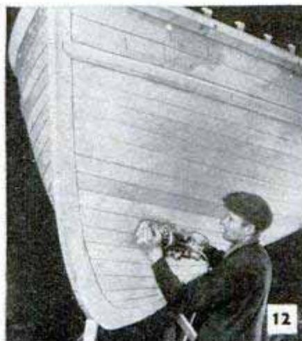
BELT SANDER IS A MUST FOR SUCH JOBS AS SANDING BOAT PLANKING
