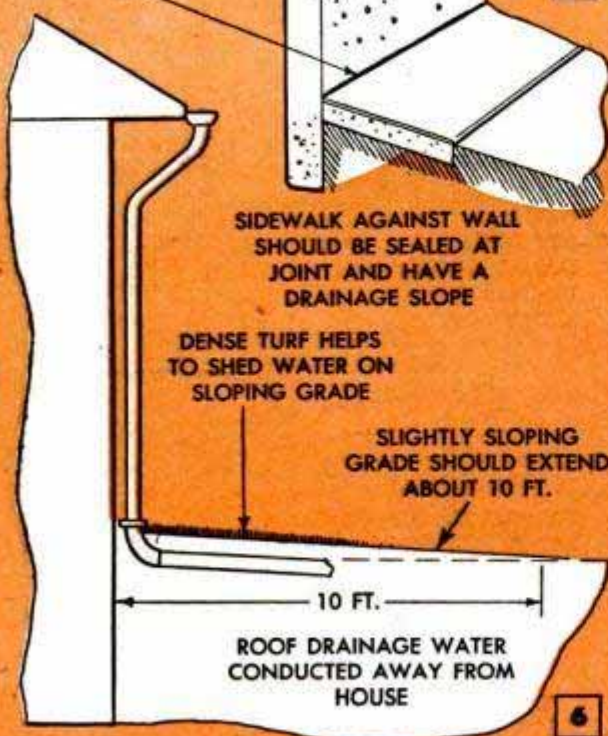
HOT TAR OR ASPHALT-MASTIC SEAL
