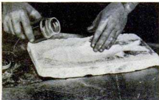
Plaster of paris is poured over the fish to make an impression mold as shown above. Below, the impression mold is oiled before the plaster casting is poured
