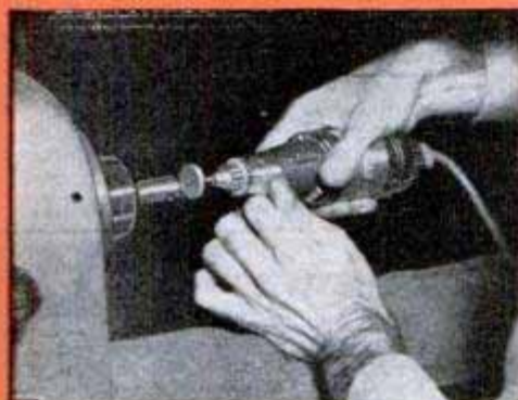
POLISHING work, with rubber bonded polishing wheel. And the CRAFTSMAN Rotary Tool can buff, rout, and drill, too!
