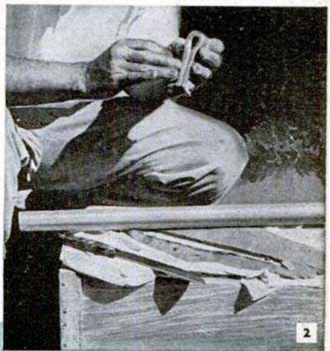
Roll the clay to a uniform thickness and then cut and bend a strip to form the skillet handle
