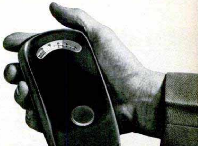
New type Geiger counter, not much larger than a hearing-aid case, is designed expressly for civilian use
