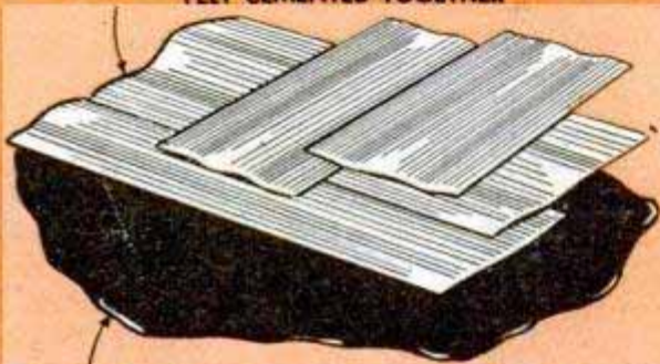
HOT TAR OR ASPHALT ON CONCRETE
