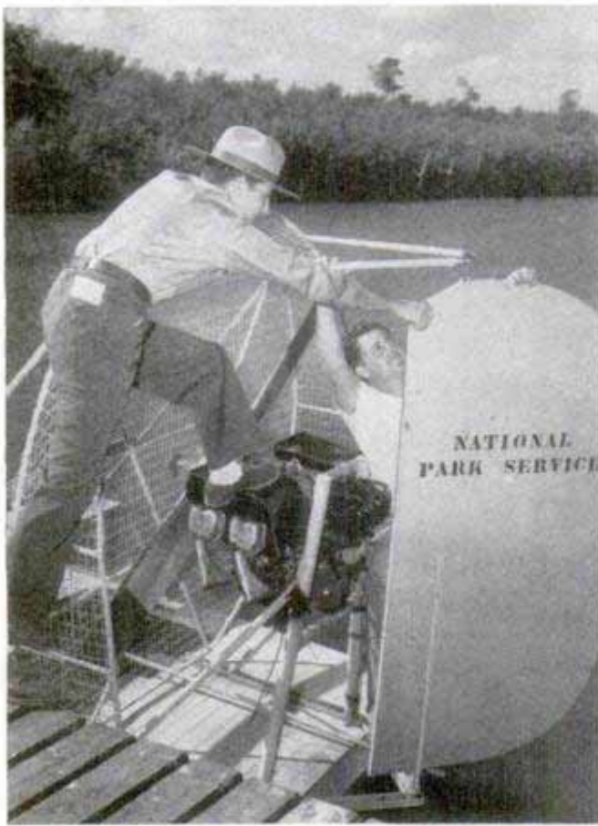
Ranger Ralph Maxwell and mechanic Jim Parker attach rudder of airboat after overhaul job. The boat has a sledlike hull with airplane engine and propeller
