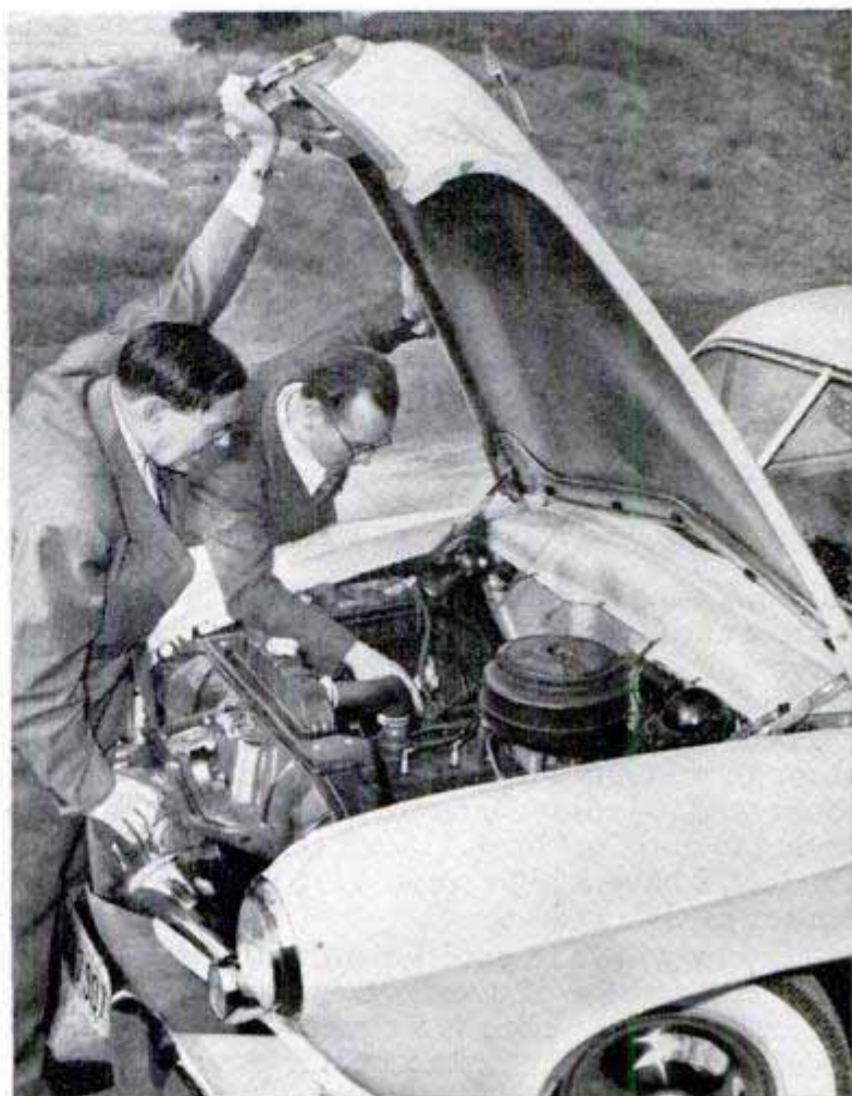
The Henry J's six-cylinder engine built by Willys is only an 80-horsepower job but plenty powerful for weight of car. Below, this high power-to-weight ratio gives the car good maneuverability, especially on rough and winding highways
