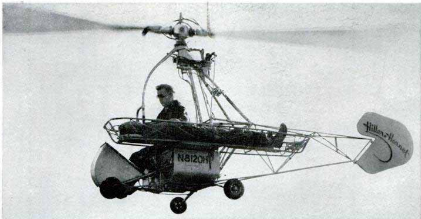
In one of the versions now being built, the jet rotary-wing craft carries a pilot and one litter patient
