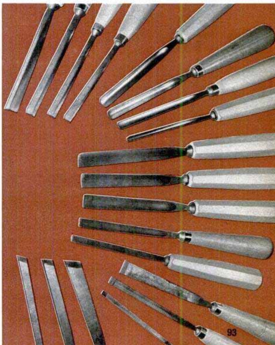
Above, Price holds a female Polynesian head he carved from a koa block and rubbed to a deep mahogany. Below, a typical set of advanced wood-carver's tools. From top to bottom: V-tools, deep gouges, shallow gouges, straight chisels and skew chisels
