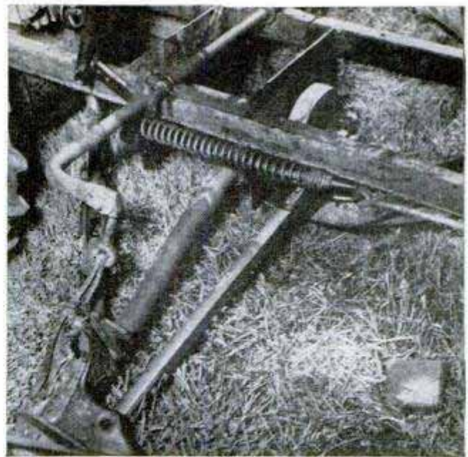
Spring-loaded raising and lowering linkage is operated by a ratchet-type implement lever mounted on tractor frame. Parts are connected by flat-iron links
