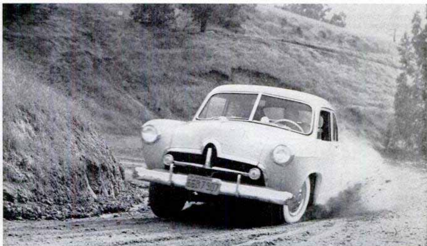
The Henry J's six-cylinder engine built by Willys is only an 80-horsepower job but plenty powerful for weight of car. Below, this high power-to-weight ratio gives the car good maneuverability, especially on rough and winding highways
