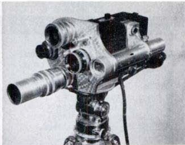
Lens turret and side-mounted adjustable view finder give the professional touch to a war-surplus camera
