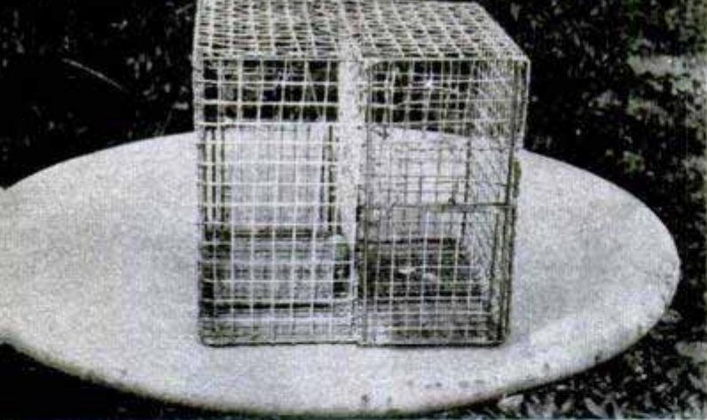
Doors on this trap snap shut when bird steps on a treadle. It has two compartments for snaring birds
