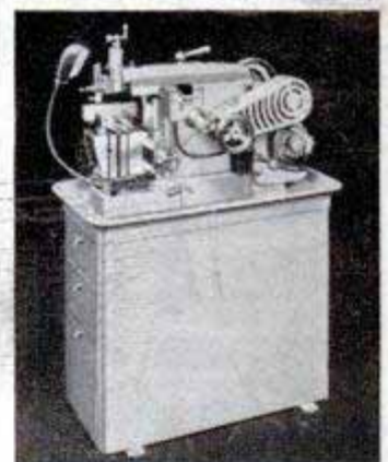
Steel stand for shaper—3 drawers and built-in chip pan.
