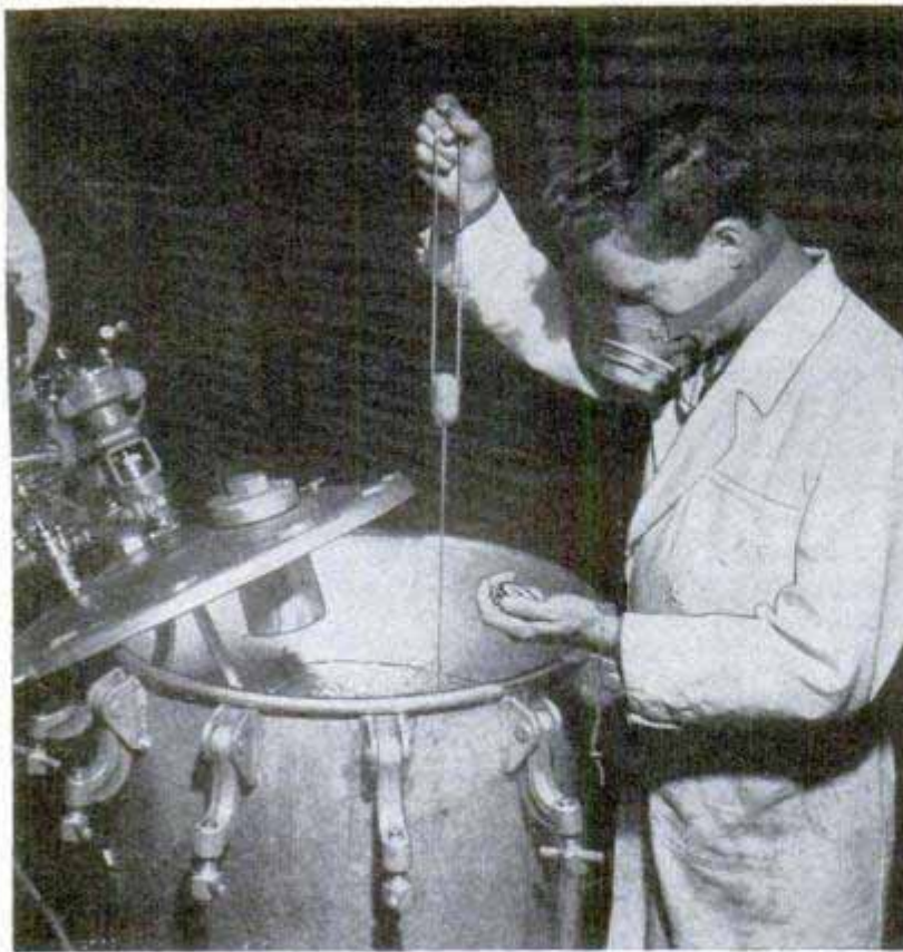
Masked worker tests viscosity of metallic brew used to spray fabric used in lining of coat shown at right
