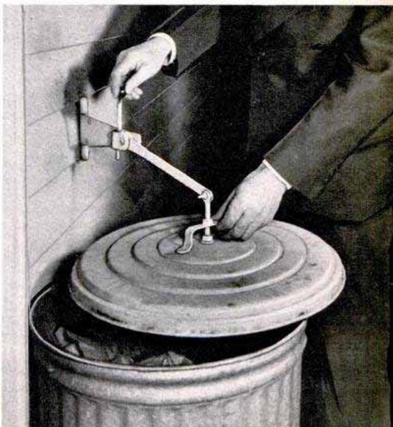
Below, Mathias took time out from his electrical hobby to make this crank-down, dogproof garbage-can lid
