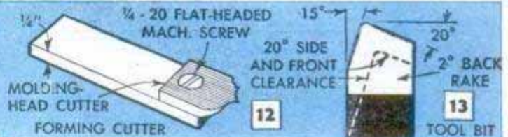
Beads and spirals are turned with a molding cutter mounted on a holder as in Figs. 10 and 12. Work longer than 4 in. should be supported on ball-bearing tailstock center as in Fig. 10. Short pieces are chucked as in Fig. 9
