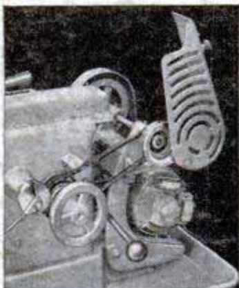
Guards on all belts and pulleys. Quick-acting belt tension release.
