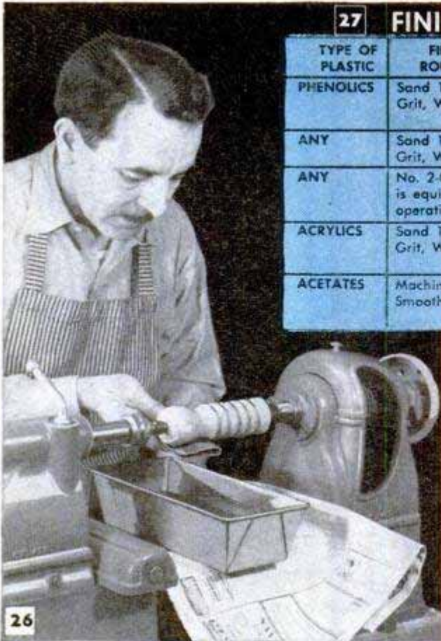
26 Wet sanding removes the tool marks and smoothes the surface ready for buffing and polishing operations
