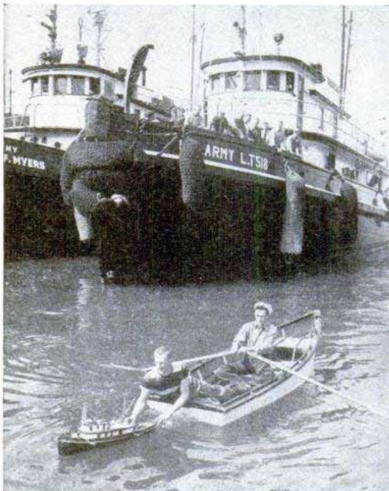
Little tug is steered by impulses sent out through the radio antenna in the foreground. It pulls its own barge, loaded with an anchor. Below, the model is cast off beside its big brother
