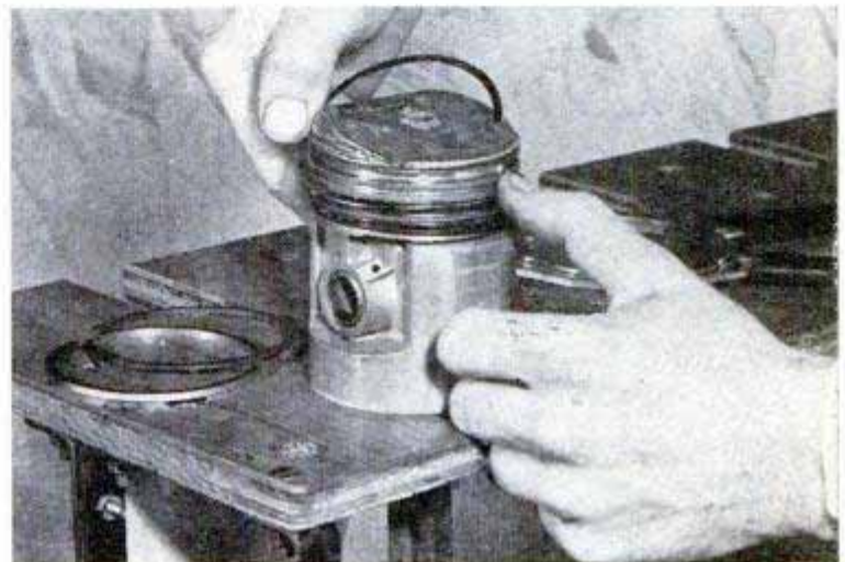
Center, installing chrome-faced, oil-stopper rail. Below, left, detail of three-ring set showing photomicrograph of top compression-ring edge, right. Solid chrome over thread finish gives highest resistance to wear
