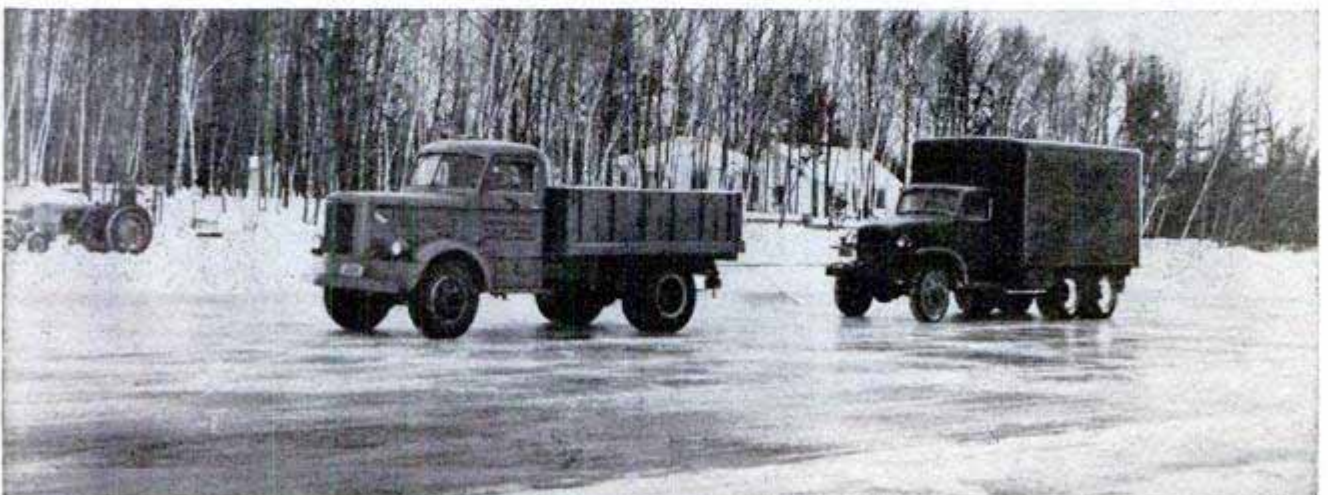
Dynamometer truck is towed on ice during traction test for University of Wisconsin's Truck Research Project
