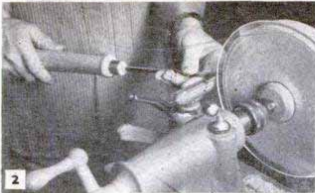
Chucking plastic disks with hardwood follow block
