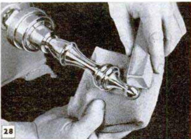
28 Above, high polish is easy to produce with buffing compounds. Below, use steel wool on wood-plastics
