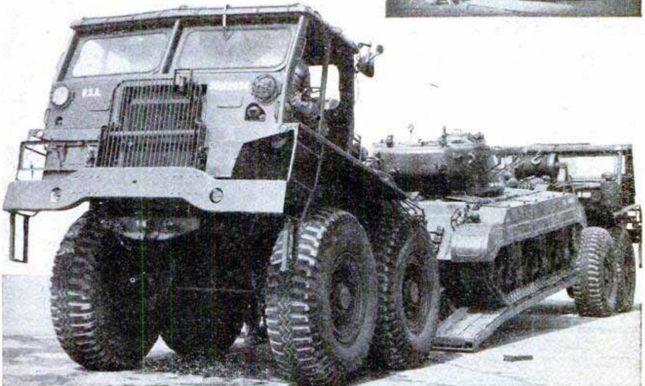
Below, T-8 transport has just "broken apart" and will pull away to allow tank to be unloaded; it can carry a heavy tank
