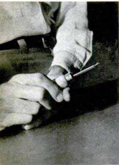
Left, special tool for punching V-shaped eyes in carved pipes was made by Ernest Mehaffey, Bertram craftsman, from a stainless-steel tube sliced off at the end. Right, meerschaum Foreign Legion skull pipe. Below, carving of a full head like this one of Franz Liszt takes 25 hours of labor. Tool is end of file with a needle point
