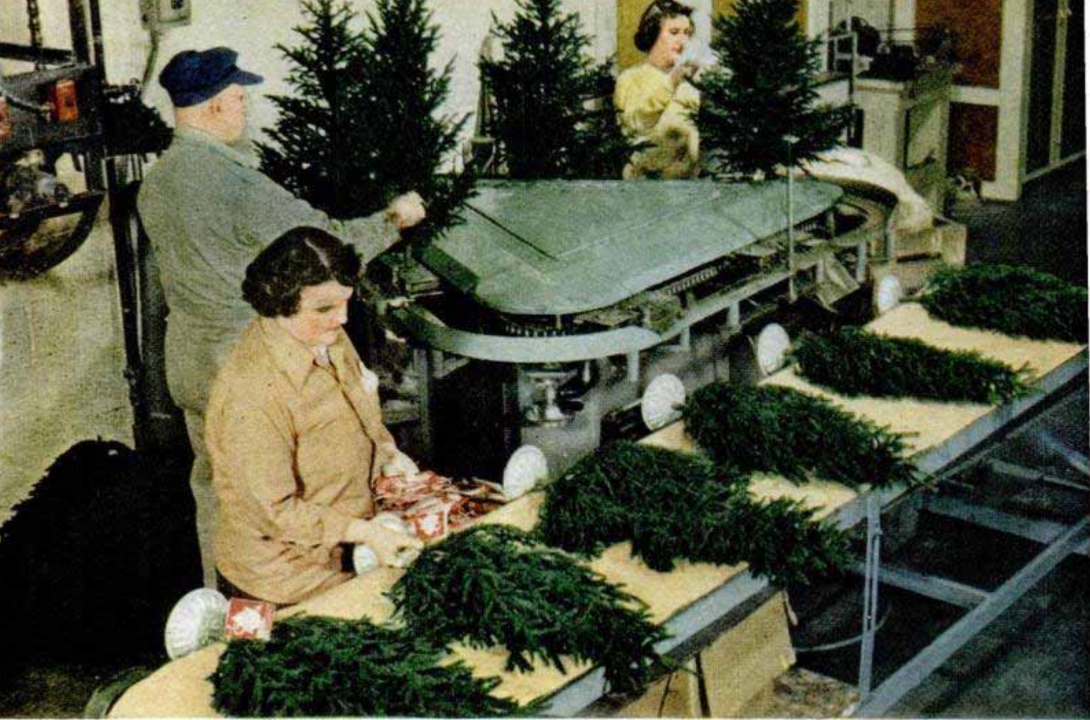
Trees circle the "merry go round" machine which installs the metal stands and fills them with an artificial sap that retards the dropping of needles. Trees are produced in three colors—green, silver and white. Below, Halvorson's daughter June trims a white tree
