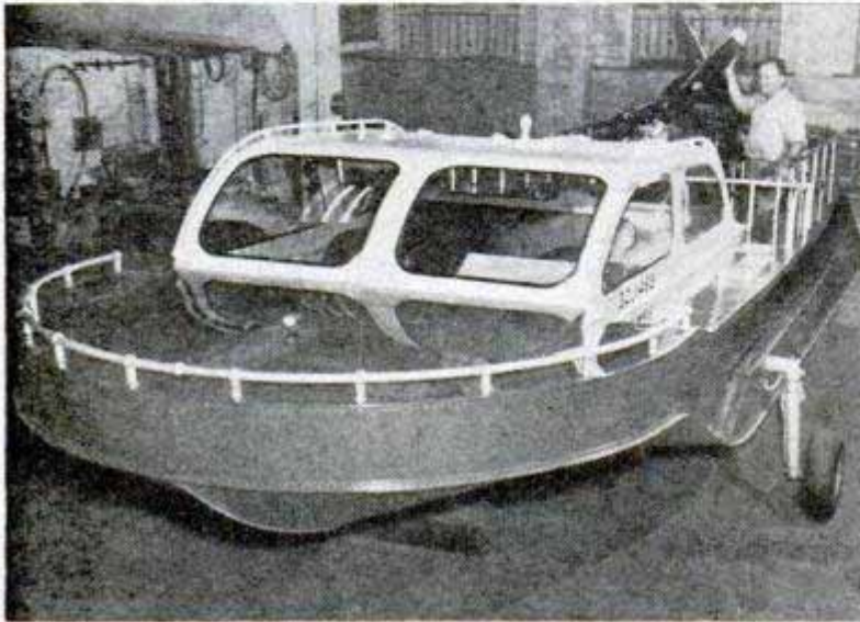
Built of aluminum, the boat is 36 feet long and weighs only 3200 pounds. There's room for pilot, copilot and five others
