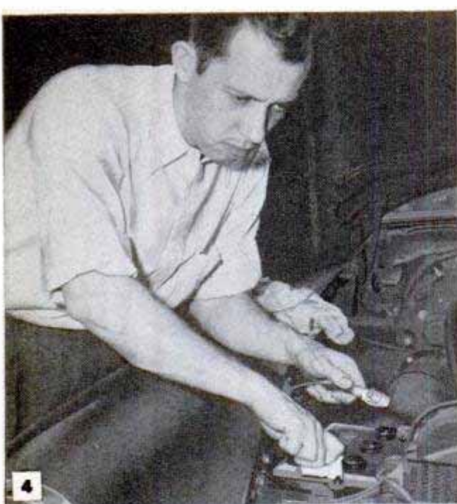
Be sure battery cables and posts are not corroded. Brighten with sandpaper and then apply baking soda
