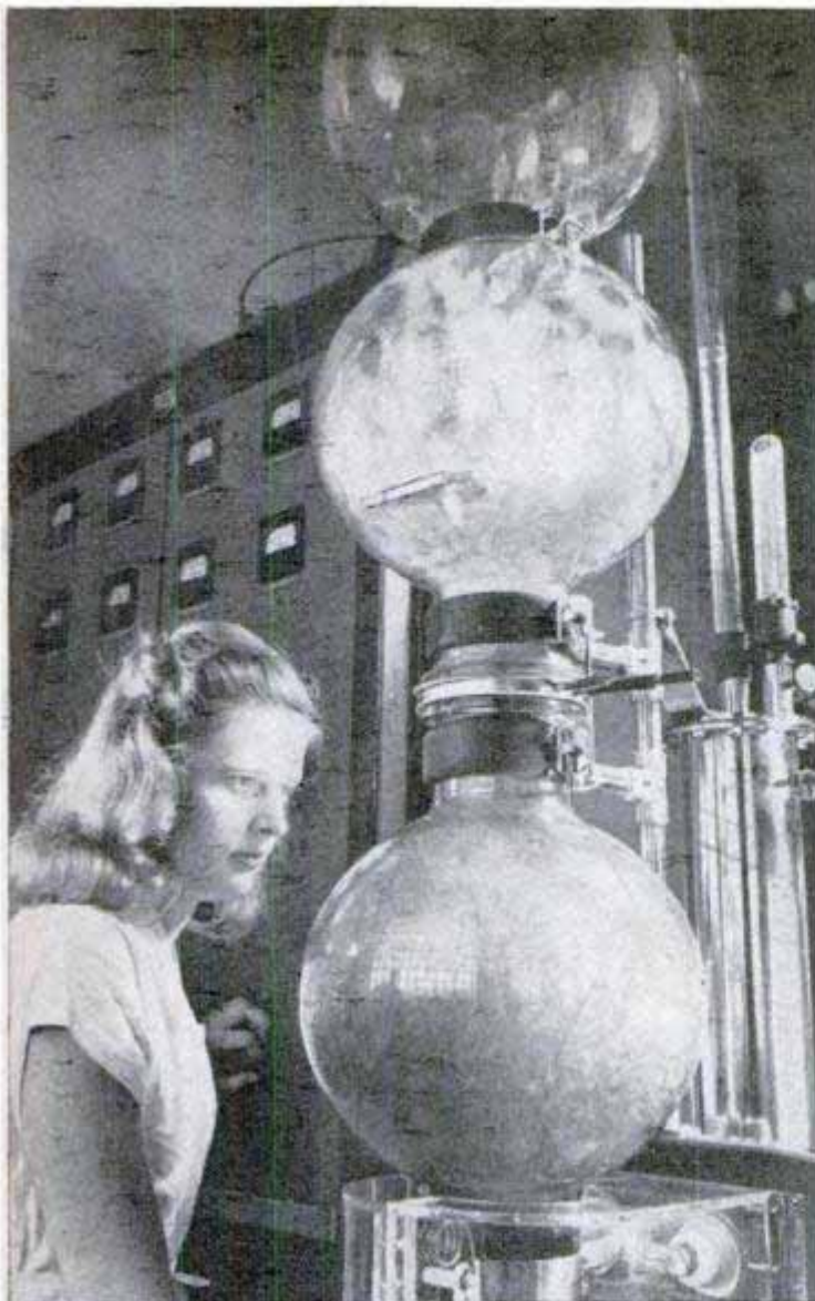
Drying time of penicillin has been reduced from 24 hours to 30 minutes with high vacuum. This bulbous device concentrates solution prior to final drying. Opposite page, the three basic types of vacuum pumps
