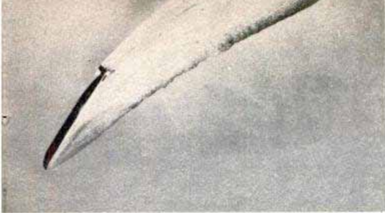
Model of torpedo dives toward bottom of test tank instead of running along the surface. Experiments enable designers to change model to correct faults
