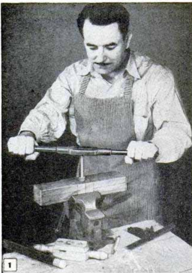
1 ABOVE, TAPPING IS DONE FIRST BEFORE MAKING SPINDLE. BELOW, CHUCKING ASSURES A TRUE START
