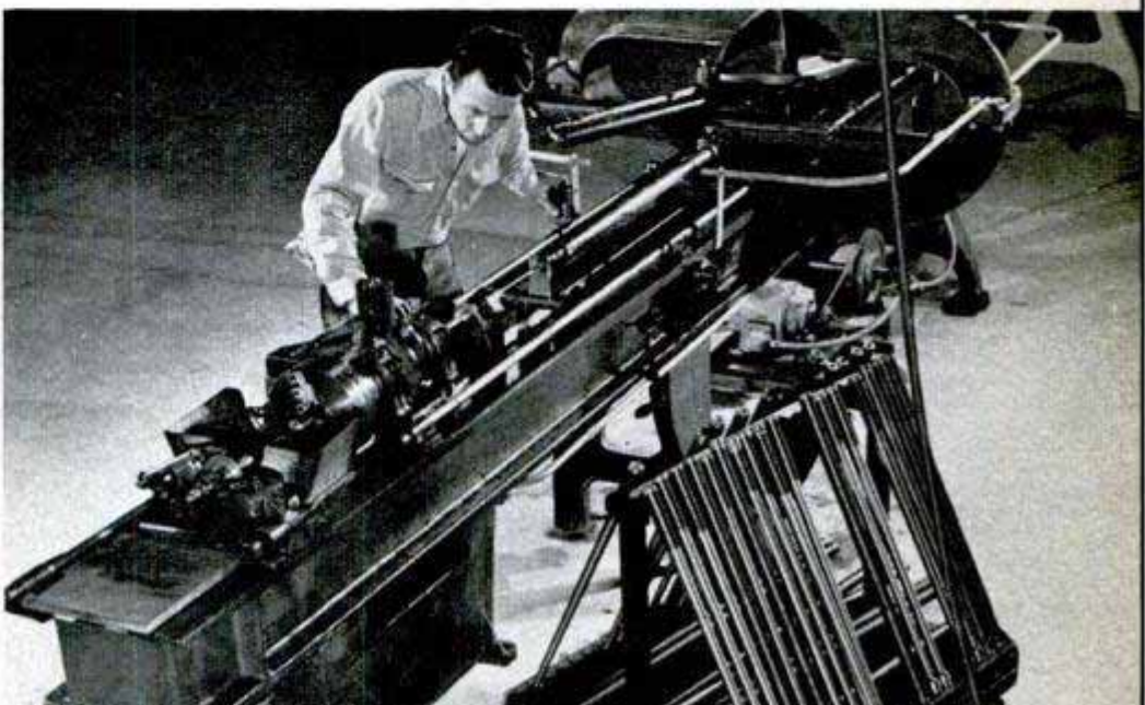
In next step the barrel is revolved against a hollow drill to produce the bore. The machine has split-hair accuracy. Below, the rifling machine produces the six narrow lands and six wide grooves inside the bore
