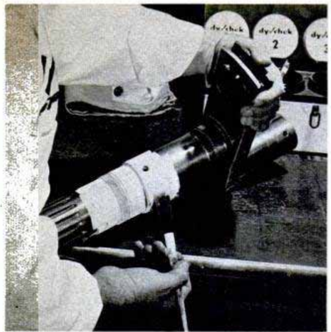
Kit contains the dye liquid, cleaning solutions and the white developer. Right, after dye has penetrated any cracks, white solution is applied to bring dye back to surface. Below, dark line shows crack in a crankshaft
