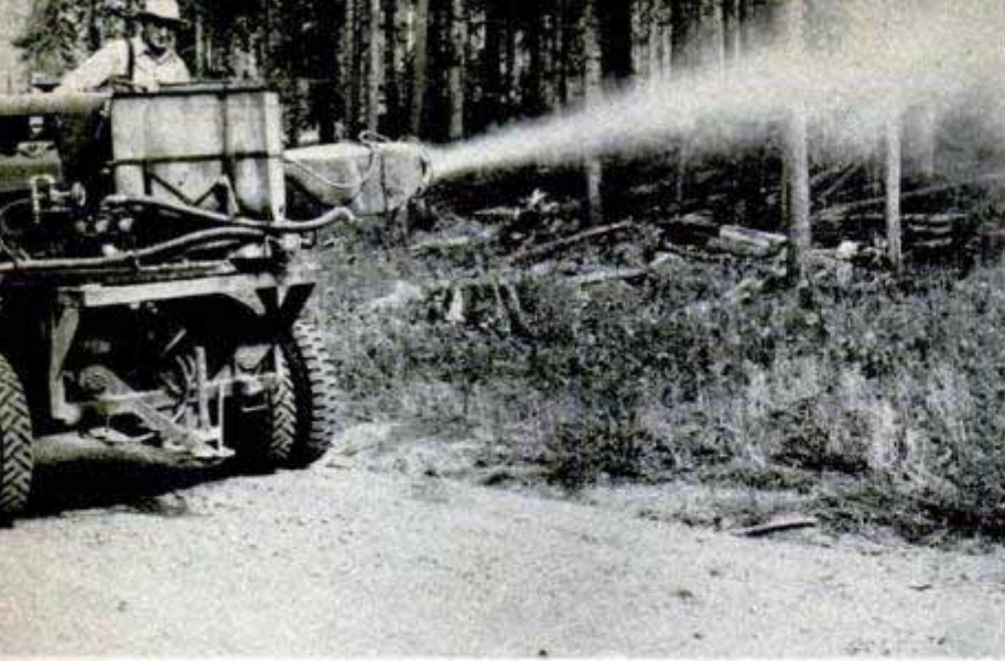
Turntable from hook-and-ladder engine is used on this roadside sprayer which fires a weed-killing fog at 145 miles an hour
