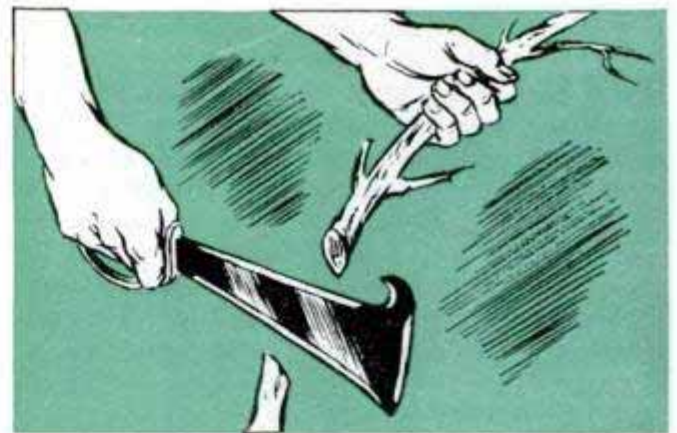
Two other uses for the combination trail knife. For slashing cuts use long edge as shown above. Below, for clearing trail in heavy undergrowth use the hook
