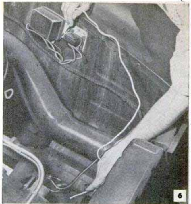
Regulator and generator frames connected together with copper wire determine poor ground connection
