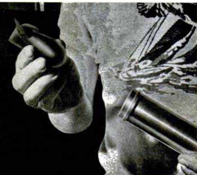
Model of mine goes into steel cylinder to be fired into water. Its behavior will be filmed
