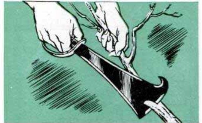
This heavy trail knife has a cutting edge across end of blade, which is useful where space is restricted
