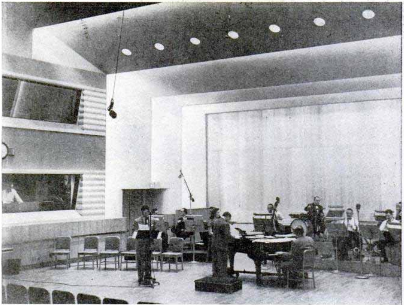
Big band-shell studio gives listeners the impression that they are seated outdoors. All sound is projected forward, then absorbed in one end of room. Below, left, banks of fluorescent lights on lazy-tong hangers have replaced old TV "hot" lights. Drawing shows how the new studios float on rubber bags filled with air
