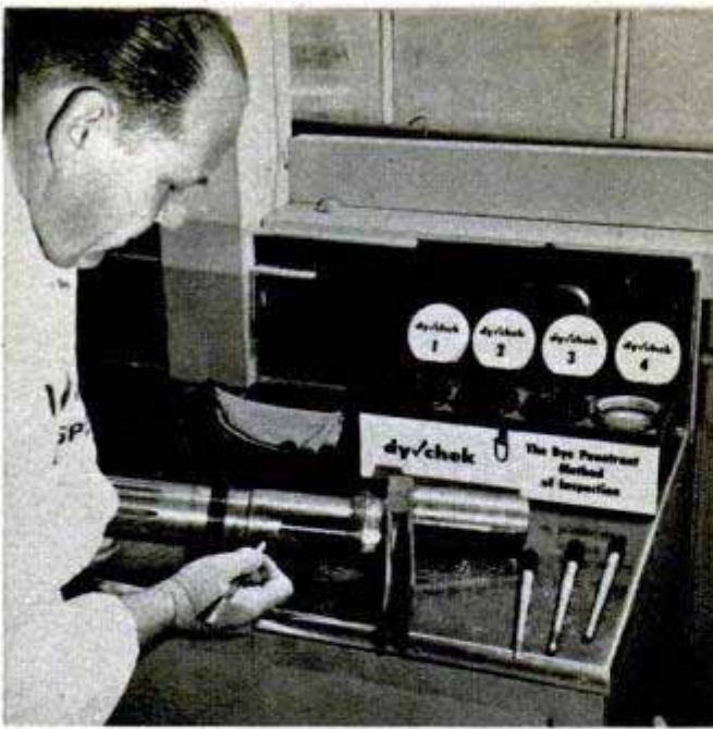
Kit contains the dye liquid, cleaning solutions and the white developer. Right, after dye has penetrated any cracks, white solution is applied to bring dye back to surface. Below, dark line shows crack in a crankshaft
