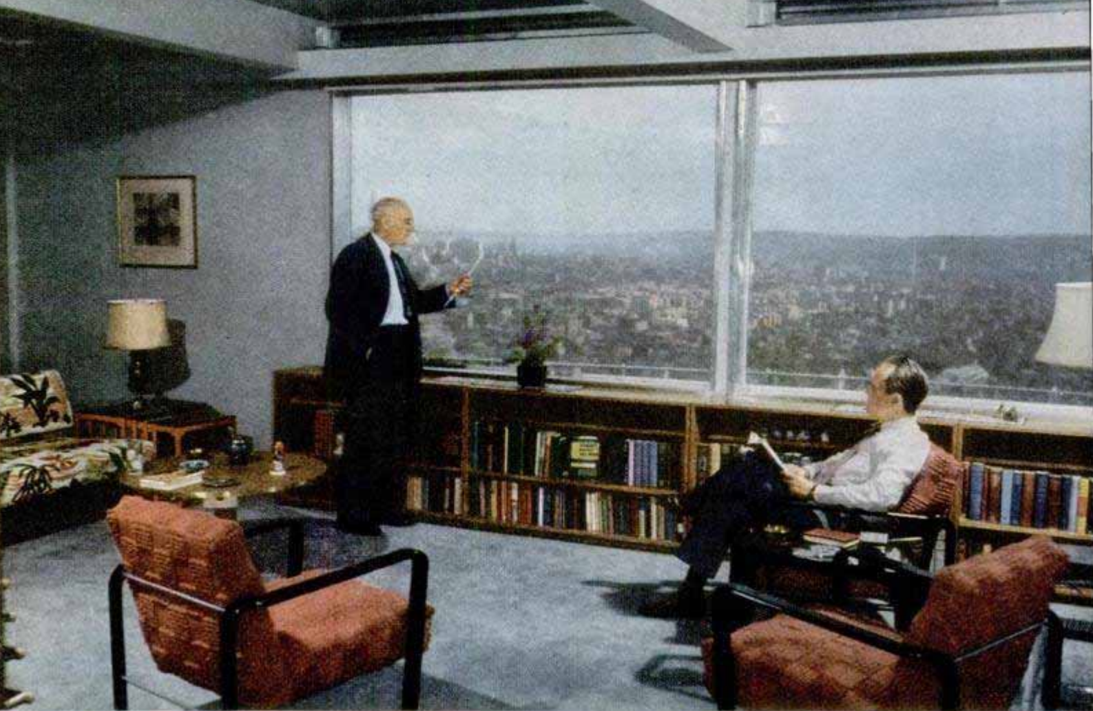
Dr. Clarence A. Mills before picture window explains conditioning system to guest. The heating-cooling cove can be seen above window. Beneath carpet is aluminum foil which reflects heat waves like side walls
