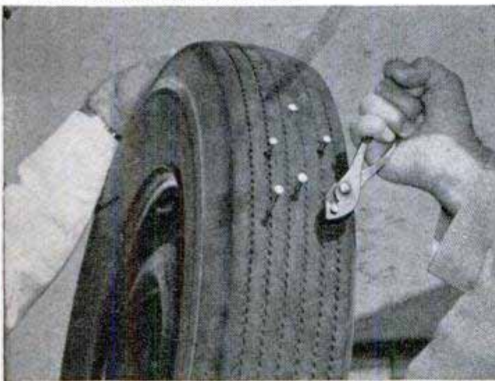
3. Here's how you "fix" a puncture when you have Seiberling Sealed-Air Tubes with patented Bulkheads. Just pull out the nail or other sharp object, and the tube seals itself permanently! No further repairs necessary!
