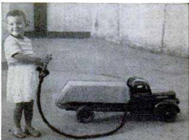
Above, realistic in all details, the tiny Chevrolet truck was built by a hobbyist in Chile. Below, the steering and driving motors are controlled remotely
