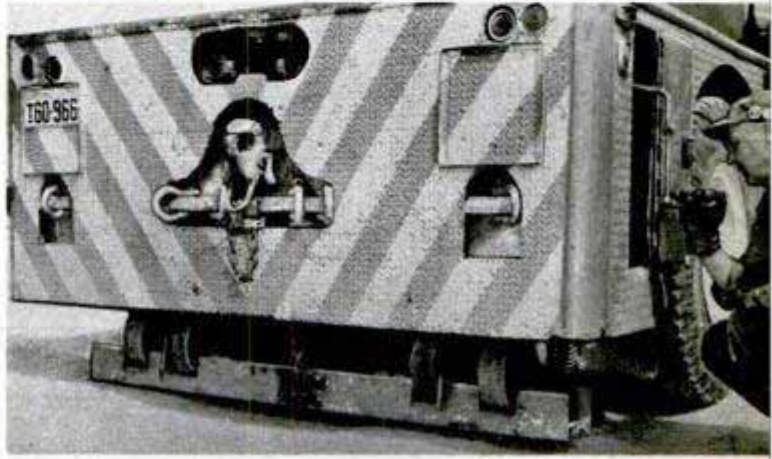
A steel bar at the rear adds stability for a hoist
