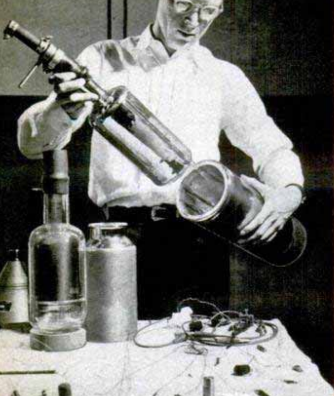
Left, liquid-helium flask is placed in container insulated with liquid nitrogen. The helium is kept in the dark, as light is warm enough to make it boil. Right, comparison of Kelvin, centigrade and Fahrenheit scales
