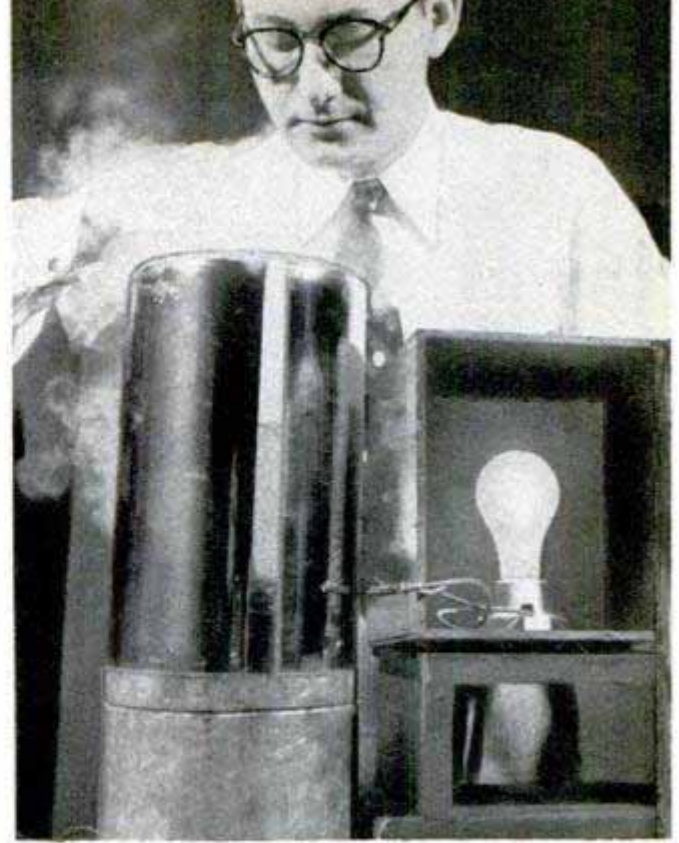
Experiment shows how supercold reduces electrical resistance. Bulb burns dimly, left, but when copper coil, carrying current to bulb, is dropped in some liquid nitrogen, right, the light output increases many times
