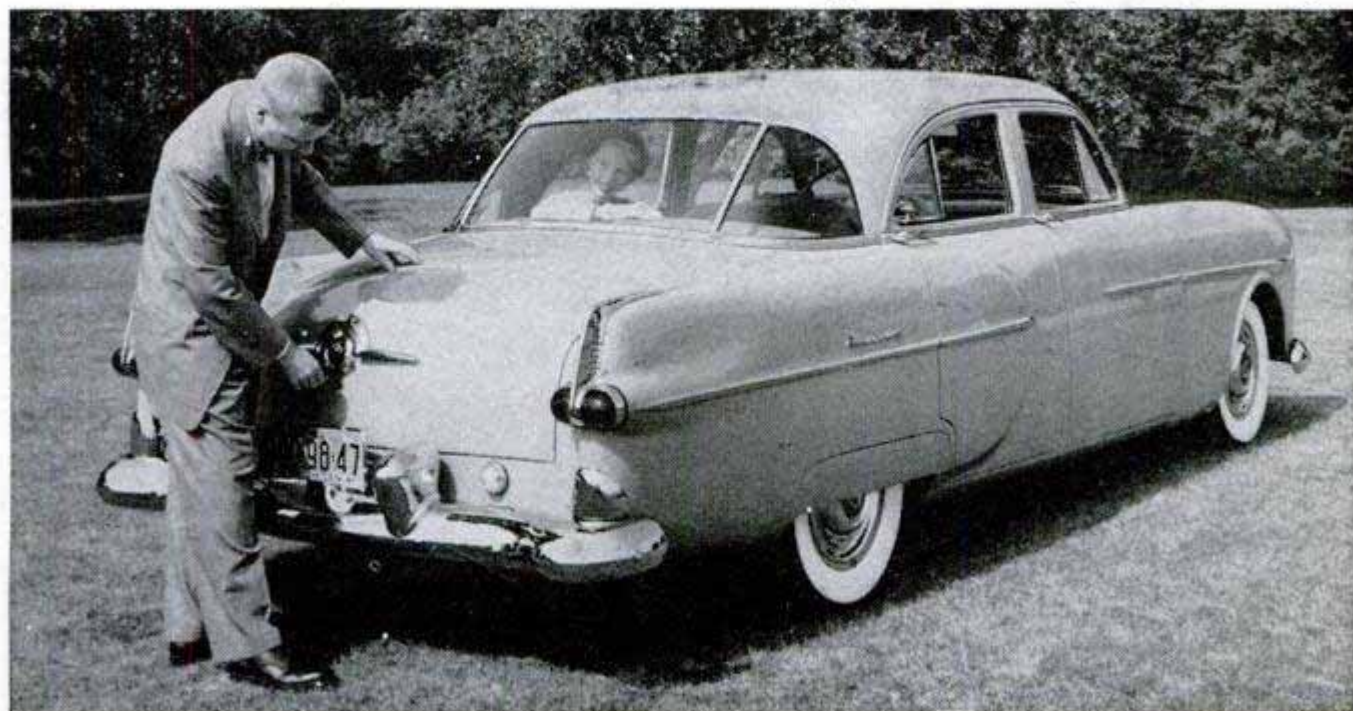
Luxuriously finished, the 300 series four-door is two inches lower than its predecessor and has a rear seat 12 inches wider. The sweep-around rear window increases visibility, and bustle back yields more trunk space
