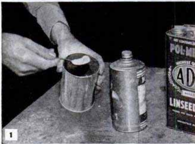
Many finishers prefer to mix their own wood fillers from separate ingredients. Mix in a clean container
