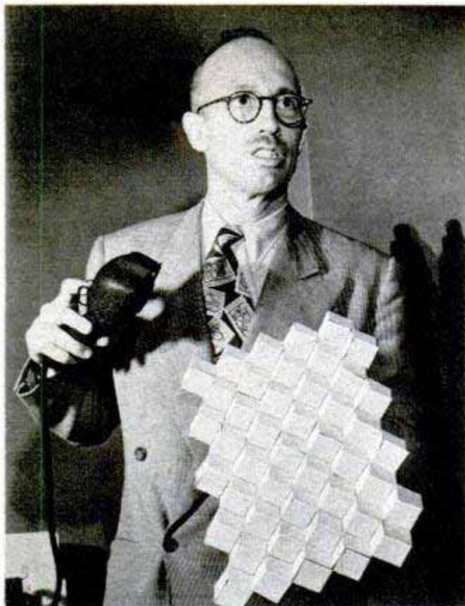
Dr. Geer demonstrates his TV system with enlarged model of screen. The prisms break light into colors
