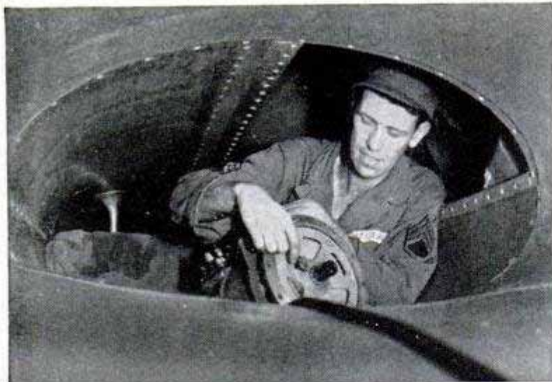
Crewman squeezes through air intake to work on engine while plane is on ground. In the air, the crewmen can crawl along narrow catwalks in wings to inspect any of the six engines
