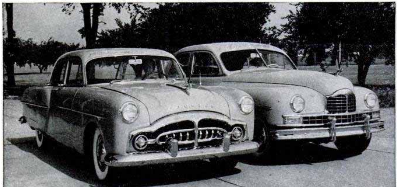
Packard 300, completely redesigned, poses with last year's model. Note lower hood, wider body, higher fenders
