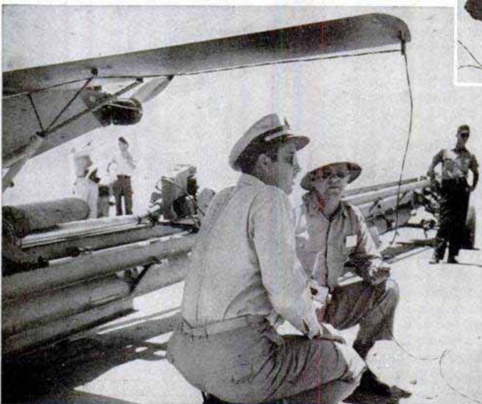
Canvas container holds a half mile of lightweight wire which unreels as the drone zooms toward target
