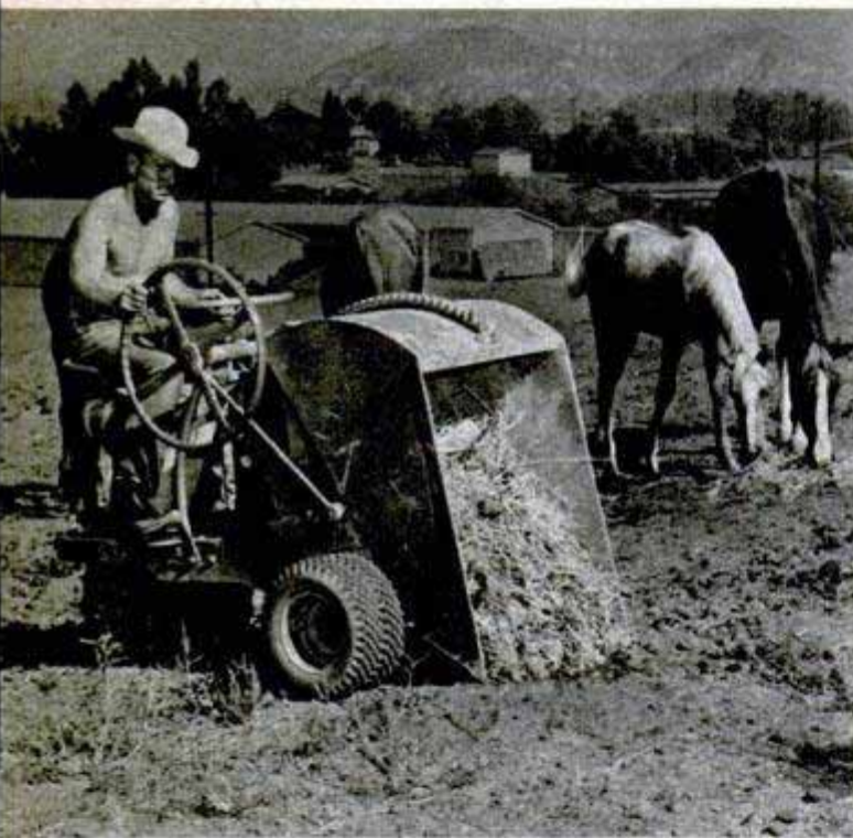
Power buggy for removing straw and debris from the stable travels 18 m.p.h. and carries 13 cubic feet
