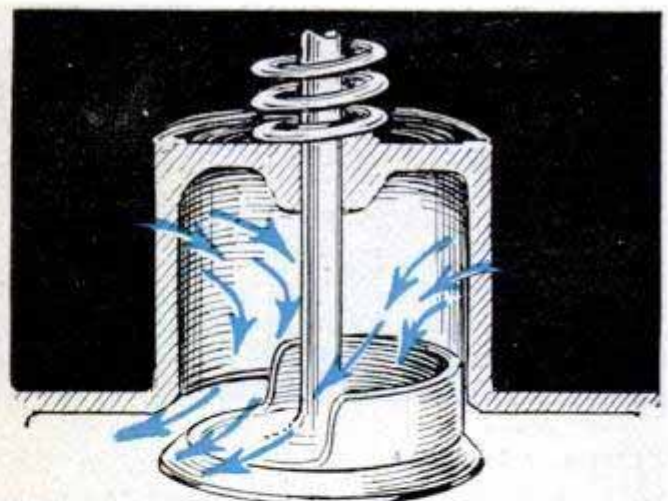
SHROUDED VALVE—AIR MOVES IN ONE DIRECTION ONLY
