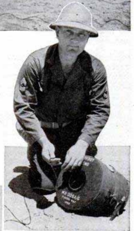
Canvas container holds a half mile of lightweight wire which unreels as the drone zooms toward target
