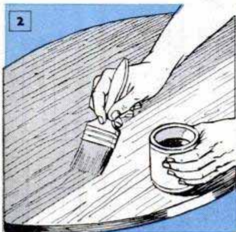
Mix the filler to the consistency of cream and apply to the wood with a brush. Allow to set, then rub across the grain with a coarse cloth. When rubbing turnings, wrap cloth around work and pull back and forth
