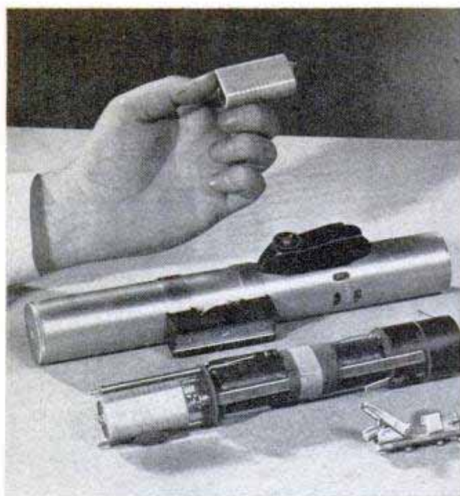
One small battery and a capacitor, shown at right, operate all the flash equipment in the left-hand photo
