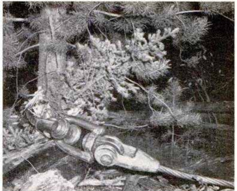
Swivel connected in steel line on each side of the big ball allows it to roll and prevents twisting of the stout lines
