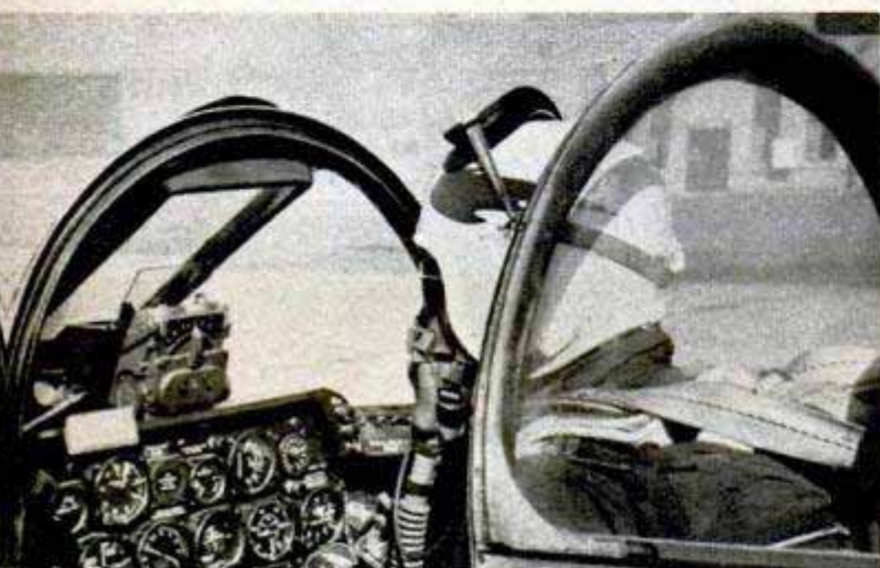
Sturdy shoulder straps hold pilot safely in place during high-speed air buffeting and high-G turns
