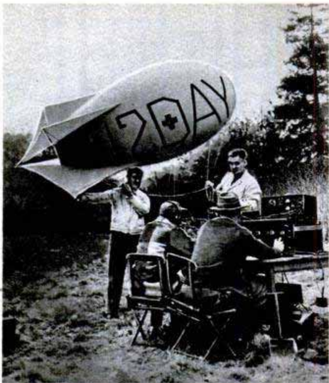
Kytoons support radio antennas high in the air. The Red Cross is testing it for disaster communications
