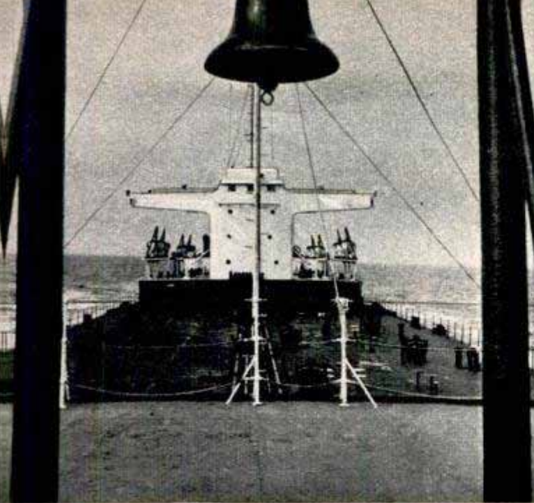
Photo from forepeak shows the "flying bridges" which give Amtank's skipper an unobstructed view of dock
