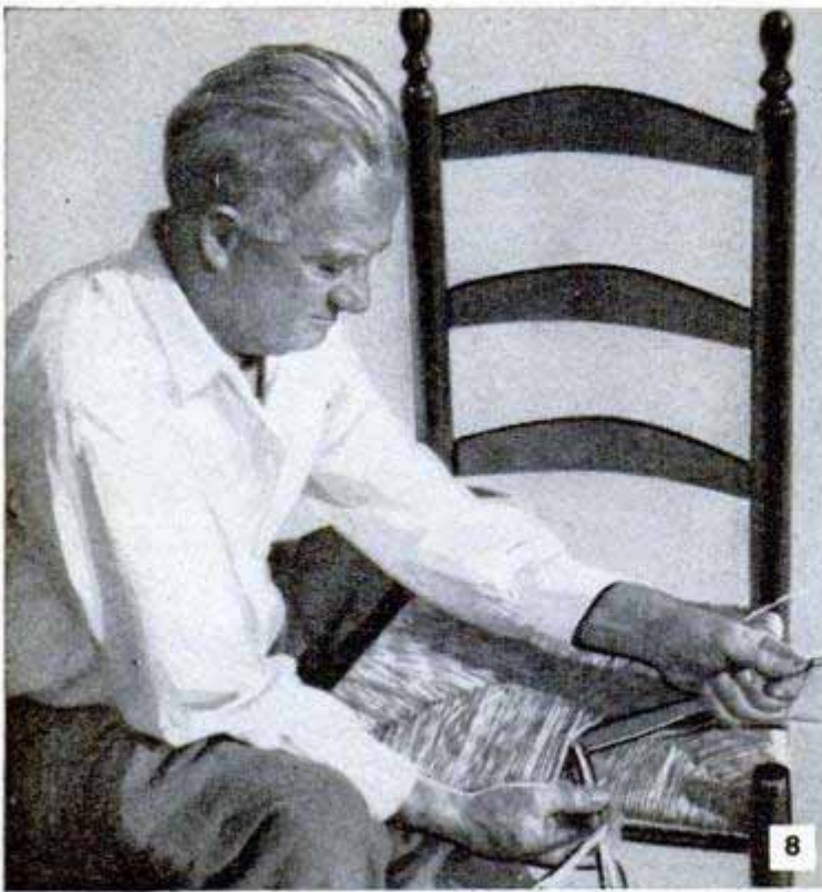
Above, after the weaving is completed, protruding strands on the bottom are snipped off close and the seat is varnished top and bottom
