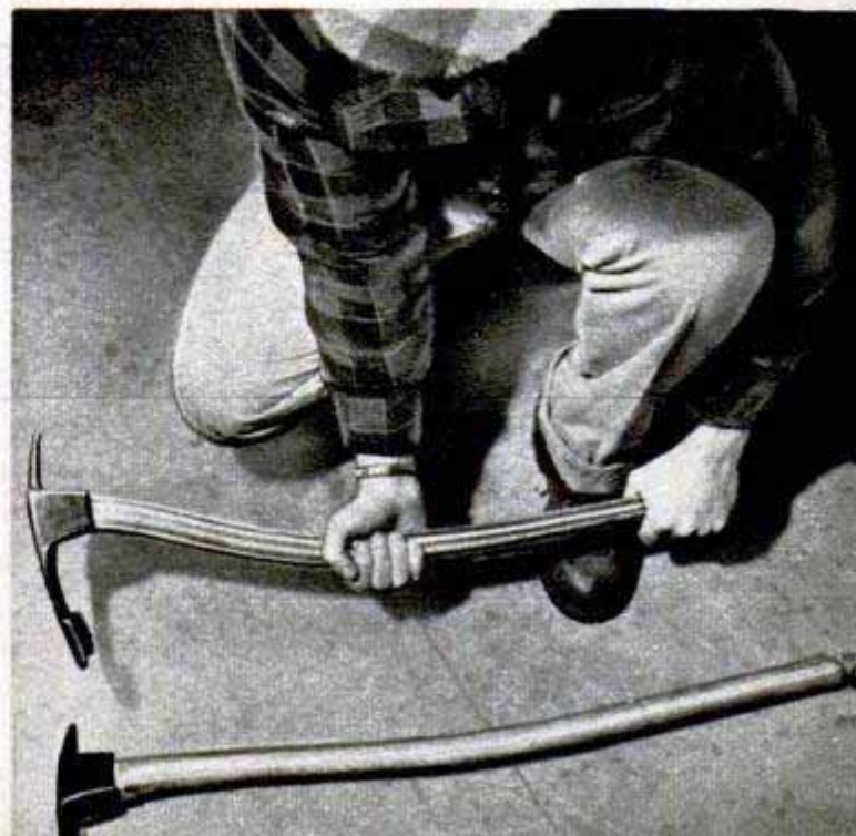
Derecktor adx, held by workman, has a handle which permits better control than commercial type on deck
