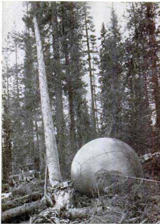
Big steel ball holds line off ground during mowing operation to avoid stumps of large trees logged out
