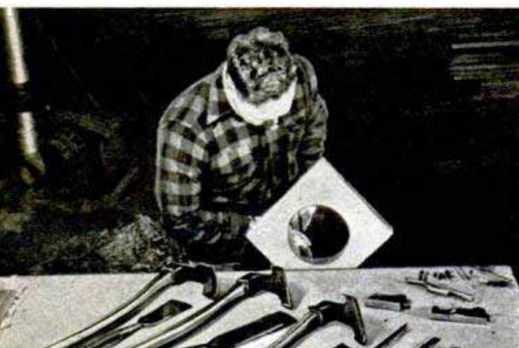
Here are a few of the hand tools used by the expert boatbuilder. They include adzes, slices and planes
