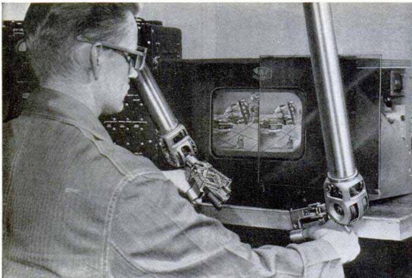
With three-dimensional television, an atomic-laboratory engineer can see to manipulate radioactive materials behind lead-shielded walls. Above, operator views double picture on screen through prismatic glasses and sees a single-depth picture. Below, left, stereo-television camera, remotely controlled "arm" in the center and operator of new-type remote-control board in background. Below, right, close-up of controls
