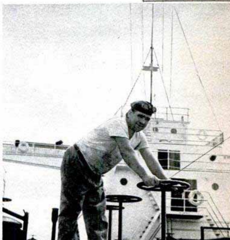
Map shows regular run of Amtank. Below, at sea, the bosun turns a valve to move oil from one tank to another in order to trim the ship
