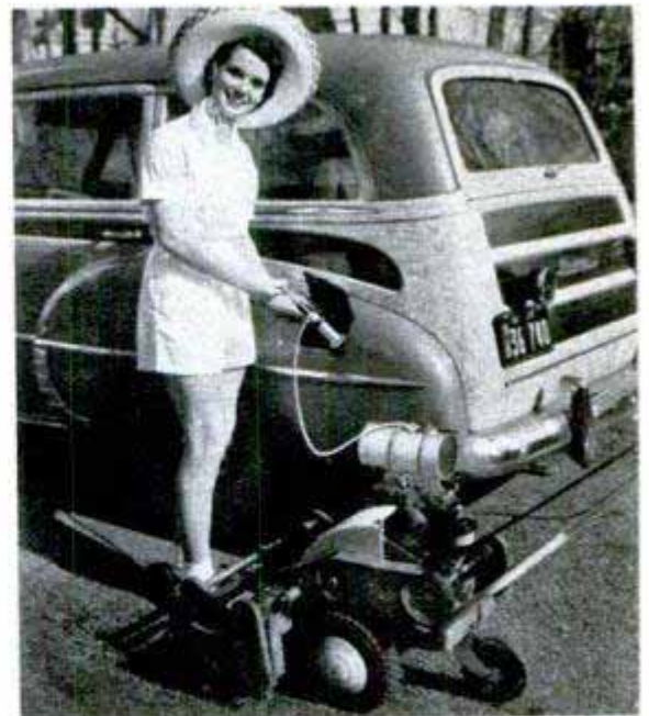
Refueling an outboard is a messy operation if the water is rough, but by using this small pump you won't spill a drop. Right, it's handy for pumping gas from your automobile, too
