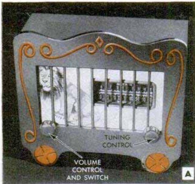
Front view of completed set showing suggested decorations in a contrasting color. The receiver panel and end panels are painted with white enamel
