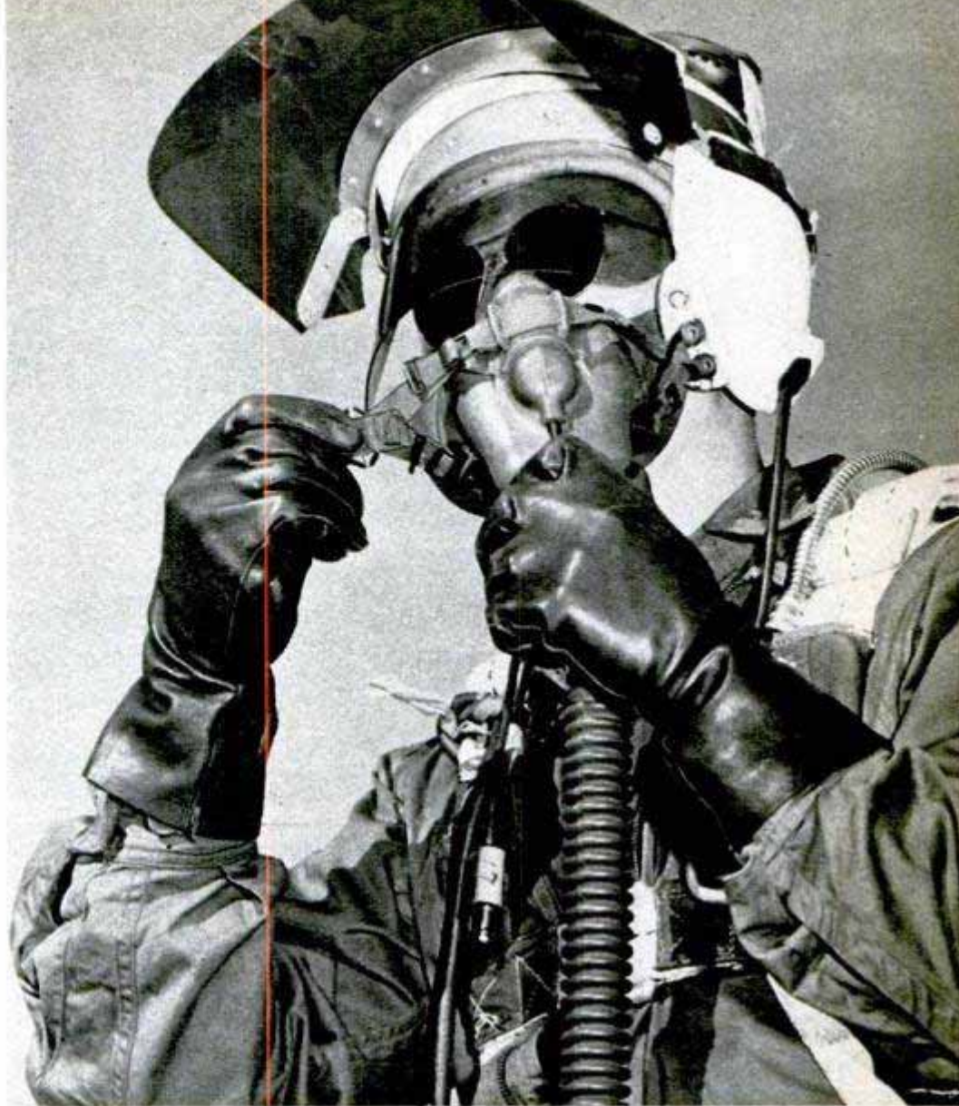
Odd double mask for blind-flying training. Inner shield's amber filter allows normal vision. When outer blue filter shade (raised here) is lowered over inner shield the pilot cannot see. To fly on instruments alone, he pulls outer shield down to where cockpit windows are obscured
