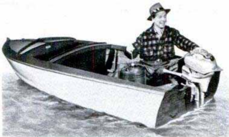
Refueling an outboard is a messy operation if the water is rough, but by using this small pump you won't spill a drop. Right, it's handy for pumping gas from your automobile, too
