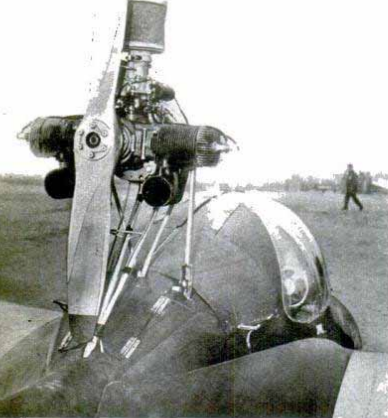
For take-off and to recover altitude, an auxiliary engine is cranked into place on top of an experimental glider. Pulling rope within cockpit starts it
