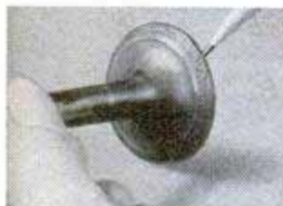
PITTED VALVE FACE
