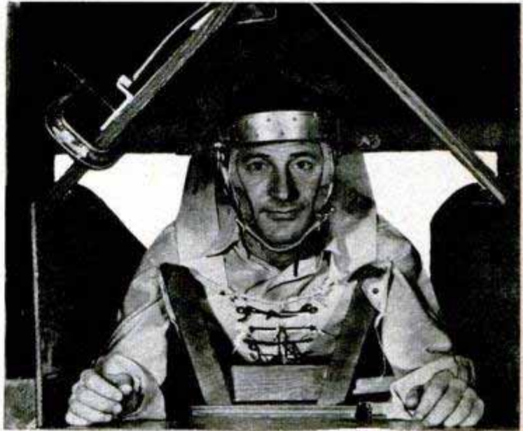
Two kinds of head harness, right and above, tested for prone-position flying proposed for future high speeds
