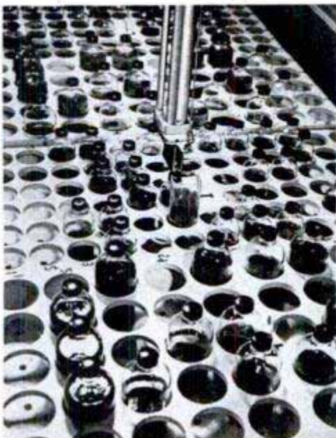
Left, remote-control tongs lift a bottle from radio-isotope storage area. Right, mirrors aid the operator
