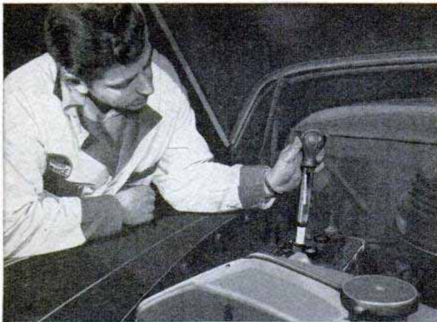
JUST ENOUGH ELECTROLYTE IS DRAWN IN TUBE TO PERMIT FLOAT TO CLEAR BOTTOM
