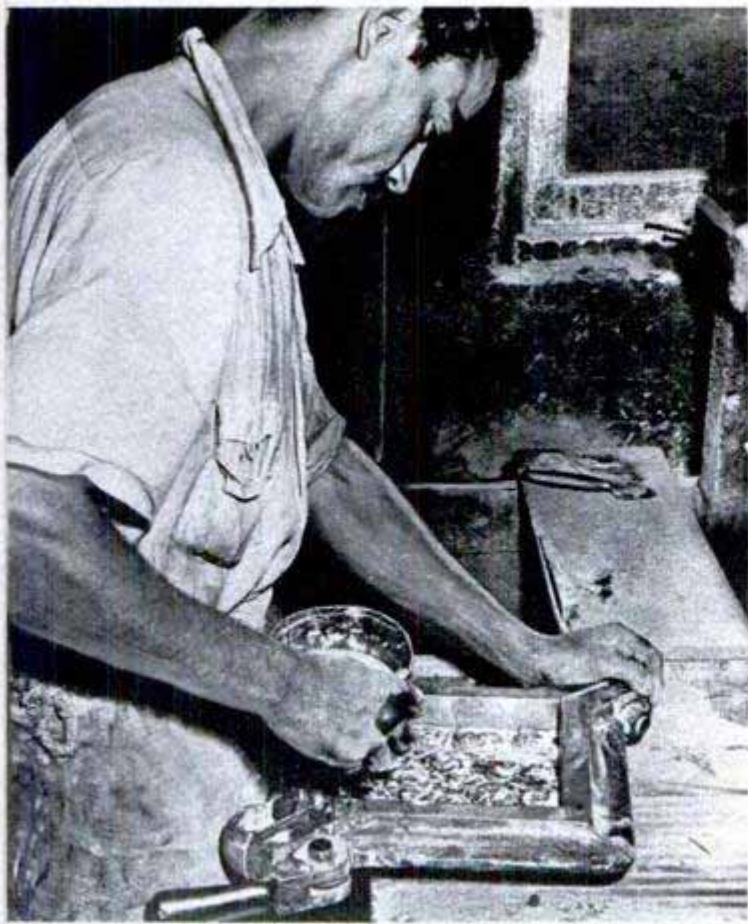
After the first layer, which has the colors and the design, the dry middle layer is placed in the mold
