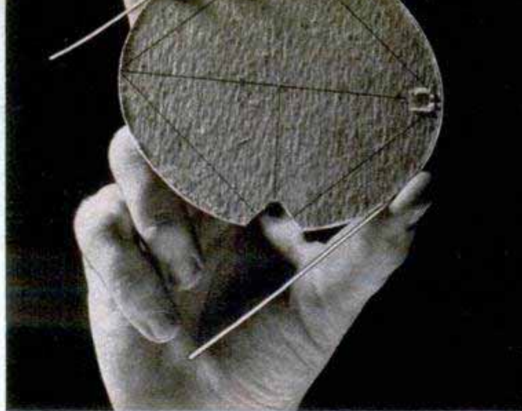
Left, wing ribs are cut from sheet balsa to mathematically figured curves. Right, this slender balsa spar is bent around a template when wet and held with tissue until dry to form the outline for circular rudder
