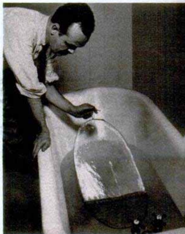
Above, left, a hypodermic syringe dispenses cement in tiny quantities. Right, microfilm is lifted from water surface with a large wire loop. Below, left, microfilm sticks to anything when wet so this brush is used to moisten fabric being mounted on propeller skeleton. Right, guy wires are one third as thick as a human hair
