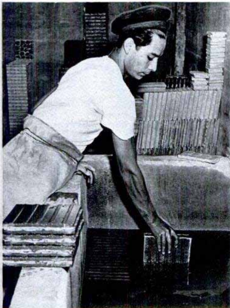
After a 12-hour period of air-drying, the tile goes into a bath of water and salicylic acid for 24 hours
