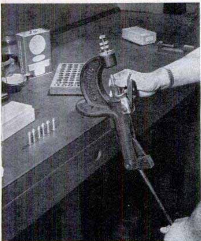
Left, with this hand-loading device, the gun experts can duplicate any of thousands of cartridges to make laboratory tests. Right, the tumbling machine that helped solve the mystery of the exploding freight car
