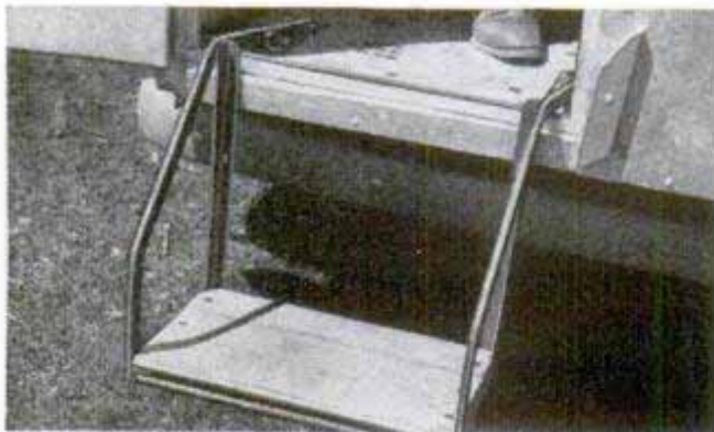
Above, novel step-seat folds inside to form a comfortable seat, thus making use of all available space. Below, underneath view of body offset and the angle-iron framing which fits inside the bed of the truck
