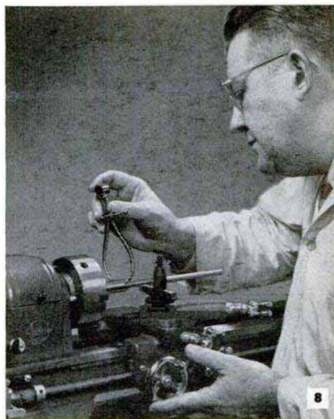
Above, always stop the lathe before checking the size of the work with calipers. Below, when transferring measurements with calipers, hold the tool so that the fingers are in contact with the legs
