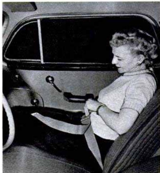
Left, for greater safety, the 1950 Chrysler has a crash pad on the instrument panel. Right, Nash further indicates trend to adopt aircraft safety devices to automobile use by featuring safety belt for passengers
