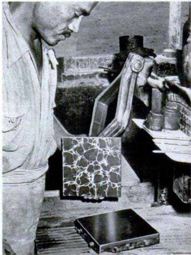
Its three layers now compressed into one, the tile is removed from the form. This is a marbled design
