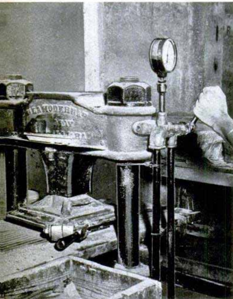
In this hydraulic press, the tile is subjected to a 60-ton pressure. The hydraulic pump is hand-operated
