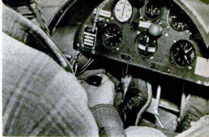
Instruments in Schweizer sailplane which set height record. Knob in center frees it from the tow plane. Below, bundled up in cold-weather flying equipment, Ross, front, and Deibert, rear, start on record attempt
