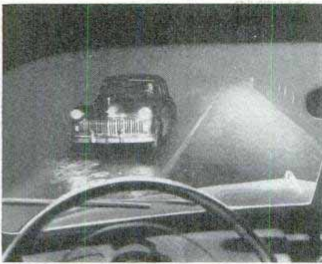
Plastic shades over headlights reduce glare from approaching car, above left, and eliminate that dangerous, "blind" instant when cars pass. The shades are hood shaped, right, and are slotted to direct light rays away from approaching car. To install shades, you remove outer rim, below left, and screw shade in place, right
