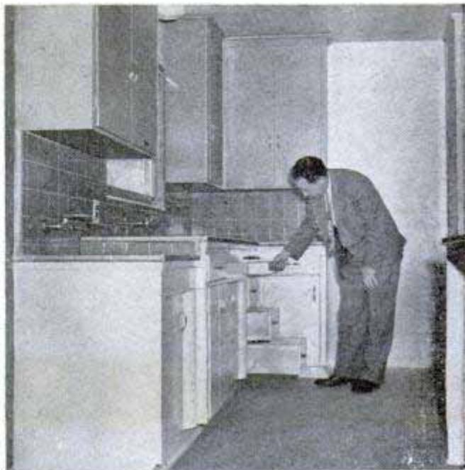
During final inspection even the drawers are tested. Then off goes the house to the home-buyer's site
