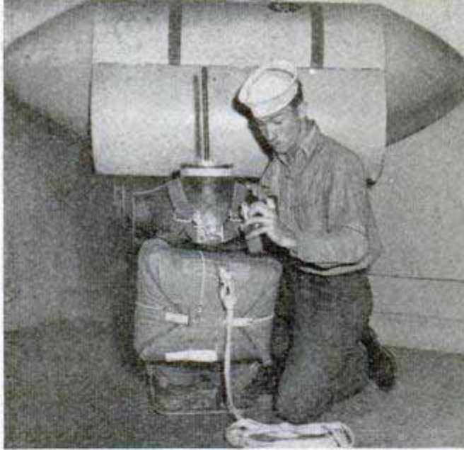
Parachute is strapped on robot jumper for a test leap. Rubber-coated antenna projects from dummy's neck
