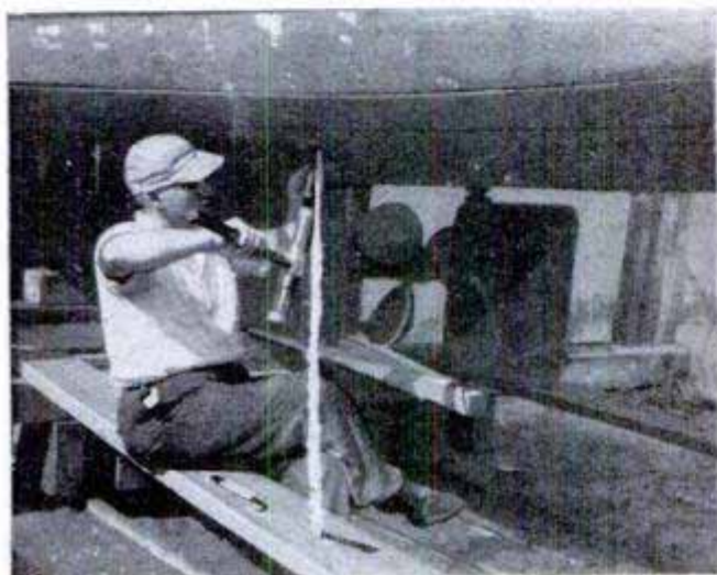
On older boats having large hulls, calking the seams is a job calling for skill and painstaking care
