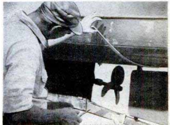
Above, repair damaged planking with any of the special fillers made for marine use. Below, use a flexible wooden strip for scribing to locate the frames
