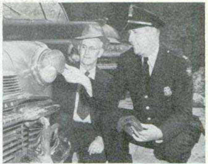
Plastic shades over headlights reduce glare from approaching car, above left, and eliminate that dangerous, "blind" instant when cars pass. The shades are hood shaped, right, and are slotted to direct light rays away from approaching car. To install shades, you remove outer rim, below left, and screw shade in place, right
