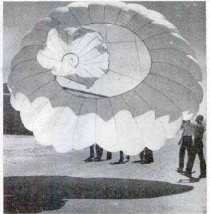
"Apex" chute has an open center with a smaller canopy above, held in proper position by shroud lines
