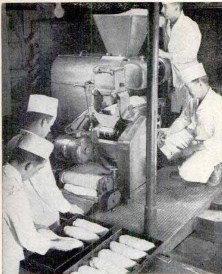
Above, the man standing in the background is feeding dough into the divider, from which two-pound pieces drop onto conveyor belt and move into molder. The two soldiers in the foreground are putting molded loaves into pans, where they will stay for 30 minutes while the dough achieves proper degree of lightness
