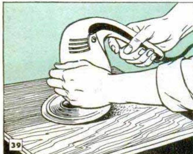
Above, compound angles can be formed on a machine like this. Below, flexible-disk sanding machine is useful for preliminary operations on wood and metal
