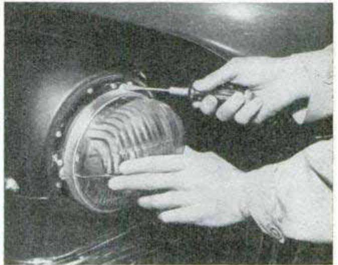
Plastic shades over headlights reduce glare from approaching car, above left, and eliminate that dangerous, "blind" instant when cars pass. The shades are hood shaped, right, and are slotted to direct light rays away from approaching car. To install shades, you remove outer rim, below left, and screw shade in place, right
