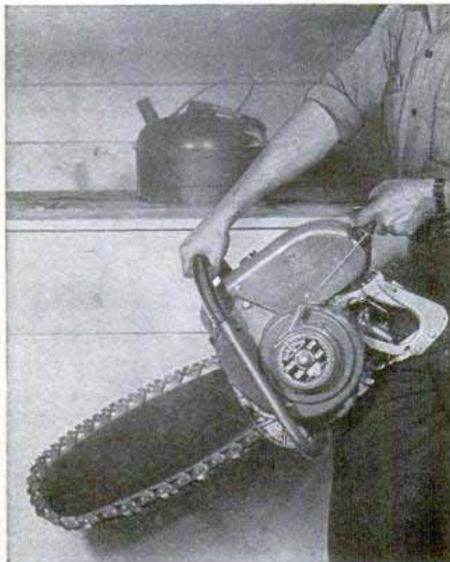
Weighing only 25 pounds, this chain saw makes tree surgery quick work. Below left, a yank on the starter cable is all that's needed to start the engine. Right, "bucking" a log into short lengths with a chain saw
