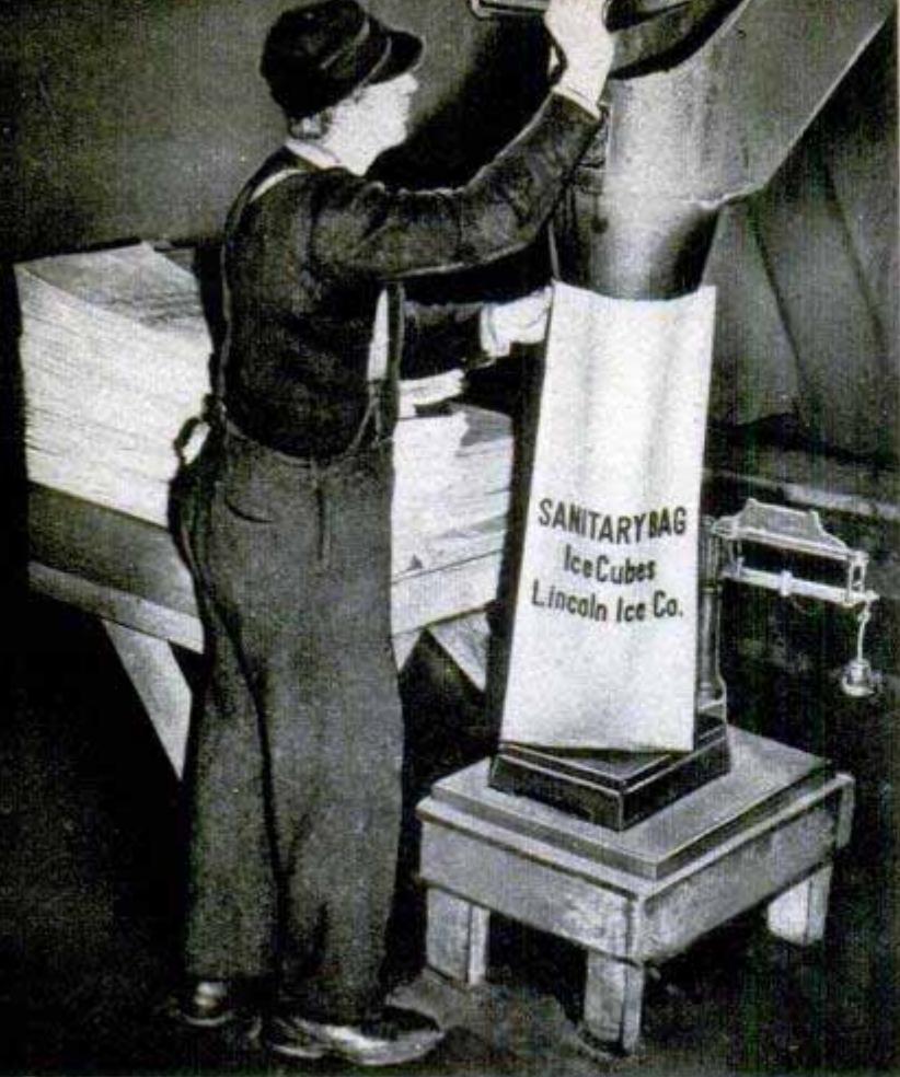
Ice cubes are packed in a paper bag treated with the plastic. Right, water is drawn across two samples of paper. It has no effect on melamine-treated paper at left, but breaks and curls fibers of ordinary paper
