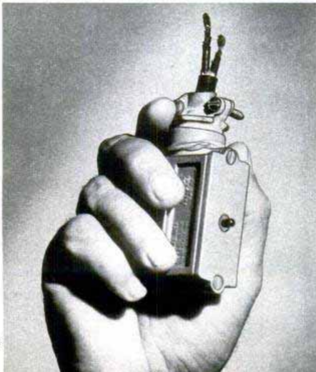
Close-up of the microswitch used to trigger the speed light. The plunger works with only slight pressure
