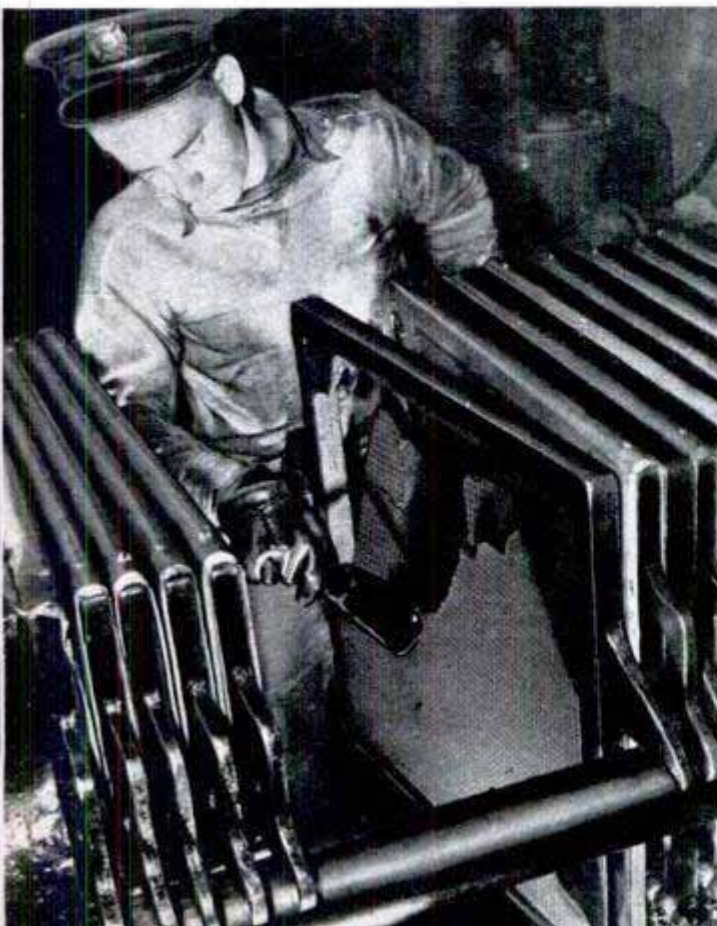
Fuller's earth, loaded with carbon, is filtered from oil by the filter press, being cleaned here
