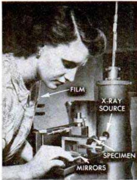
Left, research scientist adjusts the mirrors of the X-ray microscope shown in diagrammatic form at right
