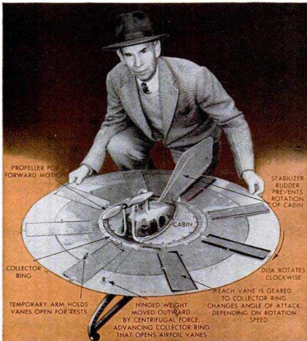
Left, Dr. E. W. Kay and 41-inch flying-disk model he designed. Its main operating features are labeled. The inventor has completed drawings for an 18-foot, one-man disk that he hopes to build
