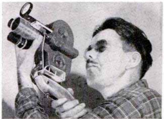
Freehand panning with a gunstock aimer, or pointer, enables the cameraman to record high-speed action
