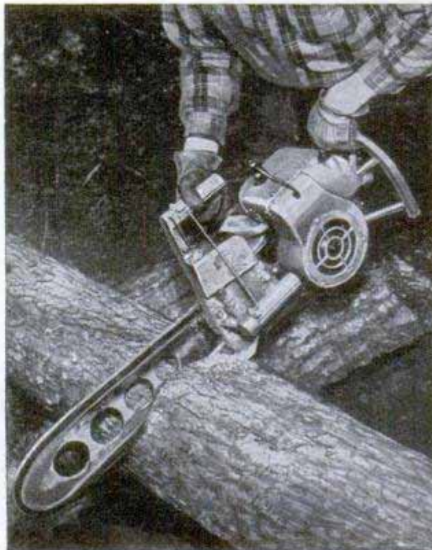
Weighing only 25 pounds, this chain saw makes tree surgery quick work. Below left, a yank on the starter cable is all that's needed to start the engine. Right, "bucking" a log into short lengths with a chain saw
