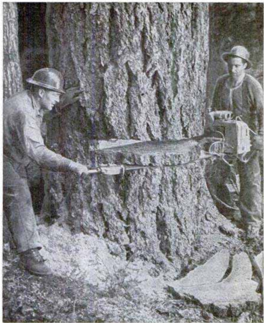
Big trees don't frighten this two-man saw. These men are making an undercut prior to felling the tree. Man at left applies pressure to the blade
