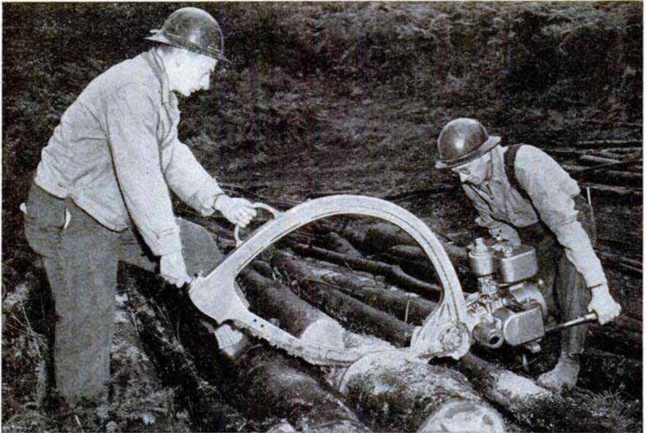
Two men handle the bow-type chain saw as it slices through logs as though they were paper. Below, one-man chain saw with various parts labeled. Bottom strip shows details of the standard and chisel-tooth chains
