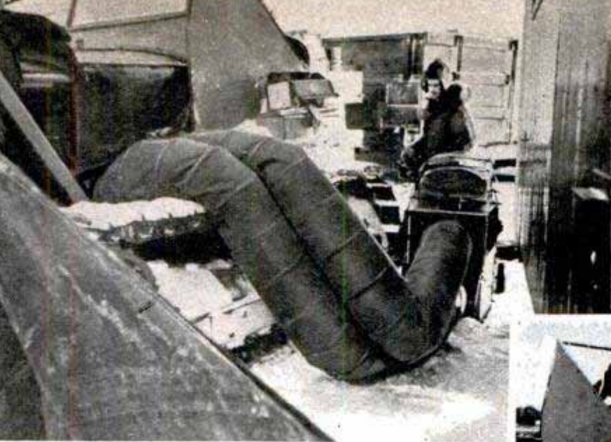
← Big gasoline heater blasts hot air over a tractor engine to warm it up for starting. After about 20 minutes of this heat treatment, the driver tries to turn over the frigid engine
