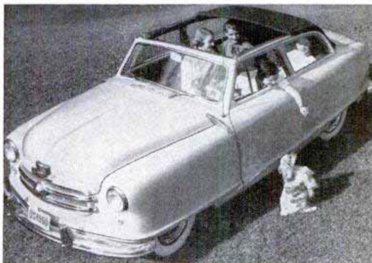
The electrically operated push-button top is advanced by steel cables and can be stopped at any intermediate position. The instrument panel below has compact easy-to-reach arrangement
