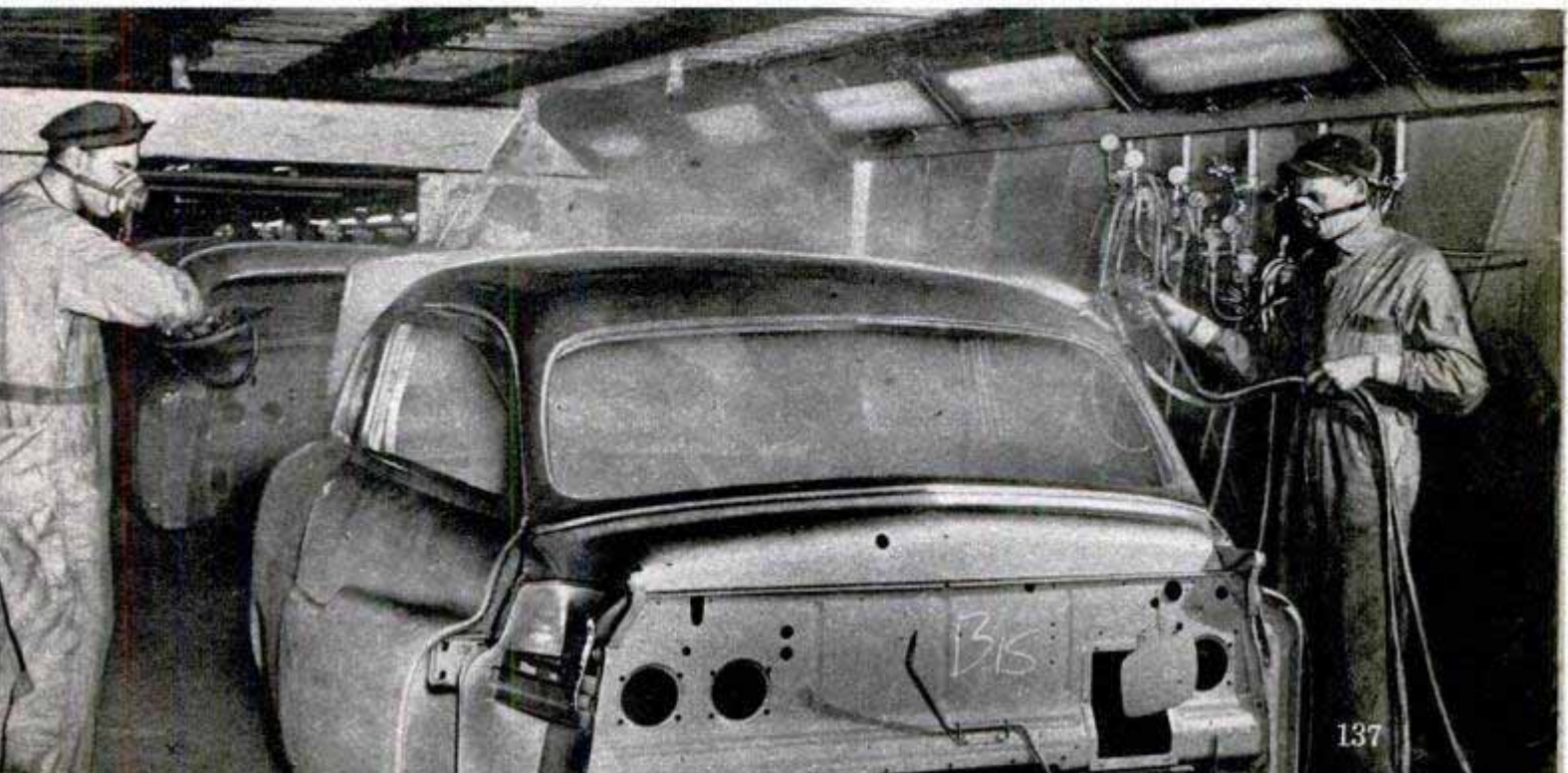
Dishes and trays made of the wonder plastic won't chip or scratch and their designs, buried in the material, won't rub off or discolor. Below, workers spray an auto body with resin-treated enamel. Melamine mix has speeded up drying by 50 percent, produces a harder finish
