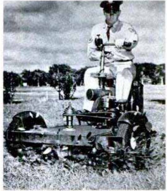
Above, left, Sergeant Chew fills gas tank preparatory to cutting lawn. Belt goes from motor to rotary spinner and sharpened spring. Right, the scooter operating as a lawn mower. Below, underside view of the machine U. S. Air Force photos
