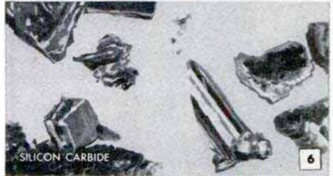
Greatly enlarged photos show the variations in the grain characteristics of the more commonly used abrasives. Although it is still available, flint is being largely replaced by the garnet and aluminum oxide
