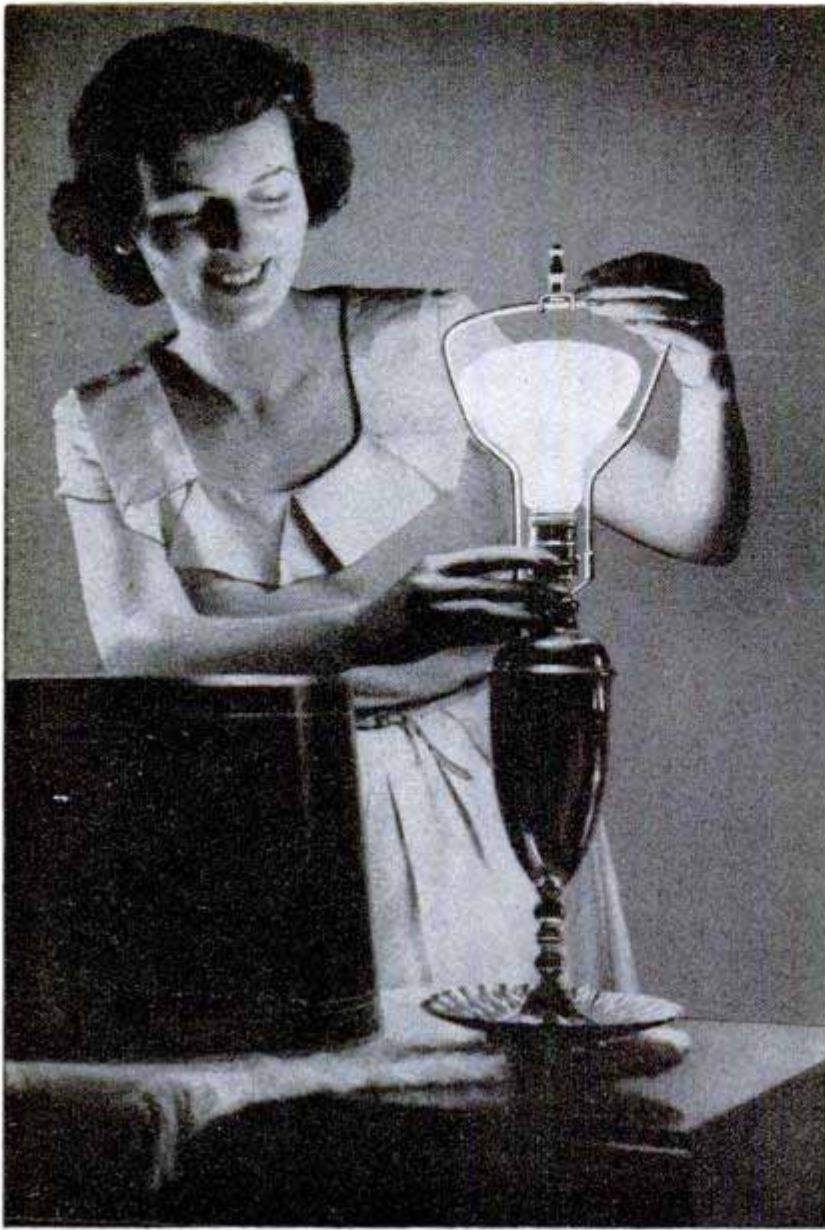
Here's the converted lamp ready for its shade. Lamp will now give twice as much downward light and considerably more upward light
