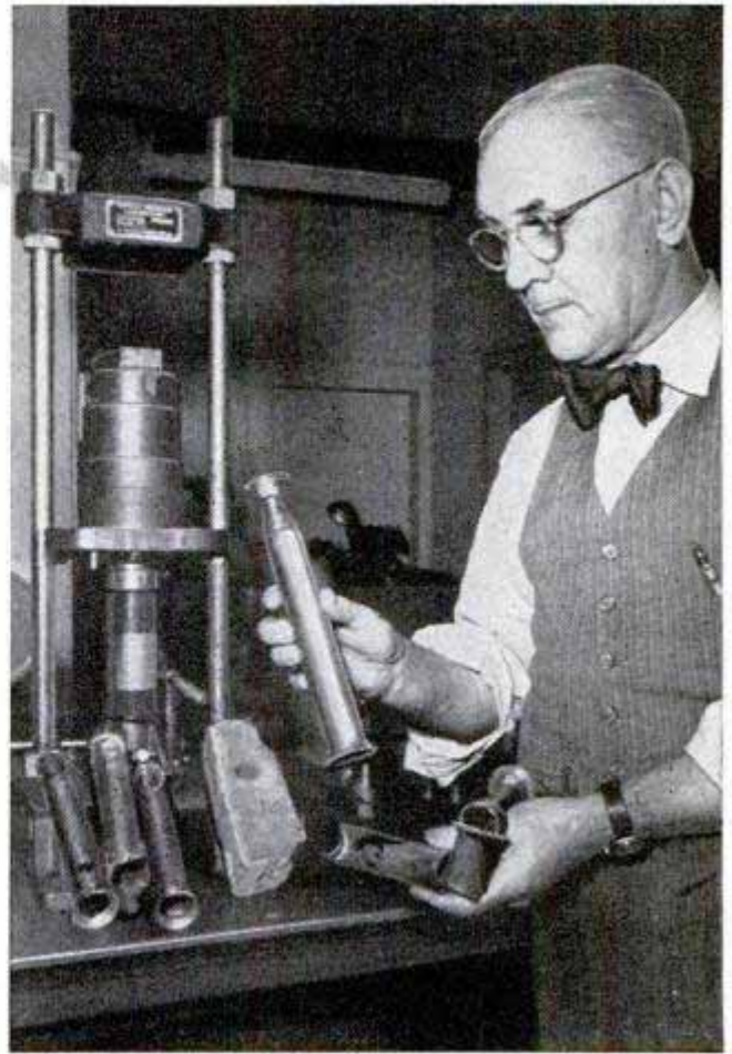
Rocket fabricator John Ashworth holds in his hands examples of steel shells before and after blowouts
