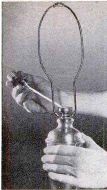
2. Remove shell from top half and pull out about 6 in. of lamp cord
