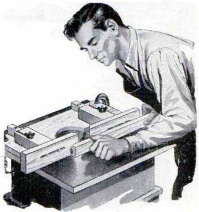
Above, shaper fence is adjustable in two directions for depth of cut and varying sizes of shaper cutters. Below, adjustable guide strips screwed to the base hold the two units of the fence in alignment. Brackets are locked in place with bolts and wing nuts.
