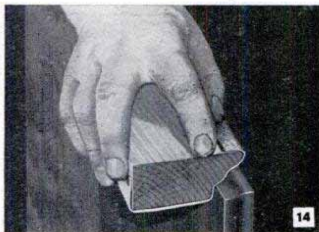
A sanding block with one edge shaped in a reverse relief of the molded edge makes it possible to remove old varnish or enamel from the mold curves
