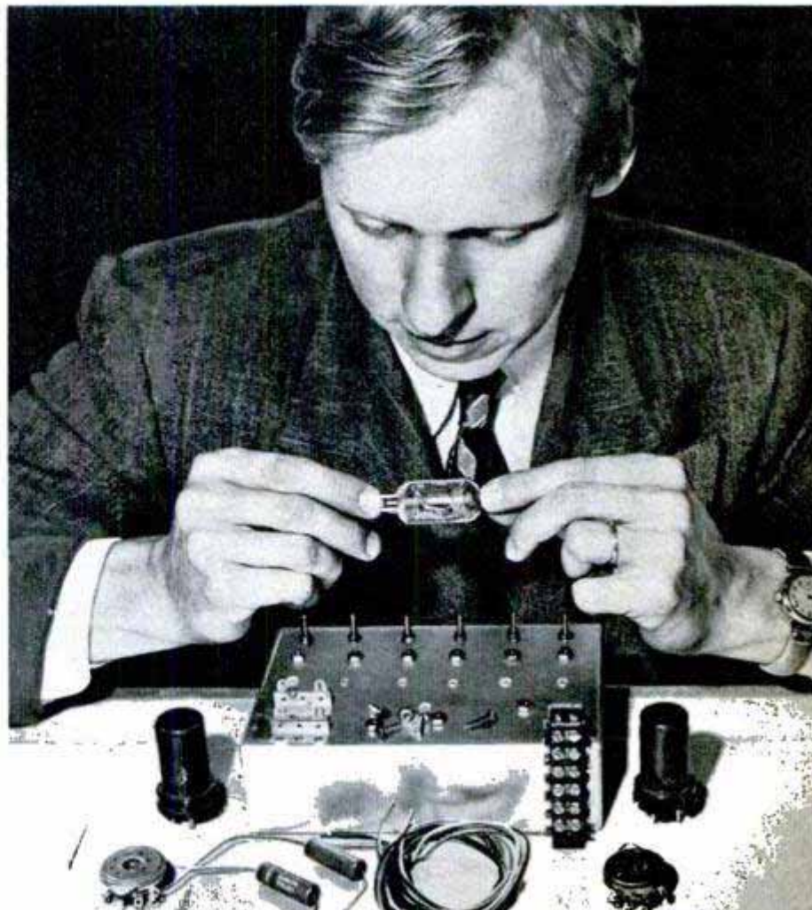
Combination transmitter and receiver, including batteries, can be held in one hand. Below, that's not a radio tube in his fingers, but a control circuit that does work of all standard components on table
