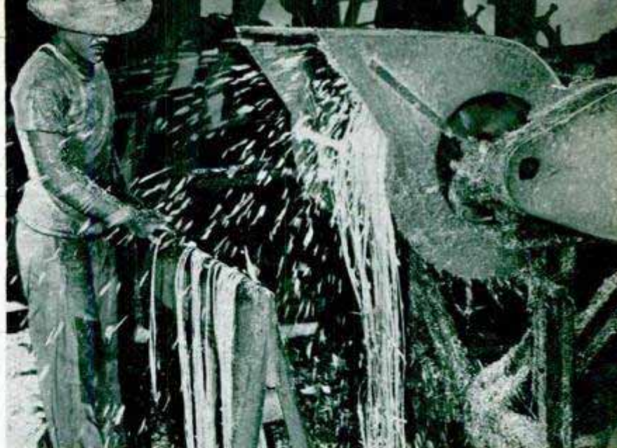
Above, the stalks are first crushed and then this beater removes woody centers, leaving fiber-bearing bark ribbons
