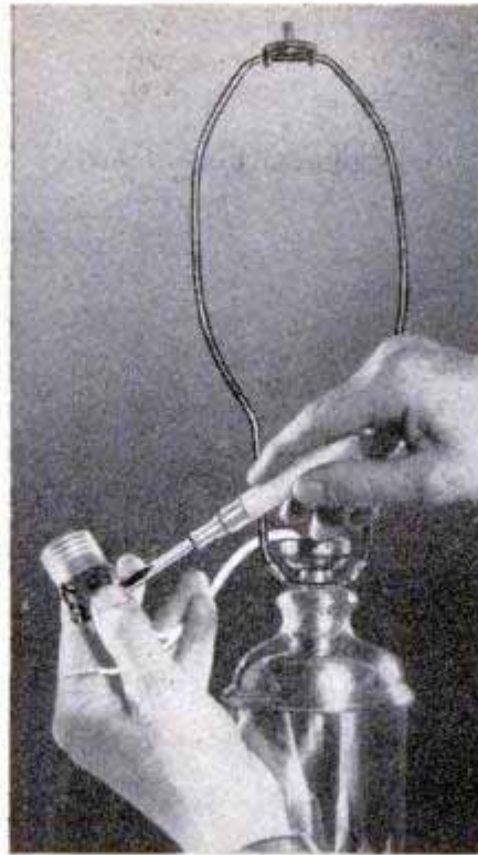
3. With screwdriver, loosen the terminal screws and detach wires
