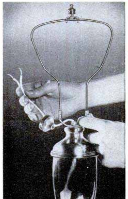
5. Replace the old harp with new wide one and rethread cord through socket
