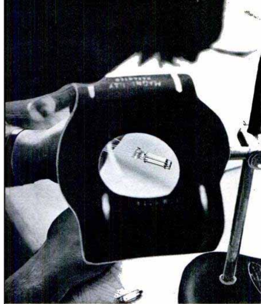
With the help of a laboratory magnifying glass a technician checks the internal structure of a subminiature radio tube. It will be fastened directly to the material upon which the circuit is printed
