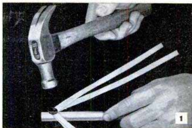
Each pair of doubled strands is laced through one another. Then pairs are spaced around a \frac{1}{2} -in. dowel and thumbtacked in place to hold them for braiding
