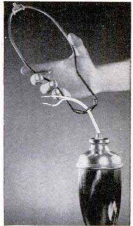
4. Unscrew bottom of socket from lamp and remove the narrow harp
