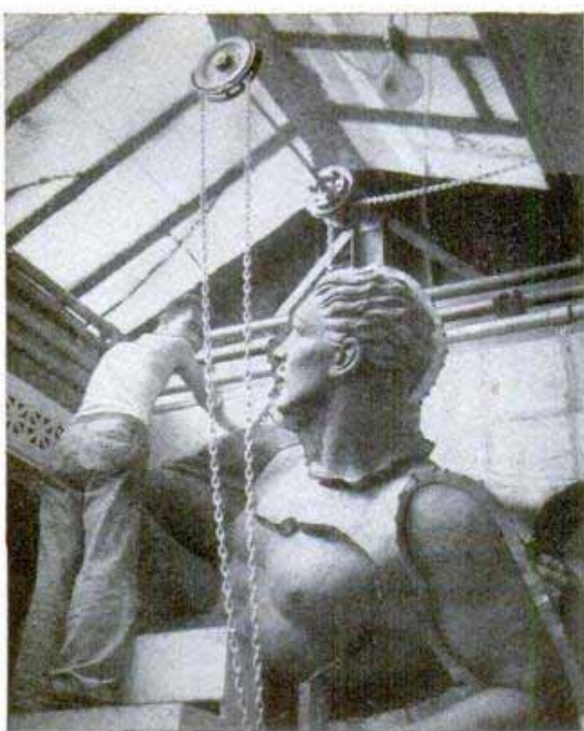
Figure is divided so sections can be lifted off. Right, original mold is chipped away from plaster mold
