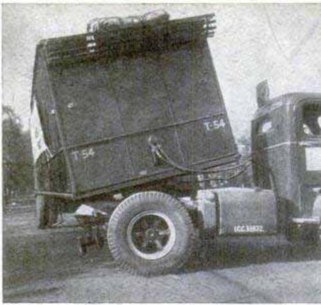
Backing a semitrailer can be hazardous. Because the fifth wheel doesn't turn, this sharp tilt results
