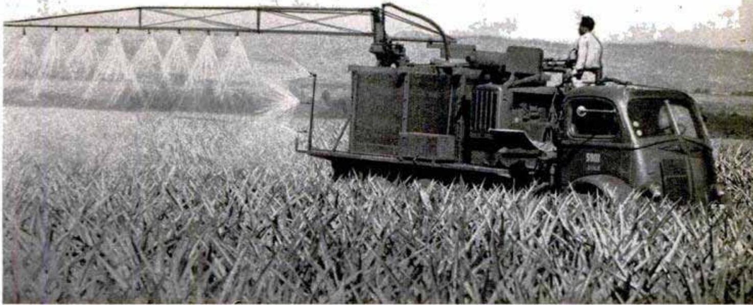
Pineapple plants must have their iron so this spray machine dispenses barrels of iron sulphate over them
