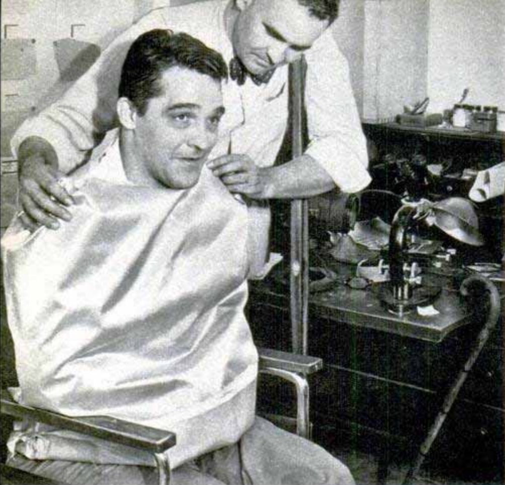
Staff members test a sleeveless jacket made of metallized cloth which stores up the heat radiated from the body. Below, wheel chair at left is operated by one finger, that at right by tongue in the mouthpiece
