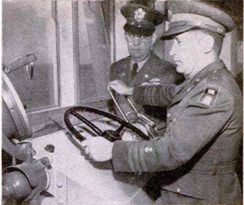
↑ Simple controls on the bridge permit pilot to spin the ship like a waterbug. Three diagrams below show how angle of blades changes direction of craft. Arrows in groups show thrust of the blades to maneuver ship in direction indicated by single arrows
