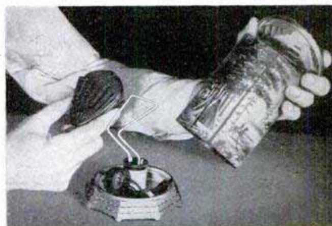
Above, a novelty lamp is just the thing for concealing the mike. Hide the lamp cord in the base as shown
