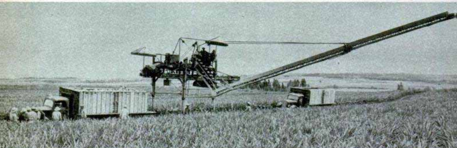
Left, a close-up of the Ginaca machine for processing pineapples. Pineapple moves side-wise down chute and is spaced as it enters machine. Cored pineapple shoots through tube on far left. The girls in the picture keep pulp moving into separate chute. Below, harvester moving through field. When truck on left was full, harvester raised up to permit it to pass through. A second truck (empty) waits its turn at the harvester
