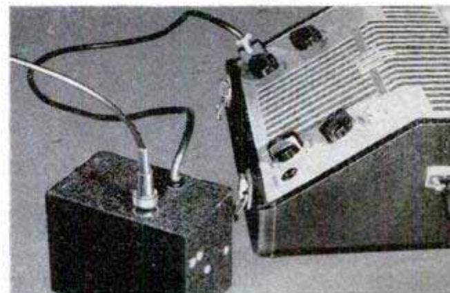
Below, sometimes a preamplifier can be used to good advantage to increase the range of the microphone
