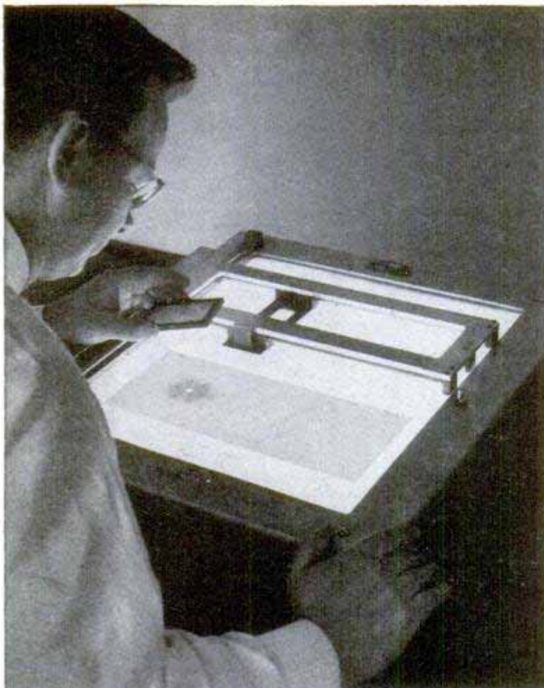
Above, a G.E. scientist studies photographic film spotted by X-rays deflected from their path by the internal structure of a decaborane crystal. The film was in cylinder form during test. Below, Dr. John Kasper holds model of a decaborane crystal
