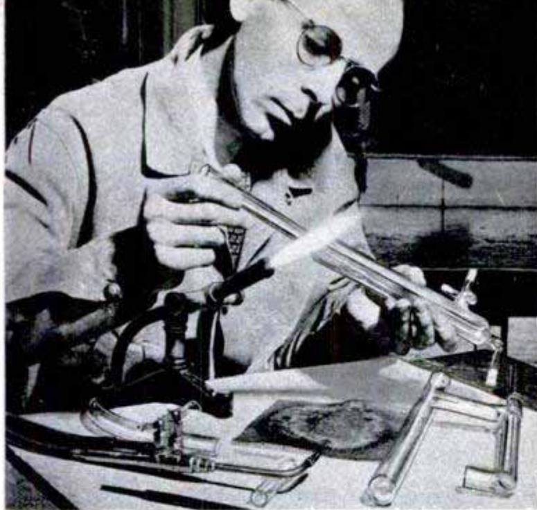
Didymium lenses used by glass blower block out 90 percent of brilliant glare from yellow sodium flame. Top photo at right shows how bright flame obscures details of the work while just below it work is shown through lens. Below, separator sorts the rare earths in accordance with their magnetic strengths
