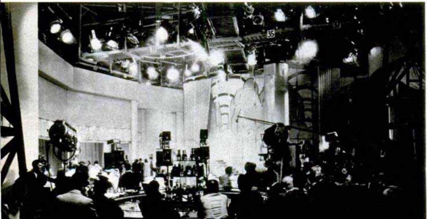
Carbon arc lights made of rare-earth oxides give this motion-picture set a natural "daylight" illumination
