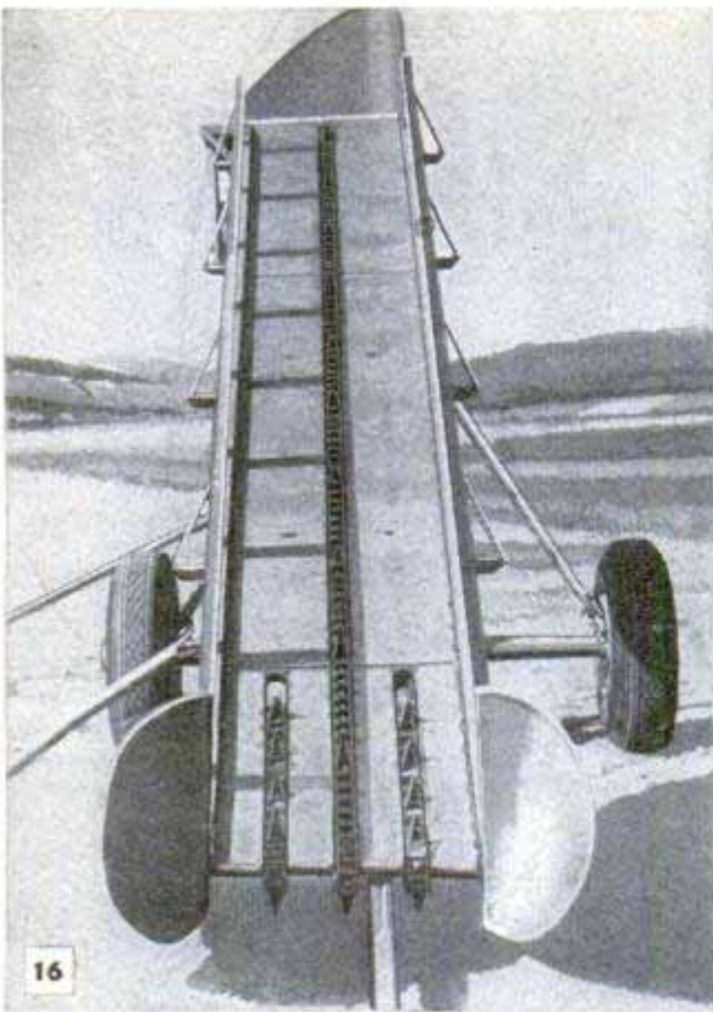
16 Short pickup chains start bale on its way up the elevator bed, or "flight," to the loading platform
