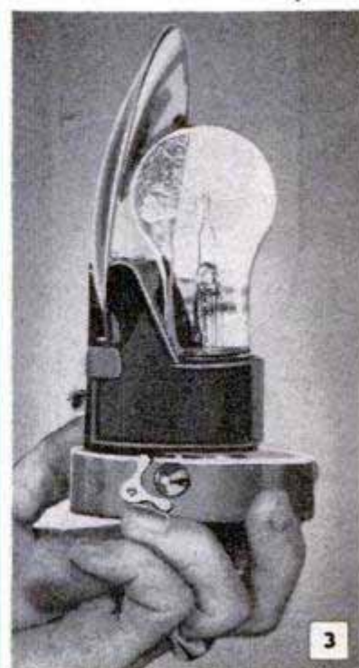
Above, contact prongs on the flash unit fit into sockets formed in the switch. Below, right, note the safety catch which is provided to lock the push button and prevent accidental premature firing of the bulb. A flick of the finger releases the catch
