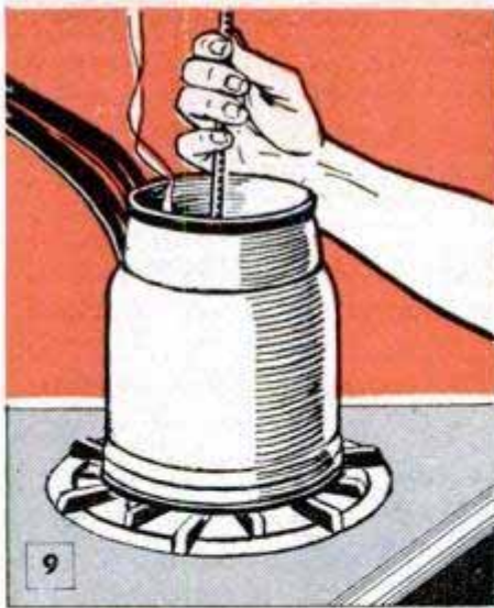
Ingredients for the flexible mold are cooked in a double boiler and then alcohol is added to the mixture
