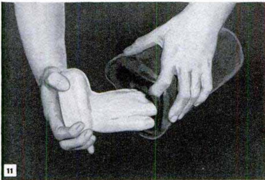
Master and subsequent castings are extracted from mold by stretching it. Open-end can provides mold form
