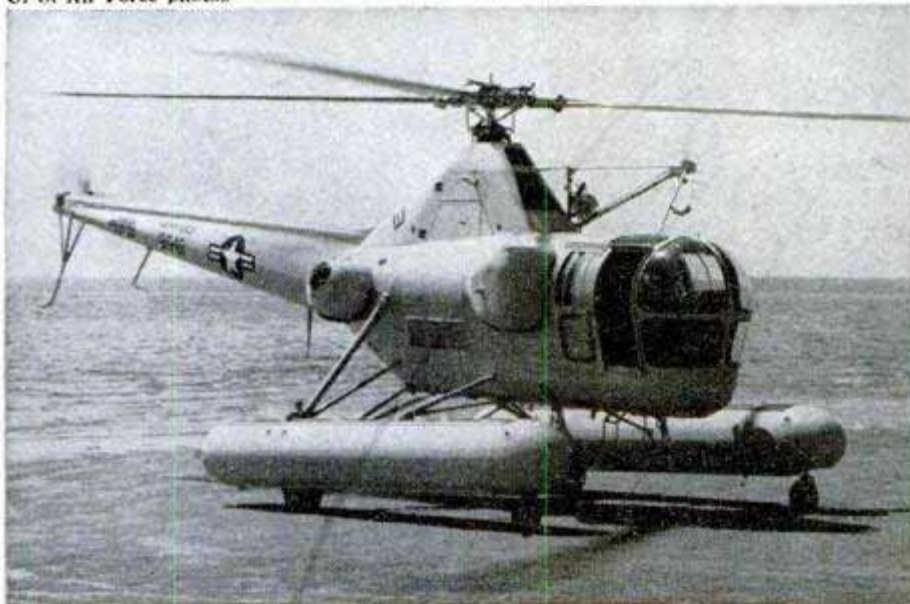
Above, left, head end of litter extending out from rear "blister" hatch of rescue helicopter. Above, right, airman closing hatch preparatory to take-off. Below, pontoons and wheels fit craft for either land or water rescues
