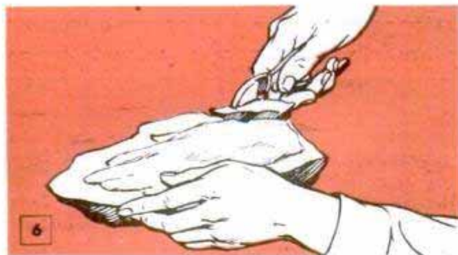
Mold is carefully chipped from master with pliers
