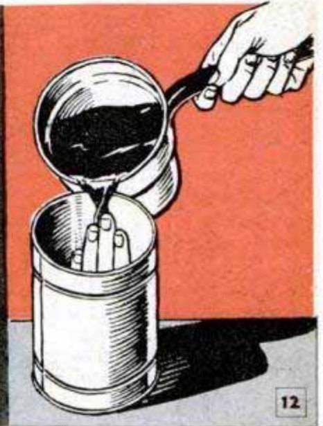
Master and subsequent castings are extracted from mold by stretching it. Open-end can provides mold form
