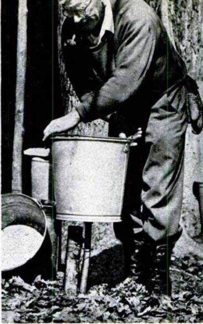
Large bucket screws to pipe to serve as a funnel. Perforated pail, left, slips inside to strain sap
