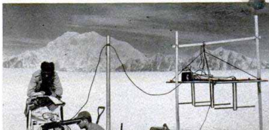
Glaciologist drives a peg into snow across crevasse and lowers a rope ladder. He'll study the annual "growth rings" beneath glacier's surface. Scientists tried radar in measuring depth of the glaciers. Experiments were inconclusive, but radar may become valuable research tool
