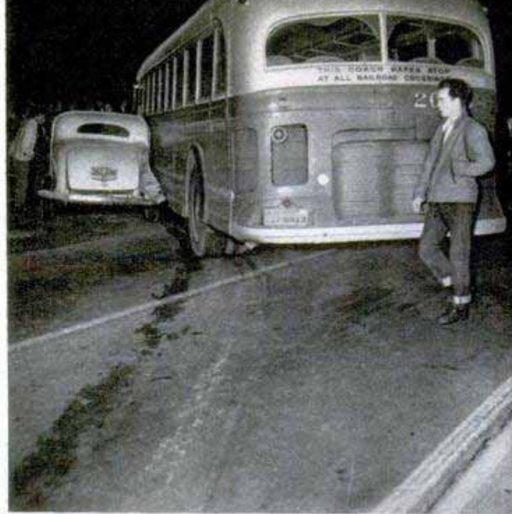
Skid marks on the pavement may indicate the paths traveled by vehicles. Center line serves as landmark
