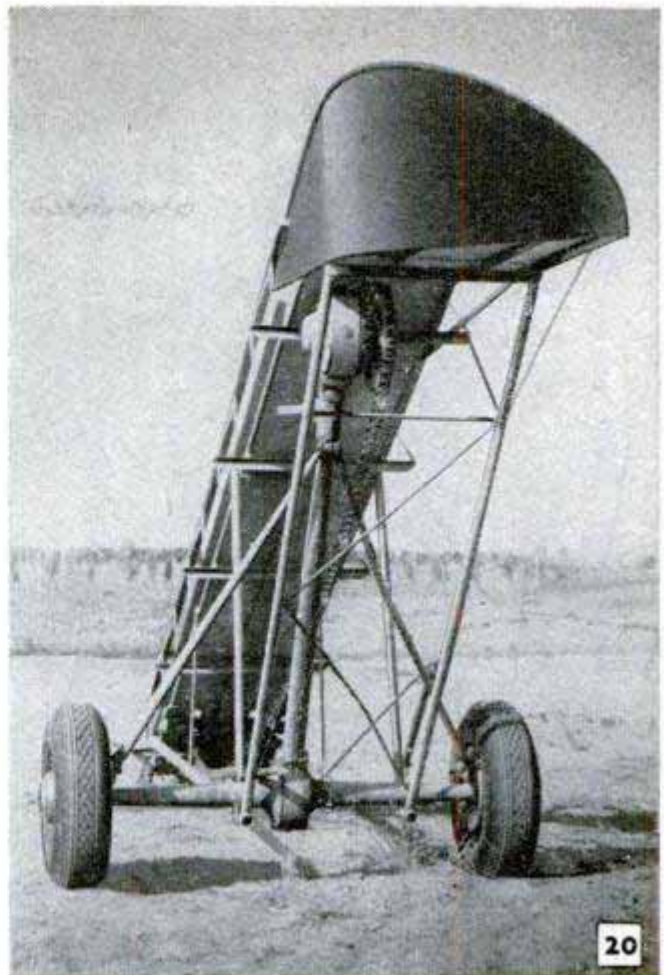
Above, rear view showing curved platform fender which turns the bale at top of elevator. Below, differential and clutch are mounted on torque tube
