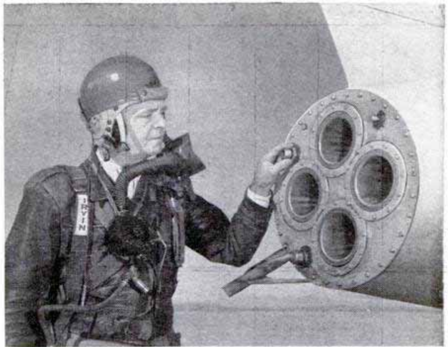
Tube extending down at an angle from below the four rocket nozzles is used for jettisoning the remaining rocket-engine liquids before landing
