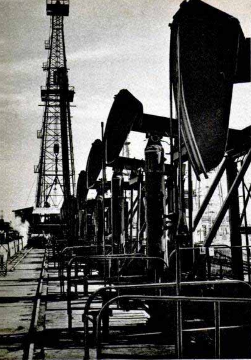
Row of pumps is removing oil from pool hundreds of feet away. Derrick on rails is drilling another well
