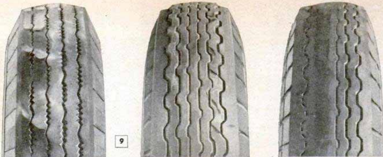
Faulty wheel alignment, worn wheel bearings or a broken spring can result in uneven tread wear
