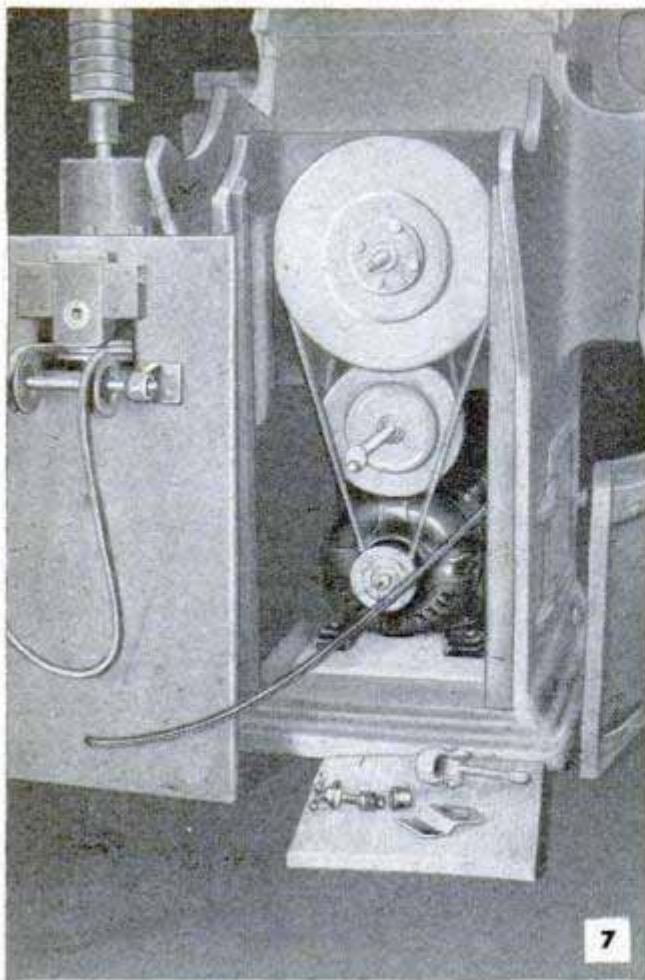
Idler pulleys mounted on detachable rear wall form right-angle drive for the oscillating spindle sander
