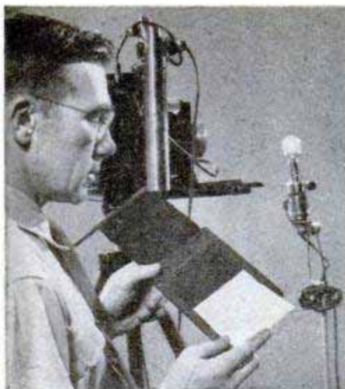
Image appearing on sensitive sheet tells you if the synchronizer is in adjustment. A—Shutter opens too soon; B—Perfect synchronization; C—Shutter is late
