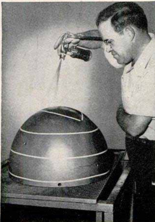
Below, conductive paint is sprayed on this plastic accessory cover for airplanes. It stops ice formation and keeps working parts at proper temperature
