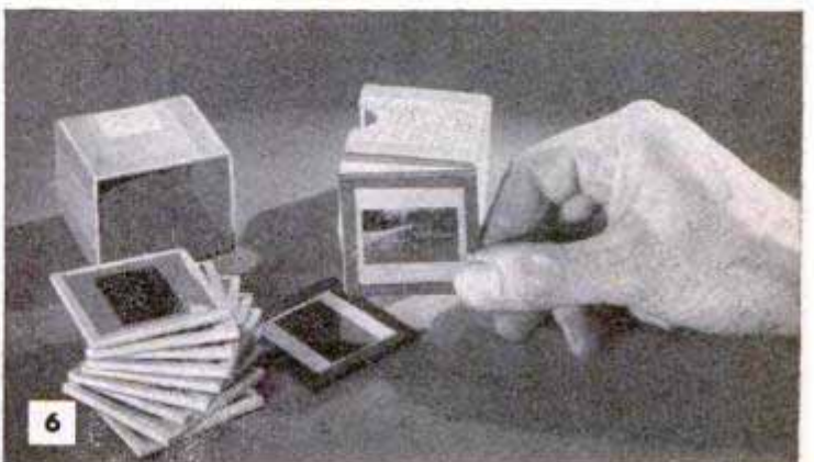
Above, binding the glasses together with gummed paper tape made for the purpose. Below, finished transparencies ready for projection. Dot in lower left-hand corner serves as a guide when inserting slide upside down in the projector
