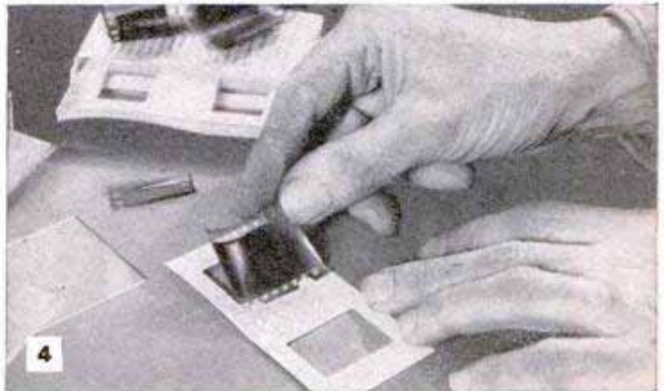
Placing the positive transparency in a ready-cut mask preparatory to mounting it between two 2 x 2-in. cover glasses
