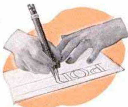
Distance between pencil points can be varied to suit the size of letters
