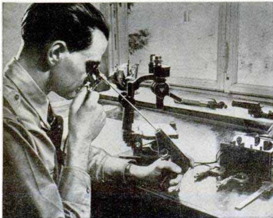
CID agent fires suspected weapon into a tube filled with waste, which prevents any marks on bullet except those made by rifling. Below, new light tube gives a clear view of the inner surface of a pistol barrel
