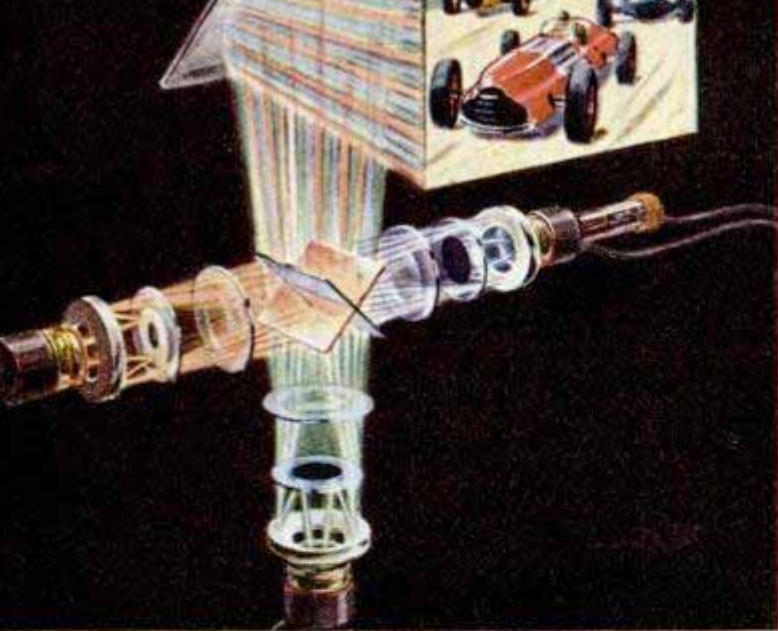
Above, drawing of RCA projection system, with its three kinescopes. The two dichroic mirrors, center, superimpose the three colors to form a single image
