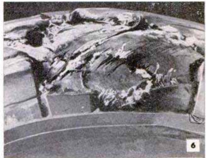
A bad blowout often tears away a portion of tread, exposing cords and making a major repair necessary
