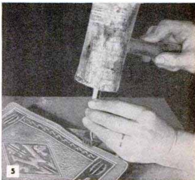
Above, a stipple effect is produced by tapping the leather with a roundnose tool, held vertically. Below, holes for a leather lacing are punched around the edge of the work with a special lacing awl made for the purpose. This is done on a hardwood block
