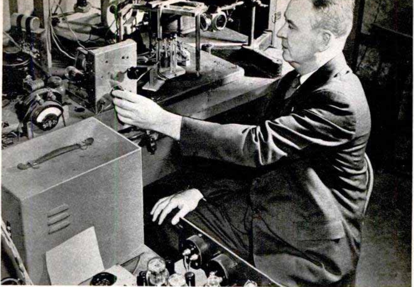
Dr. Jesse W. Beams and his ultracentrifuge which whirls at 166,000 revolutions per second in a vacuum
