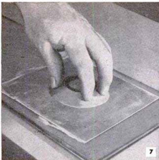
Rim of distributor cup is smoothed on emery cloth to assure watertight joint when soldered to brass plate
