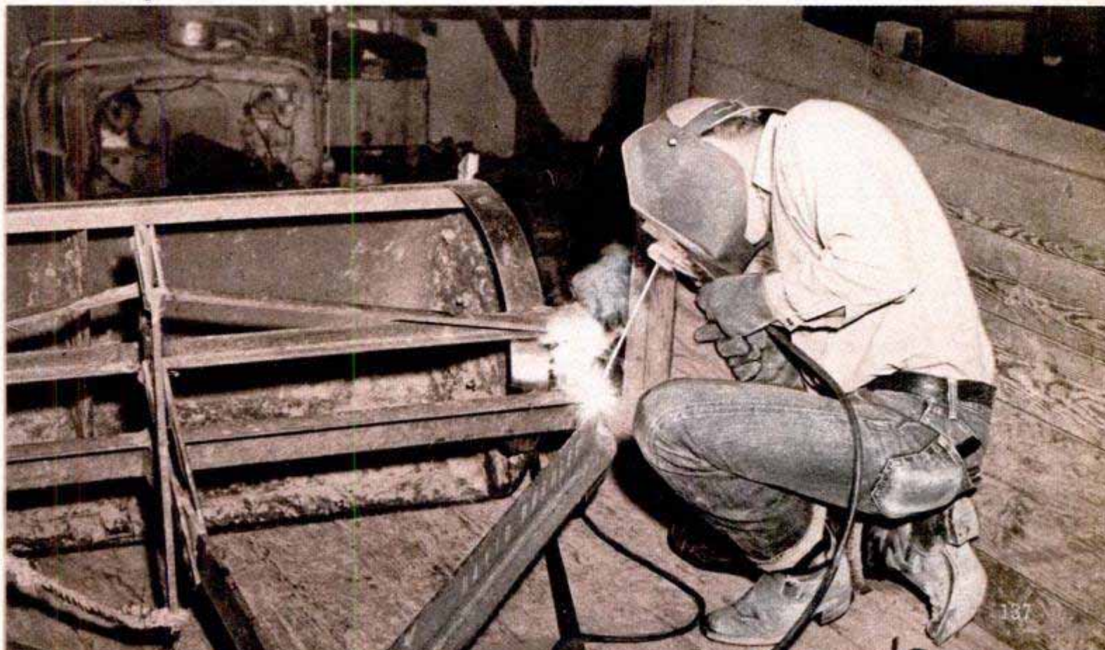
Below, a GI homesteader uses the equipment available at the Vocational agricultural School of the Minidoka Project to weld a brace on a scraper
