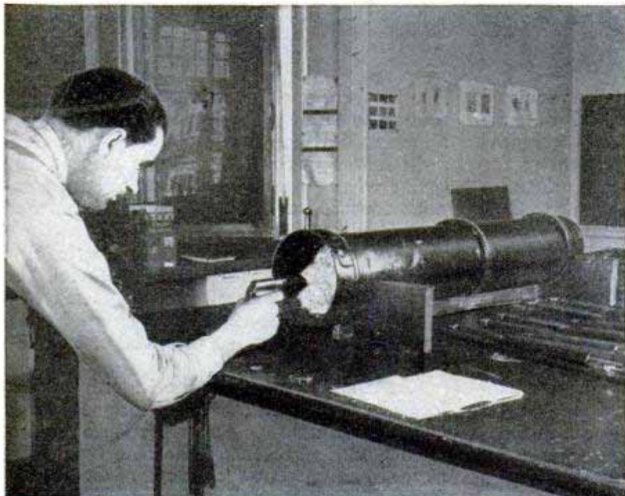
CID agent fires suspected weapon into a tube filled with waste, which prevents any marks on bullet except those made by rifling. Below, new light tube gives a clear view of the inner surface of a pistol barrel
