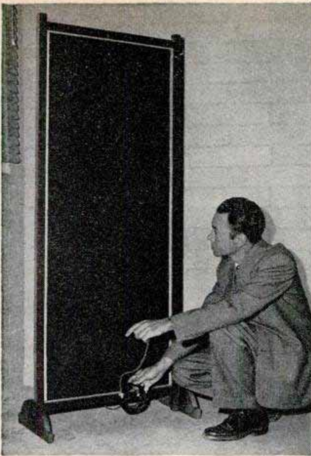
Covered with conductive paint, this panel, used in room-heating tests, keeps a surface temperature of 110 degrees. The paint can also be applied to walls
