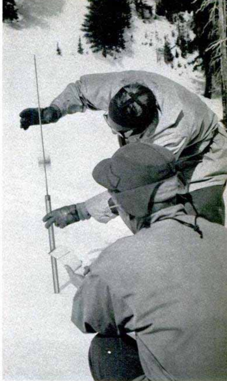
Swiss avalanche expert shows ranger how to test the snow's resistance to penetration by a ram instrument. This is an important factor in avalanche prediction
