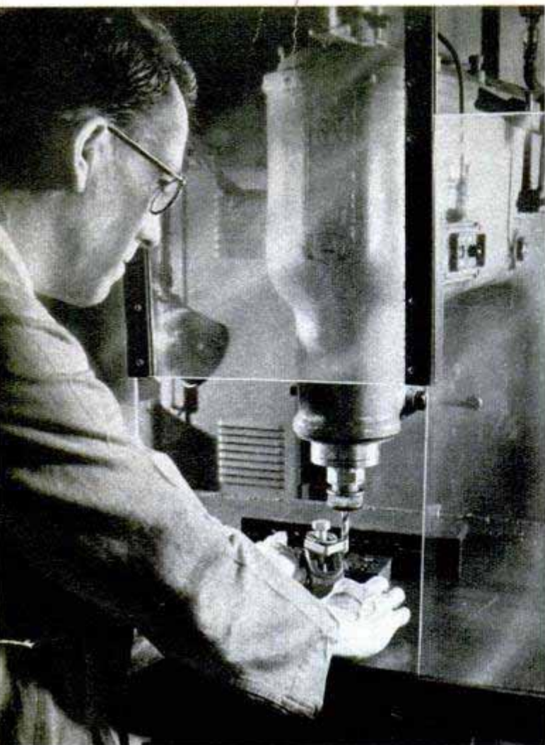
Bullet-speed drilling works 10 times faster than ordinary methods. All that's necessary is to notch the drill
