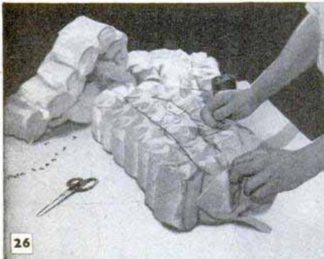
Below, the marshall unit is placed on top of the spring unit to which it is sewed around the four sides. Below, right, moss or tow filling is placed over marshall unit and then two layers of cotton
