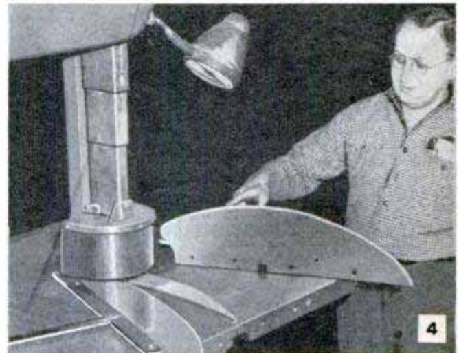
Above, special jig for cutting circle segments of varying radii. Below, detail of segment-cutting jig
