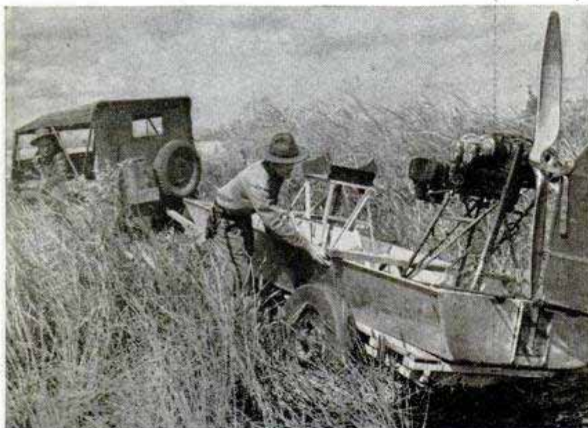
Jeep tows the Patrol's airboat (note propeller) into the Everglades as far as possible. The boat skims over the "river of grass" area (below) at 40 m.p.h. and it can jump over small logs and low brush
