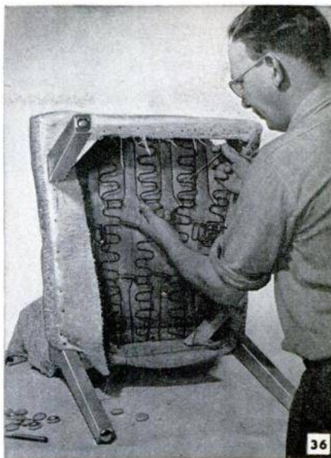
Upholstery of the hostess chair differs from the others in that springs are fastened directly to the chair frame, instead of a separate frame. Also, seat edge springs are placed across both front and back as indicated below. Fabric is brought down over rails and tacked to underside
