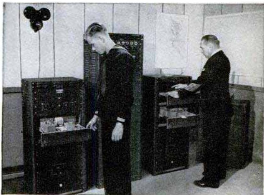
Above, diagram of firing-pin end of SOFAR bottle-cap bomb. Left, a photograph of the bomb alongside a foot ruler. Below, automatic receiver that sounds an alarm and records the signal on tape and wire
