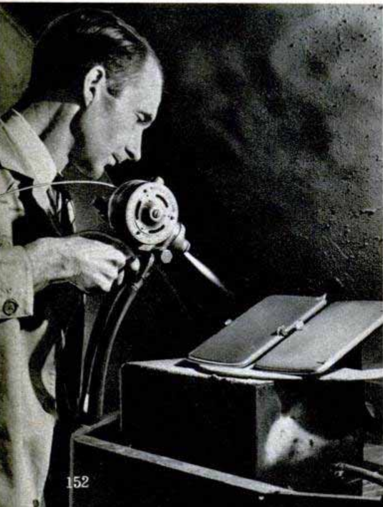
Four mechanical wizards puzzle over the problem of how to manufacture a new part for an air cleaner. Below, atomizer tool "liquefies" metal, then sprays it on worn parts to make them as good as new
