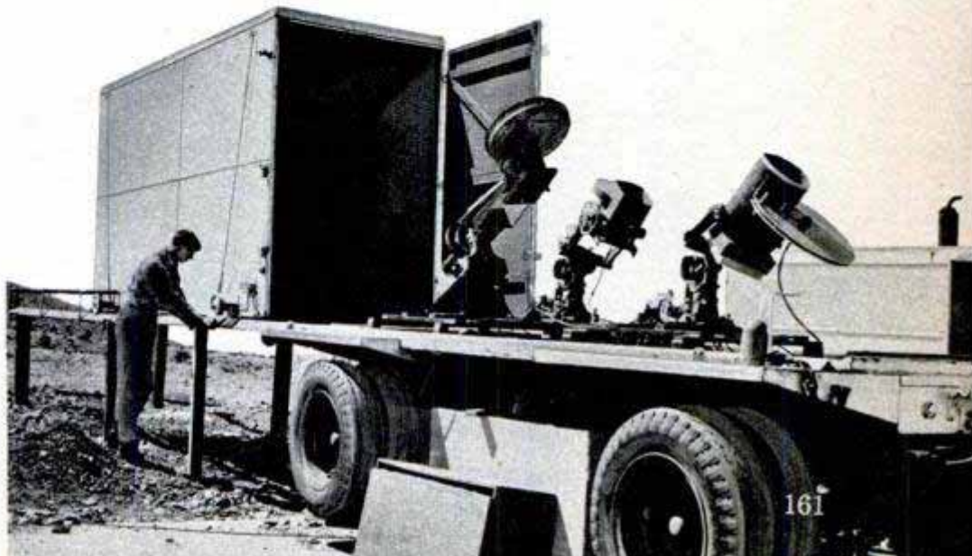
Radio-coordinated cameras also record the meteors. At dusk, roof and sides of trailer are slid back along track to open the skies to the cameras. Eighteen miles away other cameras will take matching pictures
