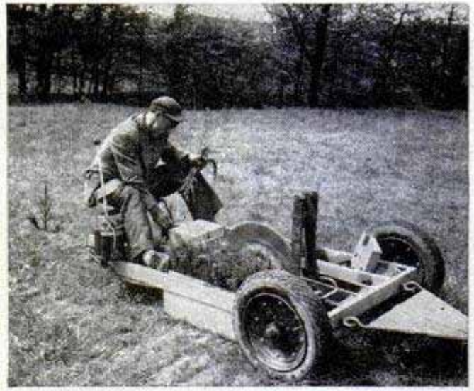
Left, the two rear wheels of the planter pack the soil around the roots of the seedlings. Above, all the operator has to do is drop seedlings into the trench. Below, close-up shows how the trench is cut
