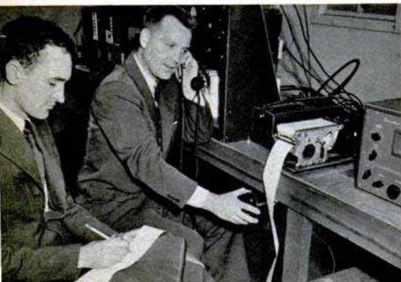
"Radio camera" is located in mountain bowl to eliminate direct signals from distant transmitter. Two antennas pick up "sounds of the stars." Below, mechanical pen records information on meteors picked up by the radio
