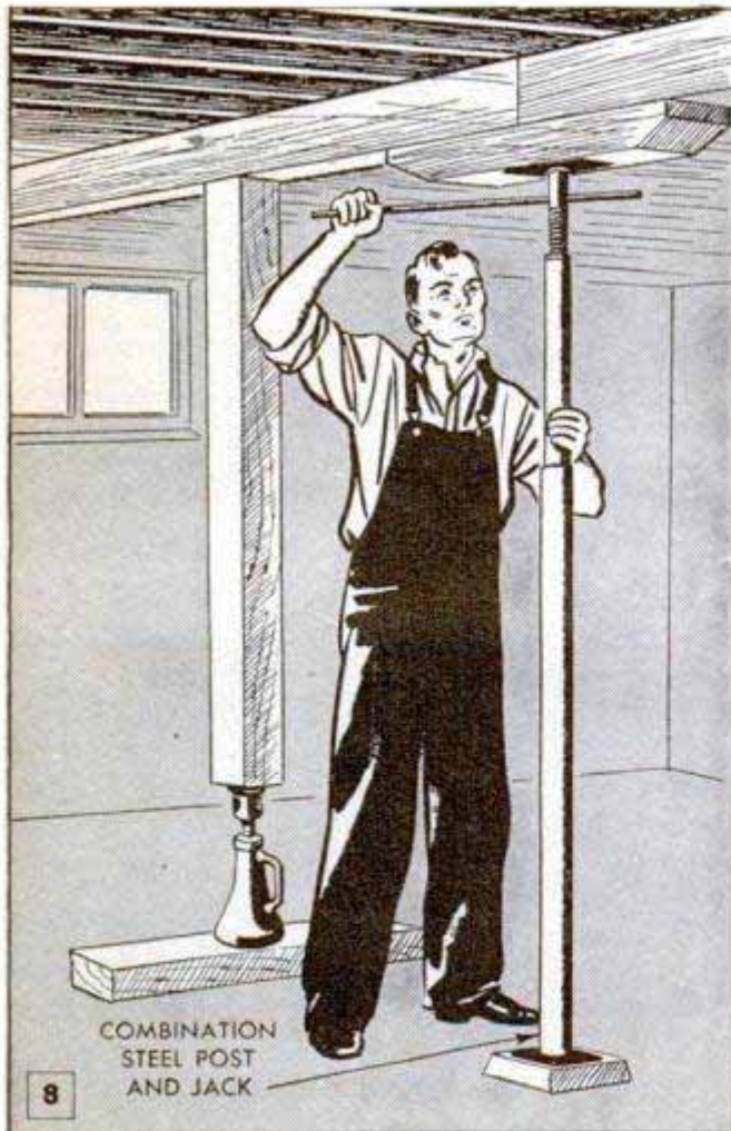
Above, to correct sagging of first floor, one or more temporary supports are placed under girder with the lower ends bearing on jackscrews. Below, the old post is then removed and replaced with a new-type steel post having a built-in jack for raising the girder
