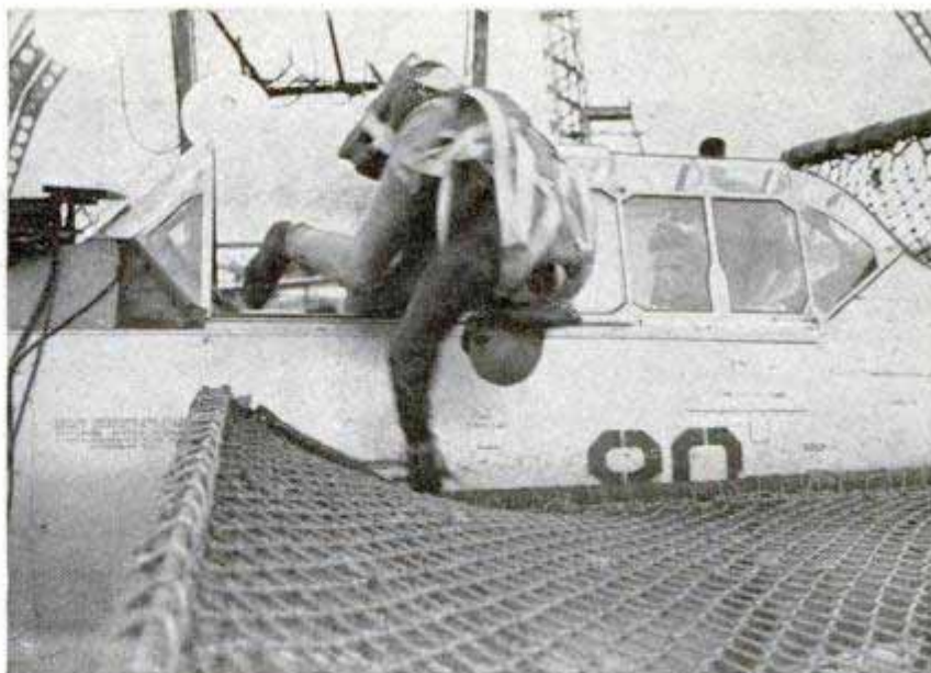
Student tumbles from an older-type plane in a practice dive. With head down, slip stream will carry him over the wing and under tail assembly
