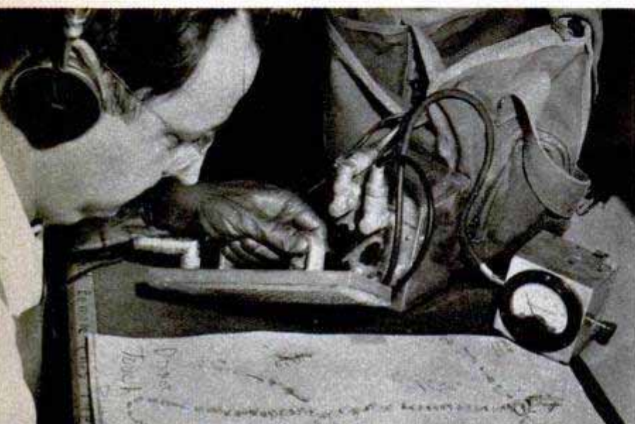
Radioactivity is tested by placing material in lead safe with Geiger tube. Below, animal skeleton is checked for radioactivity
