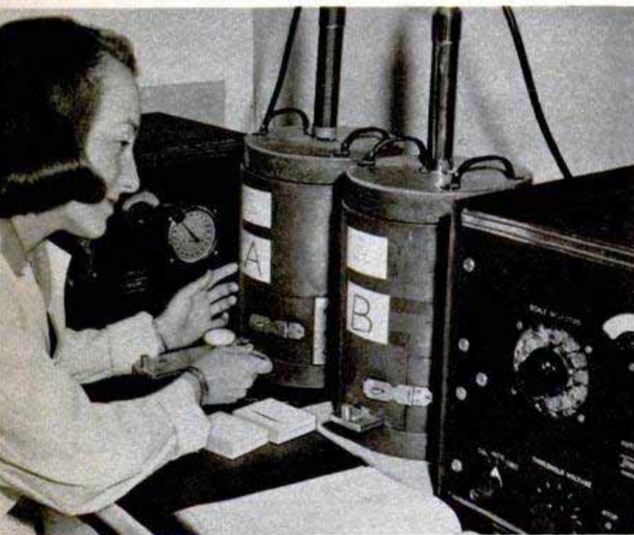
Radioactivity is tested by placing material in lead safe with Geiger tube. Below, animal skeleton is checked for radioactivity
