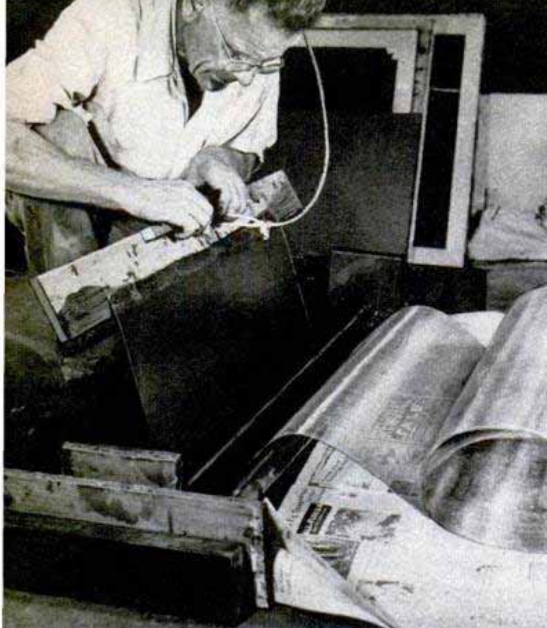
Copper screening is fed through a trough under a roller. Graphite-and-oil mixture fills the trough. Construction details of the trough are shown below
