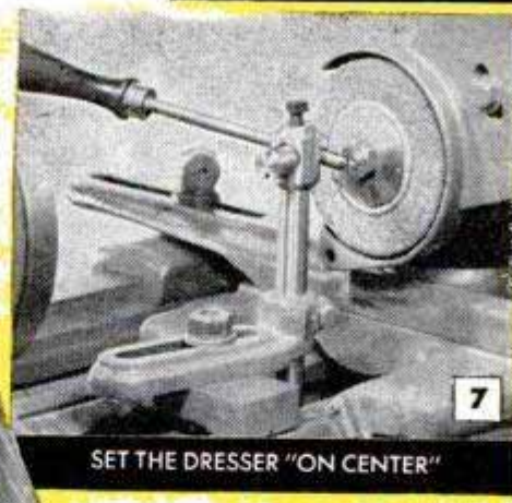
4-IN.-DIA. 46-GRIT WHEEL DOES A GOOD JOB OF EXTERNAL GRINDING WITH INFEEED OF .001" AND .005" TRAVERSE
