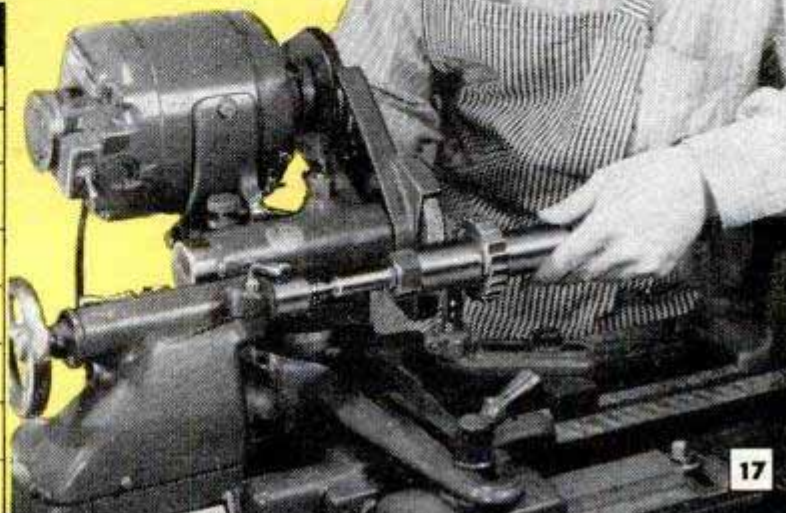
GRINDING OF MILLING CUTTERS, REAMERS, ETC., IS EASY TO DO ON A LATHE FITTED WITH TOOL-POST GRINDER
