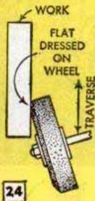
19 SURFACE GRINDING CAN BE DONE WITH CUP WHEEL, ABOVE, OR STRAIGHT WHEEL DRESSED TO CLEAR SPINDLE, BELOW
