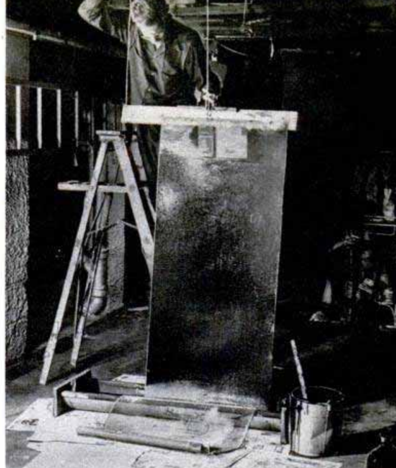
Screening is pulled through by a hoist, which prevents it from touching the edge of the trough, breaking surface tension. Detail below shows the hoist
