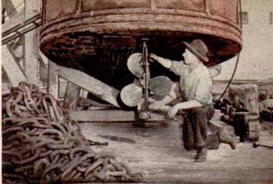
Above, left, hook on bow plate prevents the Dozer from riding over a log. Above, oversize propeller takes constant beating
