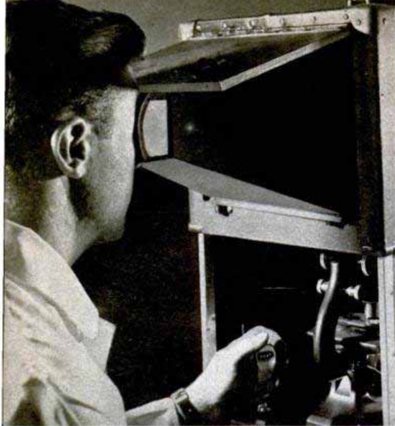
Left, a hygienist counts dust particles with the help of a microprojector. Magnified 100 times, the image is projected on an 8 by 10-inch screen for accurate counting. Right, the dust particles as seen on the screen
