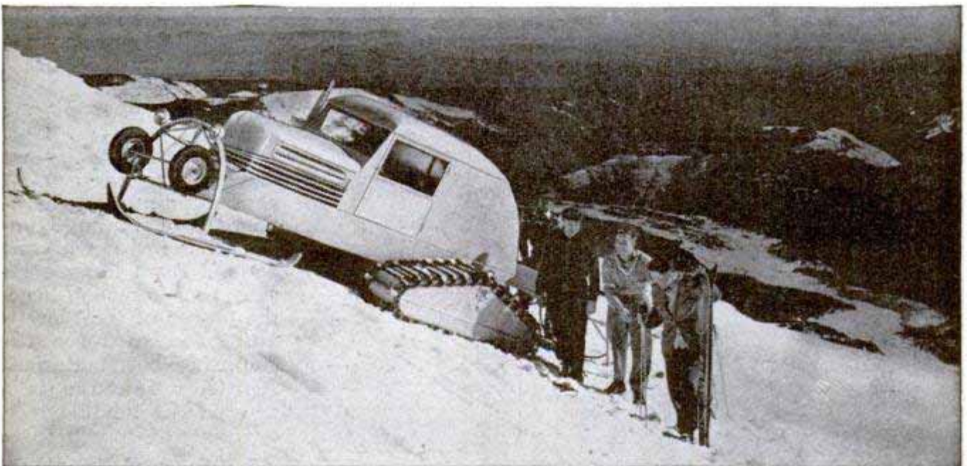
Trailer, mounted on sled runners, holds 20 skiers and their equipment. Below, the ski-steered tractor climbs hills and crosses side slopes which have a grade of up to 30 percent. Another model has four driving pontoons
