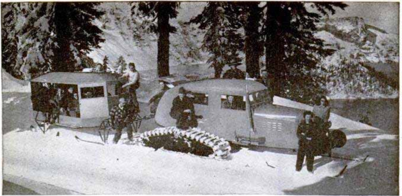
Trailer, mounted on sled runners, holds 20 skiers and their equipment. Below, the ski-steered tractor climbs hills and crosses side slopes which have a grade of up to 30 percent. Another model has four driving pontoons
