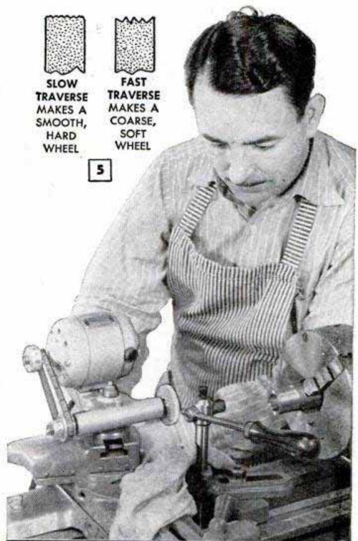
DRESSING IS ESSENTIAL FOR GOOD GRINDING. RATE OF TRAVERSE CONTROLS WHEEL HARDNESS
