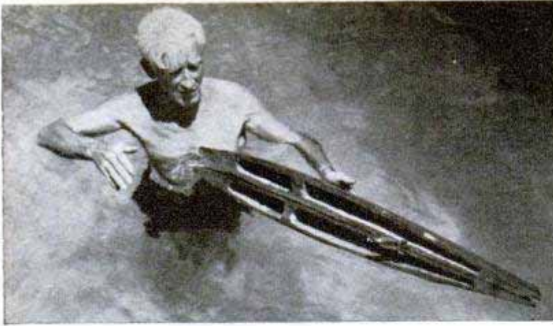
In these three photos, Gar Wood shows the basic principle of his Venturi-type construction which is designed to prevent rolling and pitching. With model above he shows how easily ordinary hull tips
