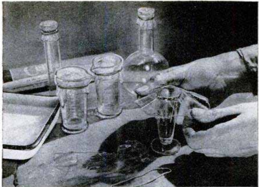
Nonmoistureproof Cellophane is used to make dustproof covers for laboratory glasses. It is first soaked in water, then held with rubber bands
