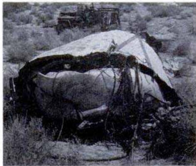
Body of the rocket falls to earth at about 100 m.p.h. Though crushed, it protects the instruments inside
