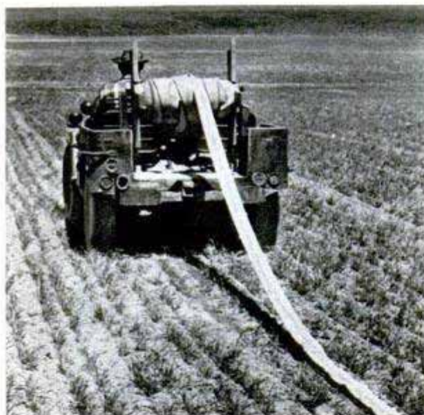
To move his irrigation system, he drives across the next field and unreels the garden hose. Below, the water area is changed by tugging on the feeder lines
