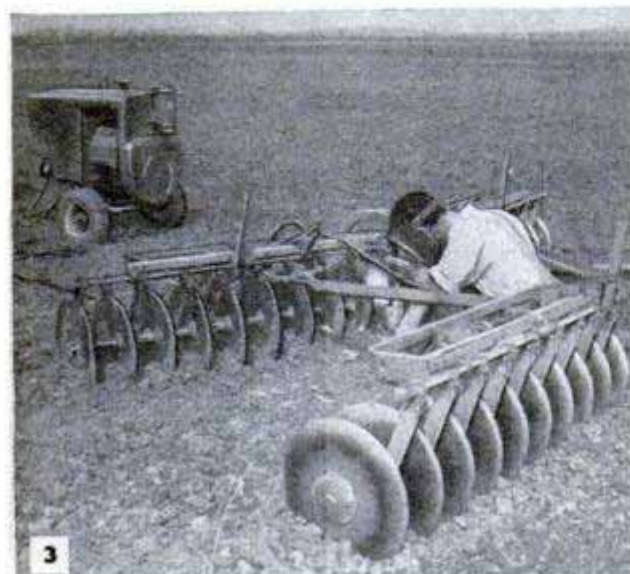
Above, repairing spring-tooth harrow with 180-amp. a.c. welder. Below, using portable d.c.-type welder for on-the-spot repairing of tandem disc harrow
