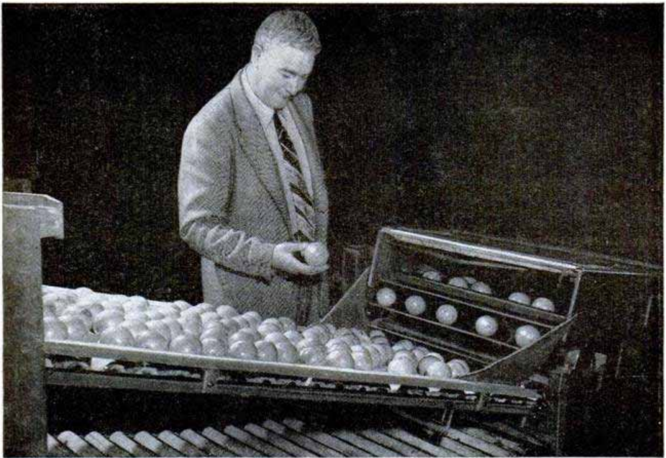
The shine on these oranges is from their transparent "second skin" of Pliofilm which retains tree freshness of fruit. The machine can wrap 800 a minute. Below, barbecue sauce is canned in Pliofilm bag
