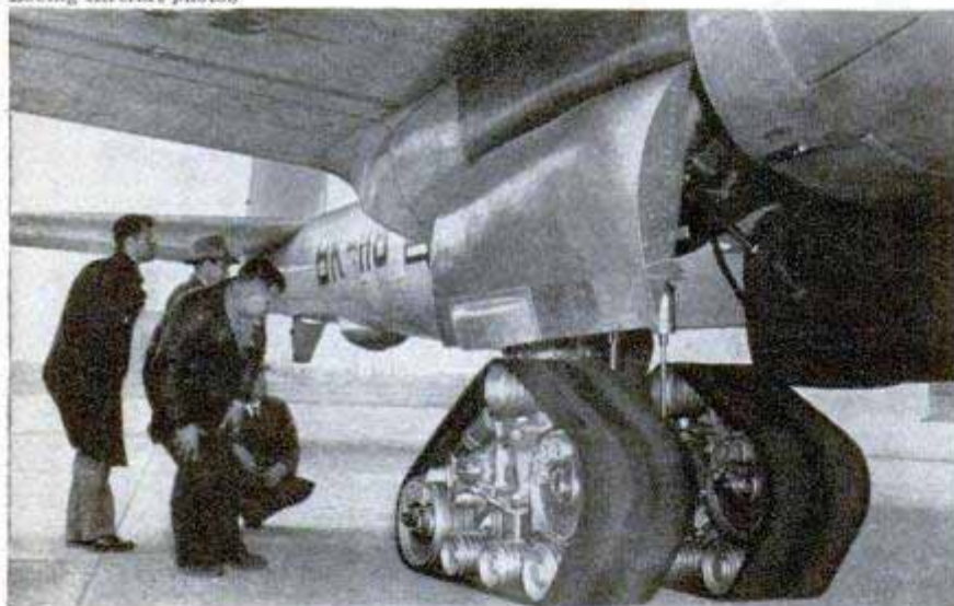
Above, inspecting camera installation for filming tractor-type landing-gear tests. Below, track tread area is three times that of double tires Boeing Aircraft photos
