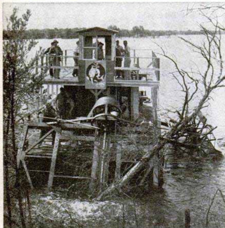
Above, the 60-inch disk saw spins out of water when the boom is raised. Below, a tree falls as it is cut six feet below the surface of the lake
