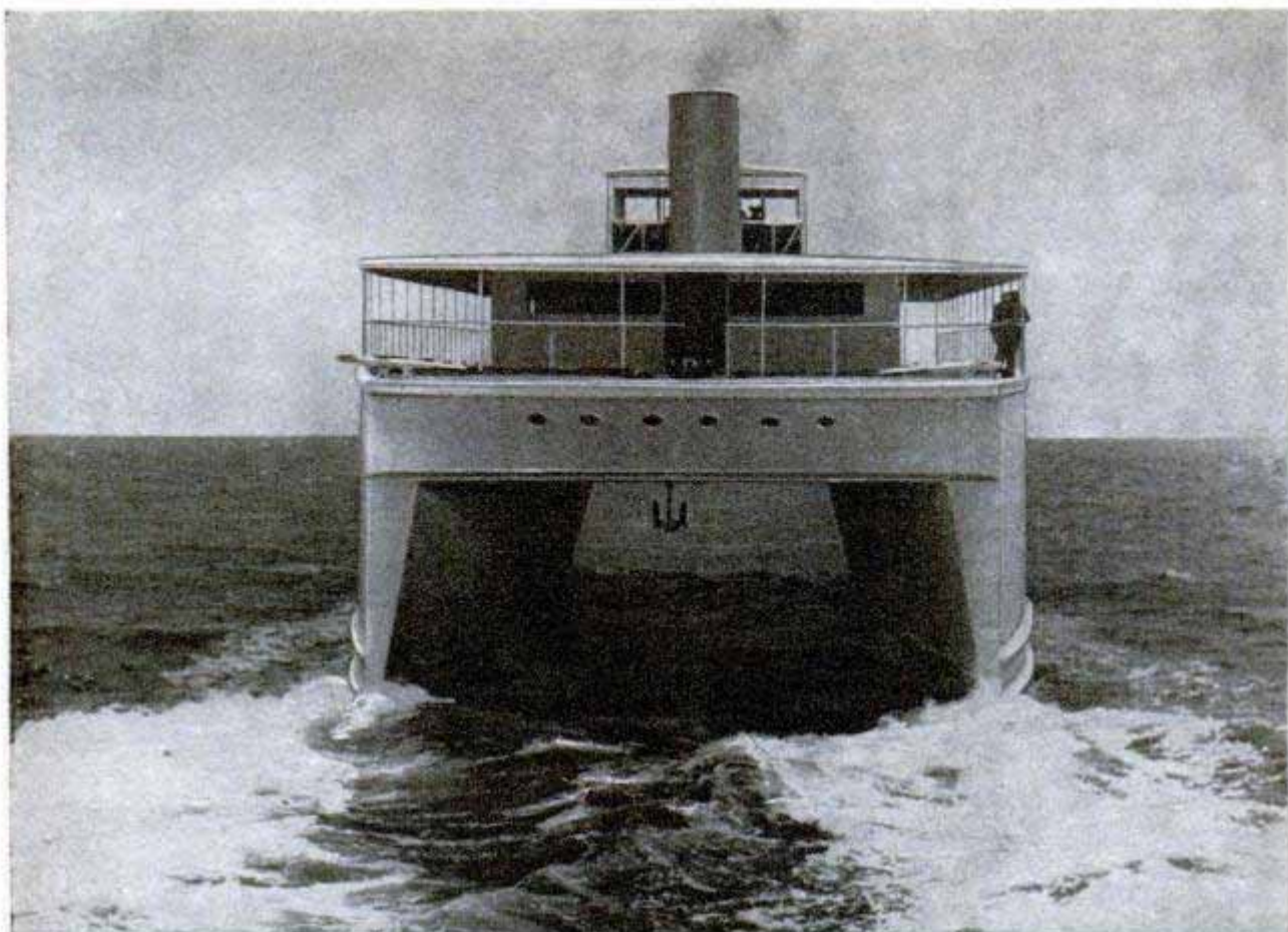
Stern view of Gar Wood's Venturi shows huge "wind tunnel" between twin hulls. Air in tunnel cushions ship
