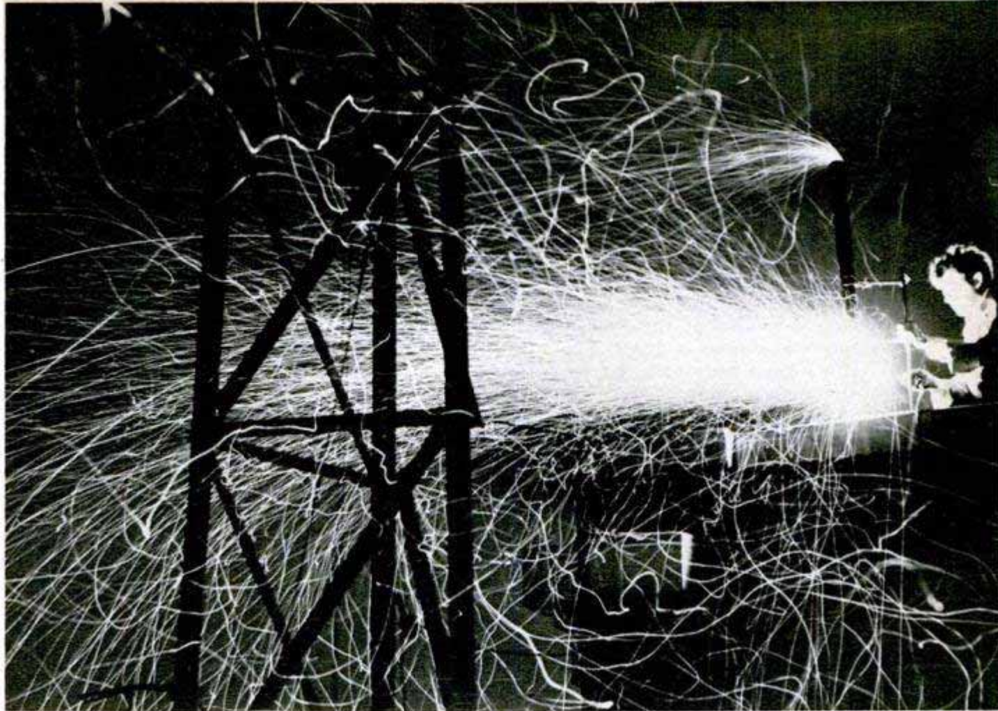
Billions of particles from this smoke generator can trick cloud vapor into freezing, creating a snowstorm
