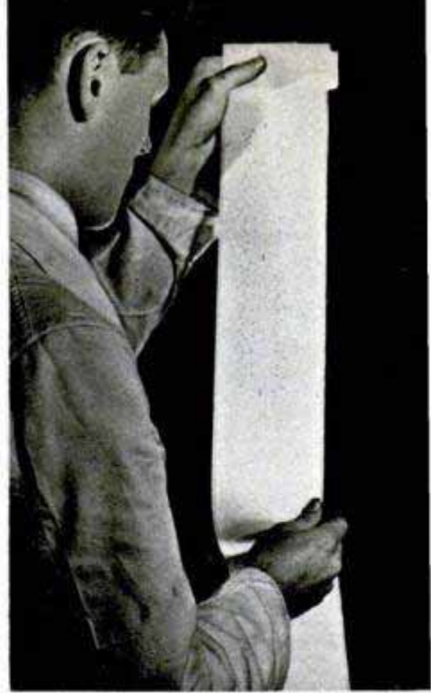
Rotofoto typesetting system starts by making a punched-paper record of the text (right) on keyboard machine
