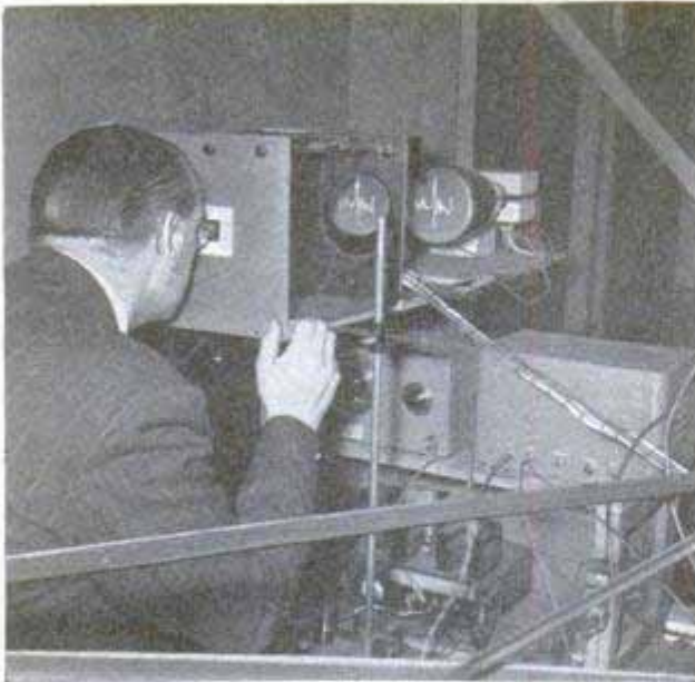
Twin tubes present two different images. The stereoscope viewer produces the three-dimensional effect
