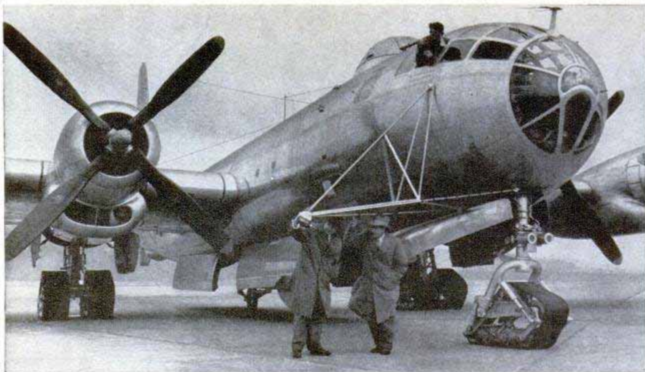
Above, inspecting camera installation for filming tractor-type landing-gear tests. Below, track tread area is three times that of double tires Boeing Aircraft photos
