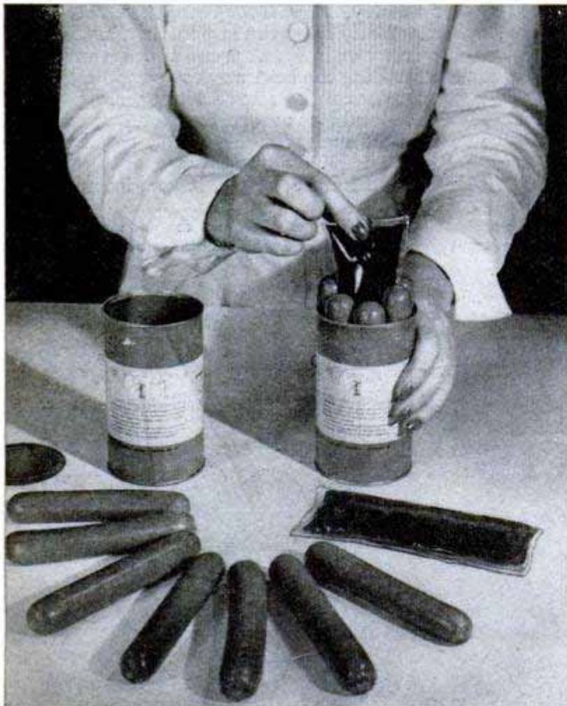
The shine on these oranges is from their transparent "second skin" of Pliofilm which retains tree freshness of fruit. The machine can wrap 800 a minute. Below, barbecue sauce is canned in Pliofilm bag
