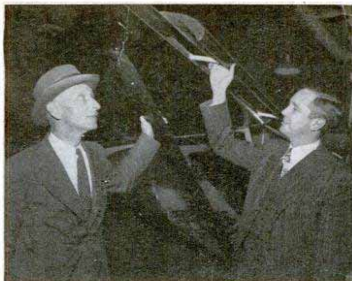
Both leading-edge slats, left, and full-span flaps (arrows), right, increase lifting ability of Heliplane wing
