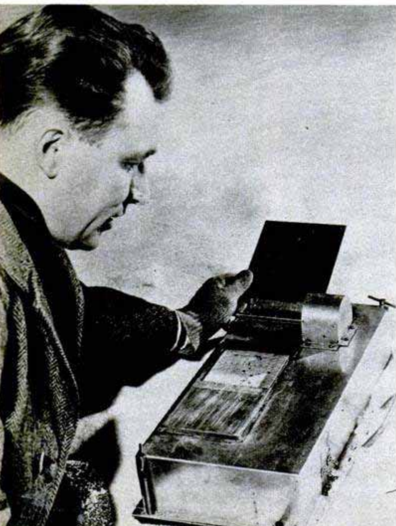
This instrument "fingerprints" a snowstorm by recording the shape, size and frequency of fall of flakes
