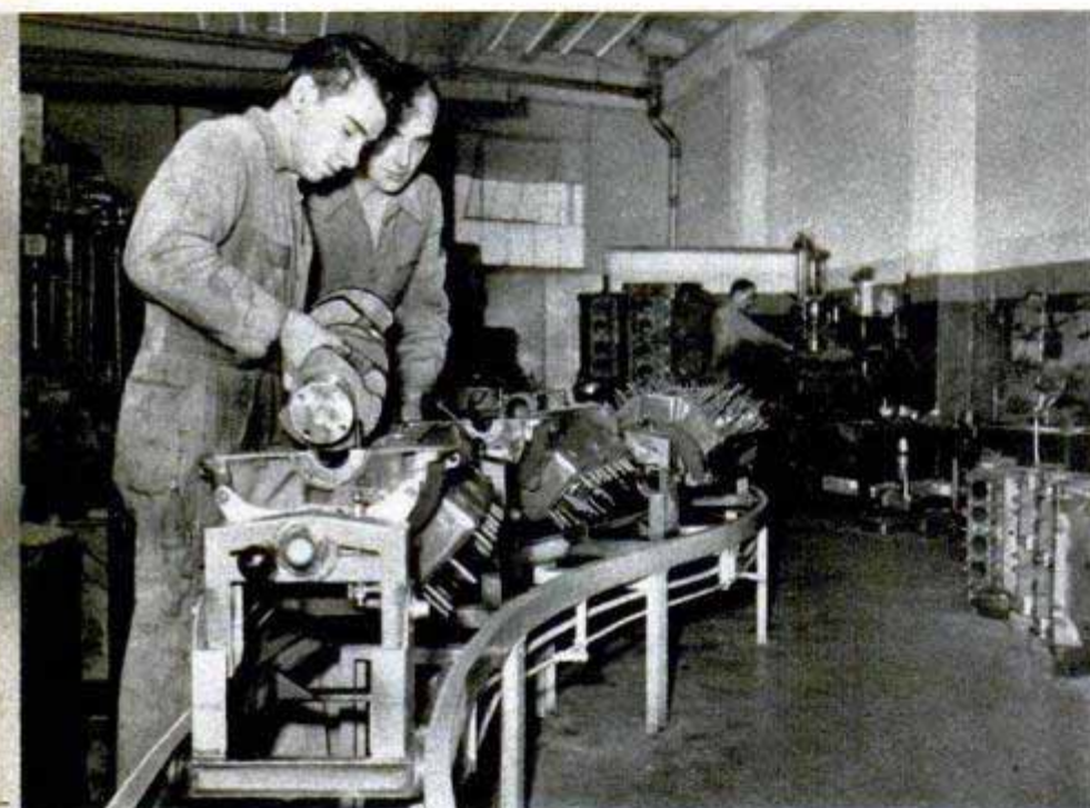
Above, assembly-line methods are used to speed the reconditioning of engines in the Automotive Center. On wheeled cradles, the motors roll along elevated tracks as parts are added. Below, bushings of connecting rods are reconditioned on a specially designed grinder
