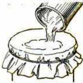
B PAINT CLEANED BY STRAINING
