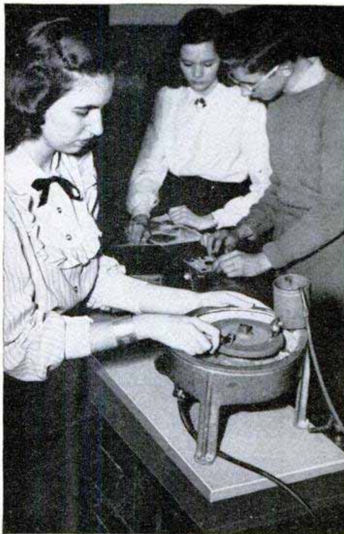
Club member progresses to the second step in gem work—roughing out the unshaped slab on a Carborundum wheel. Below, in the third step the rough cabochon is further shaped, this time by hand, with various abrasive cloths
