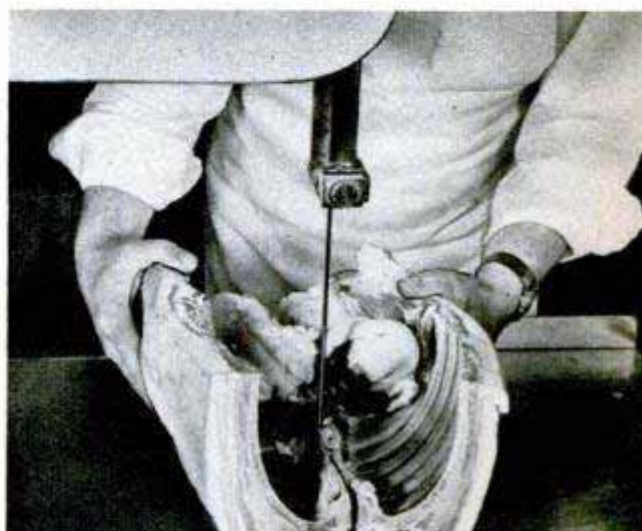
Left, diamond chips in the blade cut a pitcher in half for inspection. Right, the saw even cuts meat well
