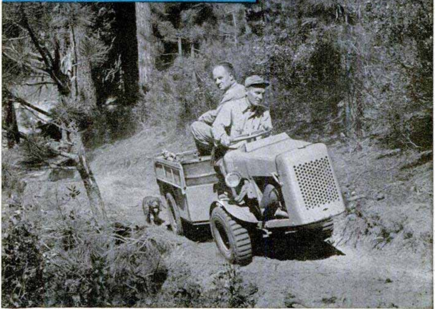
Pack horse of the fire fighters, the Mechanical Mule hauls up to 1200 pounds of men and their equipment
