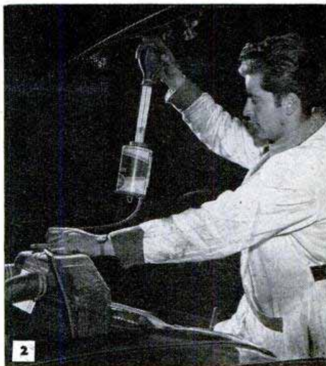
With a hydrometer made especially for the purpose, check to make sure that the freezing point of the antifreeze solution in the radiator is sufficiently low
