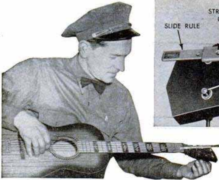
When reed vibrations are widest, the string is exactly in tune. Held in place by rubber bands, the tuner can be set for six pitches
