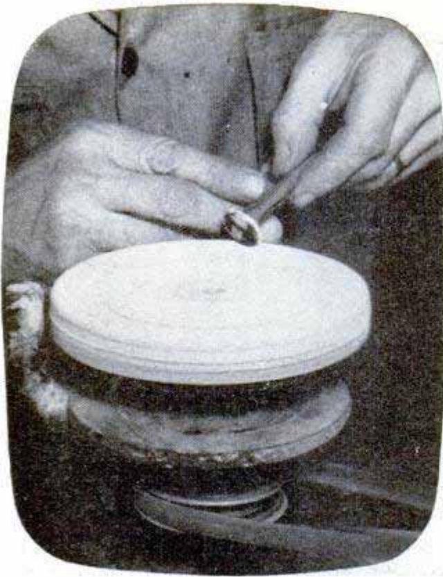
Final polish is given the ornamental gem by holding it against a felt buffer. Below, one member polishes a moss agate while another sands black jade by hand
