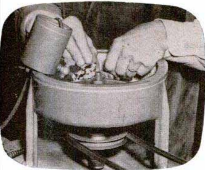
Close work! First step in making a gem is to cut a slab off the rough rock with a diamond saw. Dripping compound prevents overheating
