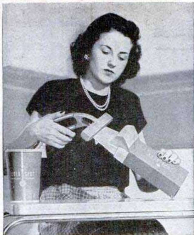
PACKAGE SEALER prepares food bags for quick freezing, sealing the opening by heat and pressure
