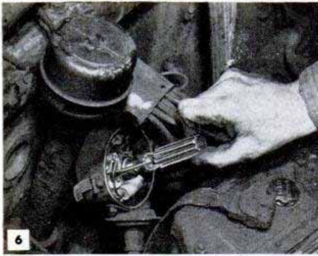
Above, set breaker-point gap by loosening screw on plate and adjusting eccentric. Below, notice dirt accumulation on outside of carburetor air cleaner
