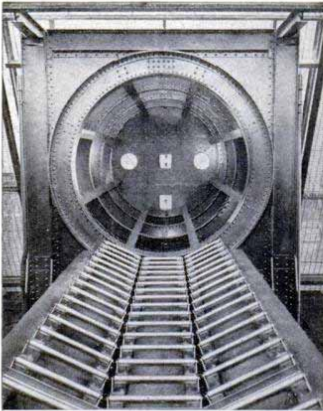
Looking up into the test frame. Rocket motors are drawn up on rollers in foreground by a mobile crane
