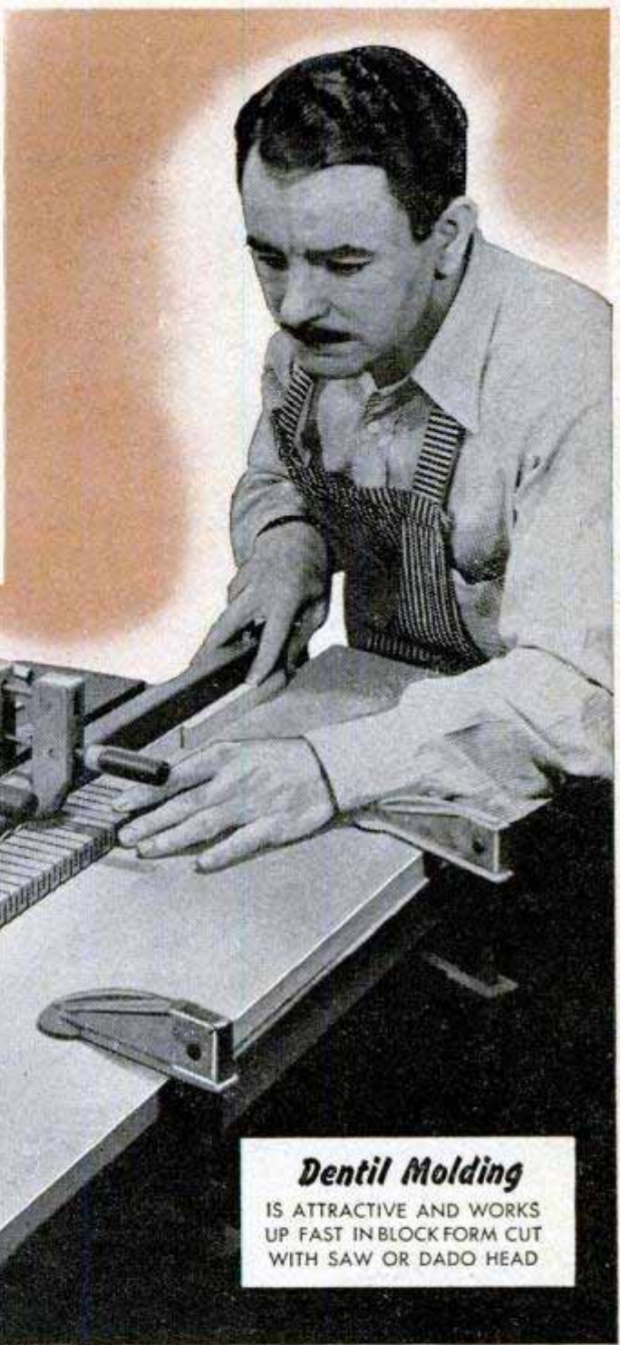
Pictured above and below is the common procedure in working out the basic dentil-mold strip on a circular saw. A block grooved alternately on both faces is sliced into strips which are glued to a base piece
