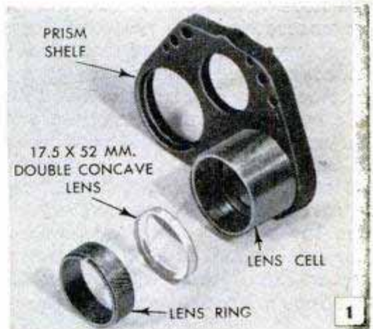
Above, assembly of negative-lens parts. Right-hand prism shelf must be threaded
