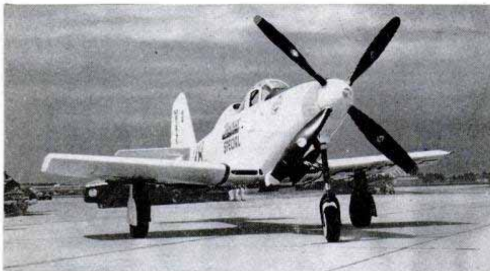
Charlie Tucker clipped eight feet off each wing of his P-63 Kingcobra and qualified for the Thompson at 392 m.p.h. He is expected to race the plane again this year. Below, P-39 owned by Chuck Brown is towed to start line
