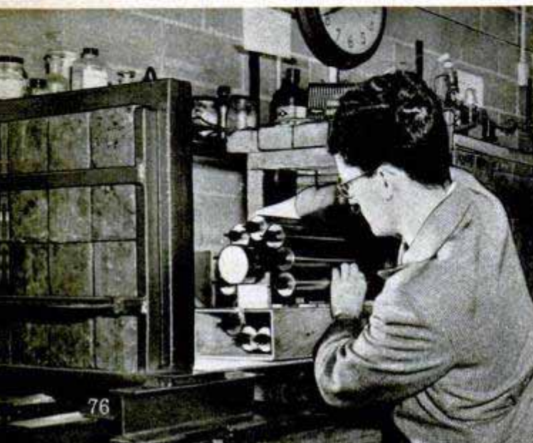
Ancient wood, above, is placed in center tube of a supersensitive Geiger counter, below, to have its age determined by measuring residual radioactivity
