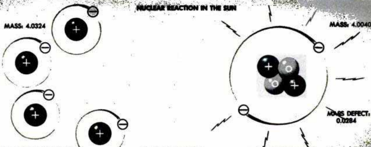
When four hydrogen atoms combine into a helium atom in the sun, there is a loss of mass, called mass defect
