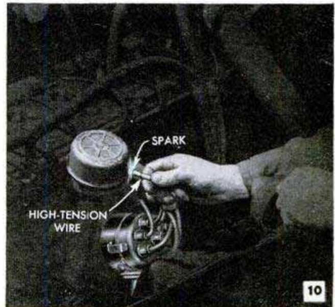
Above, a simple check will show up a faulty coil. Below, if primary current is flowing from the coil, a spark will show when the breaker points are opened
