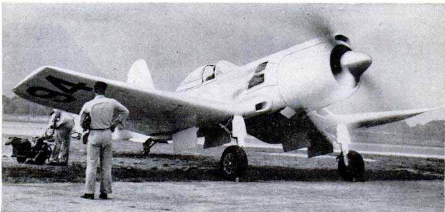
Cook Cleland revs up one of his two Corsairs (F-2-G) in preparation for the Thompson Trophy take-off in '48. The plane has a 3500-hp. radial engine
