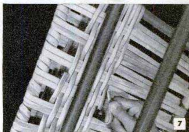
Woof is spliced by tucking end under warp strands
