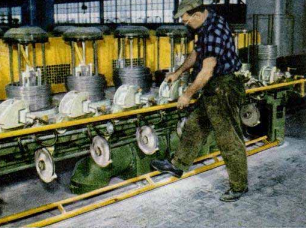
Gleaming stainless-steel wire piles up on drums after passing through dies
