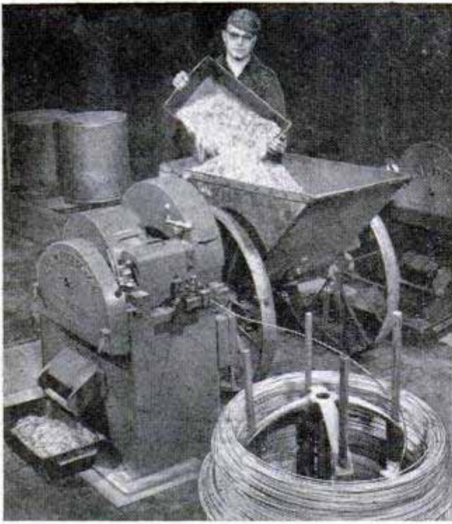
This high-speed machine turns out a real staple commodity. It stamps wire into 1000 staples each minute
