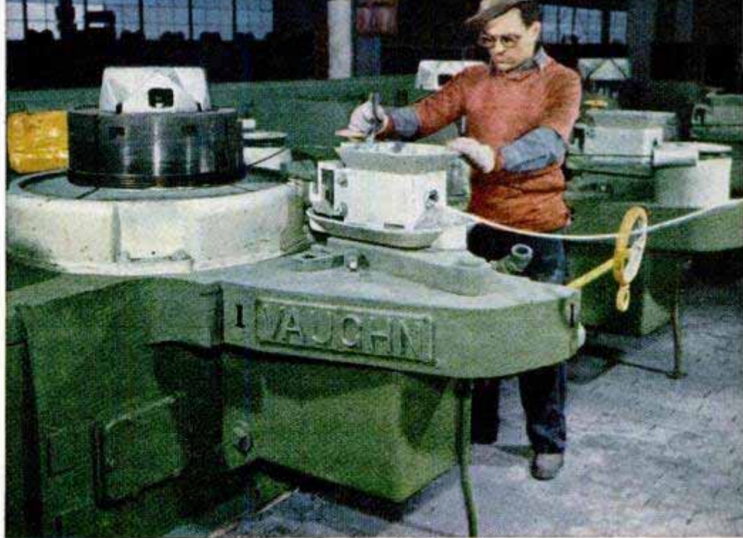
"Rod ripper" tugs rod through first die as worker stirs up soap lubricant
