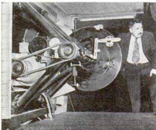
Torpedo launcher is tested by firing at target 12 feet away. Opening in curtain is \frac{1}{2} inch in diameter larger than torpedo. Left, close-up of torpedo on wheel-launching device. Below, magazines of five high-speed underwater cameras in the launching tank
