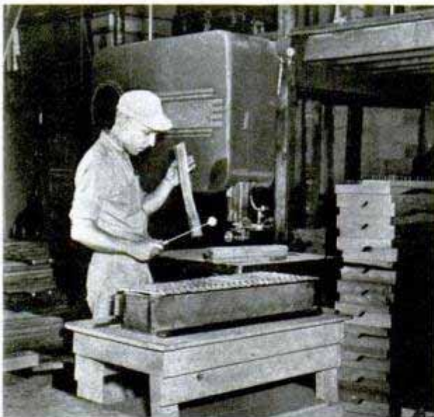
Musician tests tone of rosewood bar after cutting it on bandsaw. Right, finished bars are exactly in tune
