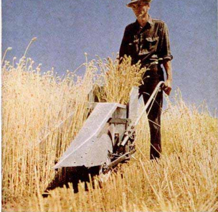
Above, research worker cuts down one row of experimental wheat at a time with this small reaper to avoid mixing the variety with adjacent growths. Below, another miniature machine for test stations is this thresher being used here on a pea crop
