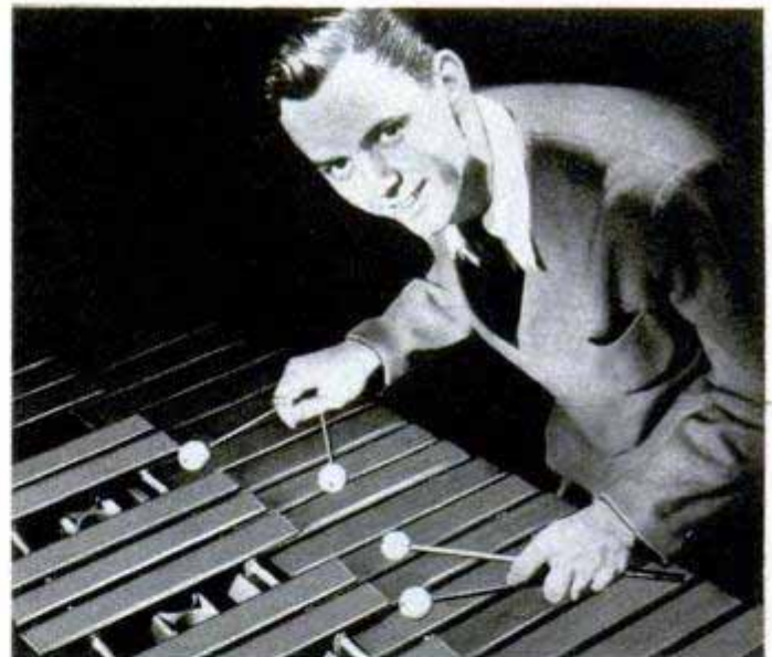
Musician tests tone of rosewood bar after cutting it on bandsaw. Right, finished bars are exactly in tune
