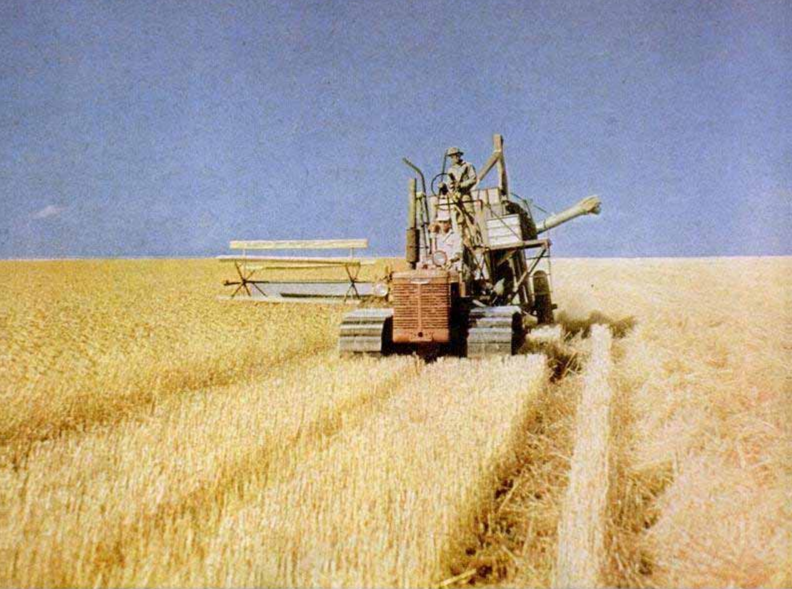
Tractor-drawn combine harvesting wheat in Washington. Pipe projecting at right unloads grain into trucks
