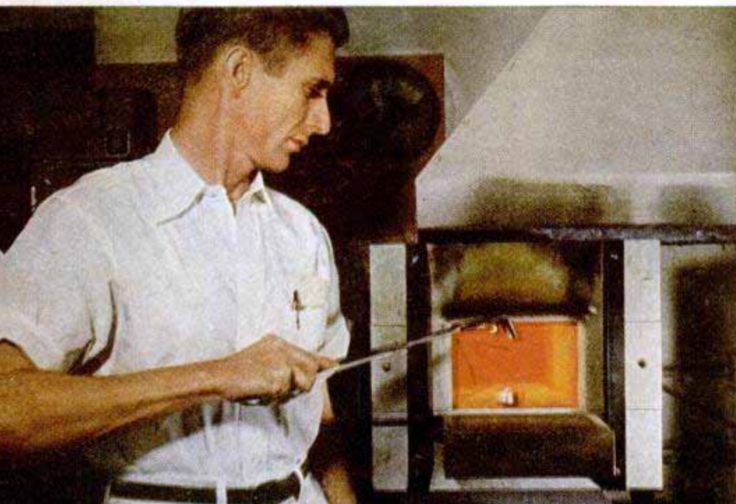
Flour sample is placed in an electric furnace to test its mineral content
