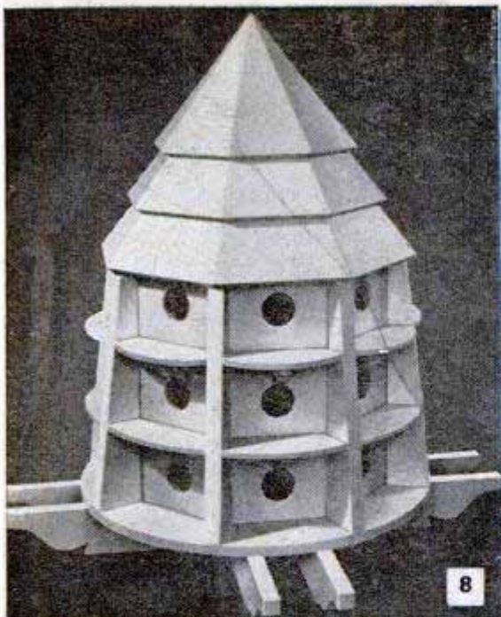
8-SIDES, 35° MITER TAKES 18 1/4° TILT AND 76 1/2° AT MITER GAUGE
