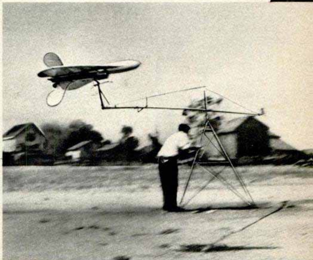
Operated by middle man in background, test stand forerunner of VJ-100 tilts over on its side and flies in circles. Experiments indicated ship had enough stability to back safely down to earth, at low speed, against the jet thrust. Below, the model whirling around stand in level flight
