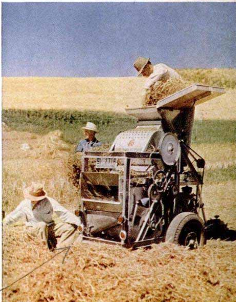
Above, research worker cuts down one row of experimental wheat at a time with this small reaper to avoid mixing the variety with adjacent growths. Below, another miniature machine for test stations is this thresher being used here on a pea crop
