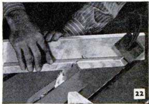
TOPS AND BOTTOMS OF CORNER BLOCKS ARE CUT WITH MITER-GAUGE SETTING FROM TABLE. SAW TILT IS SAME AS WORK ANGLE. (NOT TAKEN FROM TABLE)
