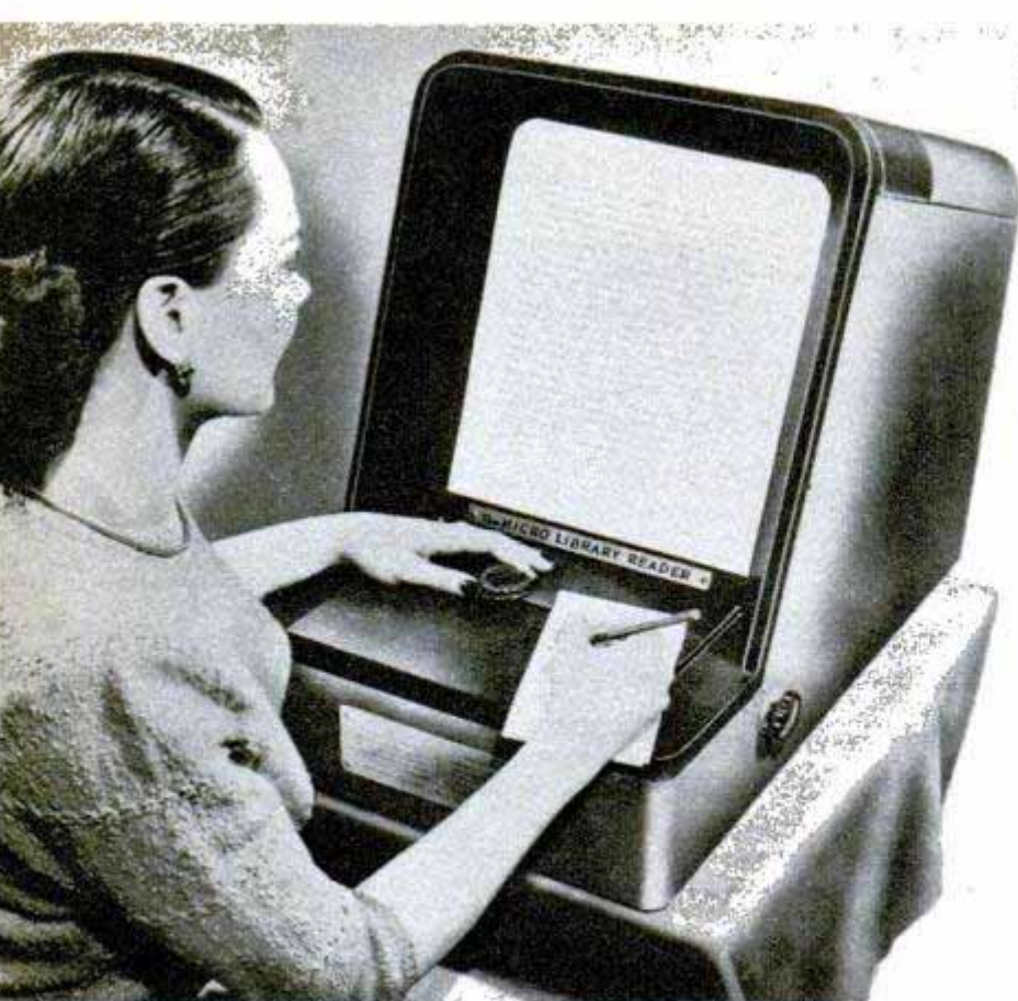
Magnified 24 times, the microtext is as easy to read as the original. Right, inserting a card in the reader
