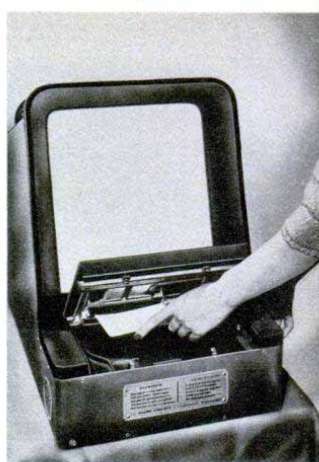
Magnified 24 times, the microtext is as easy to read as the original. Right, inserting a card in the reader
