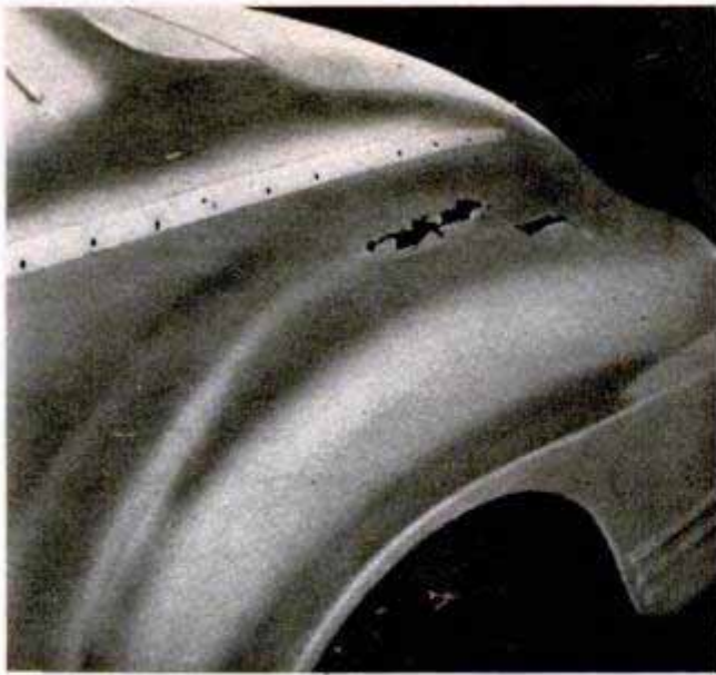
Rusted out and weakened area on top of a rear fender first is sanded to provide a clean surface for patch
