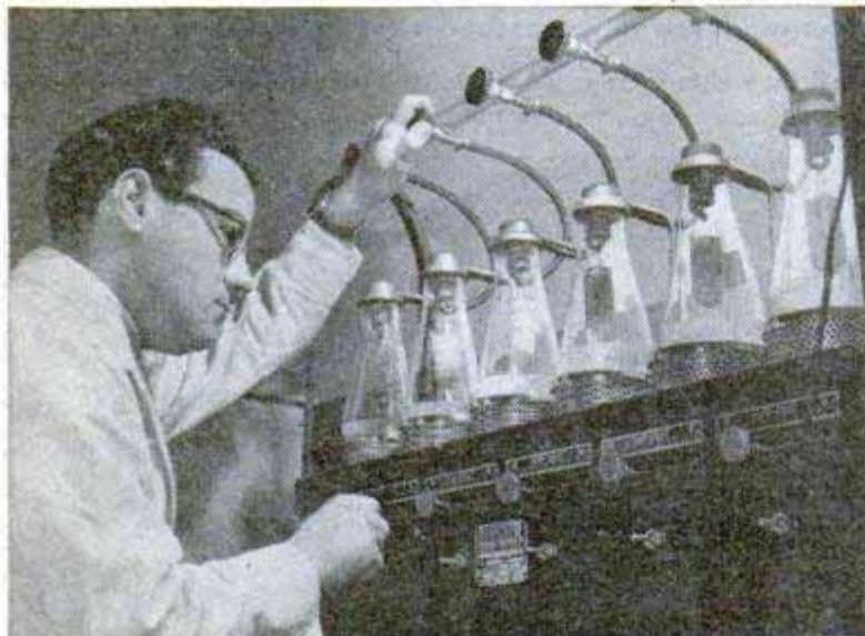
Above, extractor measures the oil, fat and grease in various materials. Below, mason's trowels are placed in this machine that rubs them back and forth on emery boards to test quality
