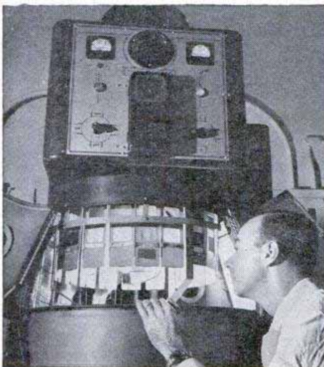
Above, test device is so sensitive it measures accurately the force required to flex the finger of a work glove. Below, left, exposing fabric to carbon arc light in this fadeometer tests its resistance to fading. Below, right, the ability of nylon thread to take dyes is measured here
