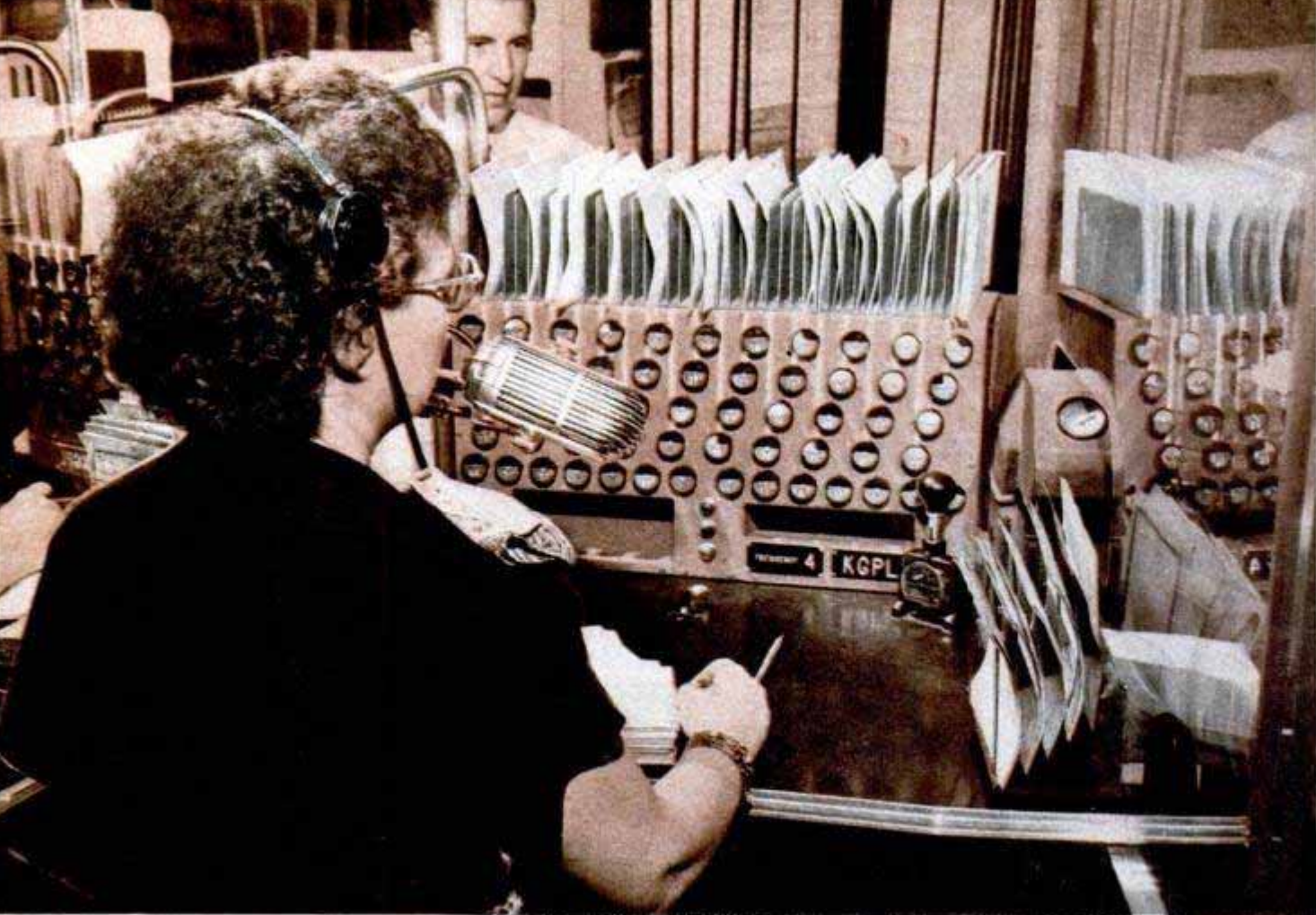
Each button on microphone-room operator's panel represents prowl car and indicates its operating status
