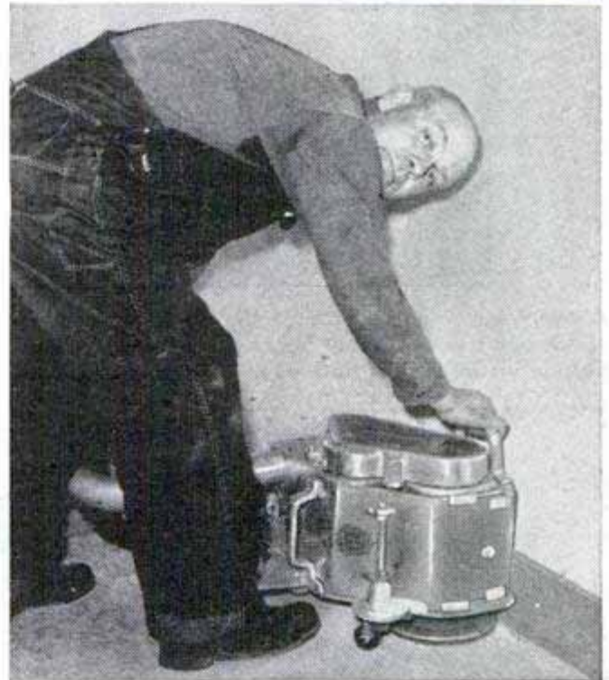
Left, the combination sander in its normal position. Right, the two-belt bowling-alley sander. Insert at top shows the new sanding drum. Below, combination sander with side spinner in place for sanding edges
