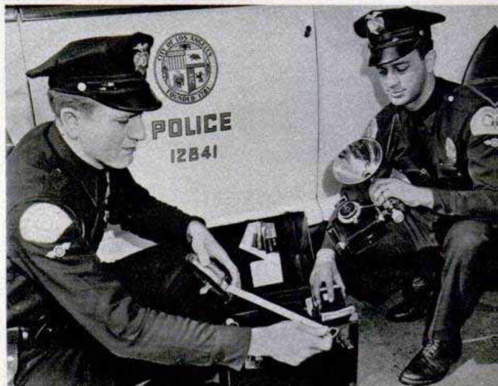
Top, operator at KGPL takes down radiogram coming to Los Angeles from East on transcontinental police relay system. Below, only two bolts have to be loosened to replace transmitter in car trunk
