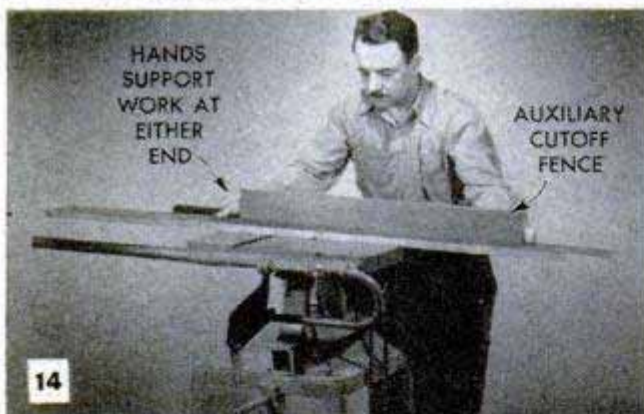
USE AN AUXILIARY FENCE WHEN CROSSCUTTING LONG STOCK. USE BOTH HANDS FOR FEEDING WORK
