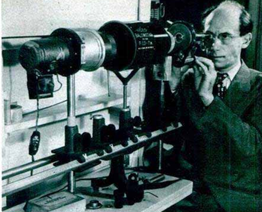
Inventor Frank G. Back inspects his "owl's eye" Video Balowstar lens. Designed for television pickups under dim light, the lens costs $2700
