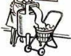
BASKET CART will haul anything from groceries to laundry. The tubular-steel frame has a folding stand that holds it upright when you park the cart. The two large wheels roll easily, even up and down stairs. The rack holds a standard bushel basket and pivots on the sides for dumping
