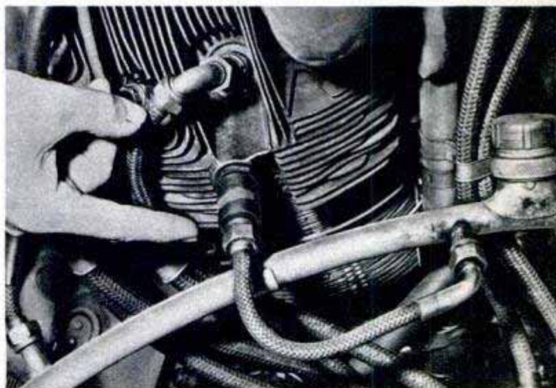
Compact engine analyzer fits the plane's control console. Flight engineer is pointing to the "scope" which shows the wave pattern. Below, nerves of the analyzer are vibration pick-ups mounted on cylinders
