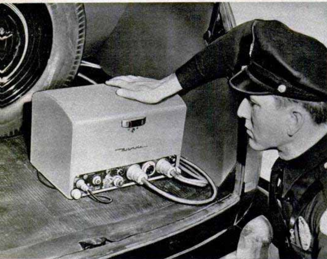
Top, operator at KGPL takes down radiogram coming to Los Angeles from East on transcontinental police relay system. Below, only two bolts have to be loosened to replace transmitter in car trunk
