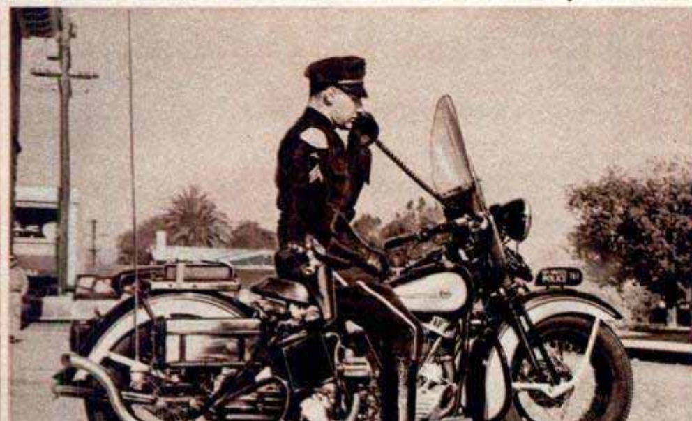
Transmitters on motorcycles are distributed between two boxes flanking rear wheel to equalize the weight
