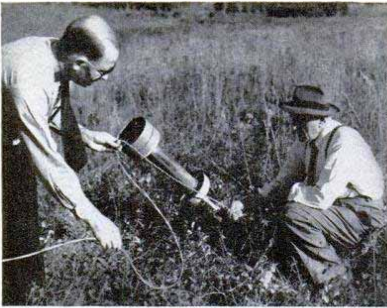
Stake fastened to the rocket motor plunges deep into the ground, providing a strong anchor that could be used with breeches buoy
