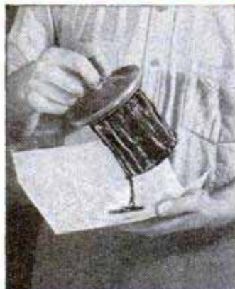
A CLOGGED OIL FILTER IS DANGEROUS. Engine-wrecking sludge and abrasives threaten sizable repair bills.
