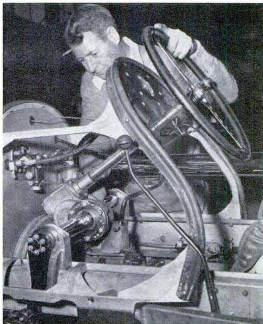
Steering wheel of one of Moore's three new racers is geared to drag-link arms that in turn are connected with the front wheels. Below, Moore's new rear-engine, rear-drive car has a 3½-inch tubular frame. It will have only five inches of clearance with the wheels installed
