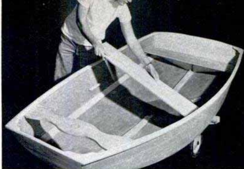
Working from official plans, this young enthusiast built his own Sabot. It takes about six week ends to complete the boat. The photo below shows the leeboard which provides the keel effect for the craft. When the boat is sailing, the leeboard is vertical
