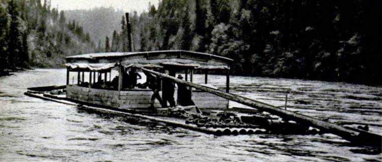
Steering the clumsy wannigan in swift water is hard work. It takes three men to handle the 50-foot rudder
