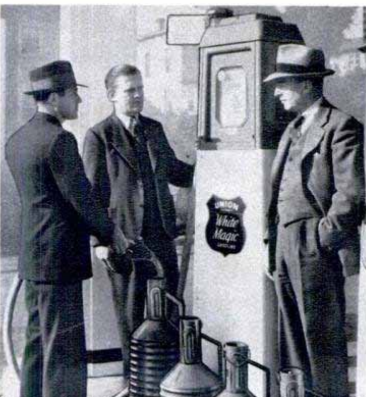
Testing accuracy of service-station gasoline pumps with cans measuring one, two, three and five gallons
