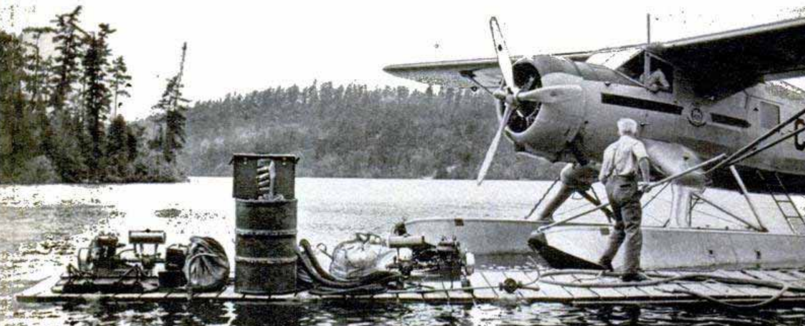
↑ Fire pump is set up to carry water from the nearest stream. Seaplanes carry all the equipment as well as the fire fighters. Below, portable equipment is loaded aboard one of the planes for quick trip above forest
