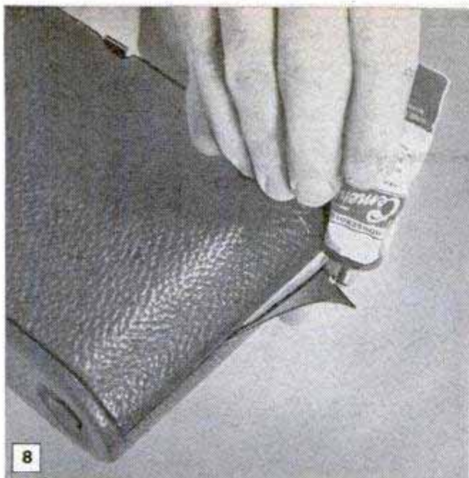
8 Torn covering can be replaced with household cement. First coat both surfaces, then press them together
