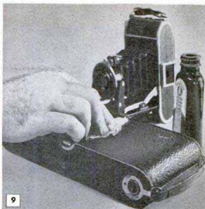
9 Leather dressing will make a worn camera look new. Use cream type which contains preservative and dye
