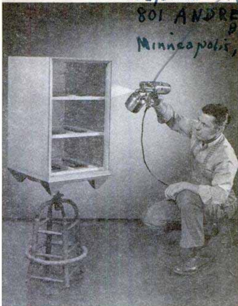
Above, a piano or draftsman's stool provides an excellent turntable when spraying lacquer on the smaller units. Below, a power sander makes play of sanding the broad, flat surfaces, but care must be used to avoid cutting through the top veneer
