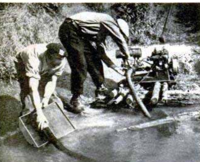
↑ Fire pump is set up to carry water from the nearest stream. Seaplanes carry all the equipment as well as the fire fighters. Below, portable equipment is loaded aboard one of the planes for quick trip above forest
