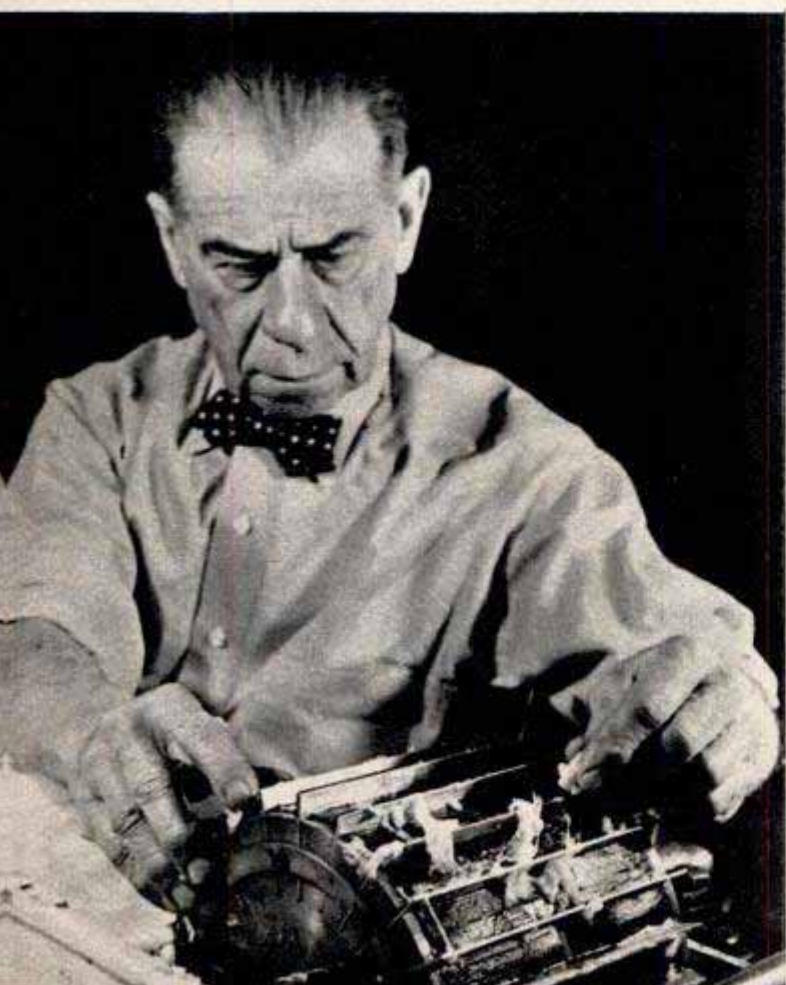
Beater roll with cover removed to show stainless-steel blades, which revolve against the corrugated bedplate, pounding the pieces of cloth into a pulp
