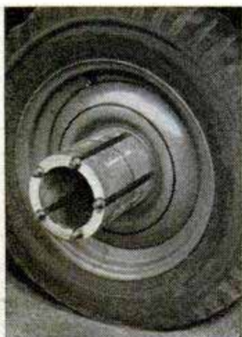
Left, bolts and spacers in place ready for extra wheel. Right, maximum traction is provided with duals on all wheels and tires at low pressure
