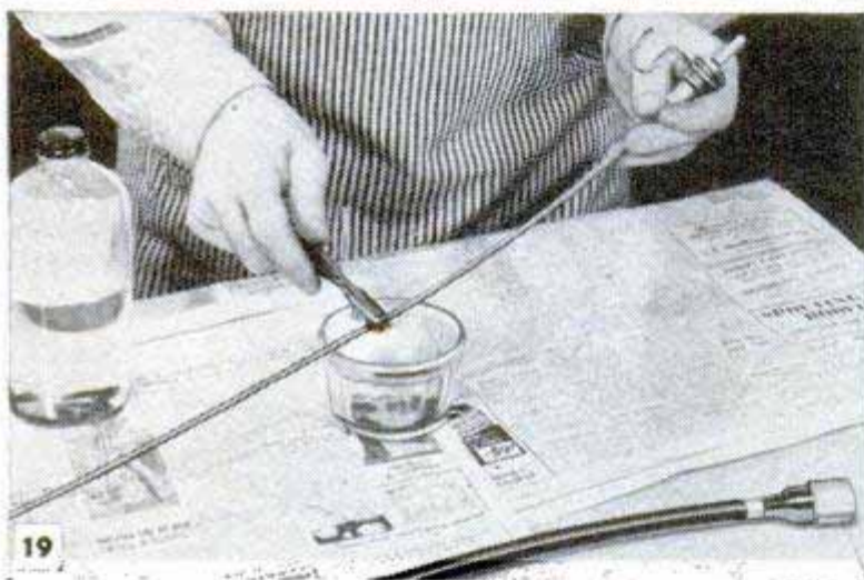
Core of shaft is cleaned and lubricated at regular intervals
