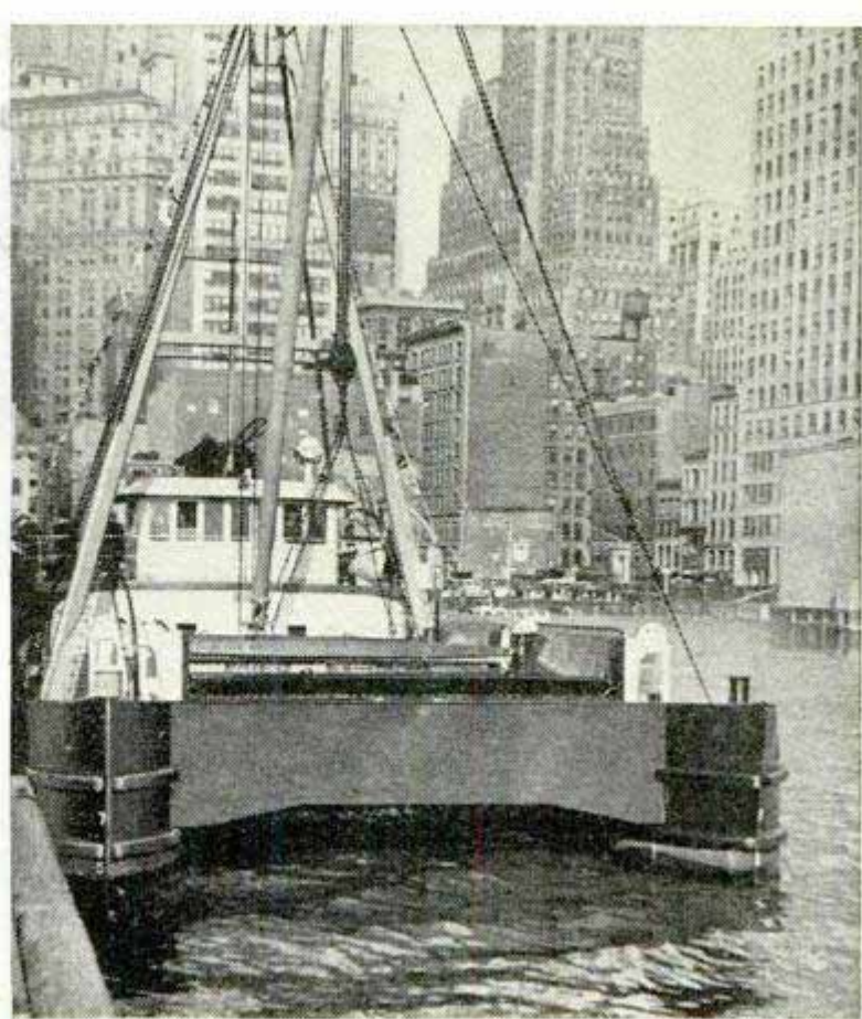
Reporters on trial run watch crewmen, upper left, guiding driftwood between hulls. Right, front view of vessel
