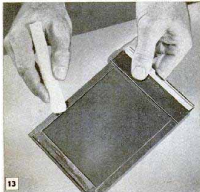
13 For a smooth sliding action, rub paraffin on sliding surfaces of film holders, above, and tripod, below
