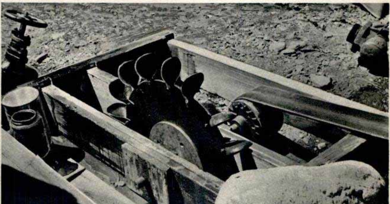
Top, sketch shows over-all plan of Sweet's homemade gold mine. Above, winch-and-gear system was built around old Chevrolet transmission. Below, water wheel is turned by gravity-flow stream piped from creek
