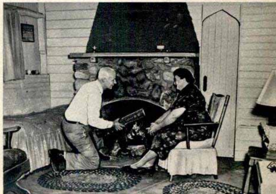
"One end of our living room is completely enclosed with glass. We poured a smooth concrete floor and marked it off like a compass card. At the opposite end is our sure-drawing fireplace with back and arch made of brick. We laid up a facing with field stones"
