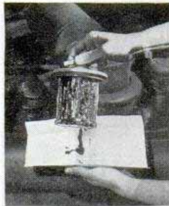
LOOK AT THAT MUCK... an oil filter element loaded to capacity with sludge, grit.
