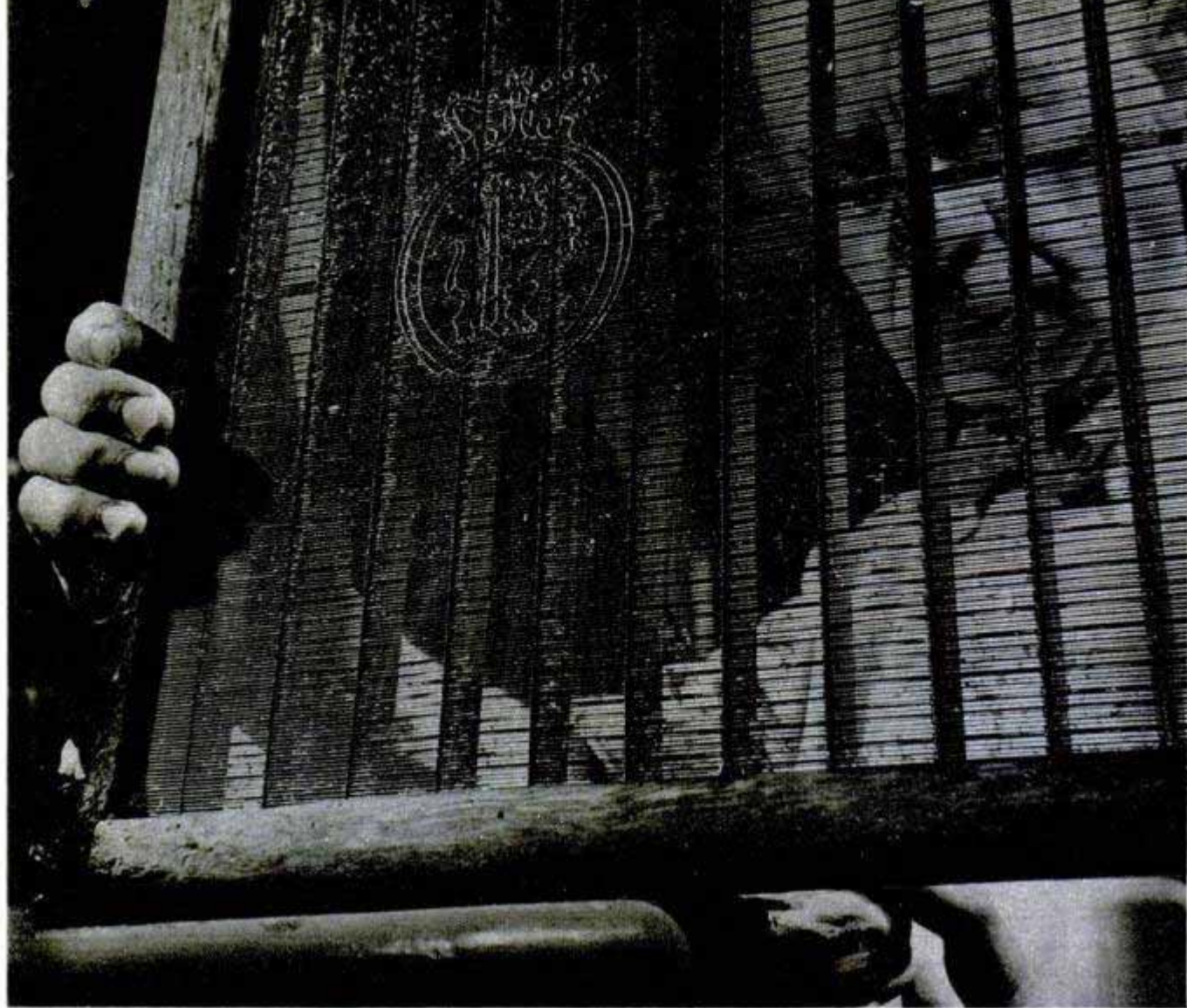
Elliott inspects the watermark design on the screen of a hand mold. The design is formed with fine wire
