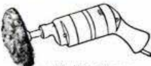
with the slip-on lamb's wool bonnet, it is a portable power-driven polisher or buffer.
