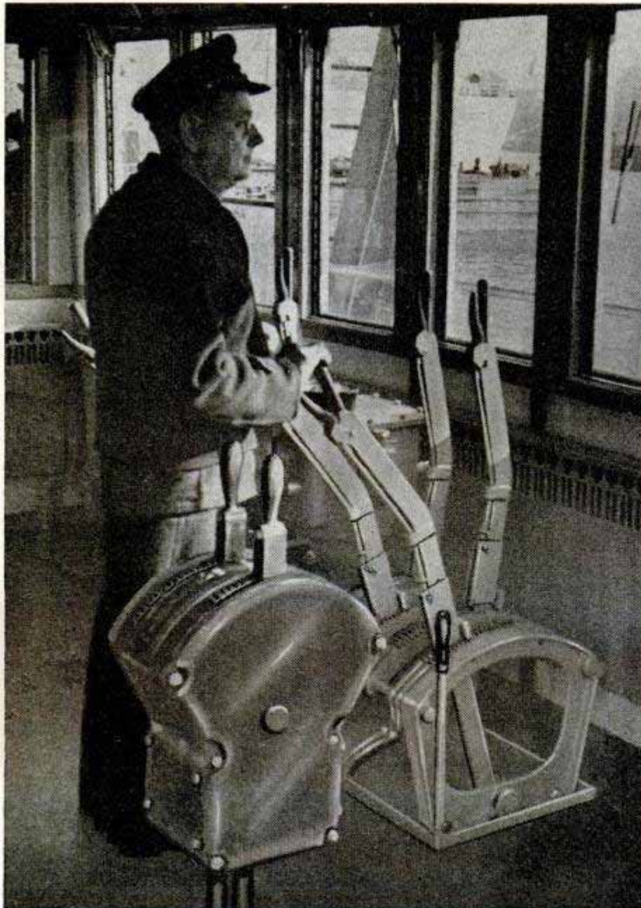
From control bridge straddling twin hulls of U. S. Army's Driftmaster, Capt. William P. Hocking operates levers that raise and lower drift nets
