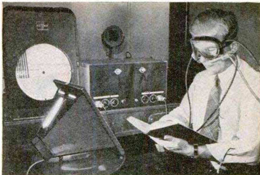
Above, photoelectric cells measure the blink rate of the eyes as smog is forced inside goggles. Light, reflected by the whites of the eyes, actuates cells. Below, Venturi scrubber washes impurities from the air
