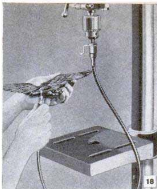
Power take-off for driving flexible shaft can be made from drill-press spindle, as above, or from lathe motor, as at the left
