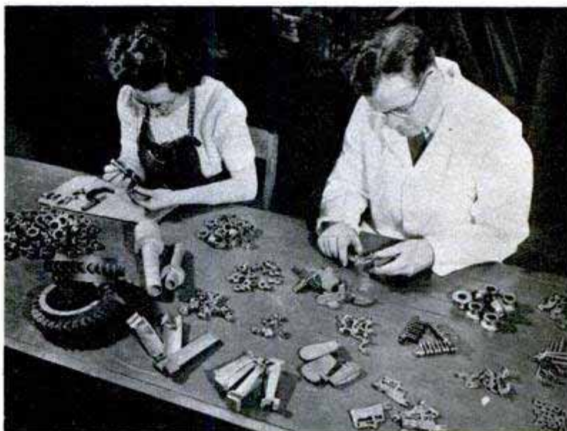
Top, left, injection molding of wax patterns. Dies are clamped in press and wax pumped in through flexible hose. Right, the molten metal is poured into molds. Above, final inspection of the castings. Parts on table are some produced by new process
