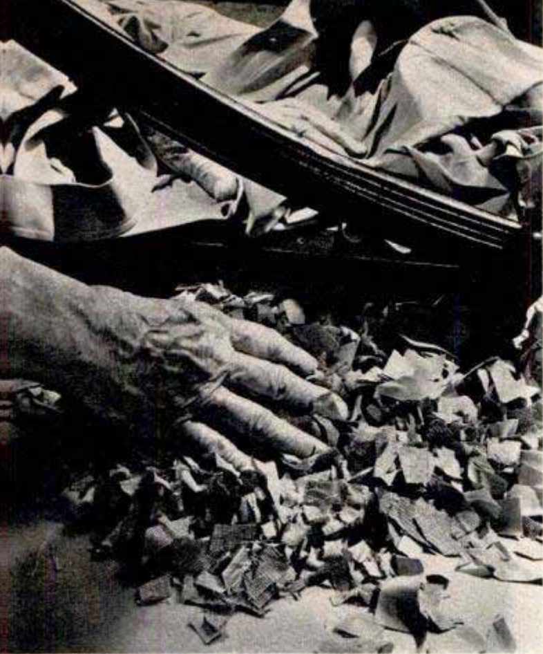
Elliott starts the process of converting a castoff shirt into fine paper by cutting the garment into many small pieces. The sharp blade of this cutter speeds the task. The buttons were removed earlier
