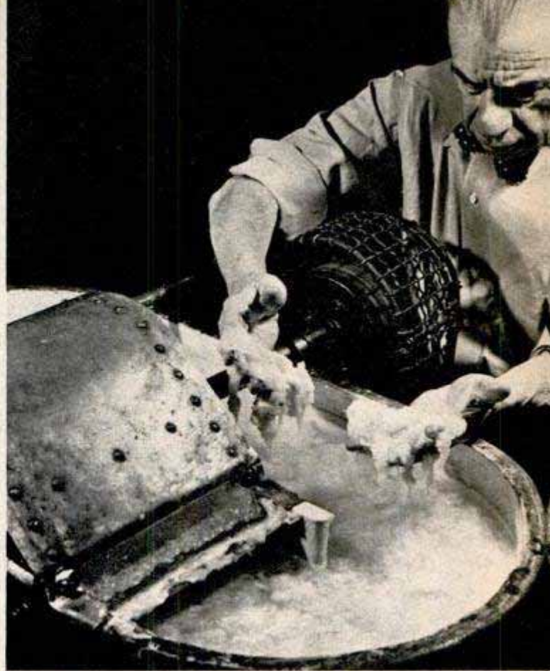
Rags are placed in this tub where the motor-driven beater converts them into a fibrous mass. It takes several hours to complete the process. Elliott is examining the pulp which is still in threaded state
