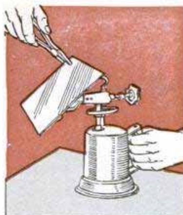
1st —Anneal copper by heating, then quenching in water
