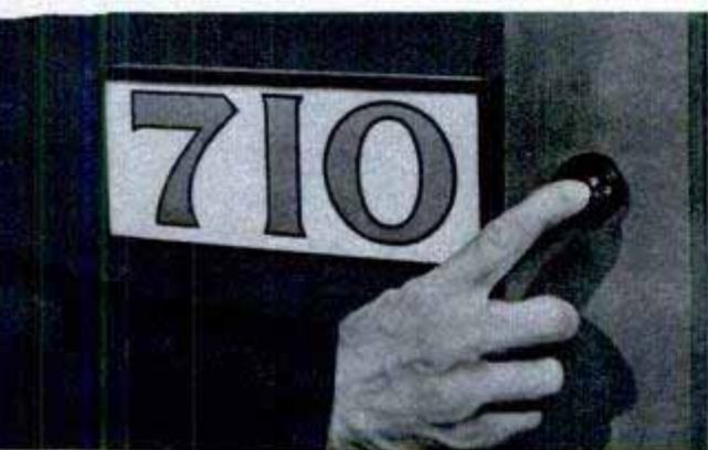
↑ GLOWING HOUSE NUMBER has wires that attach to the terminals of the doorbell button, providing constant illumination. The cost of operating the numeral is less than two cents a month
