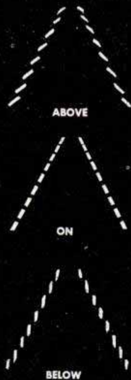
Each of the diagonal units of the slope-line lighting system pierces the sky with ten 500-watt landing lamps. Above right, diagrams show appearance of the slope lines to an incoming pilot when he is above, on and below the glide path
