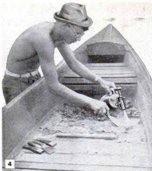
When refinishing, pay special attention to the inside of the boat. Damaged paint should be loosened with a blowtorch and scraped to expose bare wood
