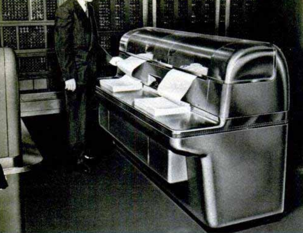
Printer publishes the running results at a rate of 24,000 digits a minute, permitting scientist to modify problem as he sees results
