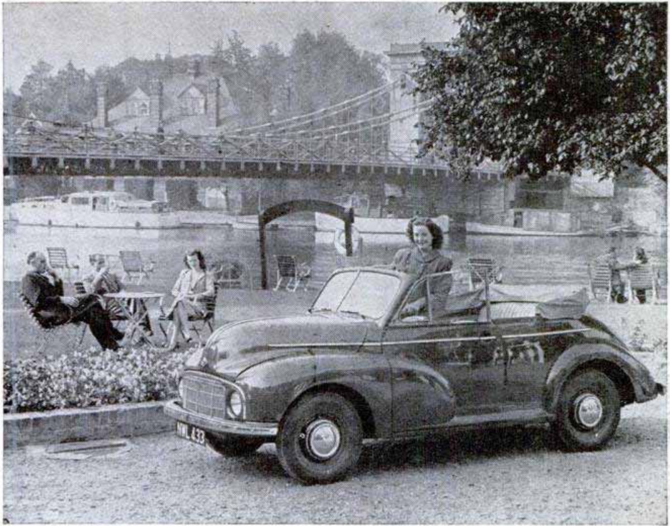
This four-cylinder Morris Minor convertible carries four persons and travels 40 miles on a gallon of gas
