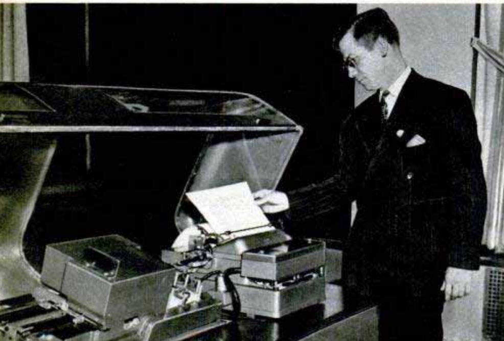
When problem is solved, typewriter reads numbers from cards and prints them in form suitable for publication by offset printing International Business Machines Corp. photo
