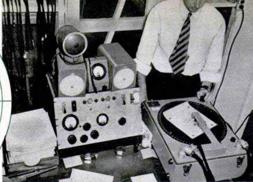
Stylus on swinging arm plots the all-around range of antennas on a 360-degree chart fastened to turntable. On the chart, shown at left, the masking effect of a ship's superstructure is very apparent
