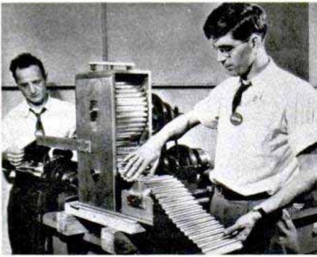
Above, left, long strips of the aluminum foil are corrugated by machine preparatory to assembling the panel. Right, several pieces of the corrugated foil are assembled for application of adhesive to form honeycomb
