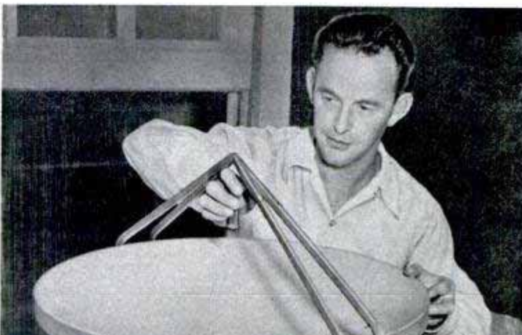
Above, this complex impedance chart is used in measuring the electrical characteristics of antenna designs. Below, worker adjusts a wave guide that emits radio waves which are beamed straight up by the parabolic reflector for the reflection tests
