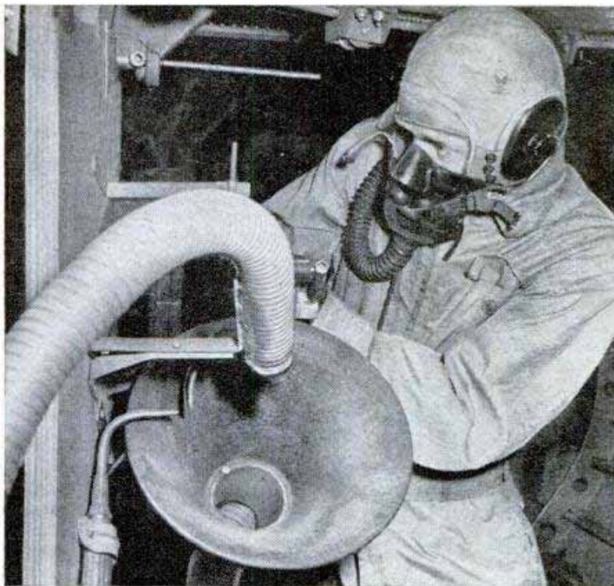
Inside this funnel-shaped chamber, twine impregnated with silver iodide is burned to send out clouds of particles that can grow into snowflakes. Below, a map of the seeded area shows how the location of intense rainfall corresponds to the up-wind location of seeding operations
