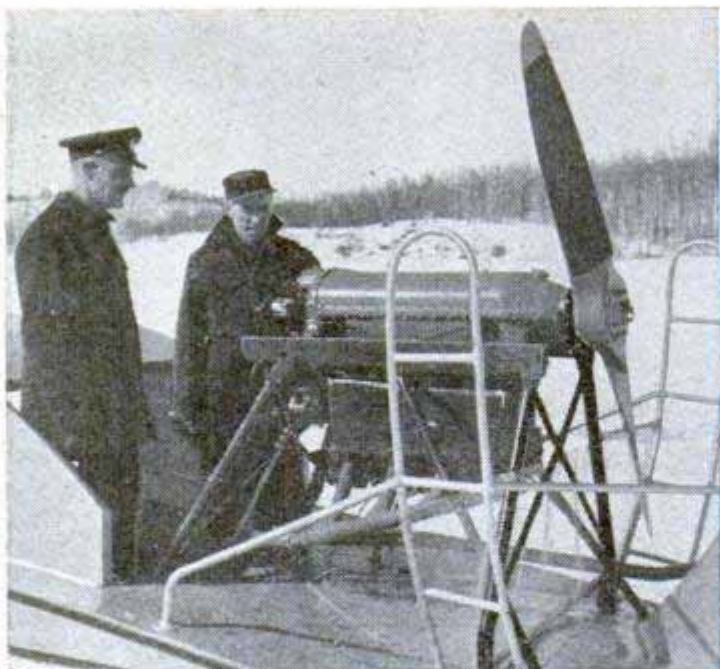
Airplane engine mounted on steel piping sends craft skimming across ice. Below, bow is covered with galvanized iron
