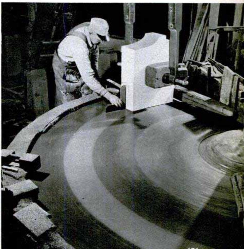
In the finishing mill, the marble is rubbed down to the exact size on huge cast-iron wheels. Sand and water are the abrasives
