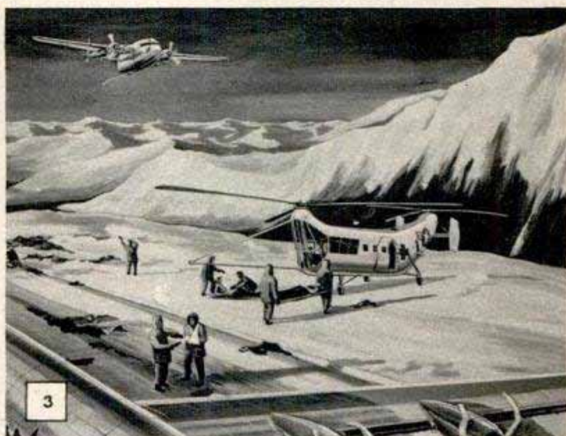
After rescued are loaded aboard (3), helicopter takes off and makes a midair pickup of trailing line (4) for tow to the nearest air base
