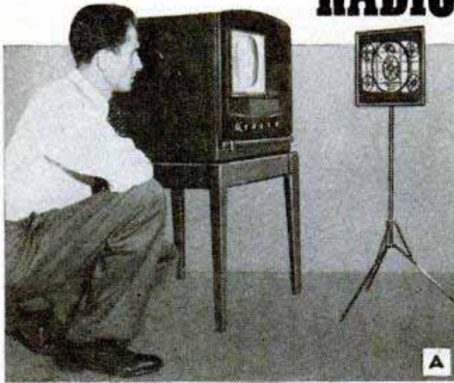
A —Portable Miro-Pix mirror enables TV serviceman to view the screen pattern of a television receiver while adjusting the rear controls and ion trap
