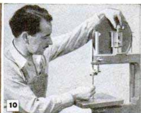
10 BLADE TENSION MUST BE SET BY FEEL. BLADE SHOULDN'T BE TOO TIGHT
