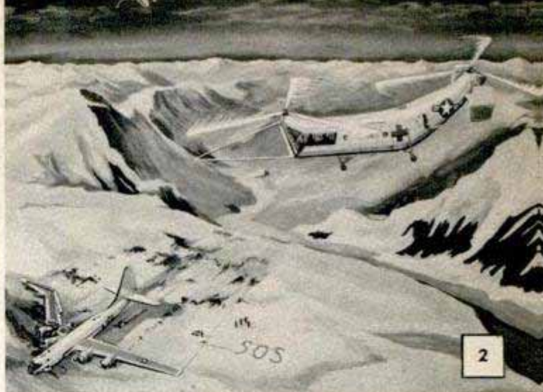
Combining virtues of each type aircraft, long-distance plane tows a short-range helicopter (1) to remote site of air crash. At the scene (2), helicopter's engine is restarted, the tow is unhitched and a landing is made
