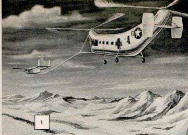
Combining virtues of each type aircraft, long-distance plane tows a short-range helicopter (1) to remote site of air crash. At the scene (2), helicopter's engine is restarted, the tow is unhitched and a landing is made
