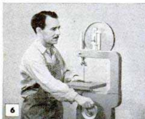
6 TRACKING SHOULD PUT BLADE IN CENTER OF WHEELS
