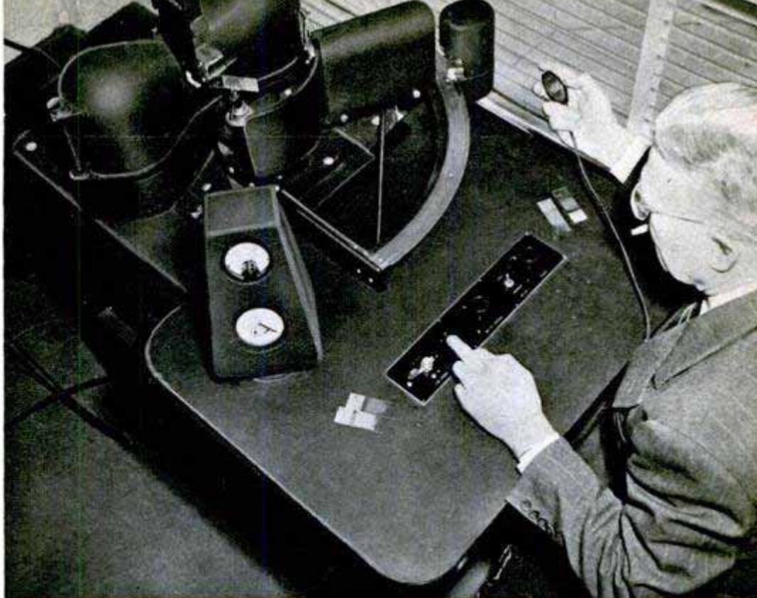
Above, final test of uranium ore is made with a $7000 Geiger-Mueller counter X-ray spectrometer that records all elements contained in sample
