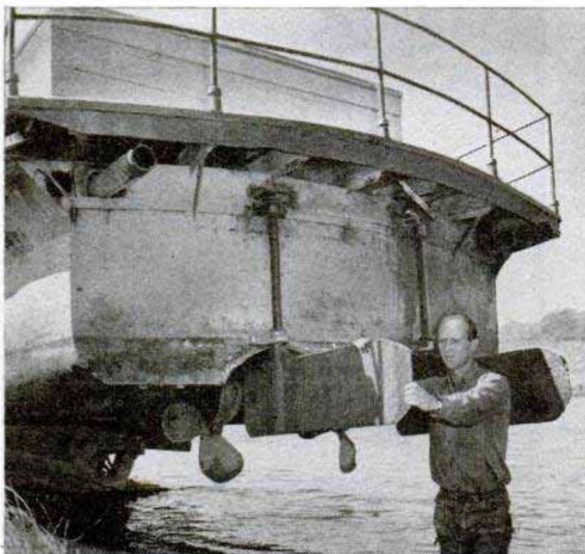
Two 165-hp. diesels power the twin screws of the Florence. The oversize twin rudders aid steering in rapids
