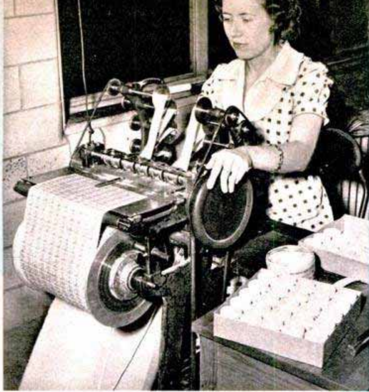
Winding machine cuts the stamp rolls into strips to fit stamp machines. Big single coil has 3000 stamps
