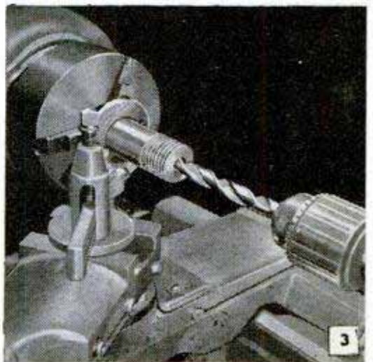
Drilling hole through center post. Drill chuck is held in ram of tailstock center
