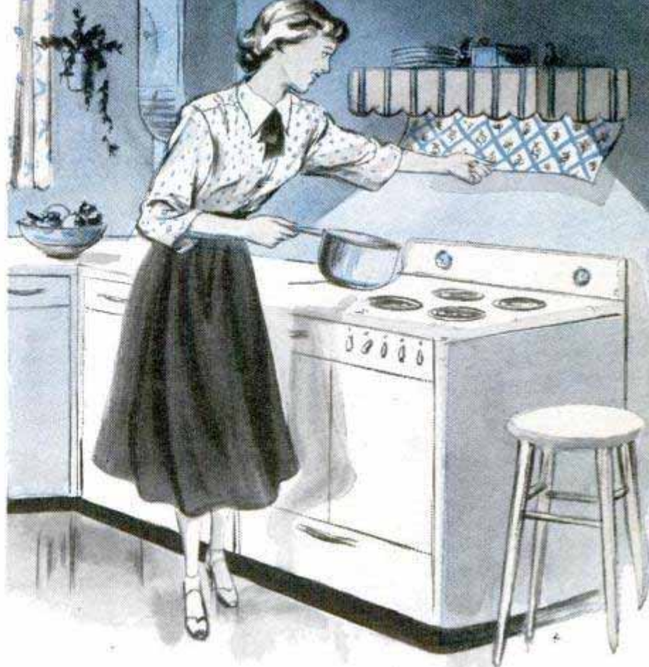
This combination fluorescent light and window-shade backdrop for the range protects the wall from grease spots and provides extra shelf space and additional illumination to make cooking easier
