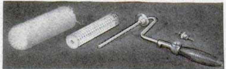
Left, painter doesn't have to stop to dip the roller. Top right, close-up shows the air-and-paint tank. Control valve is on handle of roller which consists of perforated plastic cylinder and sheepskin cover, below
