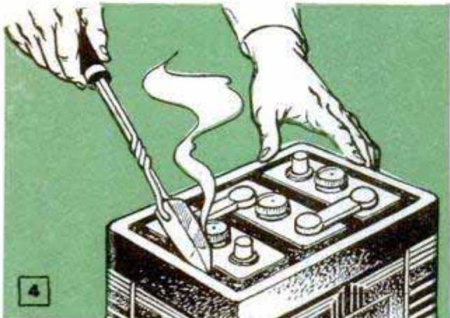
Above, soldering the cell-connector strap after cutting to remove a cell. Below, sealing a repaired cell into the battery case with a hot soldering iron
