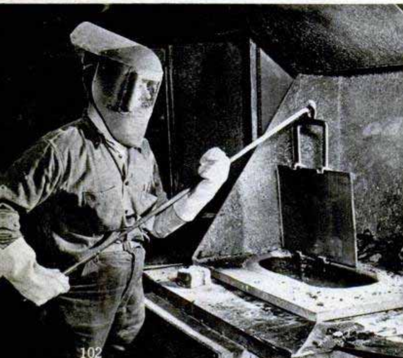
Most stamps are printed on specially designed rotary presses like this one. Below, hardening plate in cyanide bath. Right, reproducing stamp engraving on steel plate which will be bent to fit press Photos by John Drew Atkin
