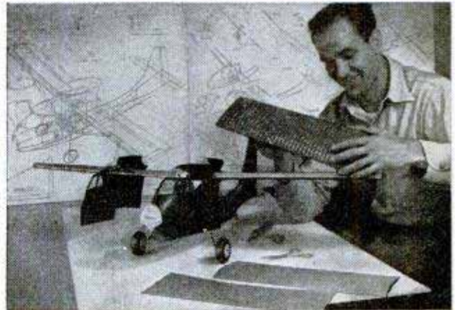
Top, model of Republic Seabee shows the accuracy of detail possible with the molded skin parts. Above, plane assembled by gluing preformed parts to frame
