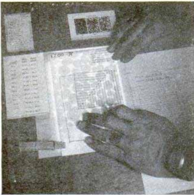
Scale, held against a photomicrograph of fleece that is magnified 500 times, shows quality of wool hairs
