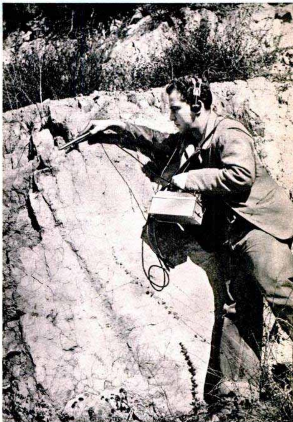
This 20th-century '49er is looking for uranium—not gold. He carries a radiation counter which reveals radioactivity in rock. Here he has lifted counter tube from unit to test ledge
