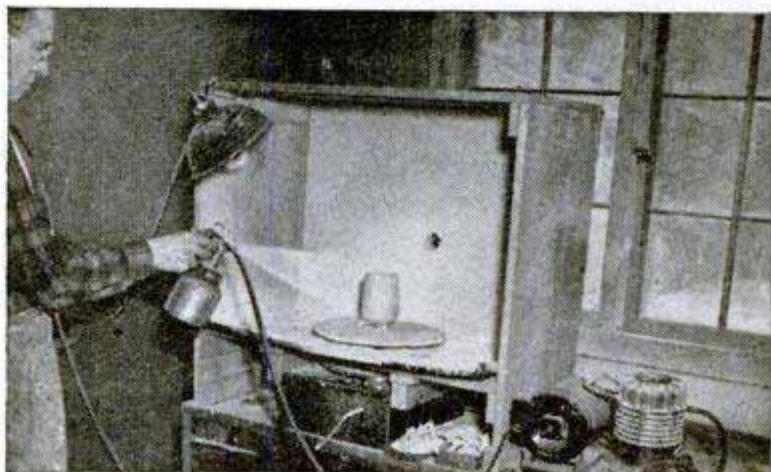
Old phonograph provides turntable in the Maxwells' spray booth where glaze is applied with a spray gun. Below, Joy uses drill press to mix clay body while her parents prepare to fire pieces
