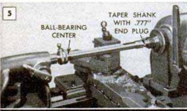
.005 SKIN CUT CLEANS OUTSIDE OF TUBING
