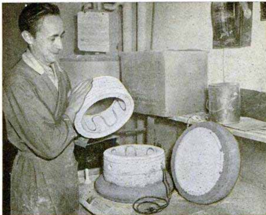
Homemade kiln was shaped in two parts by mixing clay and sawdust in a cheese carton. When it was fired, the sawdust burned out, leaving air spaces in clay. Below, adjustable rests steady hands over potter's wheel
