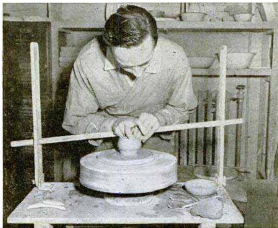
Homemade kiln was shaped in two parts by mixing clay and sawdust in a cheese carton. When it was fired, the sawdust burned out, leaving air spaces in clay. Below, adjustable rests steady hands over potter's wheel
