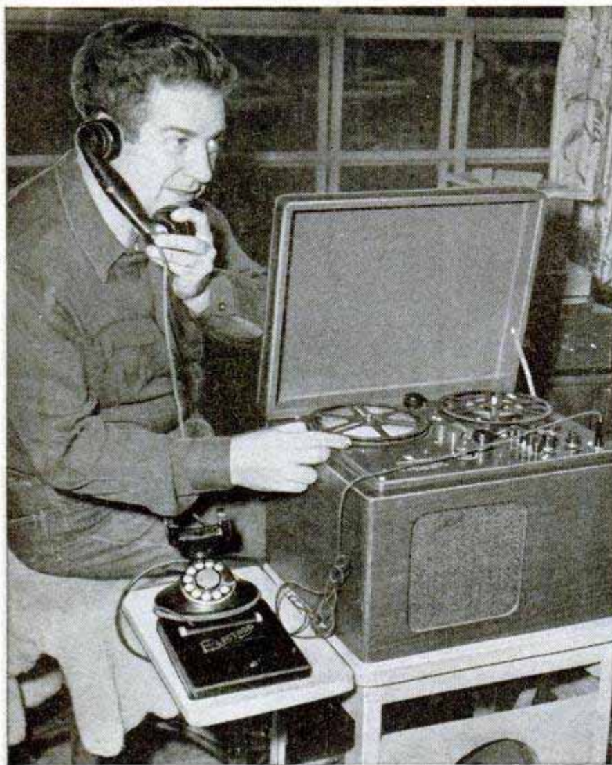
Smiley Burnette, Western film star, records important phone conversations on magnetic tape by placing telephone on top of an induction pad
