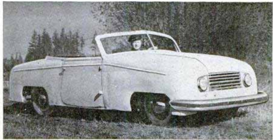
Using parts from a junk yard, inventor Victor Jewel built this car to test his fluid drive. Total cost of parts: $300. Below, no drive shaft is used. Fluid is carried by tubing from pump at motor to transmission
