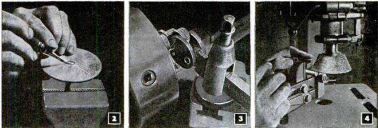
Force fits for small gears and other parts attached to standard shafting are achieved by simply knurling the shaft. The knurl has the effect of increasing the diameter of standard shafting as much as .003 in.
