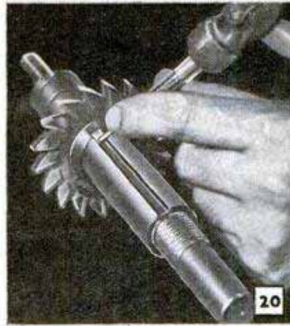
Keyways for both flat and square keys are milled in the shaft. By boring the hub of the wheel oversize and silver-soldering a slotted sleeve in the bore as in Fig. 21, the internal keyway is formed without milling
