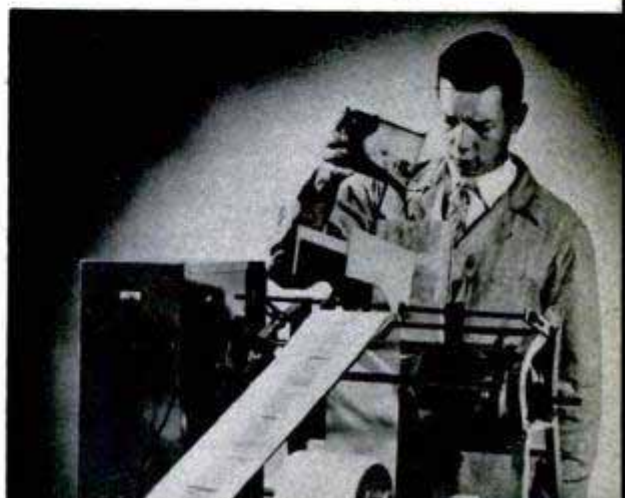
Dry printing press, below, uses no ink. Instead, a powder forms image
