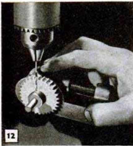
Small gear wheels to be fitted with setscrews are drilled and tapped as in Figs. 12 and 13. When seating a taper pin in the hub of a wheel, use a pin punch and tap it lightly, otherwise the pin may "freeze"
