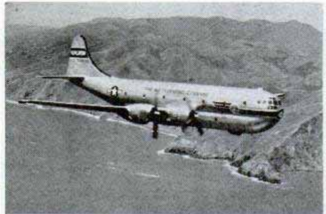
Transport sister ship of the B-29, the Boeing C-97 will move loads of about 40,000 pounds at 300 m.p.h.
