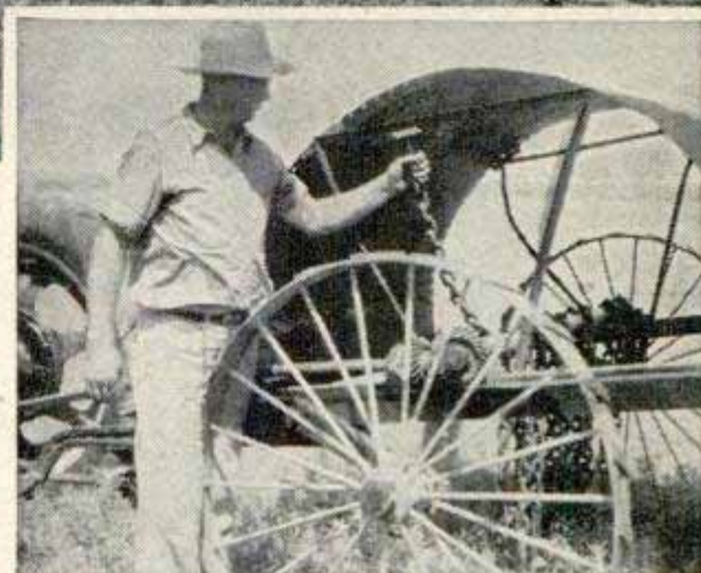
Above, brush beater or "Iron Billy Goat" flails low growths of shrubs with whirling chains. New beater below has shorter chains and shaft with power unit
