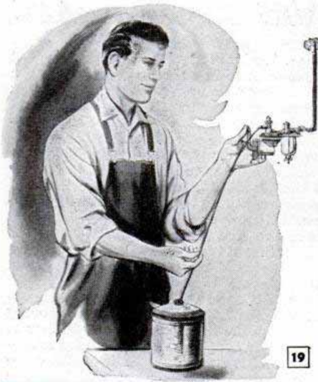
Above, checking screen in choke-control heater. Left, testing fuel pump. It should lift fuel 30 in.
