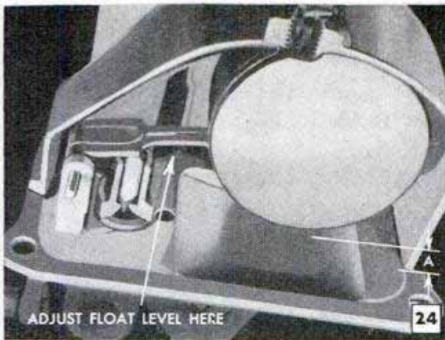
Carburetor-float level, A, is adjusted by bending the float arm. Consult instruction book for dimension
