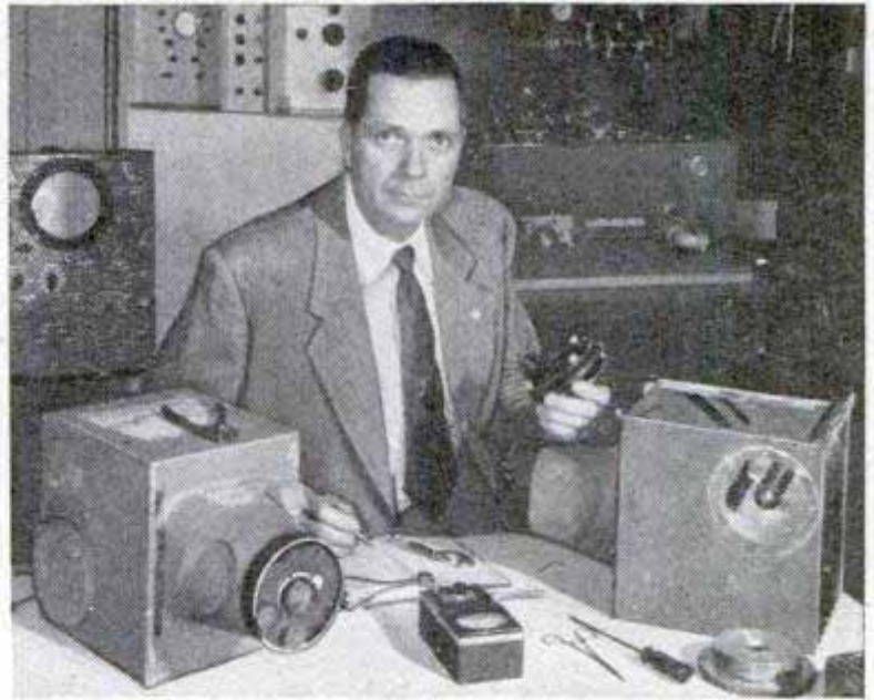
Camera at left was in the V-2, the other in the Aerobee rocket. Neither of the cameras was badly damaged in the desert crash
