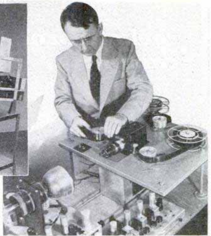
Film reel moves across table in front of scanner. Right, light from cathode-ray tube scans messages
