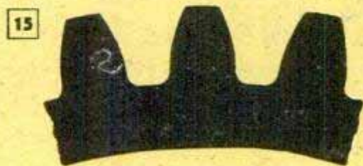
15 5 DIAMETRAL PITCH 0.6283 CIRCULAR PITCH
