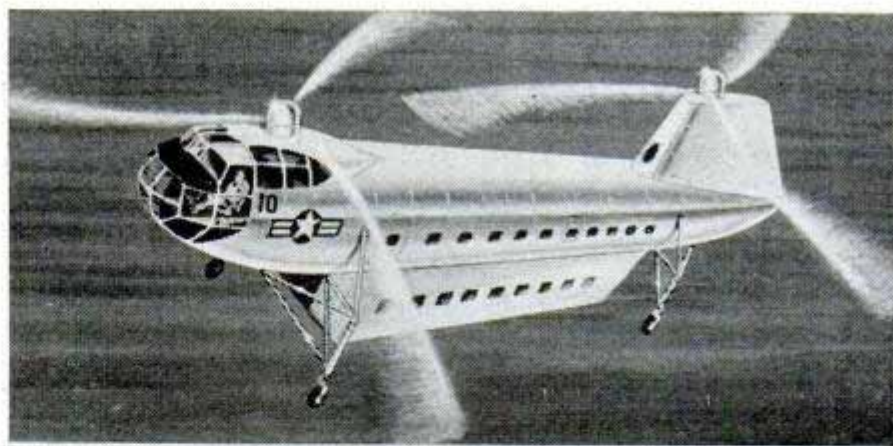
World's largest helicopter, the Piasecki XH-16 will function as a troop or cargo carrier. It will be approximately the size of a Douglas C-54. It features a quickly detachable capsule which about doubles its load
