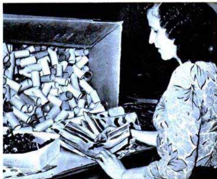
Gaily colored Cellophane is laid over the crimped paper so just the fluted ends are thrust out. Below, core of the cracker is cardboard tube which contains paper hat, plastic toy and "your fortune"
