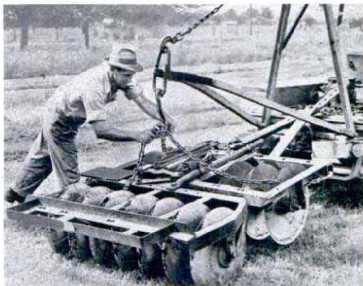
Top, built from an Army weapons carrier, this versatile tractor not only pulls farm implements but lifts them for road travel. Above, A-frame drops disk to the ground ready for use
