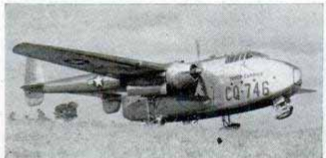
Fairchild C-119 Packets carry 42 troops with gear. Track-type gear permits landings on rough fields
