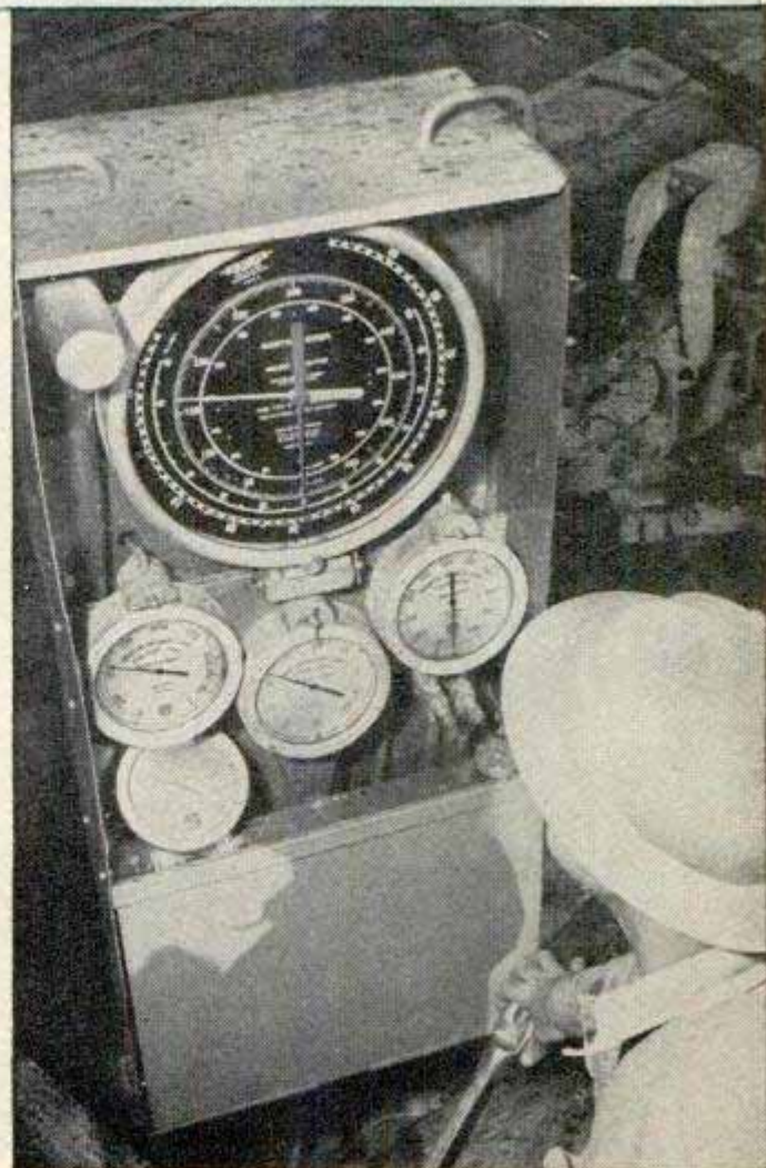
Dial panel tells the driller the weight of pipe, pump pressure, torque and revolutions per minute
