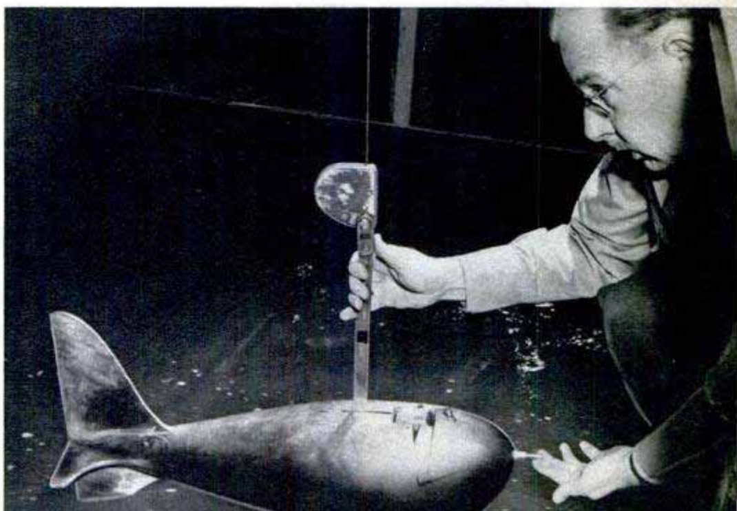
Laboratory, shown at right center, is a hospital for sick dams. Water from the Mississippi flows through maze of channels and back to river. ↓ Torpedolike instrument picks up an exact specimen of sediment. The sample then is used to calculate the amount of sediment in the stream
