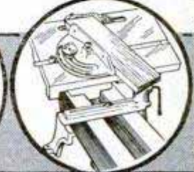
Cutting compound angle
