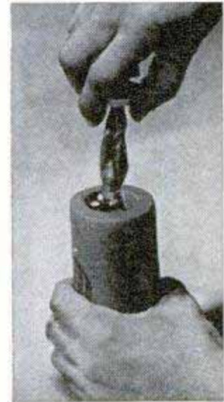
Above left, latex mixed with new material is poured over model, which is easily removed (right) when the latex coagulates. Top, the rubber molds and castings. Center mold made the plastic figures in front of it
