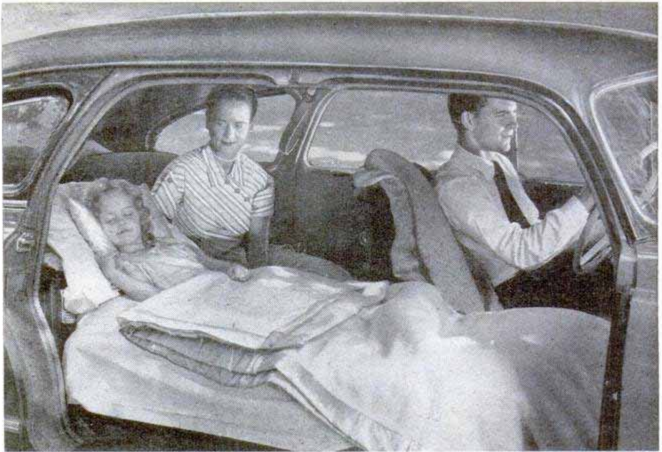
Divided front seat drops back to form single or "twin" bed arrangement without disturbing the luggage space
