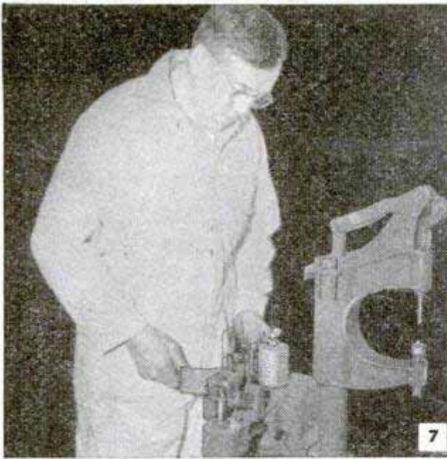
After relining, brake shoes should be ground down to the exact radius of the drum to prevent chatter
