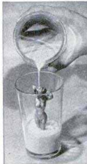
Above left, latex mixed with new material is poured over model, which is easily removed (right) when the latex coagulates. Top, the rubber molds and castings. Center mold made the plastic figures in front of it
