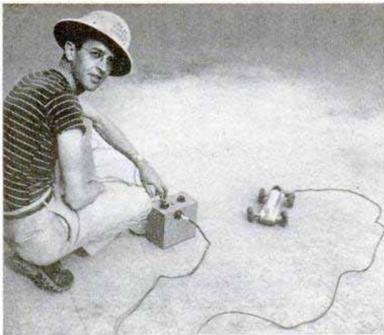
← REMOTE-CONTROL racer can be run forward and backward and steered on the end of a 100-foot wire. A knob on the control box regulates the speed of the model, which will go up to 40 miles an hour. The control operates on less than 30 volts and is said to be safe even for children
