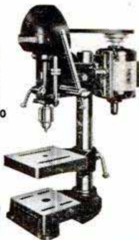
Homecraft Drill Press, No. 11-120 — Four speeds from 700 r.p.m. to 4700 r.p.m. Has capacity up to 1/2" holes in cast iron. Oil-impregnated bronze bearings in quill. Ball-thrust bearing in lower end of spindle. $4395
