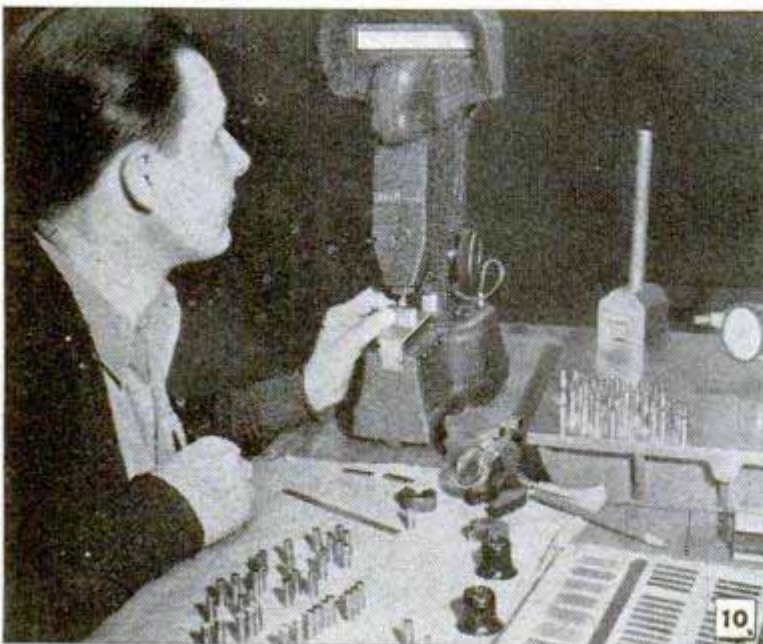
Light-beam comparator indicates size by shining light on dial
