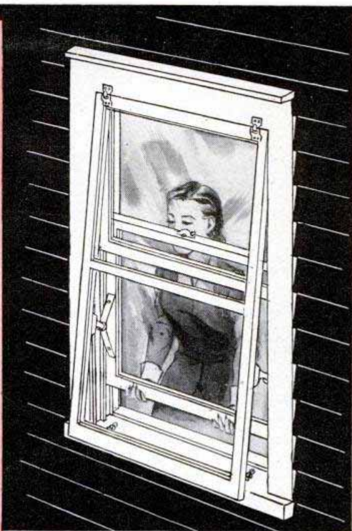
Raising the inner window will open the storm sash to admit fresh air directly into the room. Merely lowering inner sash closes the storm sash tightly
