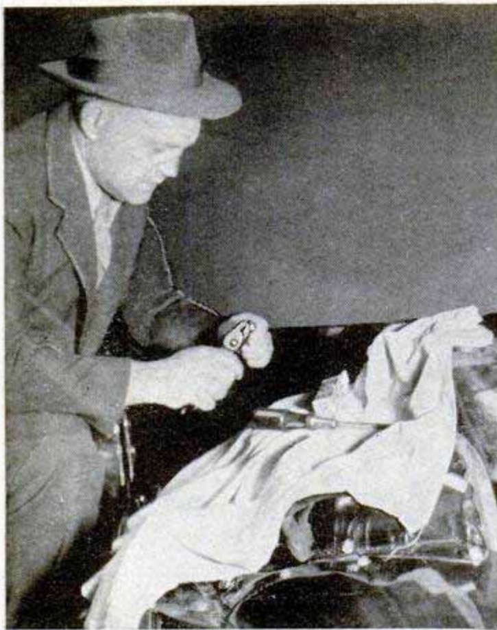
Overlubricating distributor may force grease into breaker mechanism and foul the points
