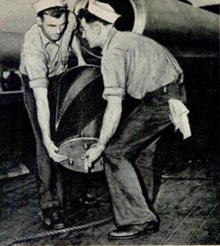
After the big gun has been fired, bluejackets clean the bore with a cylindrical brush pulled by a rope
