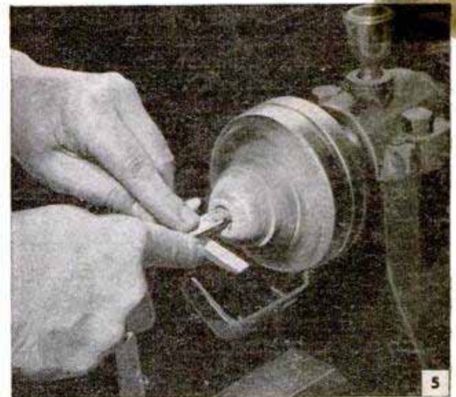
Boring the tobacco hole in the bowl, using a special chuck. Bottom of the hole is rounded uniformly.
