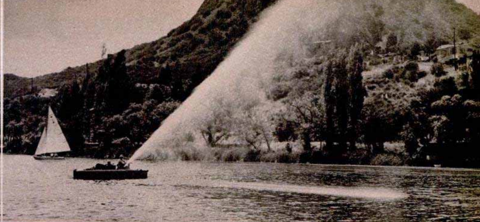
Where's the fire? Pumping unit can shoot a heavy stream of water 100 yards or more and carries ample hose
