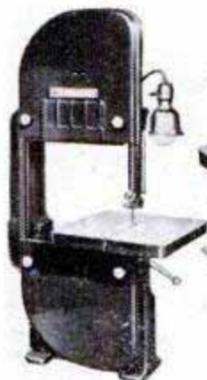
Homecraft Band Saw, No. 28-110 — Has 6 1/2" capacity under guide and throat capacity of 9 1/2". Fully-adjustable blade guides. Table tilts 45°. $3995 Lamp Extra
