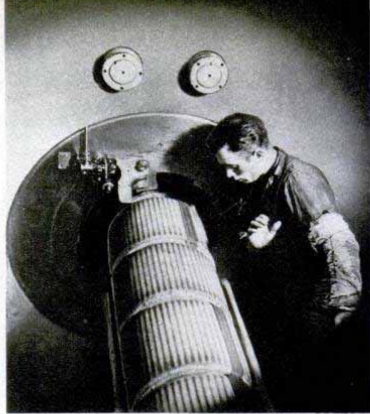
Automatic ramrod shoves bags containing 60 pounds of smokeless powder into breech of "big mouthpiece"
