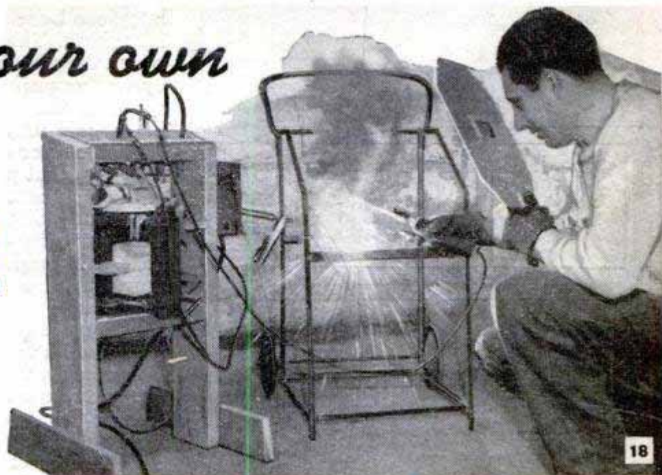
The welder parts are wired temporarily and used to weld the cabinet frame
