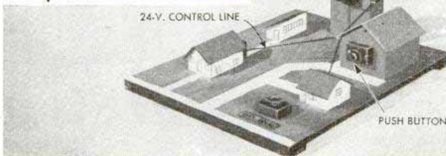
Any number of remote switches for the yard light can be used in the 24-volt control circuit shown in above model. Insert shows wiring diagram
