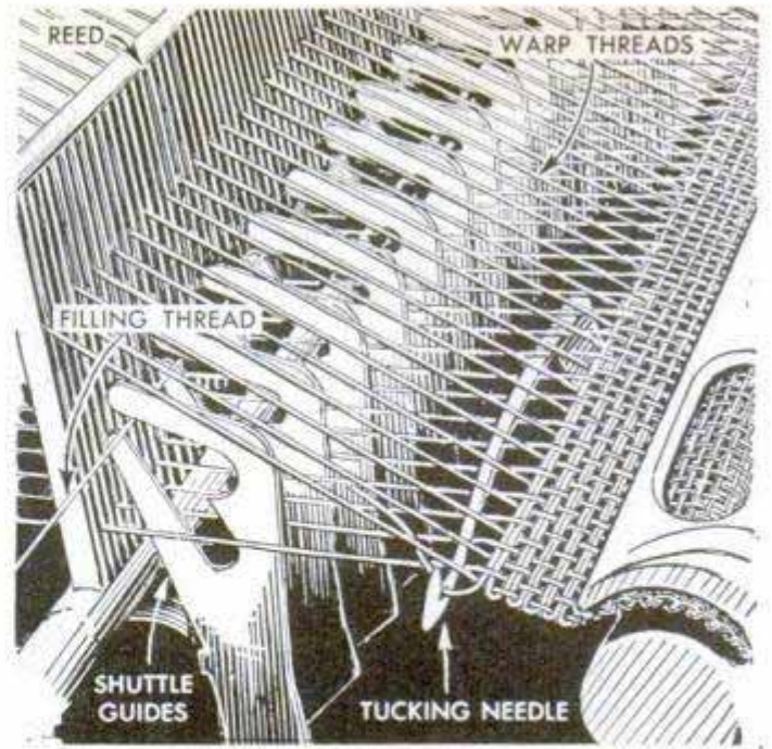
Left, shuttle (arrow) starts across loom between warp threads. Right, close-up shows tucking-needle action
