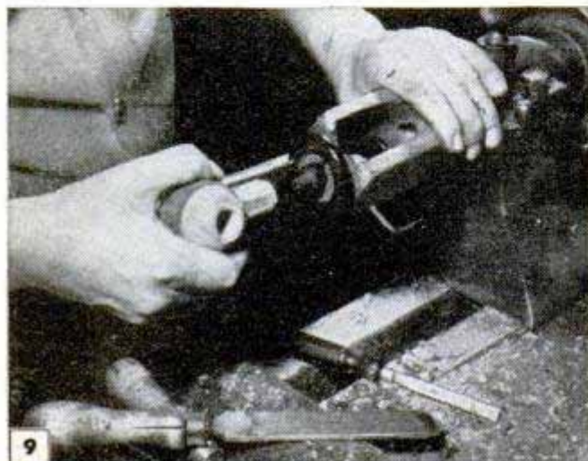
The stem is held in the same chuck when turning the tenon. Always trial-check the fit in the pipe shank
