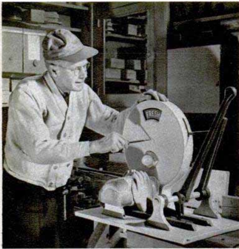
Fresh-bread tester makes squeezing unnecessary. Day-old bread gets amber light; soft bread "Fresh"
