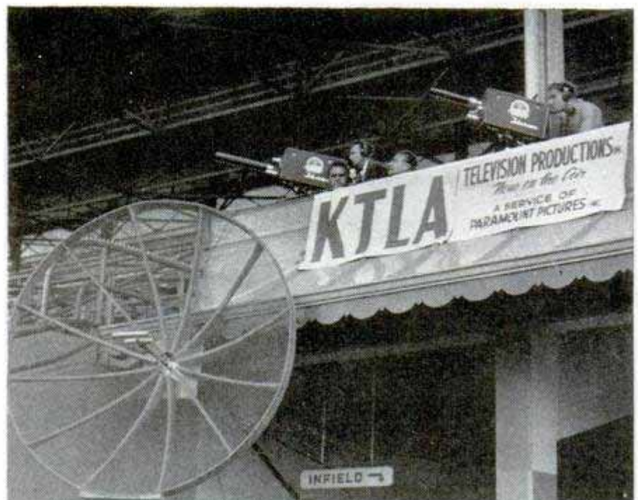
Line-of-sight "dish" antenna at baseball park beams pictures to main transmitter on mountain
