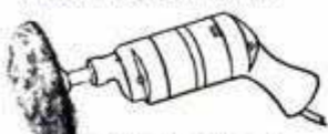
with the slip-on lamb's wool bonnet, it is a portable power-driven polisher or buffer.
