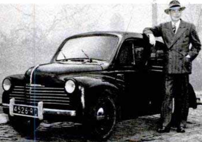
French Renault (above and below) has four-cylinder engine in rear; carries four persons, and costs $1264
