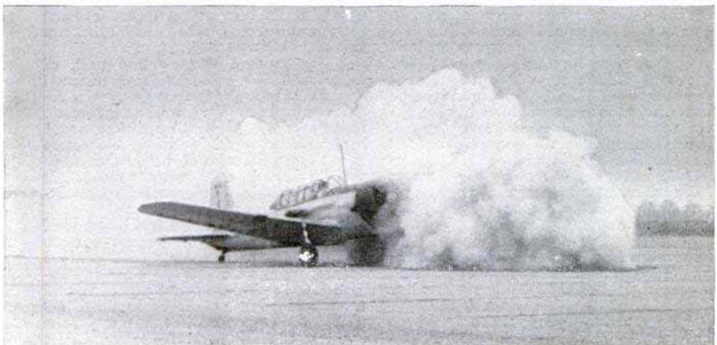
BRAKES: Used as brake for aircraft landing, rockets alone stop a BT-13 traveling 85 miles an hour in 112 feet
