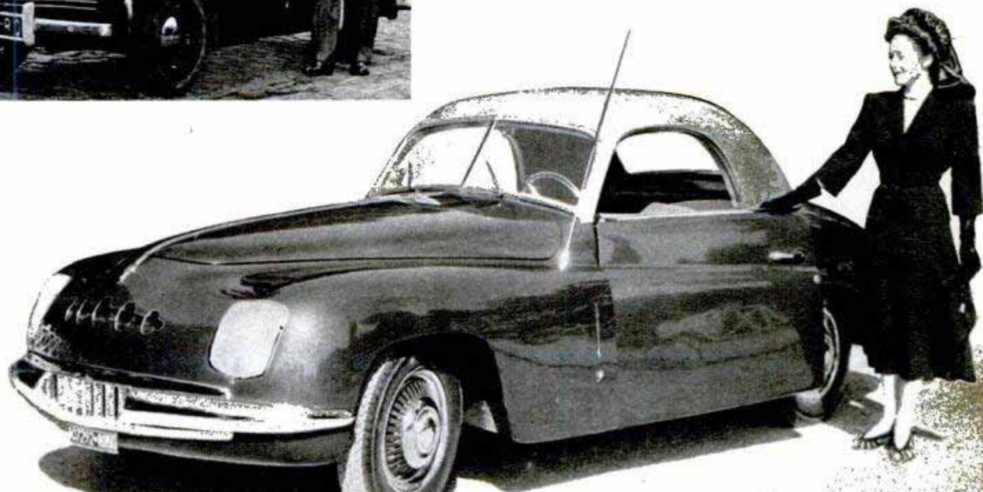
Italian-built Fiat (below) is said to run 26 miles on a gallon of gasoline. Top speed is 81 m.p.h. and the price is $3833. Note absence of chrome on body
