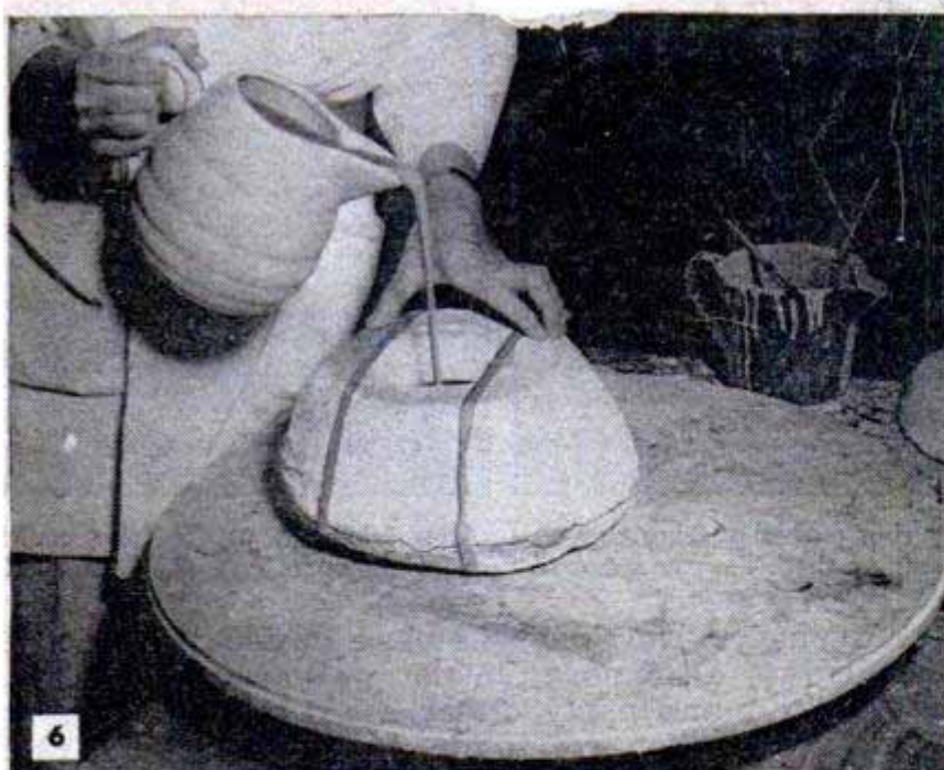
Left, mold is assembled and slip is poured in. Above, after bisque firing and coloring, piece is dipped in glaze
