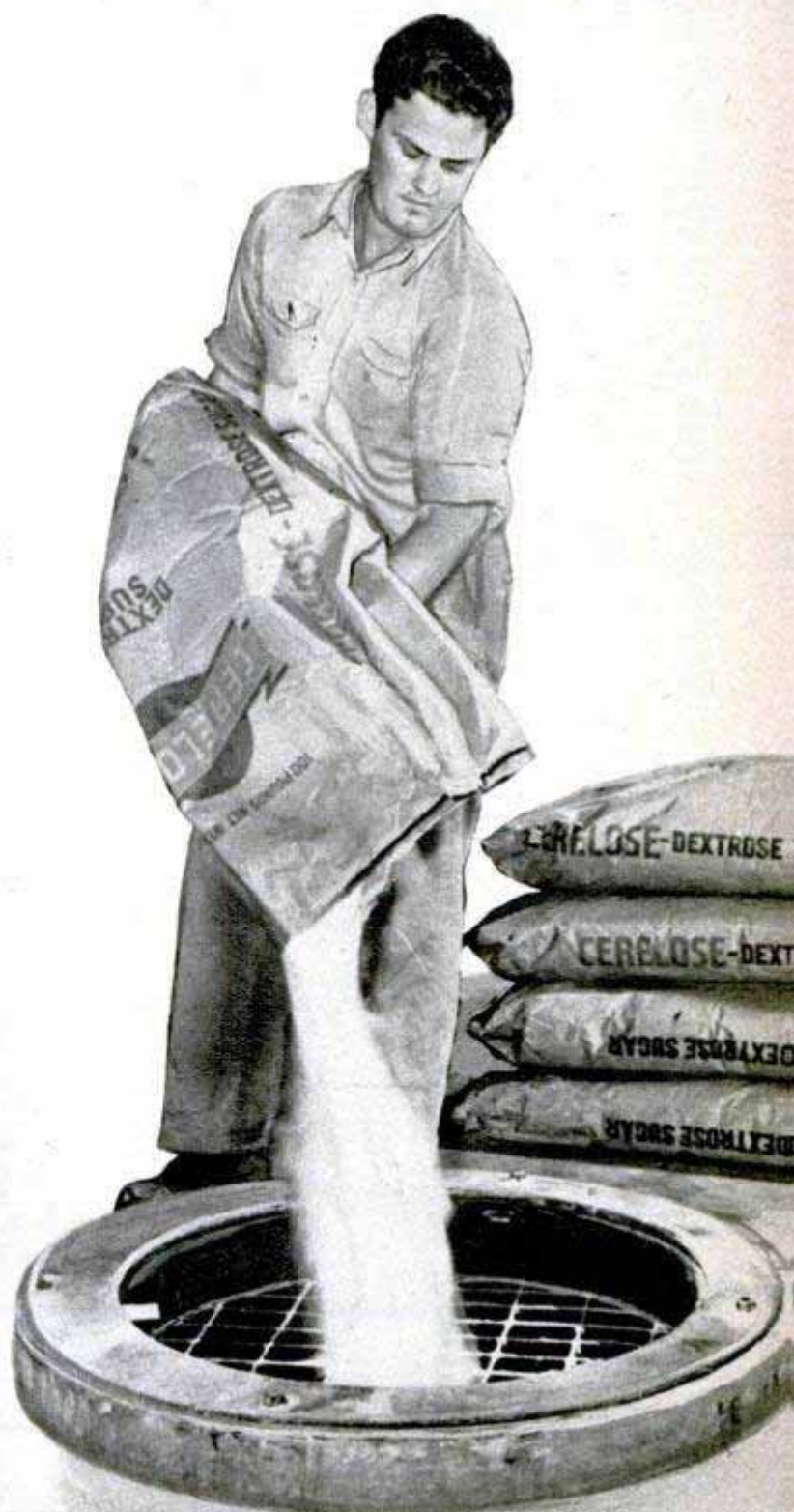
Above, ingredients for each batch are metered out precisely. Right, sugar is an important ingredient in the speed-up process. Worker pours sackful into dissolving tank. One pound of sugar is used to each 20 pounds of rubber. Below, part of the synthetic rubber plant operated by U. S. Rubber Co. in Borger, Tex. The recovery columns can be seen at the right
