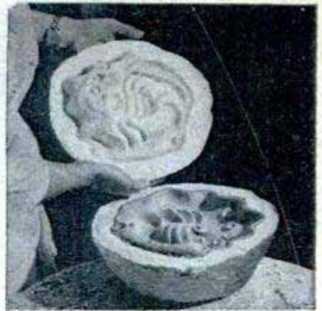
After trimming at the joint, mold is pried open and shell removed
