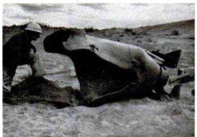
Split wide open, shell of quarter-inch steel plate was hurled 500 feet by the force of the explosion
