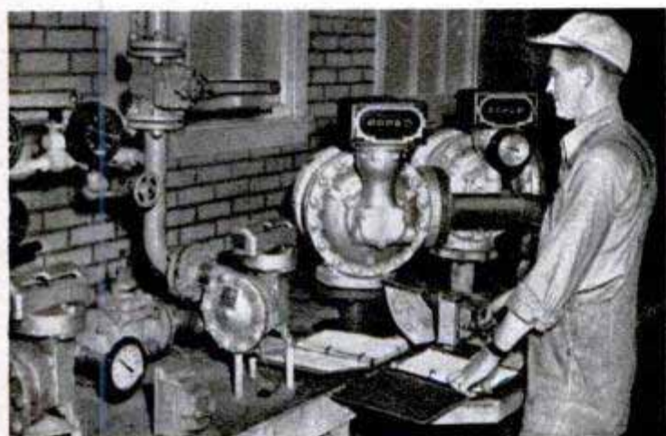
Above, ingredients for each batch are metered out precisely. Right, sugar is an important ingredient in the speed-up process. Worker pours sackful into dissolving tank. One pound of sugar is used to each 20 pounds of rubber. Below, part of the synthetic rubber plant operated by U. S. Rubber Co. in Borger, Tex. The recovery columns can be seen at the right
