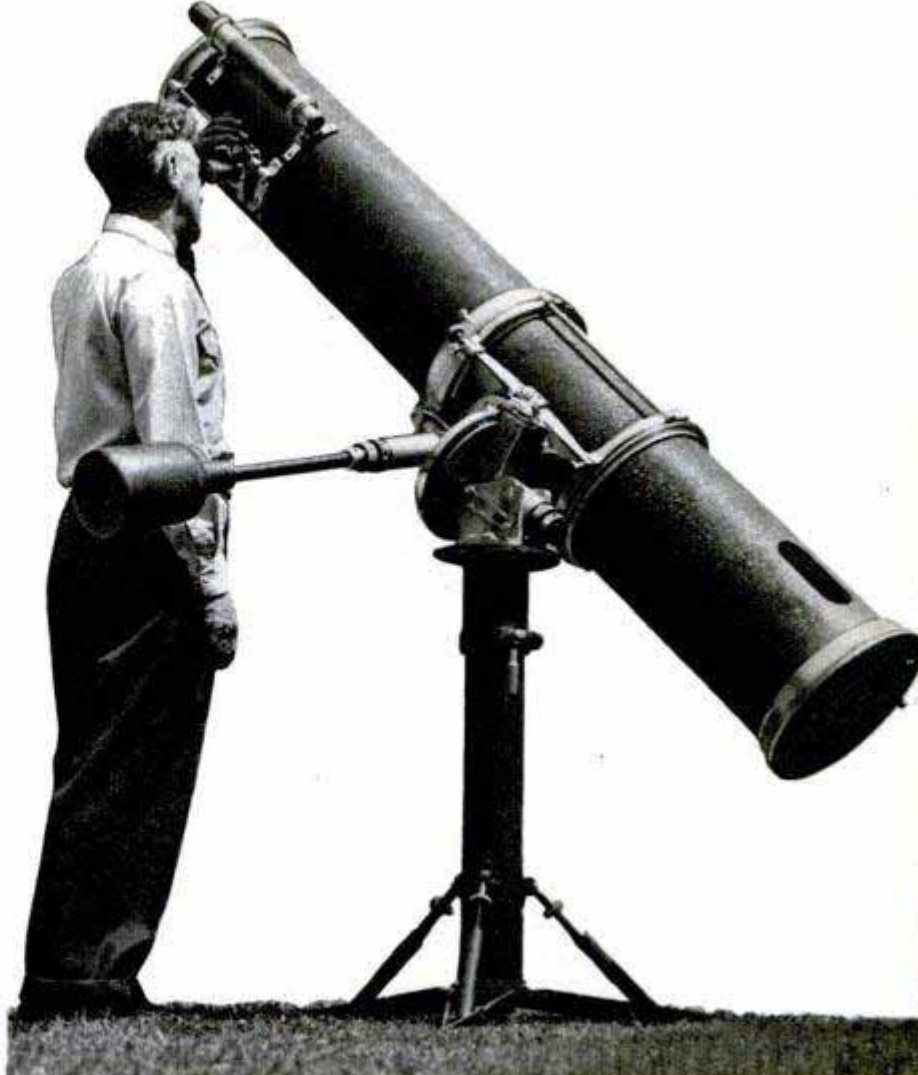
Above, this amateur astronomer tests his 10-inch reflector telescope. Below, view inside a 10-inch reflector telescope shows reflection of mirror in base of tube. Black object in tube holds prism that directs light to eyepiece on the side
