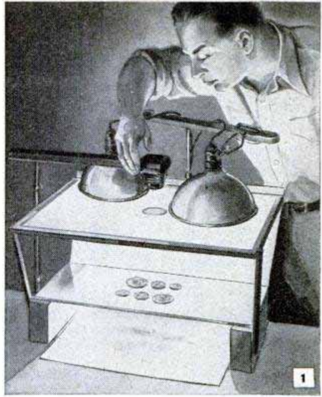
By directing two photofloods through white tracing paper a diffused light is obtained to eliminate glare and shadows. Third lamp lights background for coins
