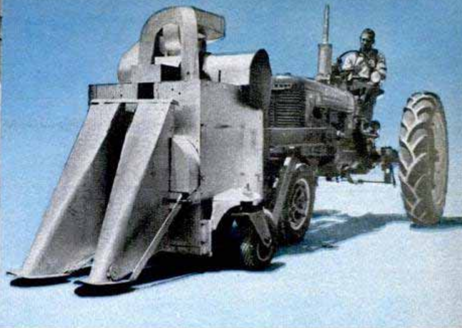
Dry cotton picker shown at right has barbed picks that rotate and move back and forth to pick up the cotton
