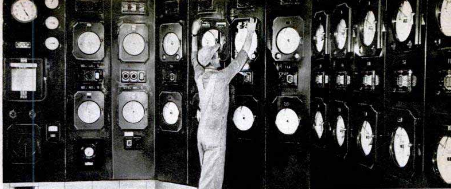
Cooking a batch of synthetic rubber is more complex than baking a cake! Worker sets one of the instruments that record the cooking action for each batch
