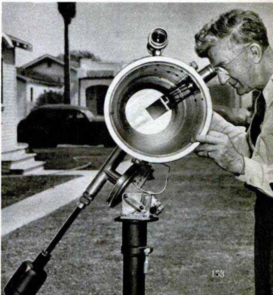
Above, this amateur astronomer tests his 10-inch reflector telescope. Below, view inside a 10-inch reflector telescope shows reflection of mirror in base of tube. Black object in tube holds prism that directs light to eyepiece on the side
