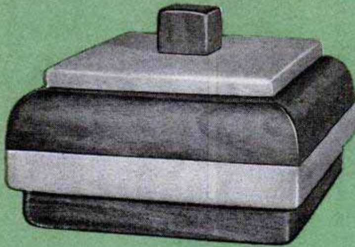
This box is built up of six parts cut square from contrasting woods and stacked alternately in order shown
