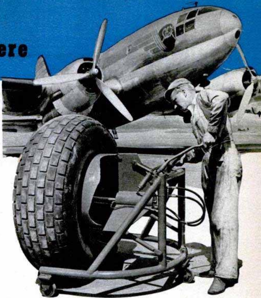
Airplane mechanic submitted an idea for a tire-change tool. Result is this hydraulic machine that removes the tire in quick time
