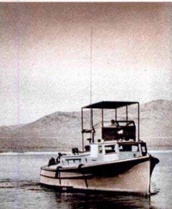
Sounding boat used in silt survey carries sensitive fathometer and when reading is made sailors (right) take bearings on two shore markers to determine their exact location on lake. The Navy is cooperating in survey
