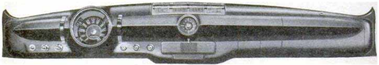
Instruments are grouped directly in front of driver, and "black lighted".
