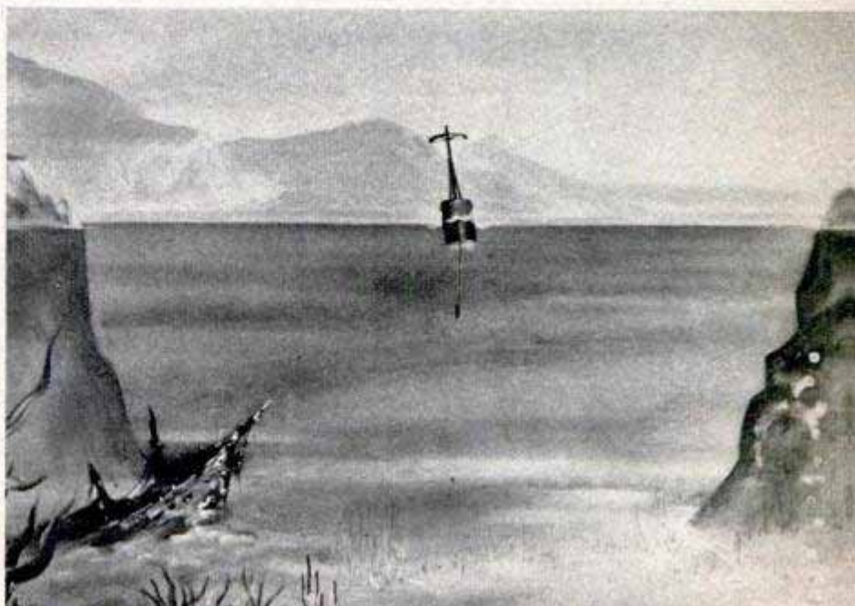
Rescue buoy (A) rises to surface if sub is sunk. It contains telephone connected to the submarine in trouble. Buoy has colored reflectors. Below, sono-buoy guarding harbor uses underwater sonar to pick up the sound of approaching sub
