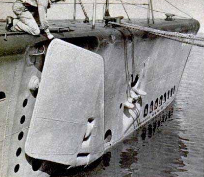
Bowplane (left) is carefully checked before start of the cruise. Right, closing exhaust valves of engines
