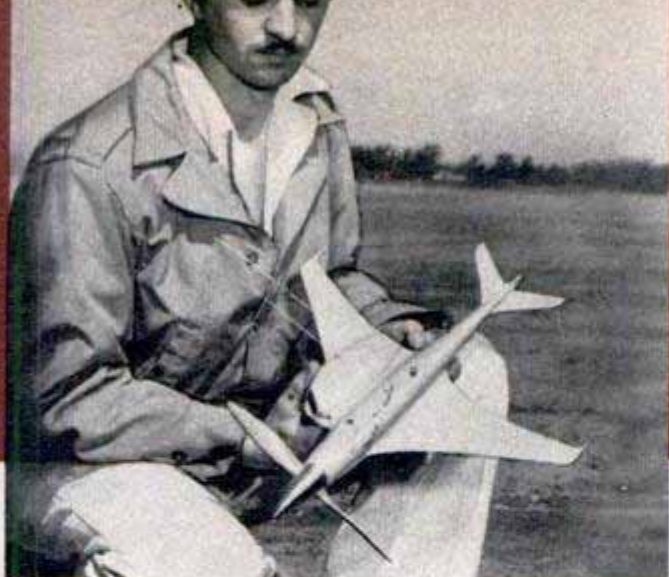
Mad Missile is what Joe Havlik, of San Diego, calls this "supersonic" Class-D racer. The engine is mounted in right wing; plane has a V-tail and no rudder
