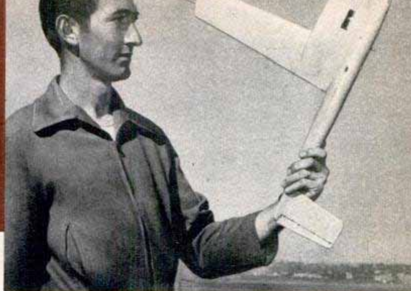
Novel one-wing half-tail "side winder" built by Glenn F. Crist of Modesta, Calif., has been officially clocked at speed of better than 150 m.p.h.
