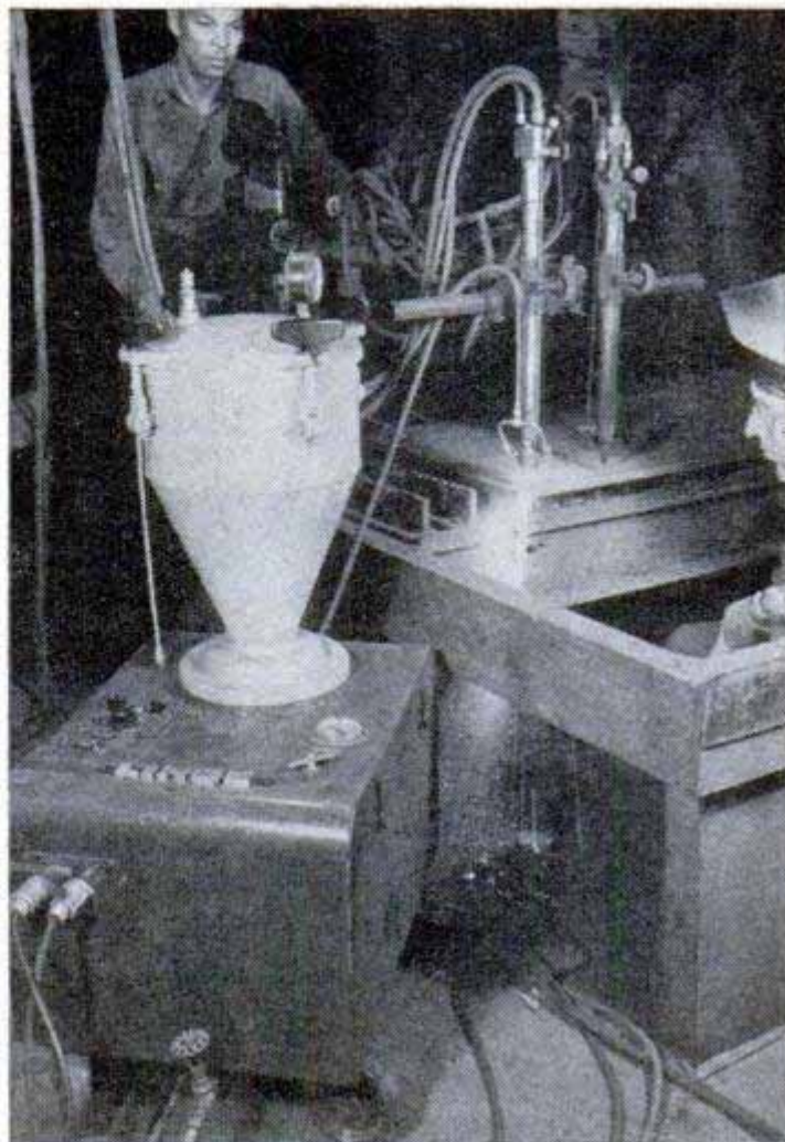
Left, hand-operated powder torch cuts stainless steel in foundry. The hilt on torch protects worker against intense heat. Right, machine cutting torch with the powder dispenser (foreground) connected to it by hoses
