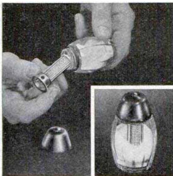
NONCLOGGING SHAKER assures free-pouring salt in damp weather. A chemical vial in shaker absorbs all moisture. When saturated, chemical turns pink and can be dried in oven
