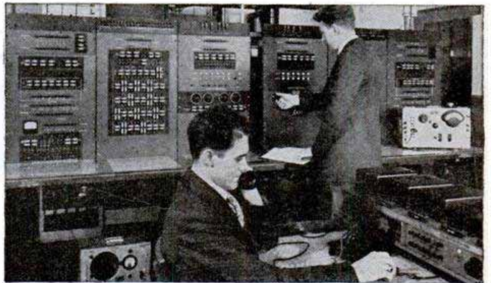
The engineer in the foreground talks over the test circuits which the other engineer sets up on a "circuit simulator."
