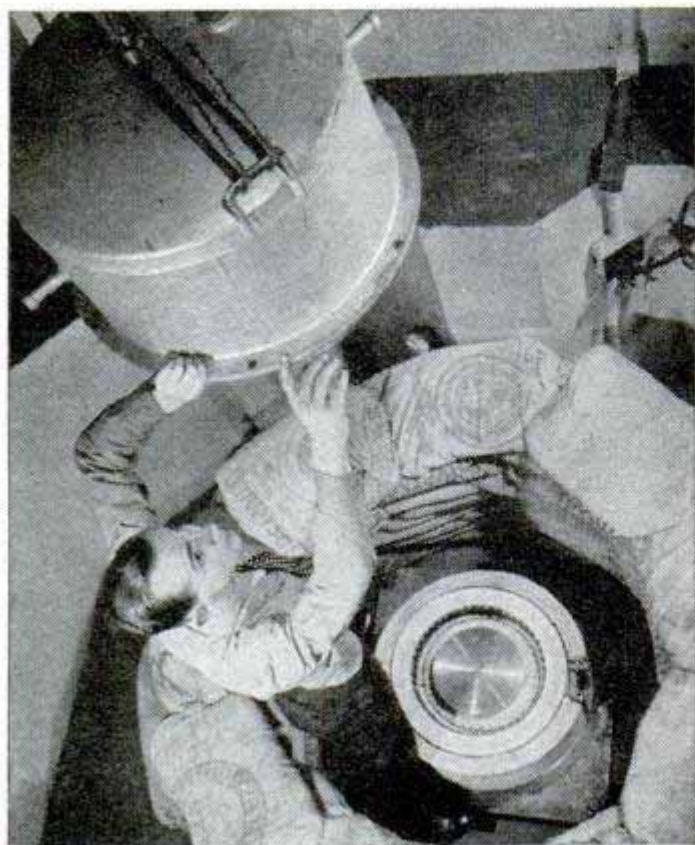
"Bombproof" dugout is used to test jet-engine disks at high speeds and a heat of 1400 degrees Fahrenheit. Below right, an ingot of new magnetic alloy (Hiperco) is poured by scientist
