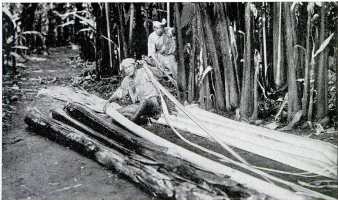
Finest Manila rope is made from abaca fiber, stripped from the inside of a fruitless banana plant grown in the Philippines. The supply of rope became critical during the war when no fiber was shipped from the islands
