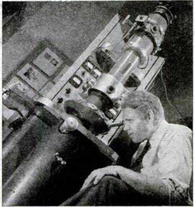
Left, electronic portrait of skin formed on nickel at 900 F. was made by the electron microscope at right
