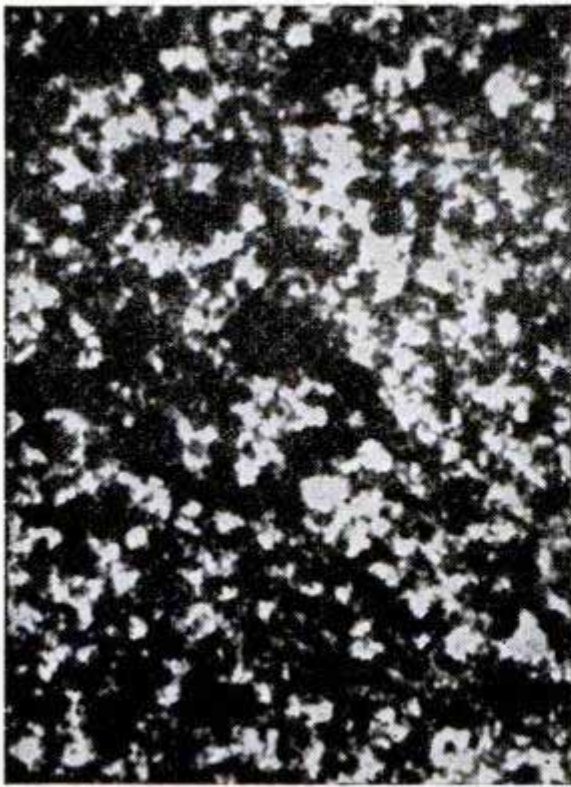
Left, electronic portrait of skin formed on nickel at 900 F. was made by the electron microscope at right
