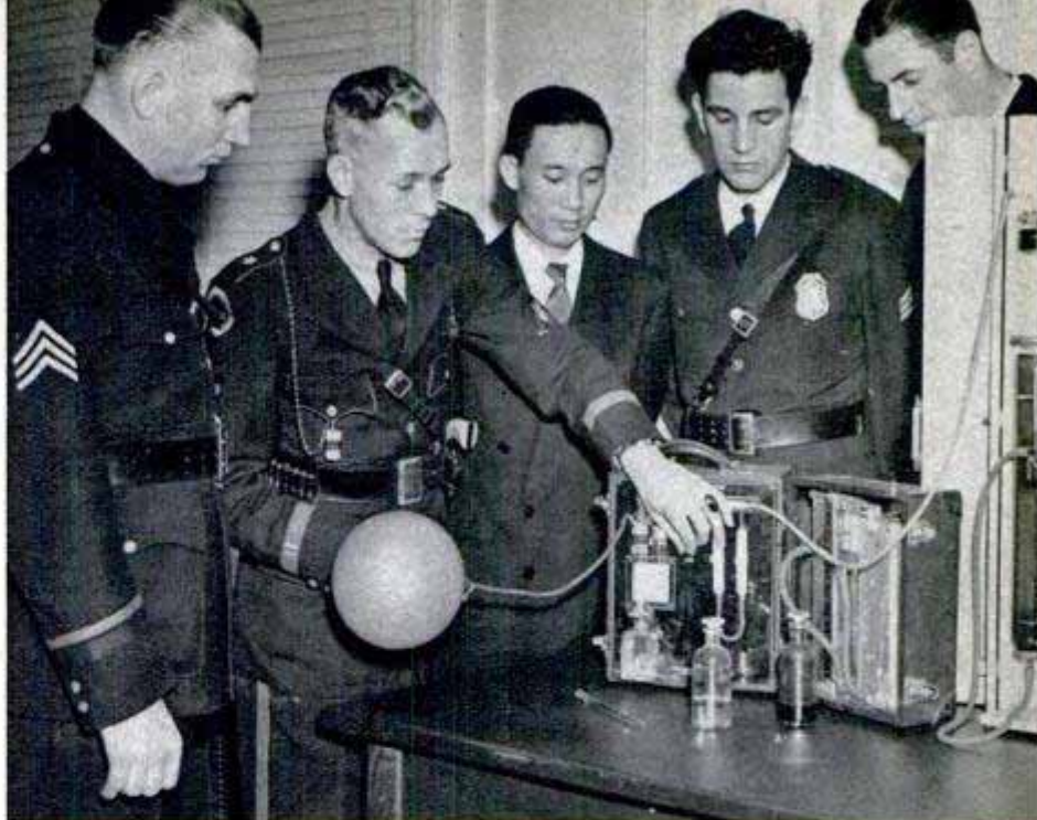
Student cops learn to use the "drunk-o-meter," an instrument that puts suspect's breath from balloon through chemical tests
