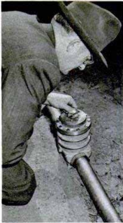
Left, setting the pointer to desired time of flow. Center, cutaway shows piston that is forced down to shut off water. Right, one or more of several faucets can be controlled by timer with this T-shaped arrangement
