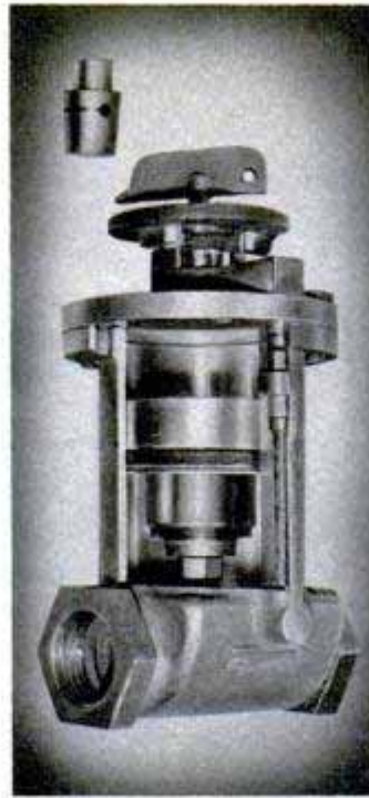
Left, setting the pointer to desired time of flow. Center, cutaway shows piston that is forced down to shut off water. Right, one or more of several faucets can be controlled by timer with this T-shaped arrangement
