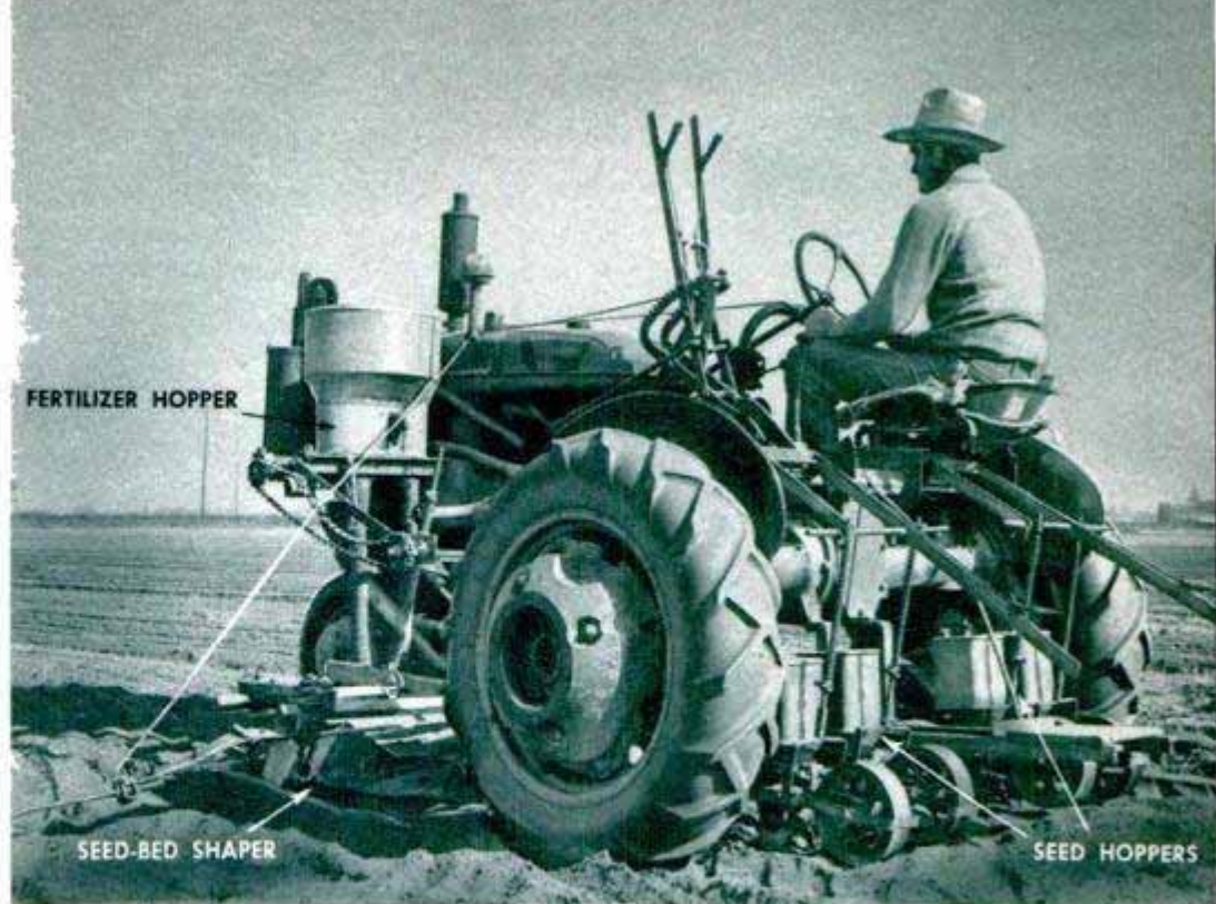
Combination planter built of several machines speeds work by laying four rows of fertilizer, shaping seed beds and planting them in one operation
