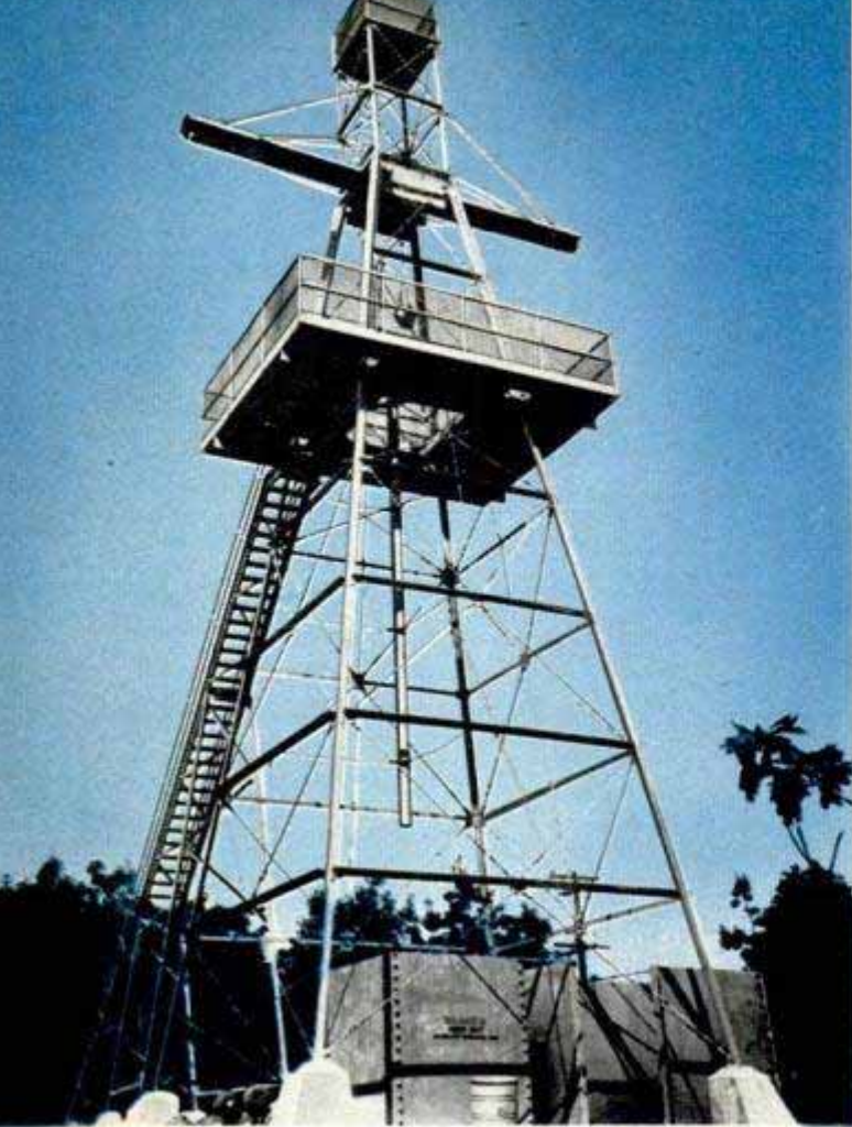
Fuses under test are put in dud bombs and projectiles weighing up to 1000 pounds and dropped on sand or armor plate from 75-foot tower at left. Right, machine shop where pilot models of new weapons are developed
