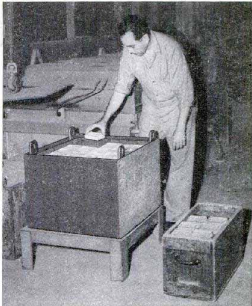
Removed from the molds, the optical-glass blanks are packed in big metal boxes and placed in furnaces for a critical annealing process
