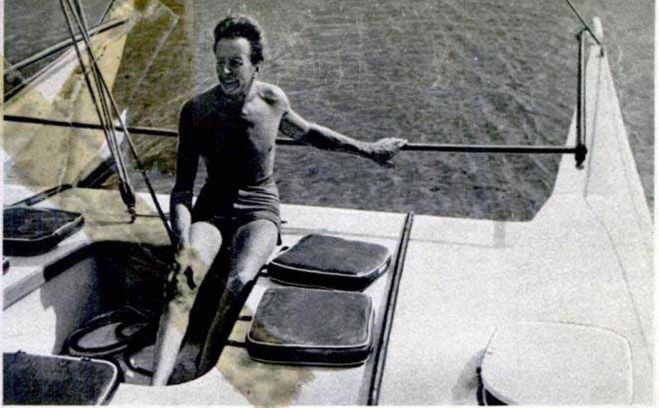
One man easily handles the 40-foot catamaran. Lines from both jib and mainsail run into the small cockpit
