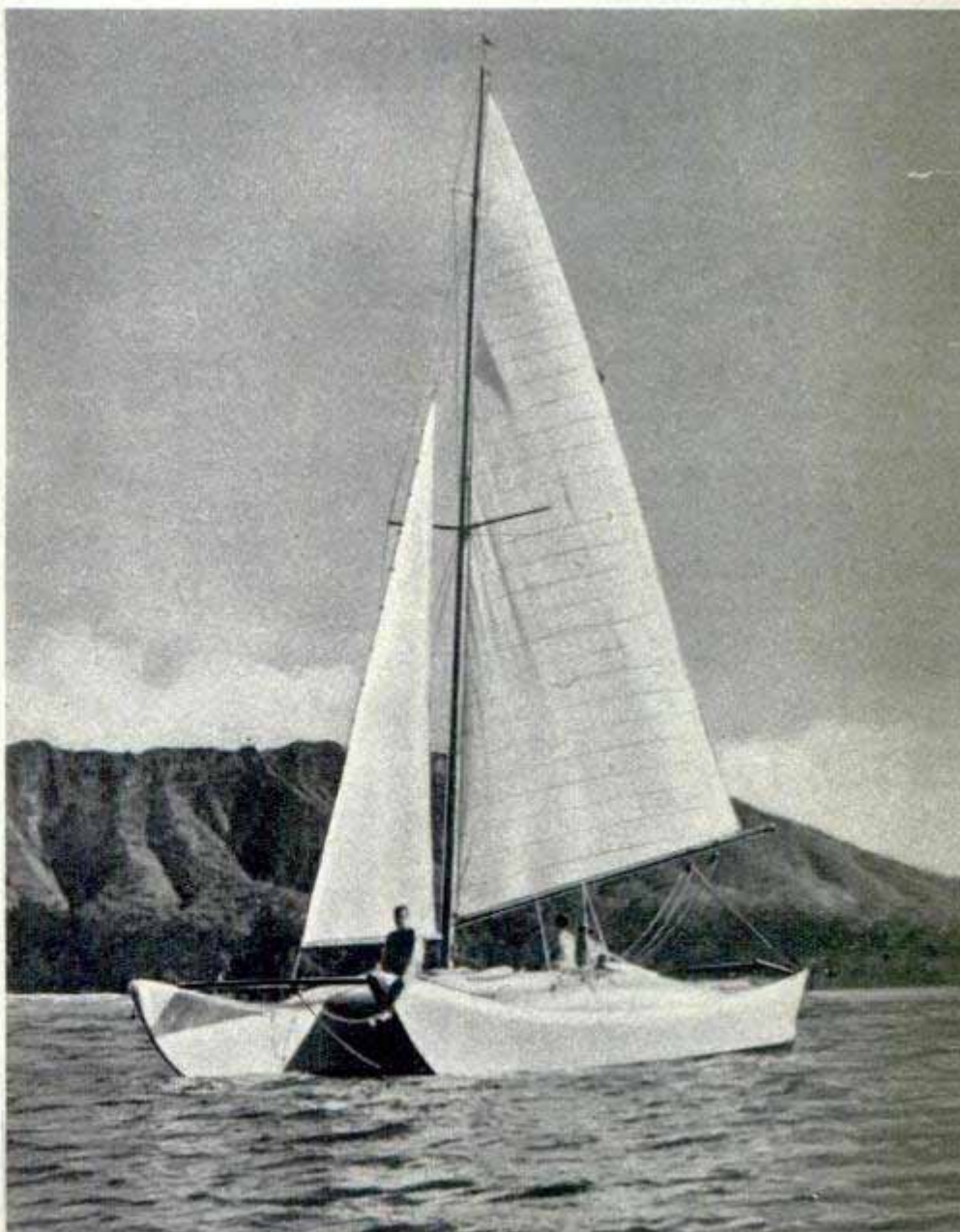
Six can be slept comfortably in the craft. Four are put in the wing section, which is entered by the hatches on deck, and there is space for one in each of the after hulls. Below, the Manu Kai carries only 370 square feet of sail, which is considerably less than half of that carried by one of the fastest catamarans developed in the early '30s
