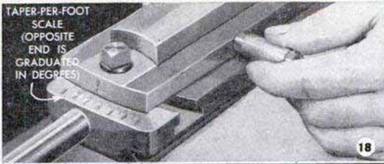
SETTING TAPER ATTACHMENT FOR 1" PER FOOT TAPER
