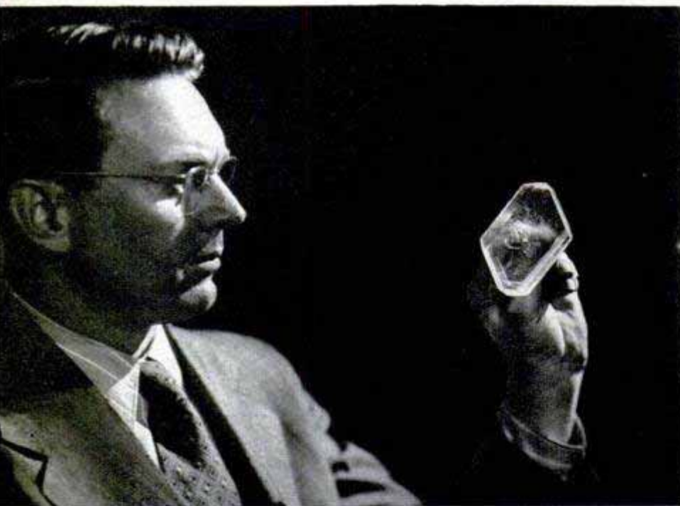
This 340-gram lithium-sulphate crystal, used in underwater weapons, was grown in 23 days. Below, a wind-tunnel nozzle with mirrors used to photograph air flow around supersonic projectiles
