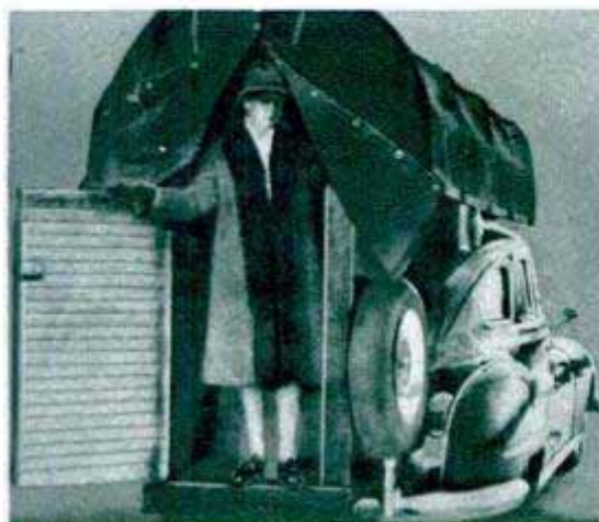
Left, 6½-ft. dressing compartment extends into the car trunk. Right, the three-foot-high sleeper is collapsible
