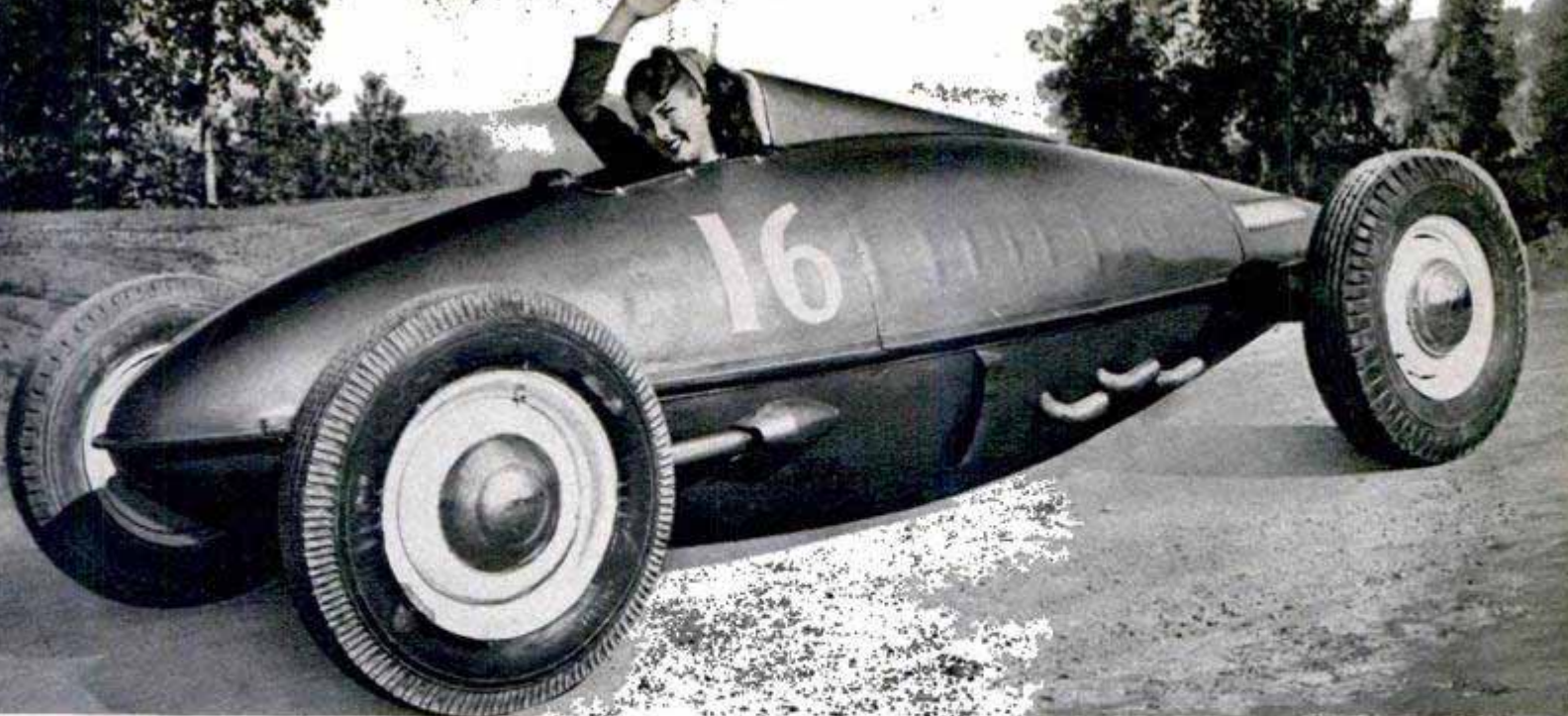
Above, an airplane belly tank mounted on Ford frame, this streamlined "hot rod" has topped 139 miles an hour
