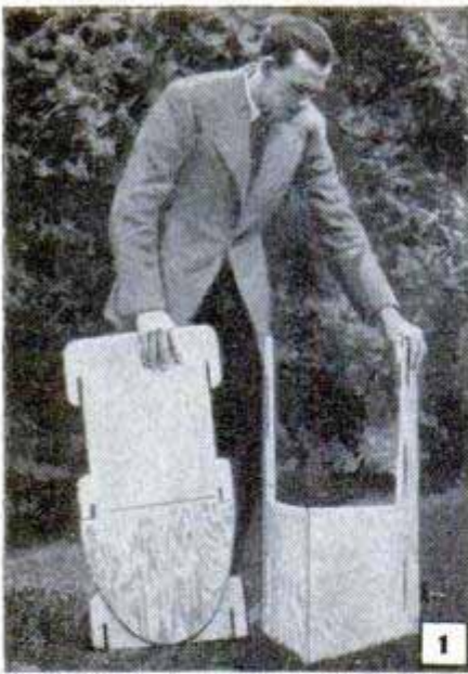
The chair goes together in a jiffy. Just open up the sides, raise the seat, insert the back in the slots and push down to interlock the parts
