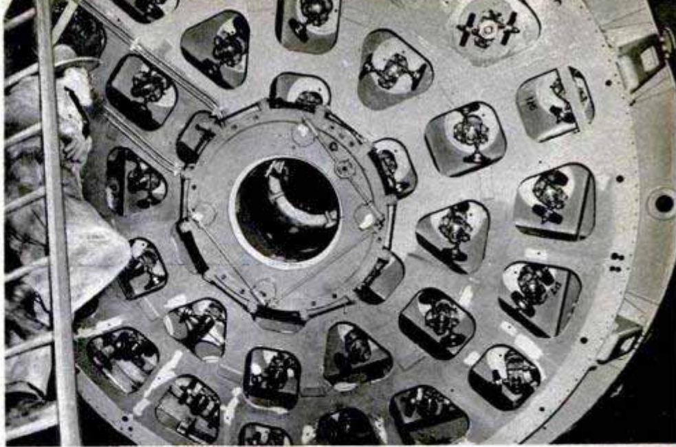
Complex system of counterbalances under the 200-inch mirror keeps the surface from distorting as the mirror is shifted
