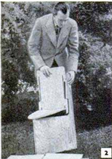
The chair goes together in a jiffy. Just open up the sides, raise the seat, insert the back in the slots and push down to interlock the parts
