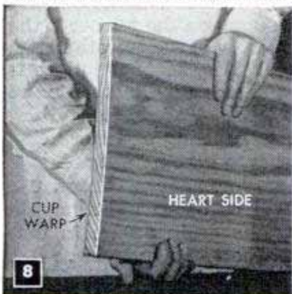
A TYPICAL FLAT-CUT BOARD — NOTE CUP WARP AWAY FROM HEART SIDE
