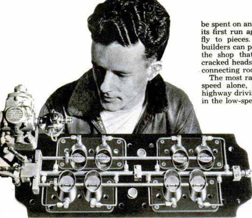
Young designer holds a fuel-injection system that replaces usual carburetor. Fuel metering changes automatically as butterfly valves open and close
