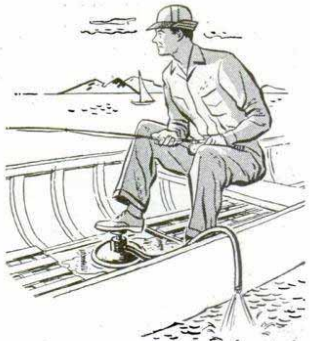
BILGE PUMP is also powered by foot. Its pumping rate is about 3\frac{1}{2} gallons of water per minute
