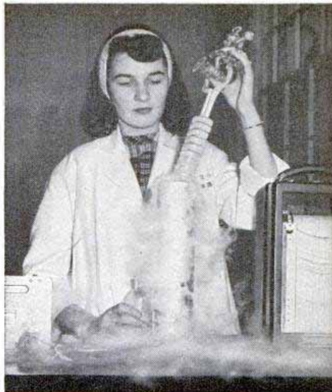
Used in plant experiments, radioactive carbon dioxide is trapped in spiral glass tube by plunging it into a beaker of liquid nitrogen where it freezes
