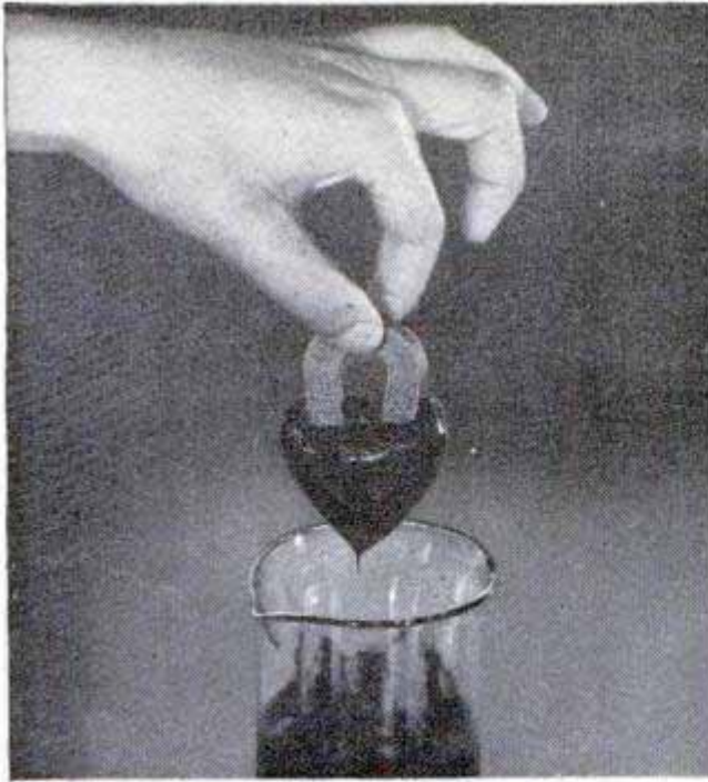
Fluid mixture of fine iron powder and oil such as used in new clutch "solidifies" in magnetic field
