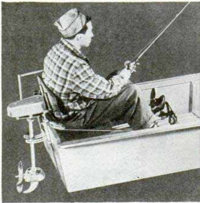
LEG POWER spins the propeller of this motorless boat by pedal action. Being silent, it's ideal for trolling
