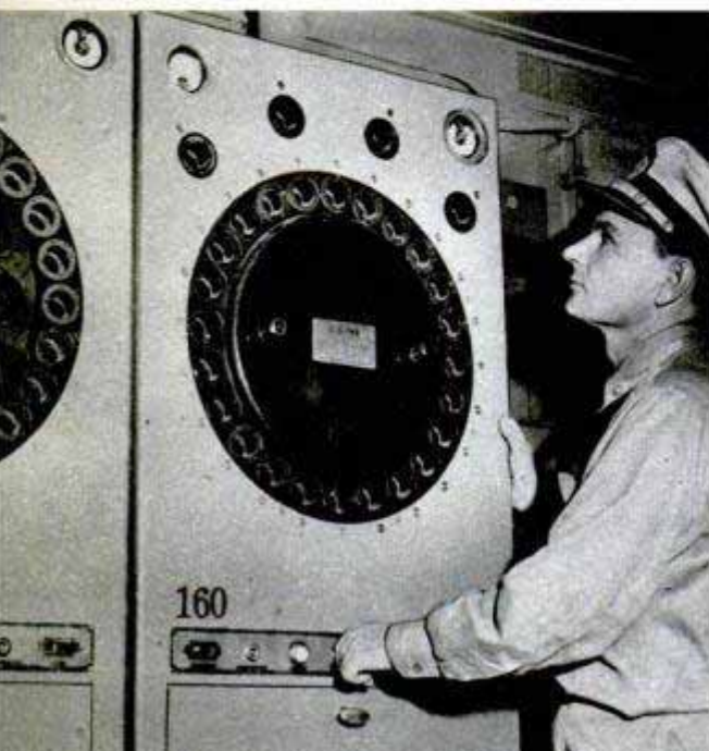
Left, 48 electric eyes examine air throughout the ship. If smoke is present, a light flashes on this board. Right, master indicator board operates 38 steel doors that divide the ship into 14 watertight compartments
