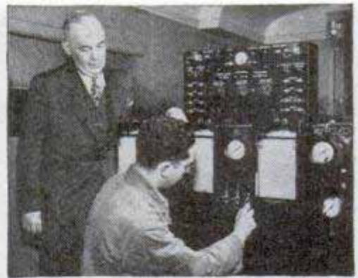
← Classroom's forward panel reproduces action of brakes. Above, instrument records all essential information about train. Below, instructor explains brakes
