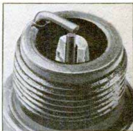
Insulator broken at the lower end may be due to hot operating conditions or careless installation
