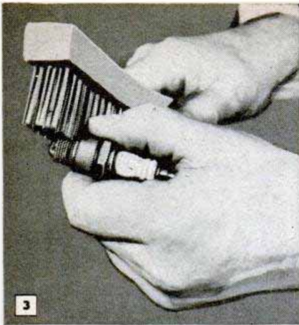
3 Clean the threads of the shell thoroughly. Carbon deposits here will retard dissipation of heat
