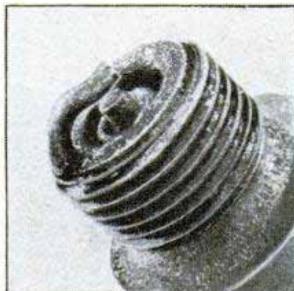
Plug has been running too cool. Shell, electrodes and insulator are fouled with hard carbon deposits
