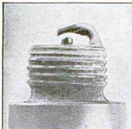
This happens when a plug runs too hot. Undue wear of the electrodes shows in comparatively short time
