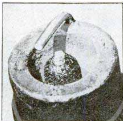
According to reliable tests, plugs in this condition may waste as much as one gallon of fuel in ten
