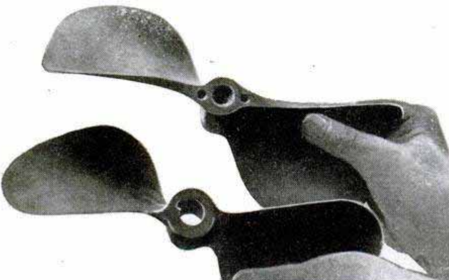
"Cleaver" propeller of new design (top) compared with conventional blade
