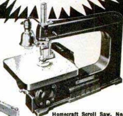
Homecraft Scroll Saw, No. 40-110 — Cuts up to 2" thick, to center of 32" panel. Has speed of 1275 cutting strokes per minute. Table tilts 45° right, 15° left..... $29 95
