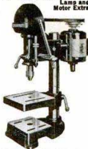
Homecraft Drill Press, No. 11-120 — Four speeds from 700 r.p.m. to 4700 r.p.m. Has capacity up to ½" holes in cast iron. Oil-impregnated bronze bearings in quill. Ball-thrust bearing in spindle pulley..... $41 95
