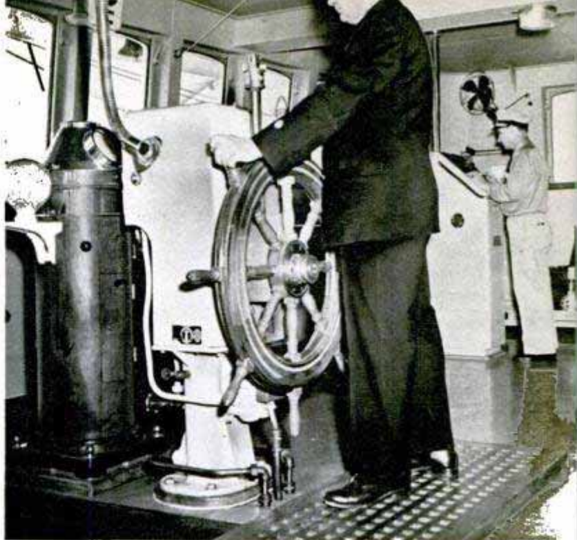
Left, speed and direction of movement of propellers are regulated at this main propulsion control board. Right, quartermaster operates hand steering gear as ship nears harbor. Officer (rear) watches radar screen
