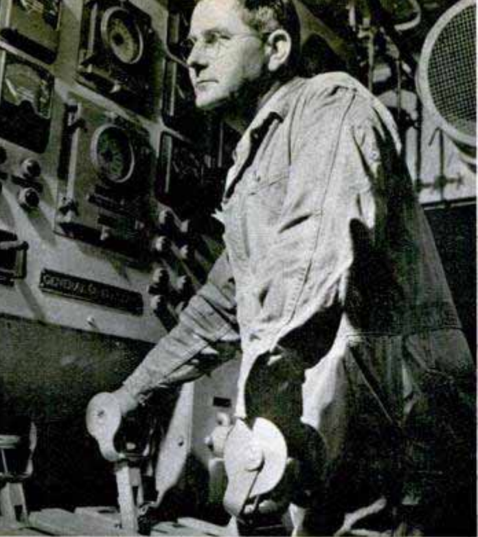
Left, speed and direction of movement of propellers are regulated at this main propulsion control board. Right, quartermaster operates hand steering gear as ship nears harbor. Officer (rear) watches radar screen
