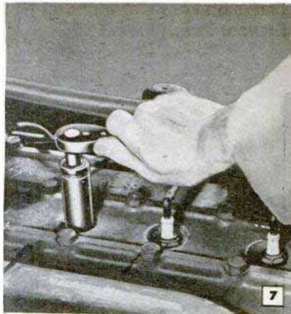
When removing or tightening plugs, use a socket wrench. Other wrenches may burr the hex section
