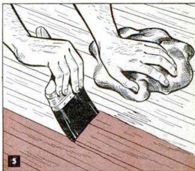
Some finishers apply the filler with the grain as shown; others insist that it is better to apply it across the grain, as this method promotes greater absorption
