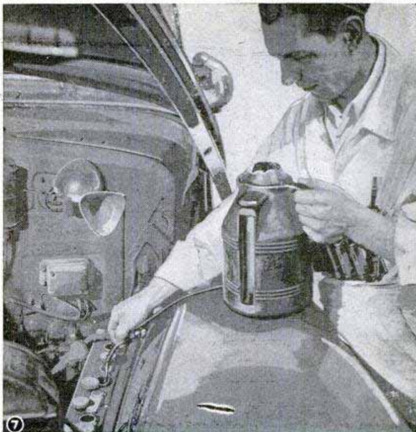
Keep the water level in your battery about \frac{3}{8} in. above the top of the plates and use only pure distilled water. Do not overfill
