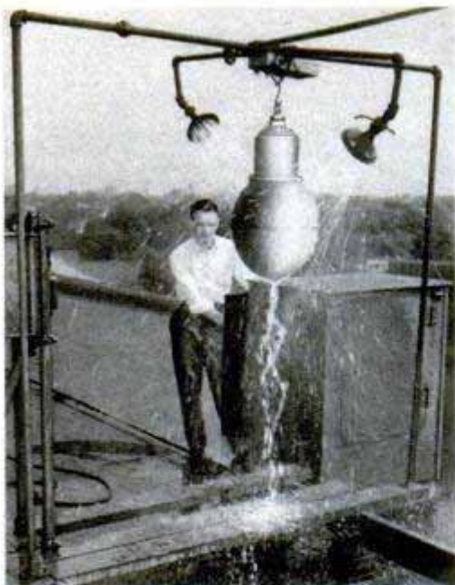
Street lights have to operate during all kinds of weather. A new model is tested for waterproofing under roof-top shower
