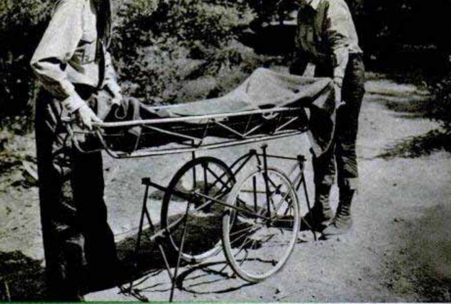
Light stretcher dolly, above, designed at Yosemite to carry sick or injured. Loaded, it can easily be lifted over rocks and depressions by two men, where six were formerly required
