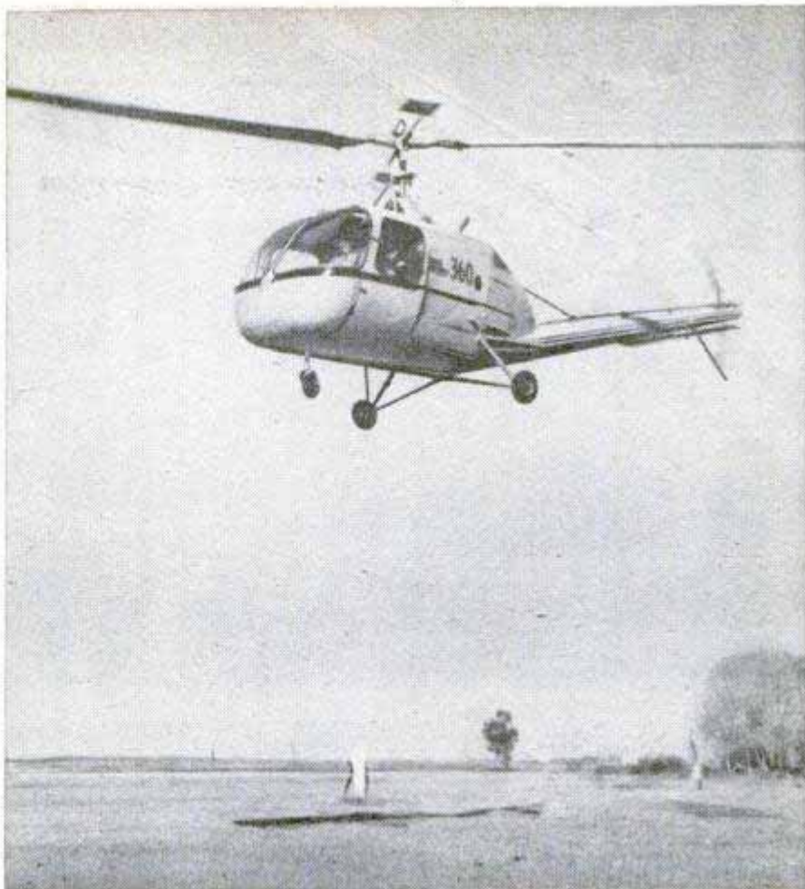
First helicopter using the simplified control system is Hiller's 360 model, above. Less than a pound of pressure on the control stick guides the craft. Below, close-up of the rotor head. In contrast to the several hundred moving parts of other systems, this method involves only seven
