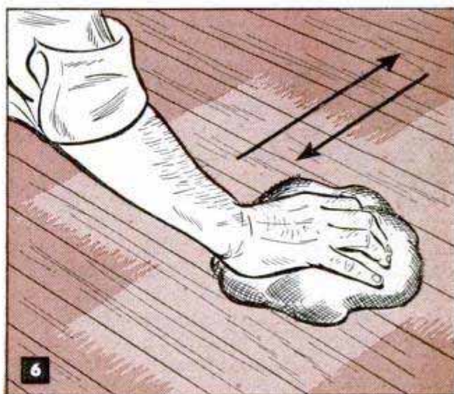
Filler should always be rubbed in across the grain with a coarse cloth. Double the cloth several times to make a soft pad which will pick up excess material
