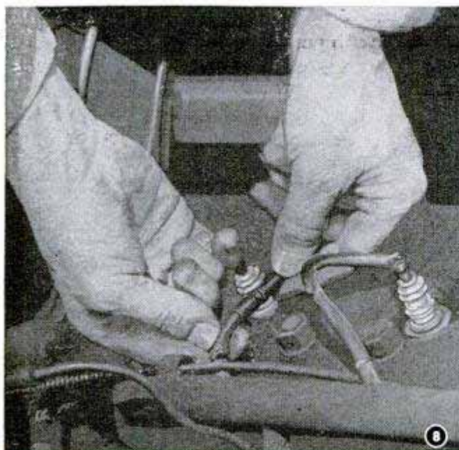
Ignition wires should be examined periodically to see that there are no bare or frayed spots
