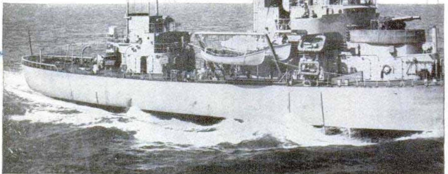
Chart shows currents which propel icebergs from Greenland into the shipping paths. Below, Coast Guard cutter Mendota has cruising range of 10,805 miles at 11 knots. Its motor is turbine-electric
