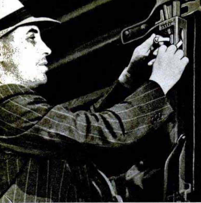
Lt. C. J. Buttimer of the Illinois Central police placing seal on freight-car door. This seal consists of a loop made of a metal strip and must be broken to open door. If cargo is particularly valuable, latch (above) is "hog tied." Flat nail is pushed through the slot and one end twisted into curly pigtail effect
