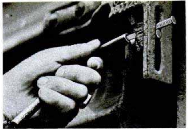
Lt. C. J. Buttimer of the Illinois Central police placing seal on freight-car door. This seal consists of a loop made of a metal strip and must be broken to open door. If cargo is particularly valuable, latch (above) is "hog tied." Flat nail is pushed through the slot and one end twisted into curly pigtail effect
