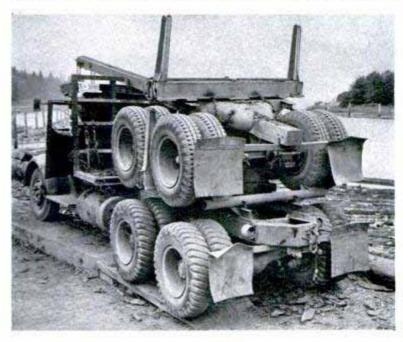
Top, stakes lock in place automatically when they are lifted. Top right, tripping bar inserted in one side releases stake on opposite side. Above, trailer rides truck on return trip
