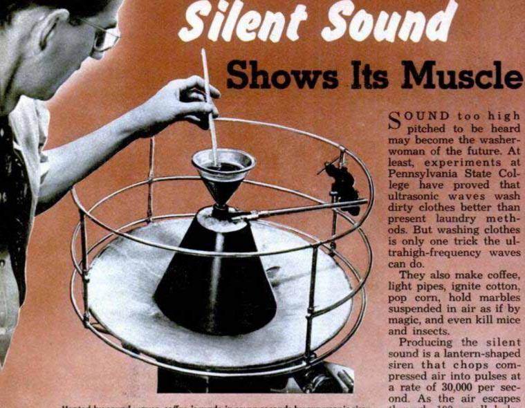
Heated by sound waves, coffee is made in seven seconds by supersonic siren
