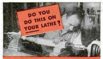
NORIZONTAL BORING ON THE LATHE . . . is easier and far more accurate than with brace and bit . . especially good when piece is too long for drill press. Extension bits and a JACOBS HEX-KEY CHUCK make deep holes easy to bore.
