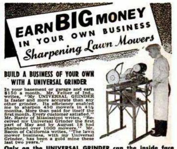
Only on the UNIVERSAL GRINDER can the inside face and edge of the stationary blade, as well as the reel blades, be ground to proper clearance
