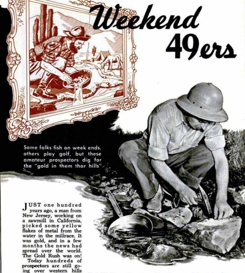
Prospector crushes white quartz before testing for gold content by swirling it in water in frying pan
