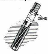
it will break, in most cases, at the groove rather than at the threaded part. When this happens, the tap can be reclaimed by grinding new wrench flats on the shank. If space permits, another groove may be ground and the tap reused a second time.
