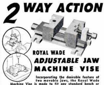
Incorporating the desirable feature of two movable jaws, the Royal Wade Machine Vise is made to fit any standard bench or floor type drill press. It serves as readily as a twojawed chuck for a machine lathe. Jaw faces measure 314" x 114" with 3" maximum opening-Weighs only 71/2 pounds.
