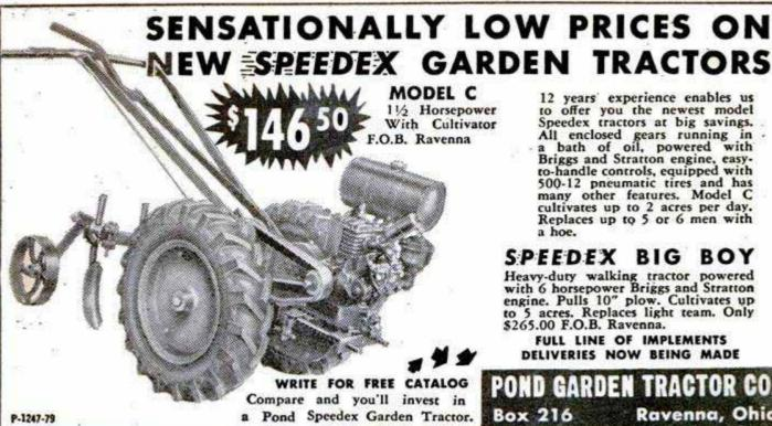
12 years experience enables us to offer you the newest model Speedex tractors at big savings. All enclosed gears running in a bath of oil, powered with Briggs and Stratton engine, easyto-handle controls, equipped with 500-12 pneumatic tires and has many other features. Model C cultivates up to 2 acres per day. Replaces up to 5 or 6 men with
