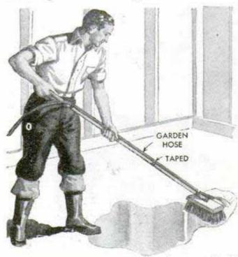
You can save time and do a better job of cleaning concrete floors in shops, farms and garages by using a floor brush like this one. It is merely a regular floor-scrubbing brush which has a garden hose taped to the handle so that the nozzle directs water in front of the brush as it is pushed over the floor.
