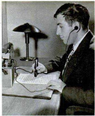
Left, a supersonic guidance device detects obstructions and warns the user by changes in earphone signals. Right, the electronic pencil "reads" printed letters and translates them into sound for the blind person
