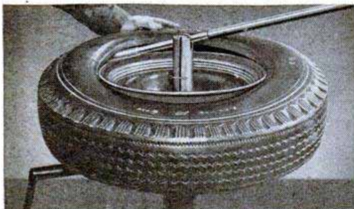
TIRE MOUNTER rolls tires onto the rim as easily as turning a crank. Bottom photo shows tire being mounted merely by turning the crank after tire is centered on the machine. Top, tire is taken off rim by inserting bar and rotating
