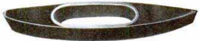
Above, steps in making hollow-blade propeller. Core at left fits inside sheet-metal-formed blades. Black sponge-rubber fill, shown in cross section at right below, prevents thin walls from "breathing." Above right, even slight distortions of blade's shape can often increase its efficiency 5 to 10 percent or more
