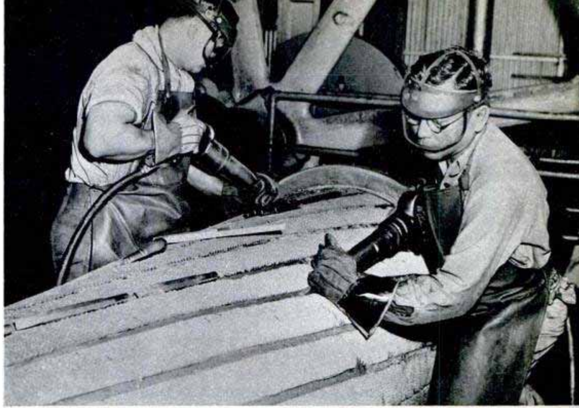
Mechanics working on one of the big rollers that squeeze juice from cane
