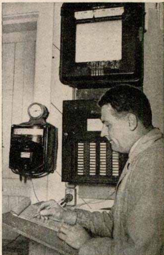
In this UCLA "hot box" Dr. Craig Taylor withstood record 262-degree heat. Many-buttoned potentiometer, below, records temperatures of parts of body
