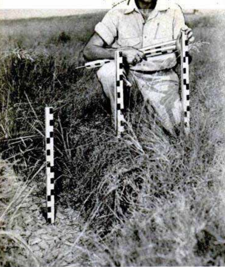
These two channels were exposed to the same flow of water, yet a gully a foot deep was scoured in the weeping lovegrass at the left, while the Bermuda grass at right shows no signs of damage from flowing water
