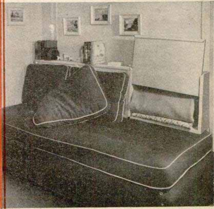
STORAGE CABINETS convert an ordinary studio couch into a comfortable sofa and also provide convenient storage space. Made of plywood, the cabinets are attached to the wall. The tops of the cabinets form an attractive shelf for books and knickknacks
