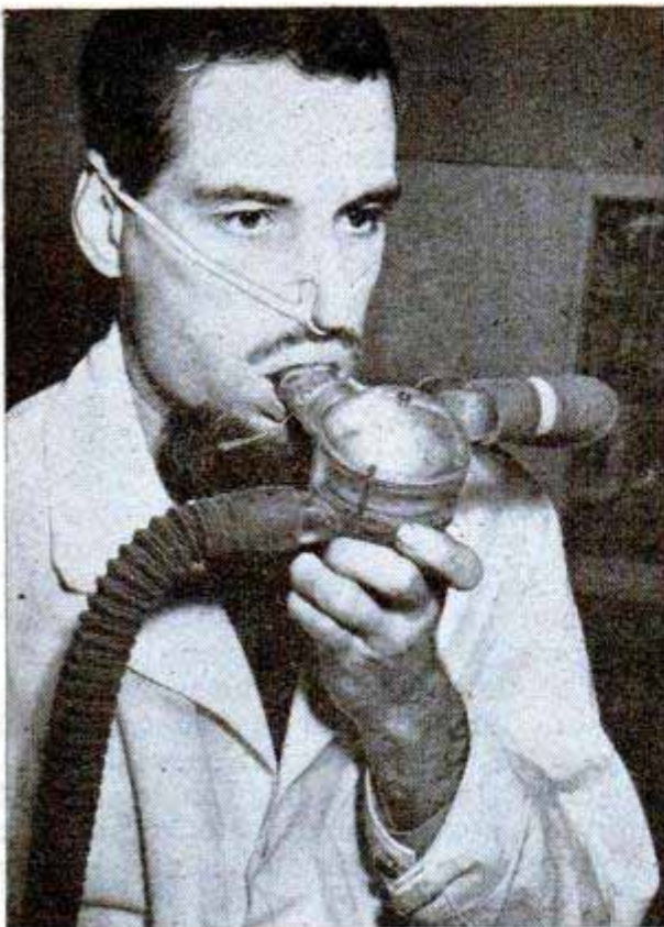
Respiration valve, left, separates exhaled and inhaled air so that volumes can be measured on meter at right
