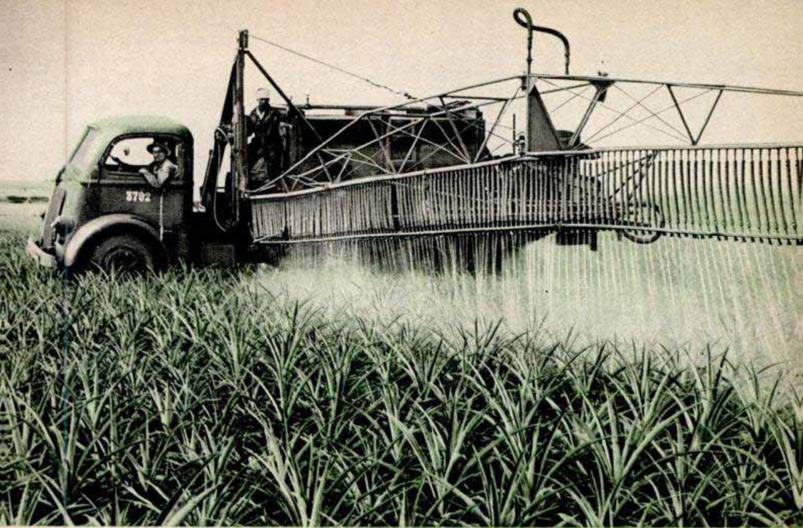
Above, boom sprayer used in pineapple fields against mealybug, which once nearly wiped out the industry. Below, machine grading pineapples according to size
