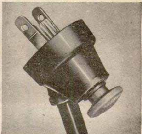
NONSLIP PLUG assures good contact and cannot be pulled out accidentally. The plunger forces wedges along the prongs
