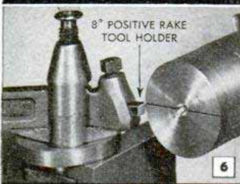
POSITIVE RAKE IS RECOMMENDED FOR LIGHT CUTTING
