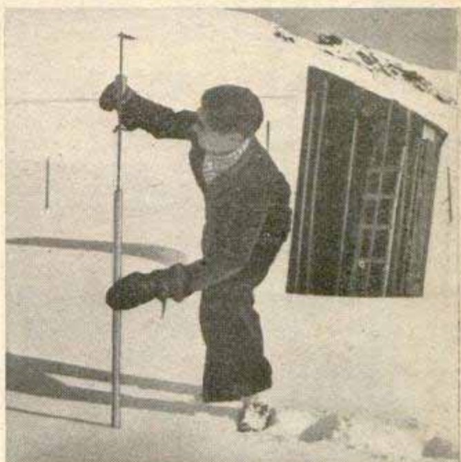
↑ Simple gauge to determine snow's water content. It helps foretell future behavior of big masses
