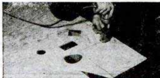
UNI-TOOL and saw attached to 1/4" 2500 RPM Electric Drill, cutting openings without necessity of drilling opening holes.
